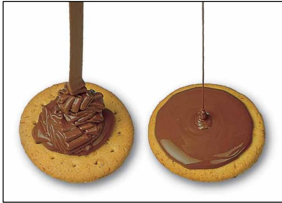
Figure 1.1: The effect of the yield value when pouring chocolate. Left-hand side – yield value: 15.0 Pa, plastic viscosity: 3.5 Pa.s. Right-hand side – yield value: 5.0 Pa, plastic viscosity: 3.5 Pa.s (Palsgaard, Denmark).
