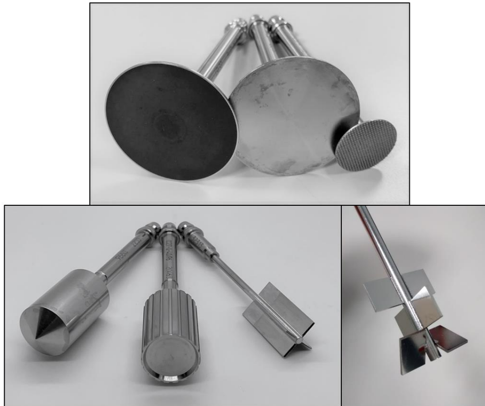
Figure 1.11: Photos of some measuring systems (MS). The top photo shows two 50 mm diameter cone MS and one 25 mm diameter plate MS. The left-hand geometry has a black coating that means it can be used for Tru-Gap measurements – the rheometer can adjust the gap during extreme temperature ramp measurements to ensure that the gap remains the same even if the metal expands. The middle cone has a smooth surface, and the 25 mm plate is serrated. The bottom left photo shows a smooth bob, serrated bob and the vane. The bottom right photo shows a starch stirrer.
