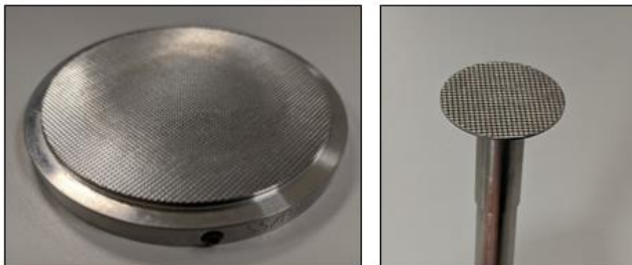
Figure 6.2: Serrated parallel-plate geometry used in the small sample volume protocol. These were: Top plate (PP25/P2: Diameter 24.948 mm) with a serrated bottom plate (SS/P2) attached to a Tru-Gap Peltier plate (P-PTD200/62/TG).
