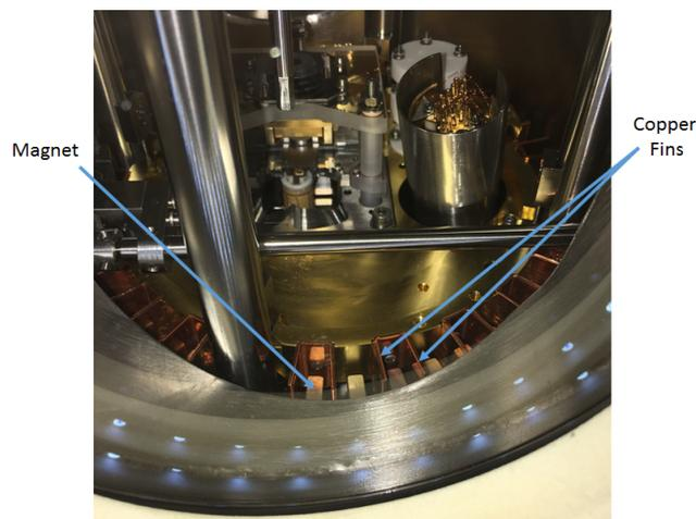
*Figure 2.14: Photograph of the scan head including the copper fins*
