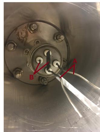
(b) **A**: The wires through which a current is passed to heat the crucible in the K-cell. **B**: The probes of a thermocouple allowing for the temperature of the deposition source to be monitored.
