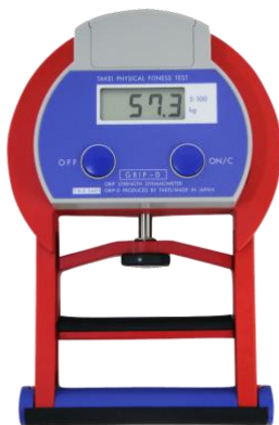
Figure 3.6: A Takei digital handgrip dynamometer (GRIP-D, measuring range 0 – 500kg, produced by Takei, made in Japan) used to in this study.
