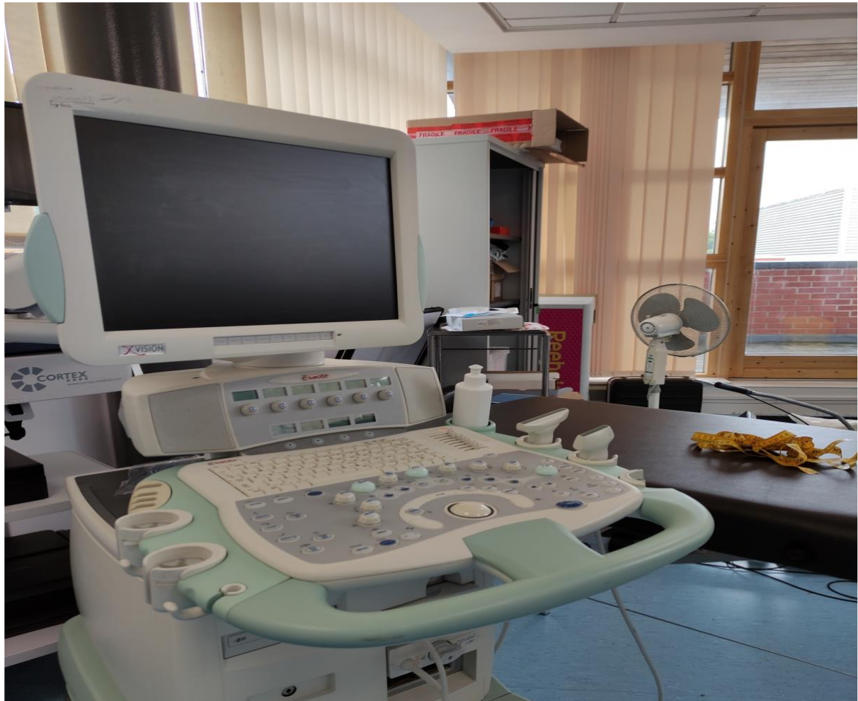
Figure 3.3. This picture shows the USS machine, the Mylab 70 (Esaote Biomedica) with a 10-15mHz, 100mm, linear array probe (Esaote Biomedica, Modle: 9600184000), used for assessing muscle architecture.
