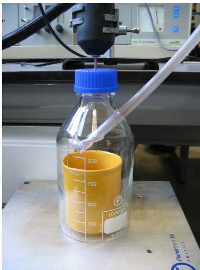
Figure 2-2 – Schematic diagram of tea infusion headspace sampling apparatus
