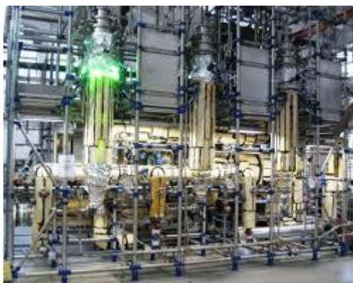
**Figure 9: Sanofi's photochemical Artemisinin production plant in Italy.<sup>27</sup> From the image it is possible to observe the photochemical section of the reactor (top left). Using this manufacturing facility Sanofi were able to produce 60 tons of Artemisinin (average batch sizes of 370 kg) in 2014. This crystalline product was of sufficient quality to meet purity requirements of a drug and did not need any further purification.**
