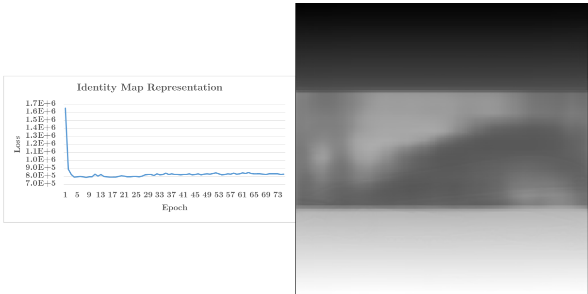
Figure 6.3: This figure shows the network’s prediction of the images in Figure 6.2. It shows that the output had three distinct bands of predicted labels. This pattern was present in all predictions. Additionally, the central band did not resemble the input image.
