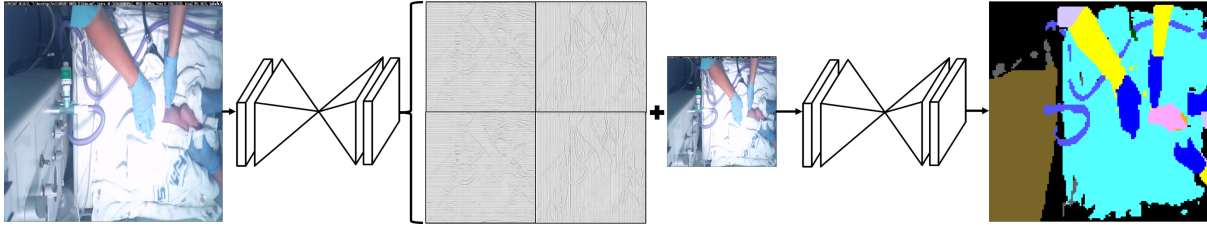
Figure 7.5: This figure shows the network structure that each of the pipelines in this Chapter use. It takes an RGB image as input and first passes through the superpixel generator hourglass sub-network. The first sub-network predicts the four MCGs that represent the deep learned superpixel, one for each direction. Then the deep-learned superpixels output plus the original RGB image are piped directly into the input of the second hourglass sub-network to predict the semantic segmentation. For illustration purposes the output masks have been combined into a single RGB colour image with each class having its own colour.
