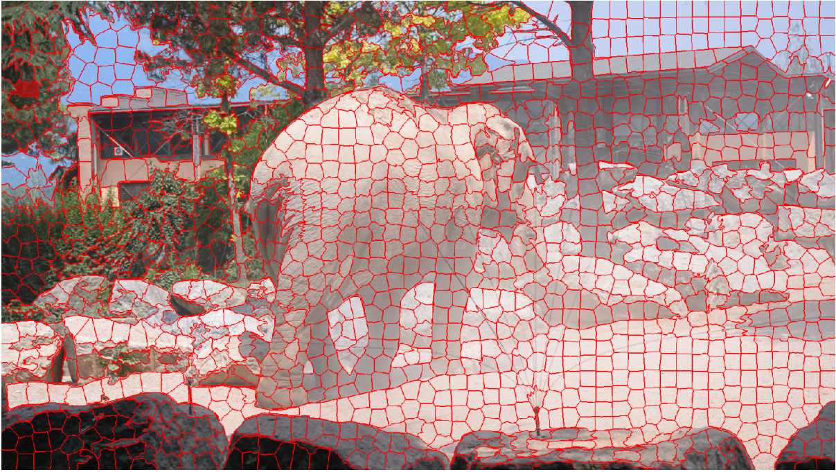
Figure 2.3: This figure shows an example of the SLIC algorithm performed on a sample from the DAVIS dataset [83]. This implementation is in Python using the scikit-image package with a target number of superpixels equal to 1500, a sigma value of 2 and a compactness value of 10. These parameters allow the algorithm to follow the structure of large objects such as the elephant and the rocks, but are less precise with smaller objects such as the foliage.
