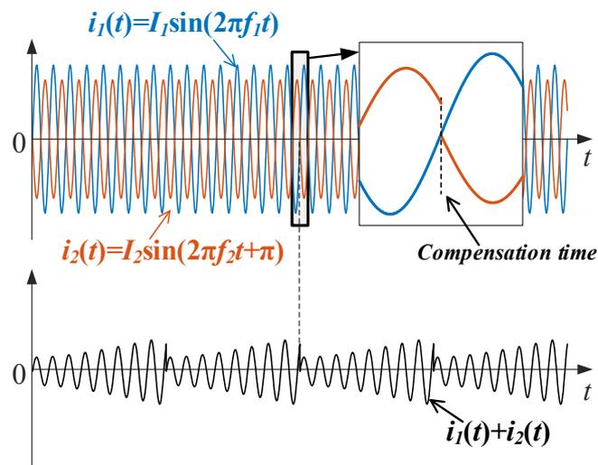
Figure 5.14: Compensation actions on accumulated errors.
