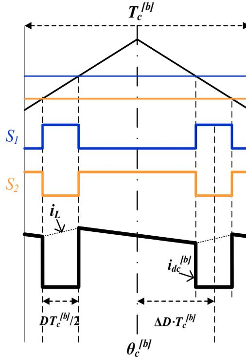
Figure 5.6: Equal-Gate-Width (EGW) PWM
