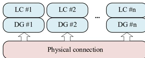
Figure 2.15: Operation principle of decentralised control.
