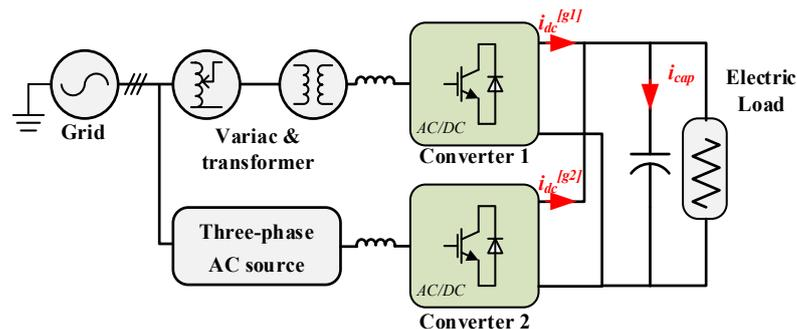
Figure 7.11: Experiment diagram of the dual-generator system under SPWM operation.
