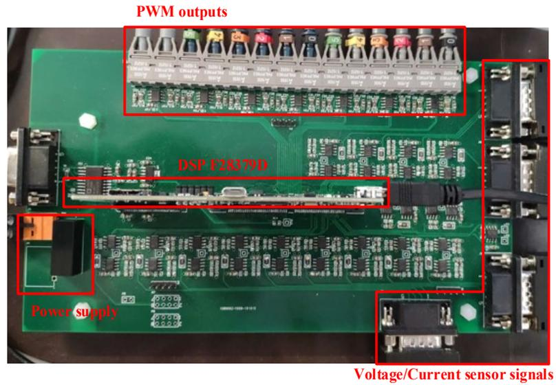
Figure 7.3: DSP Interface board.
