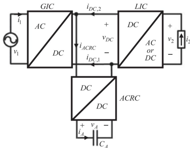
Figure 1.9: Harmonic suppression using additional switches [49].
