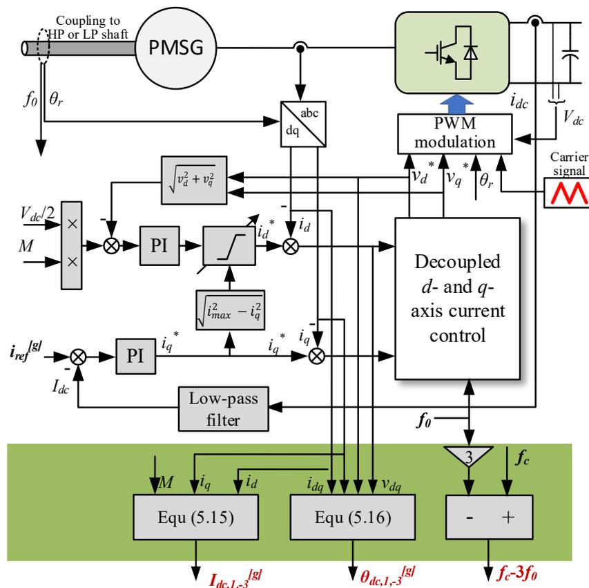
Figure 5.10: Control diagram of the PMSG system.
