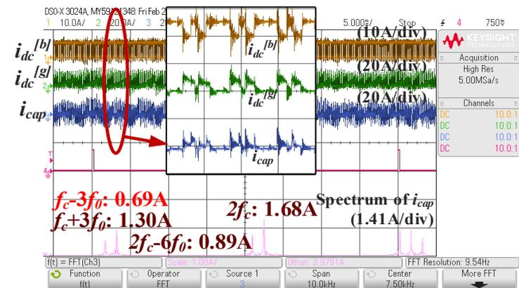
Figure 7.21: Harmonic suppression with EGW suppression when  $P^{[g]}=1\text{kW}$ ,  $P^{[b]}=1\text{kW}$ ,  $V_{\text{bat}}=180\text{V}$ .
