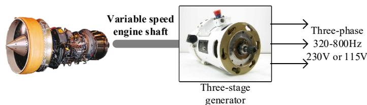
Figure 1.4: Variable speed variable frequency generation system.
