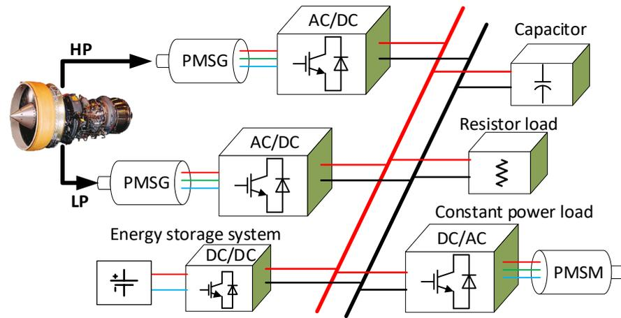
Figure 6.1: Typical dual-generation power system
