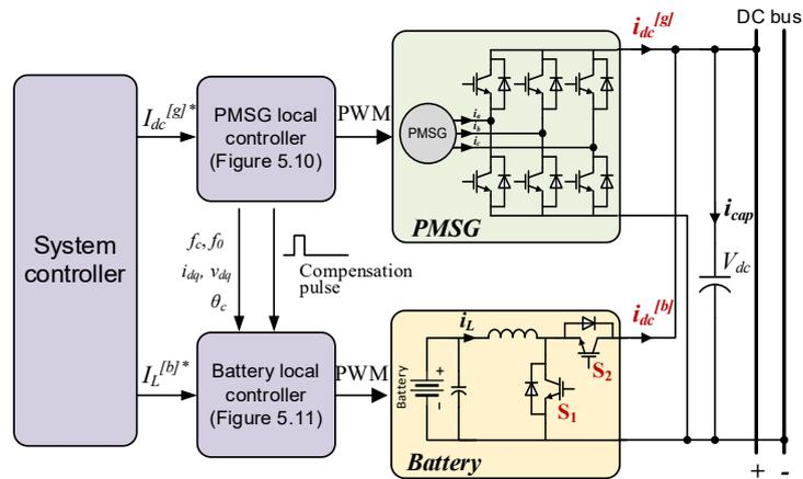
Figure 5.16: Control architecture of the hybrid generation system considering PWM compensation.
