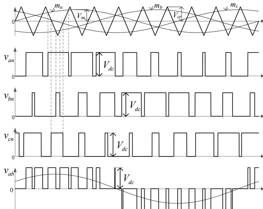
Figure 2.4: Sinusoidal pulse-width modulation (SPWM).
