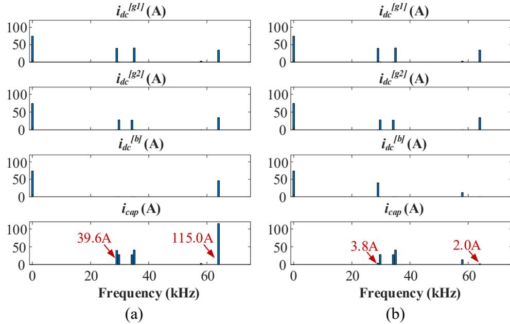
Figure 6.5: Simulation results of the spectrums. a) Without suppression. b) With suppression.
