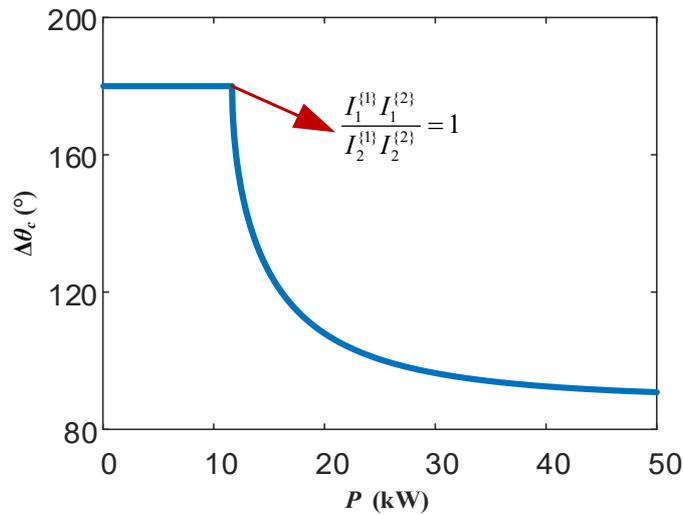
Figure 4.8: Optimised  $\Delta\theta_c$  when power sharing ratio between two converters is 1:1.
