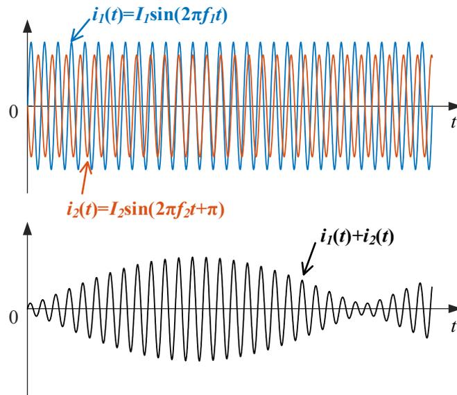
Figure 5.13: Sum up of two un-synchronised components.
