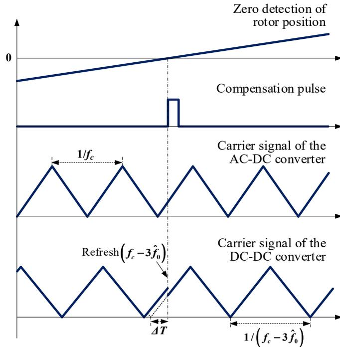
Figure 5.17: Compensation actions on carrier signals from PMSG and battery.
