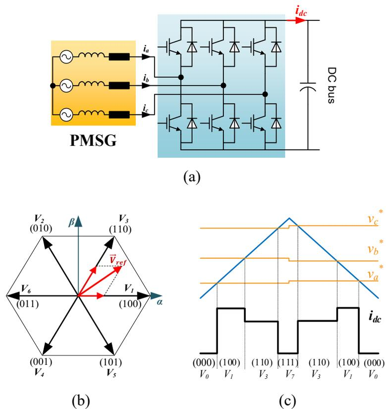
Figure 4.1: Two-level three-phase converter and SVPWM operation. a) Topology, b) Switching vectors and voltage reference, c) Modulation waveform.
