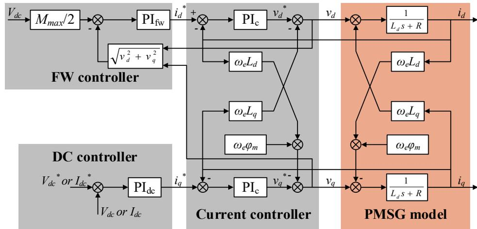
Figure 2.2: Diagram of PMSG system.
