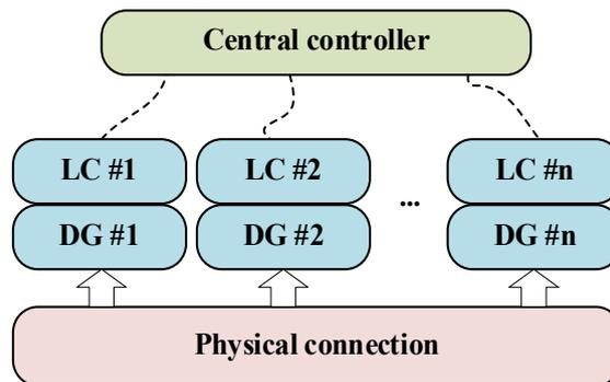
Figure 2.11: Operation principle of centralised control
