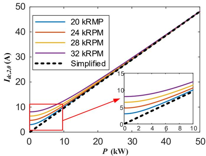
Figure 4.5: Comparison of second carrier harmonic component from accurate (4.24) and simplified (4.29) models with increased generator power and speed.
