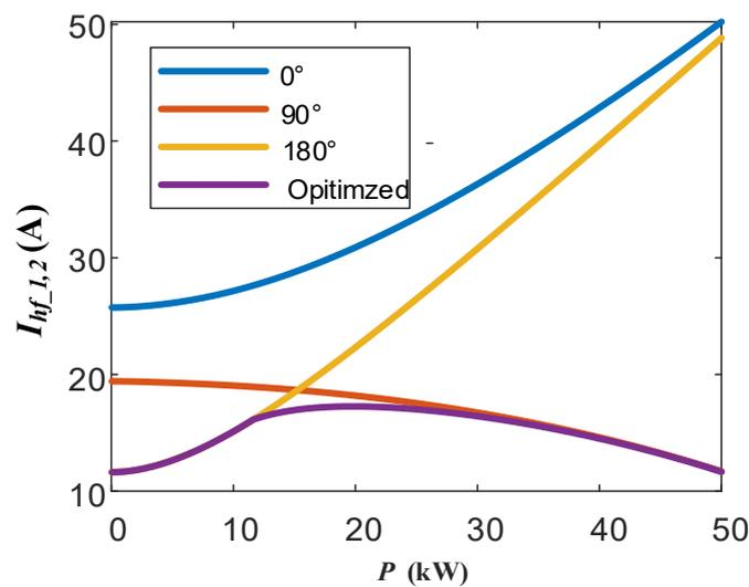
Figure 4.9:  $I_{hf\_1,2}$  versus output power of single converter.
