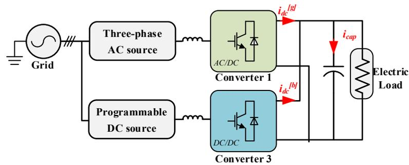
Figure 7.18: Experimental diagram when only one AC-DC converter and one DC-DC converter are involved in the system.
