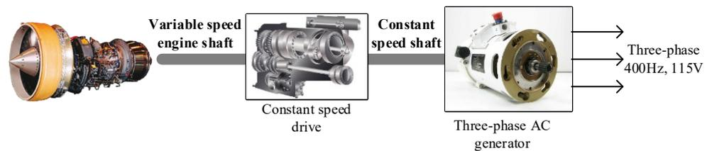
Figure 1.2: Constant speed constant frequency generation system.
