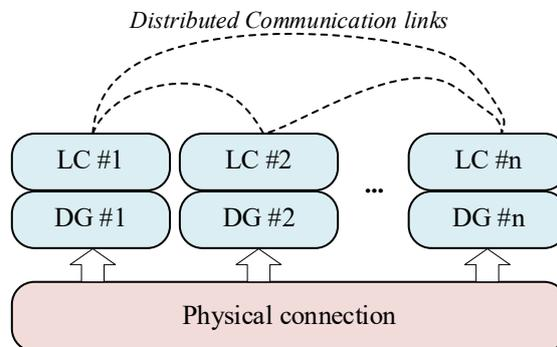
Figure 2.14: Operation principle of distributed control.
