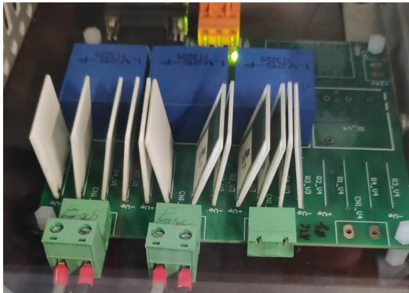
Figure 7.6: Voltage sensor board.
