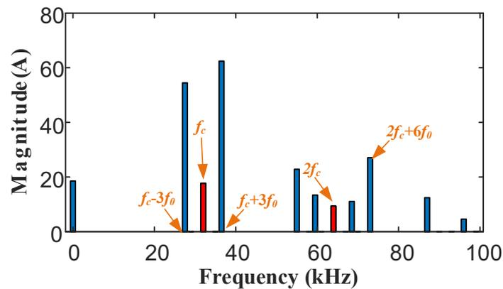
Figure 4.2:  $i_{dc}$  spectrum.
