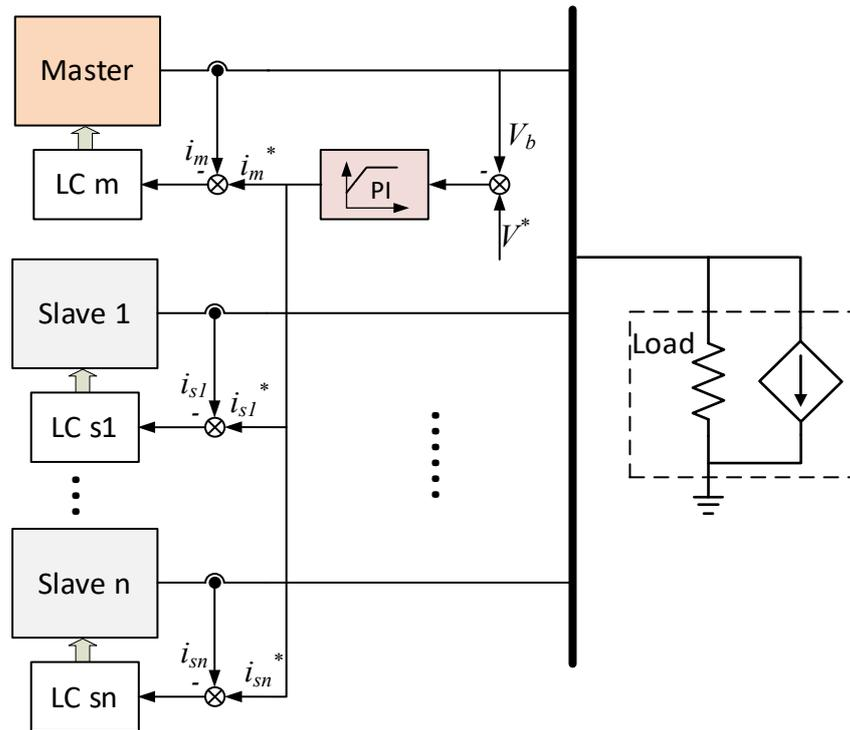
Figure 2.13: Control scheme of master-slave control.
