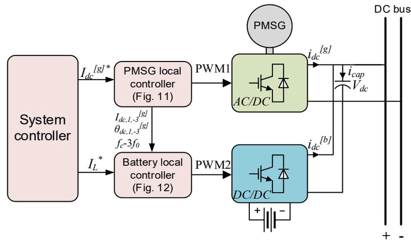
Figure 5.9: Control architecture of the hybrid generation system.
