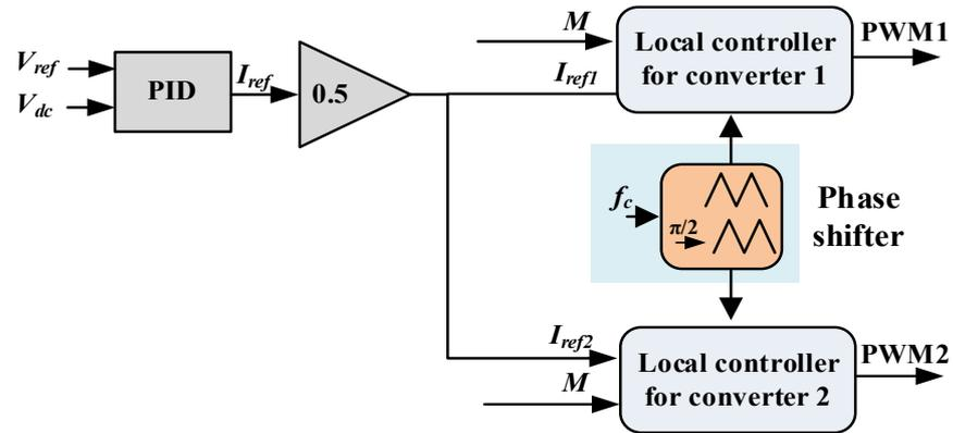
Figure 3.5: System controller when the power sharing ratio between the PMSG1 and the PMSG2 is 1:1.
