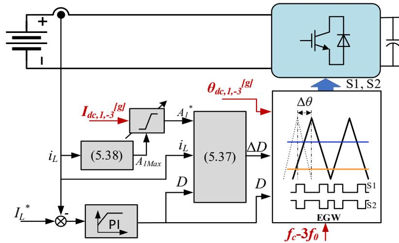
Figure 5.11: Control diagram of battery system.
