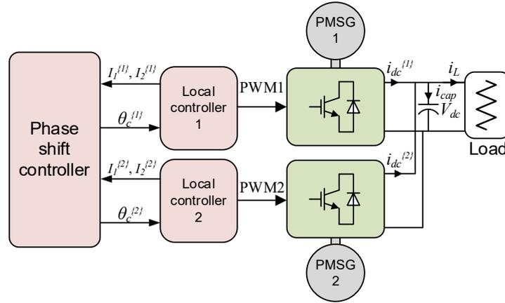
Figure 4.6: Control diagram of a dual-generator power system.
