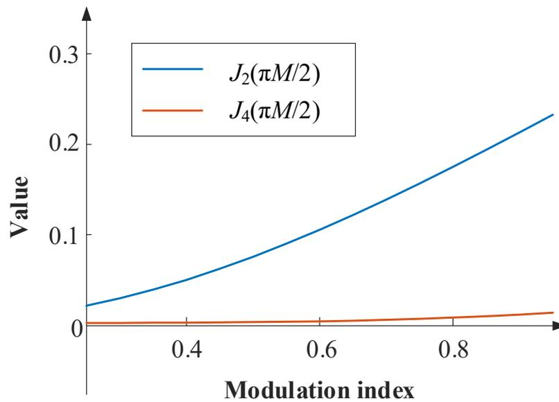
Figure 5.1: Comparison between  $J_2(\pi M/2)$  and  $J_4(\pi M/2)$  with increased modulation index.
