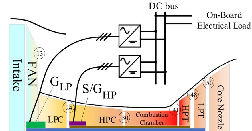
Figure 1.8: Concept diagram of the dual-channel power generation system [18].
