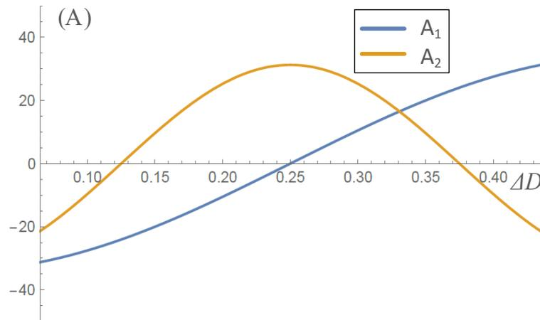
Figure 5.8: Magnitudes of the first and second carrier harmonic with  $\Delta D$  changing ( $f_c^{[b]}$  and  $2f_c^{[b]}$ ).
