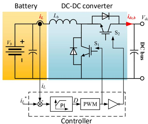
Figure 5.4: Bidirectional buck-boost converter.
