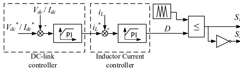
Figure 2.10: Controller of the DC-DC converter .
