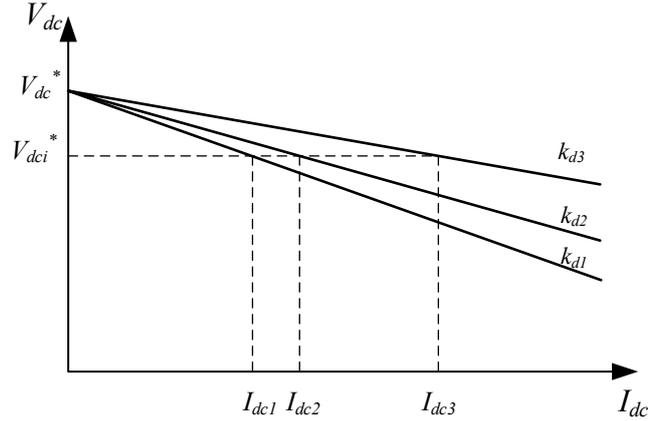
Figure 2.17: Power sharing characters of V-I droop control curve.
