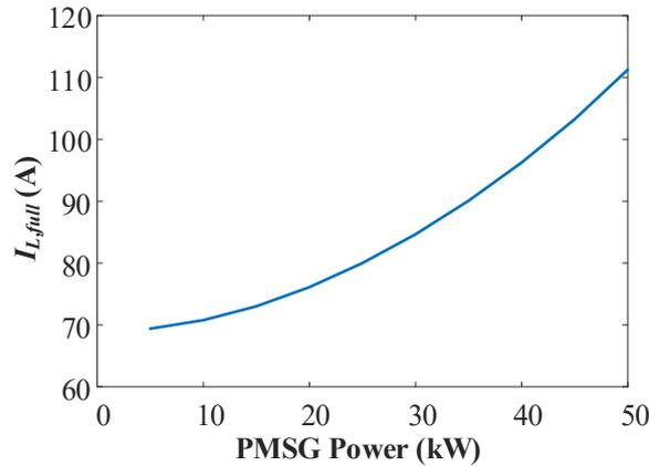
Figure 5.12:  $I_{L,full}$  when the output power of PMSG varies.
