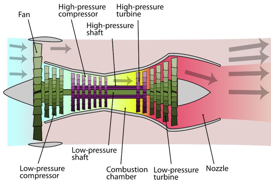
Figure 1.7: Schematic of a twin-spool, high-bypass turbofan engine.
