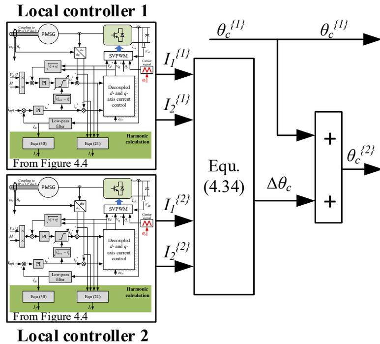
Figure 4.7: Phase-shift controller.
