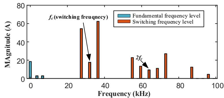
Figure 1.12: Spectrum of DC-side current.
