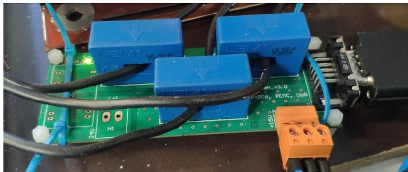
Figure 7.7: Current sensor board.
