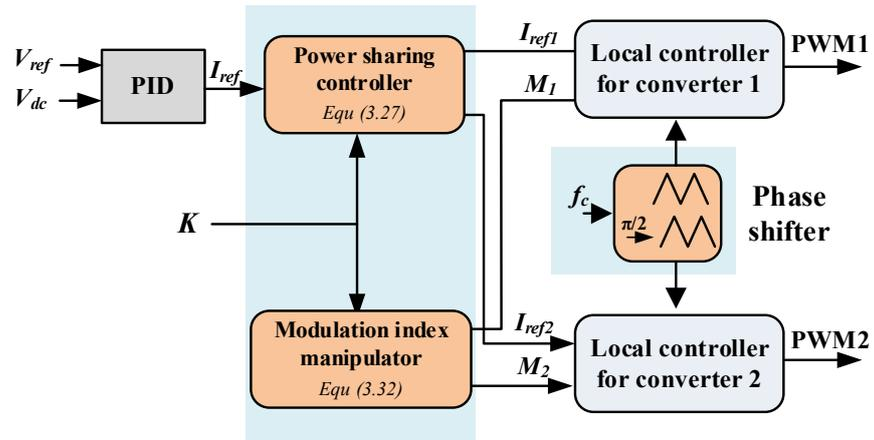
Figure 3.6: System controller when the power sharing ratio between the PMSG1 and the PMSG2 is unequal.
