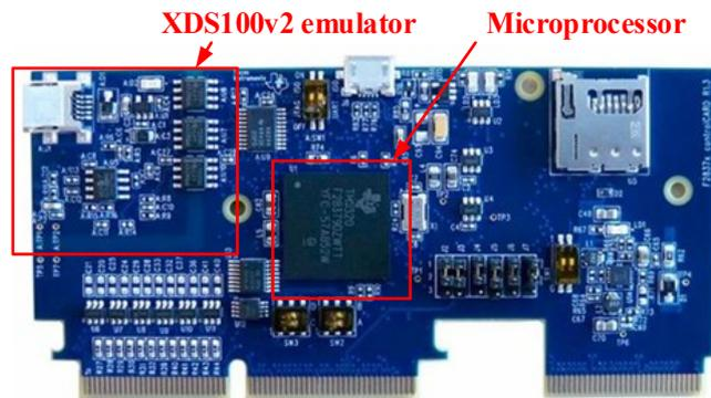
Figure 7.2: Texas Instruments F28379D controlCARD.
