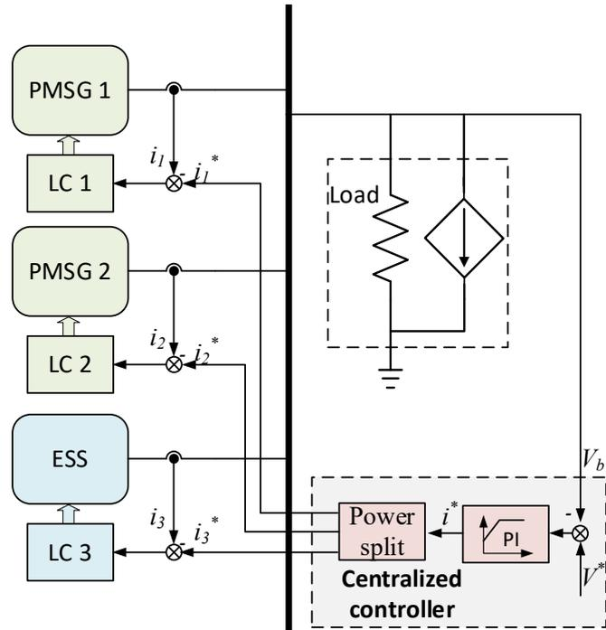
Figure 2.12: Control scheme of centralised control.
