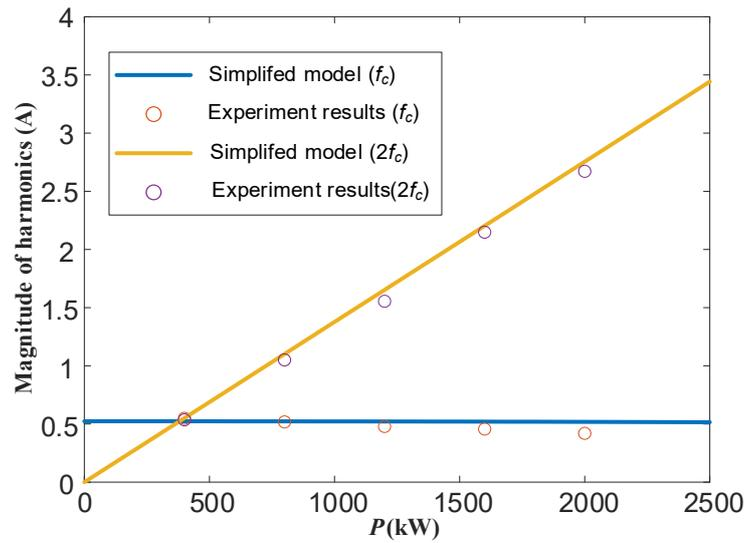
Figure 7.15: Comparison between simplified model and experiment.
