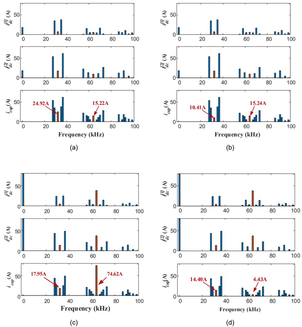
Figure 4.11: Current spectrums of  $i_{dc}^{\{1\}}$ ,  $i_{dc}^{\{2\}}$ , and  $i_{cap}$ . a) 5kW, no phase shift, b) 5kW, optimised phase shift, c) 40kW, no phase shift, d) 40kW, optimised phase shift.
