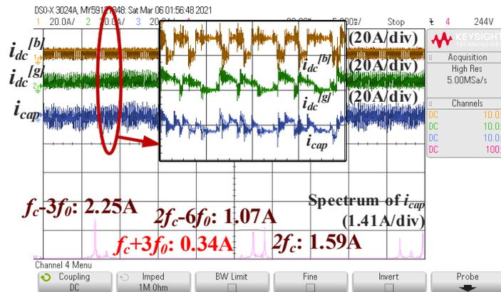
Figure 7.22: Harmonic suppression on  $f_c+3f_0$  with EGW suppression when  $P^{|g|}=1\text{kW}$ ,  $P^{|b|}=1\text{kW}$ .
