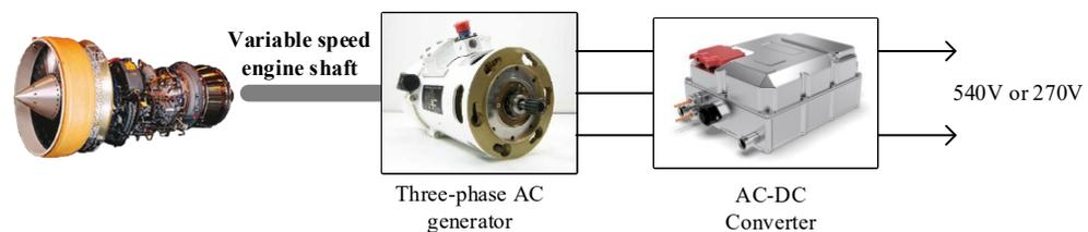
Figure 1.5: DC-voltage generation system
