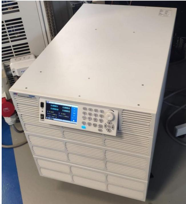
Figure 7.8: Programmable DC electronic load (EL600VDC19800W)
