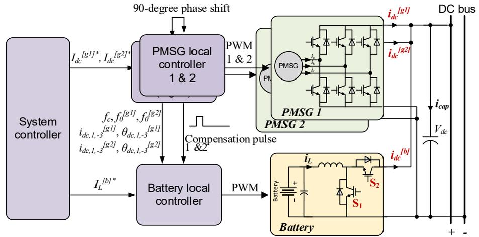
Figure 6.2: Control diagram of the dual-generator system together with a battery system.
