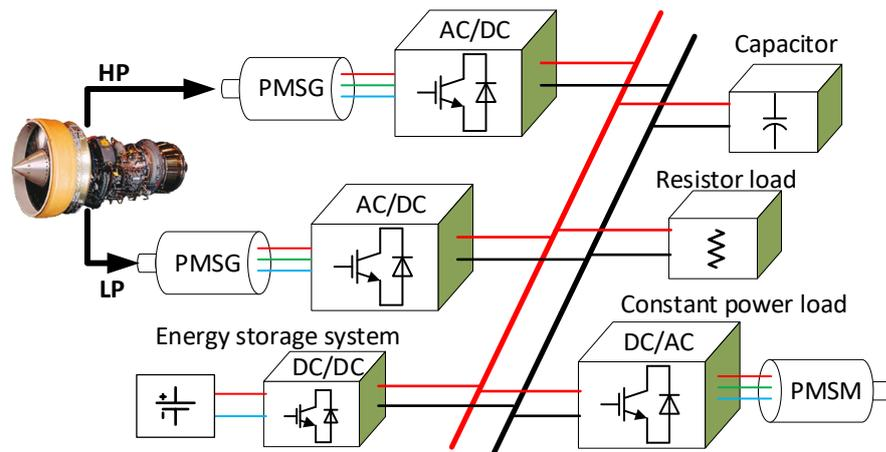
Figure 1.6: “Single bus” EPS structure.
