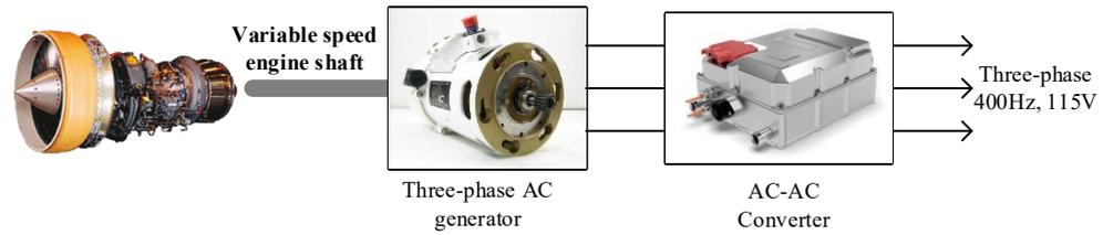
Figure 1.3: Variable speed constant frequency generation system.
