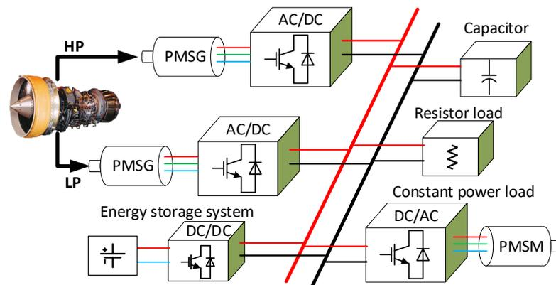
Figure 2.1: Typical dual-generation power system
