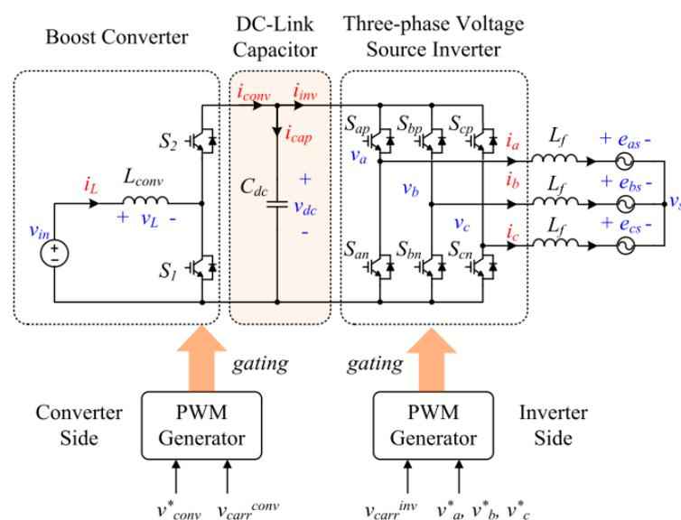
Figure 1.10: DC-DC converter connecting with a three-phase inverter [64].
