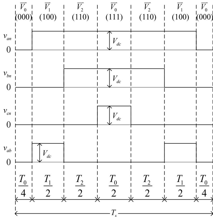
Figure 2.7: Seven-segment switching sequence in Sector I.
