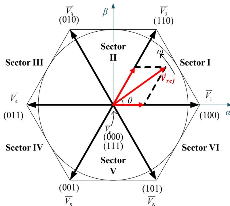
Figure 2.5: Space vector diagram for the two-level converter.
