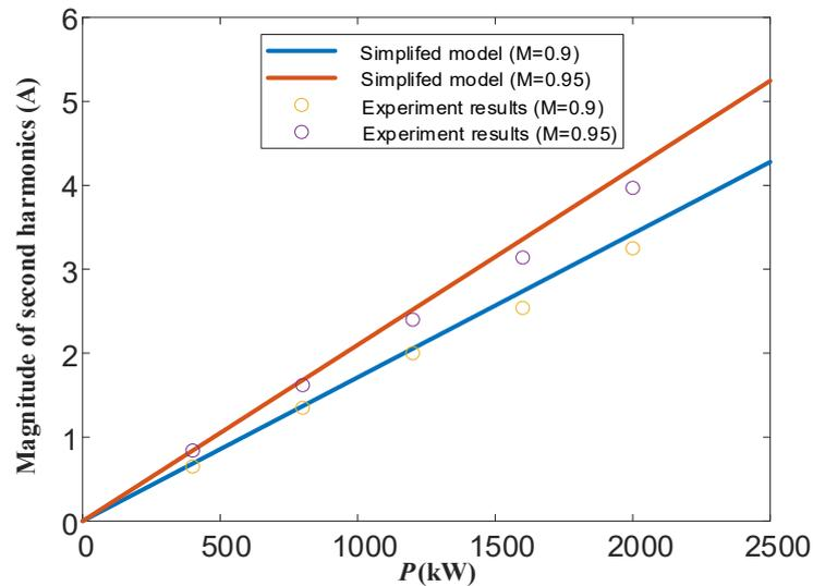
Figure 7.10: Comparison of second carrier harmonic components ( $2f_c$ ) between experiment results and simplified model.
