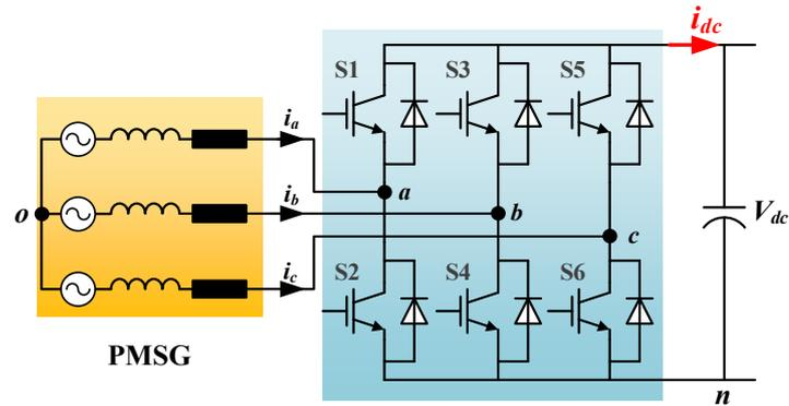
Figure 2.3: PMSG and two-level AC-DC converter.
