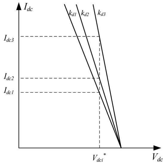
Figure 2.18: Power sharing characters of I-V droop control curve.
