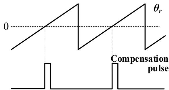
Figure 5.15: Compensation pulse generation.
