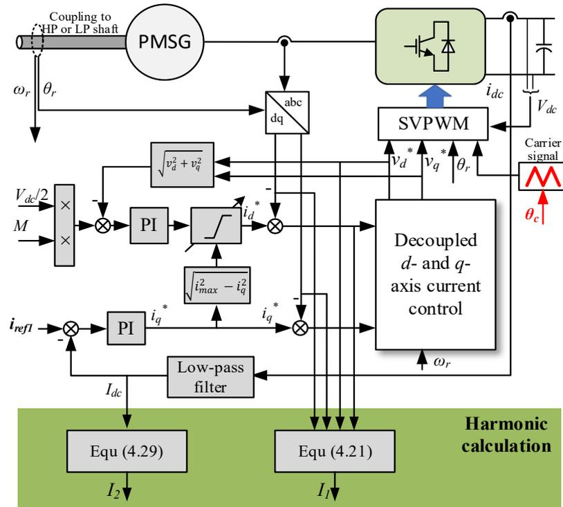
Figure 4.4: Control diagram and harmonic calculation scheme of single PMSG system.
