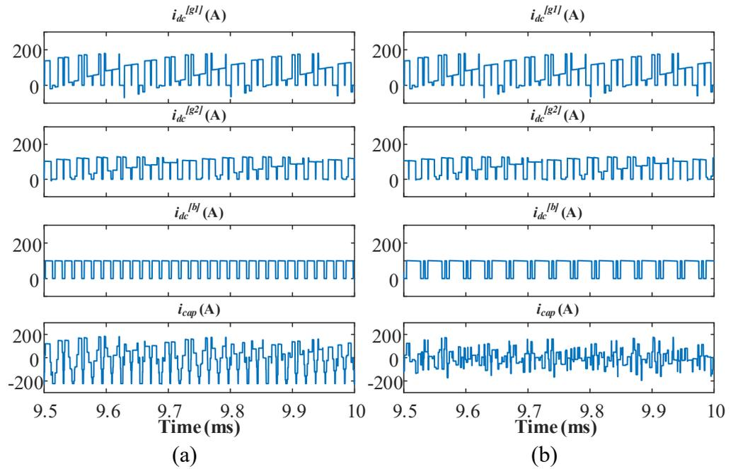
Figure 6.4: Simulation results of  $i_{dc}^{[g1]}$ ,  $i_{dc}^{[g2]}$ ,  $i_{dc}^{[b]}$ ,  $i_{cap}$ . a) Without suppression. b) With suppression.
