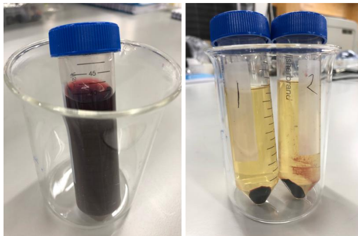
Figure 95. Photos of the crude mixture in the preparation of Ru-1 before (left) and after (right) centrifugation following the addition of excess ether, showing the yellow supernatant containing primarily symmetric hybrid POM 3 .
