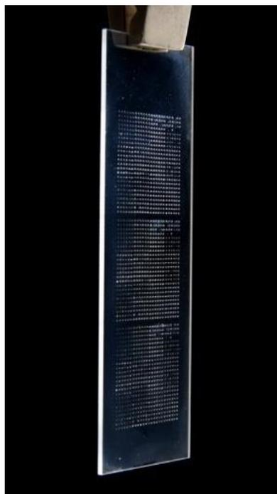
Figure 1.8 Example of a typical polymer microarray.<sup>176</sup>
