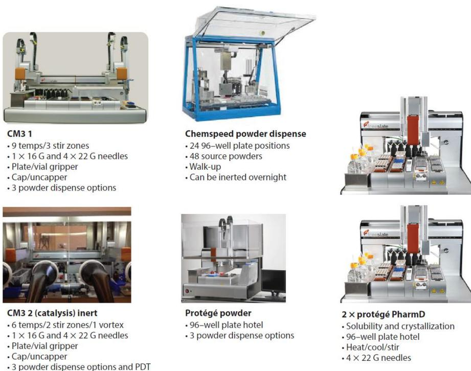
Figure 1.7 Example of automated equipment for chemical process.<sup>155</sup>
