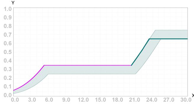
**Figure 4.3:** The fired FOU of a CIT2 FLS (shaded) and the AES with the lowest centroid value. The magenta section of the AES is obtained following the leftmost AES after the implication with the upper firing value in the firing interval, while the section in green is obtained following the leftmost AES after the implication with the lower firing value.
