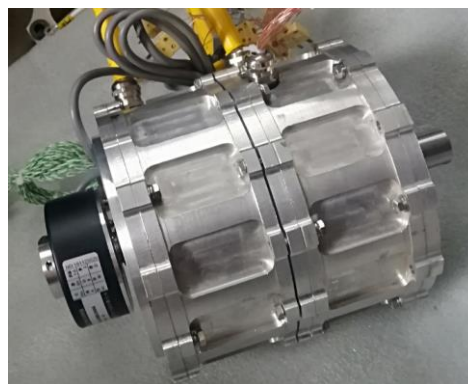
Figure 8.24 Two interconnected EMA motors assembled together
