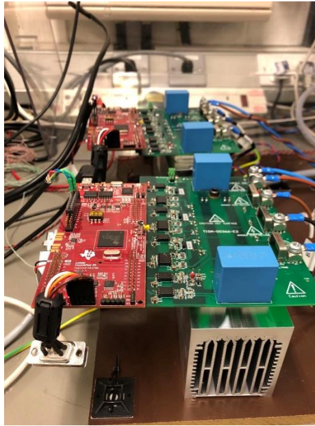
(a) Back-to-back 3-phase voltage source inverters (VSI)
