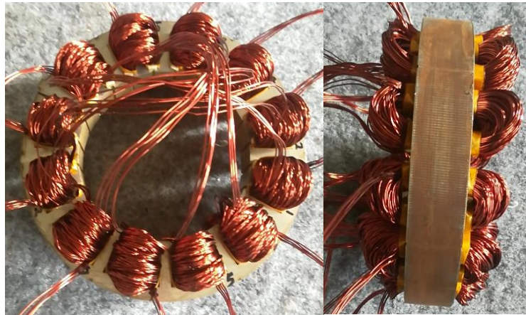
Figure 8.20 Laminated stator core with winding of the EMA motor
