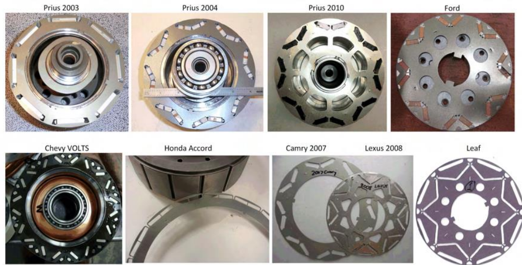
Figure 2.3 Rotor of different PM synchronous motors [24]-[27]
