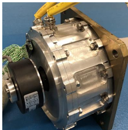
Figure 8.22 EMA motor prototype assembly
