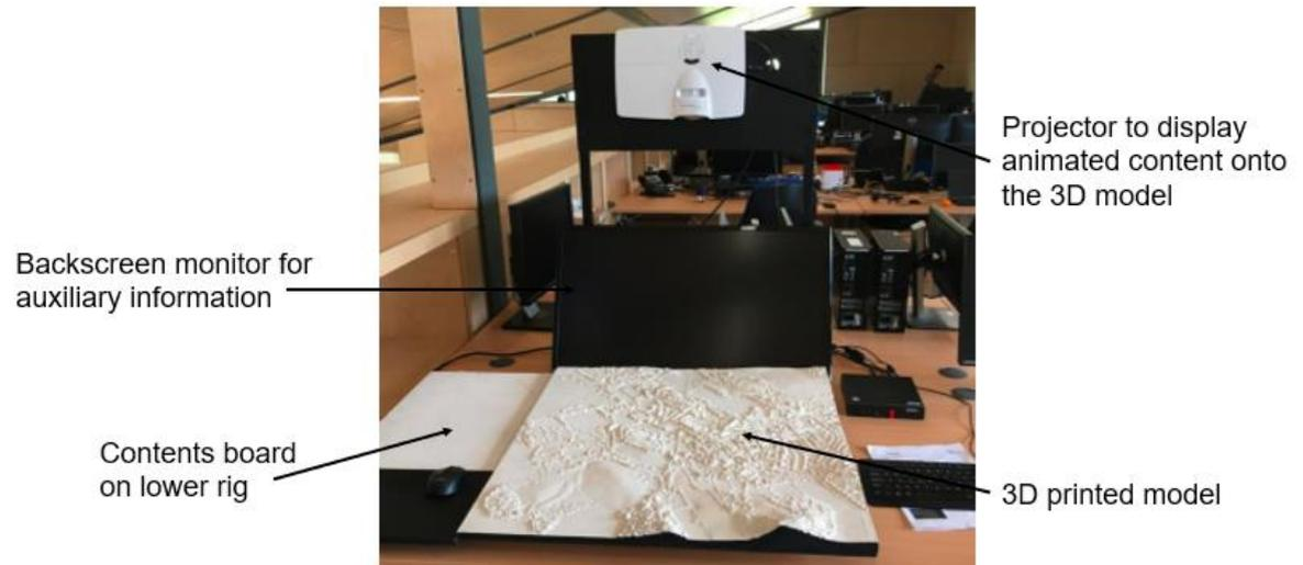
Figure 12. Annotated PARM display rig.
