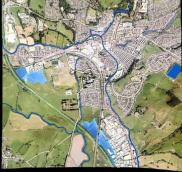
Figure 24. Section 7 – ‘Scenario Animations’. The final thematic section uses animated video to compare the extent of flooding with and without the Skipton flood alleviation scheme defences. This was included to show how the alleviation scheme has reduced flood risk.
