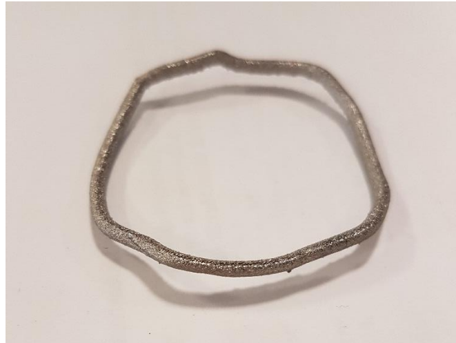
Figure 25: A bespoke annuloplasty device manufactured in Ti6Al4V using SLM, using individual patient scan data to produce CAD models (CAD shown in Figure 24)
