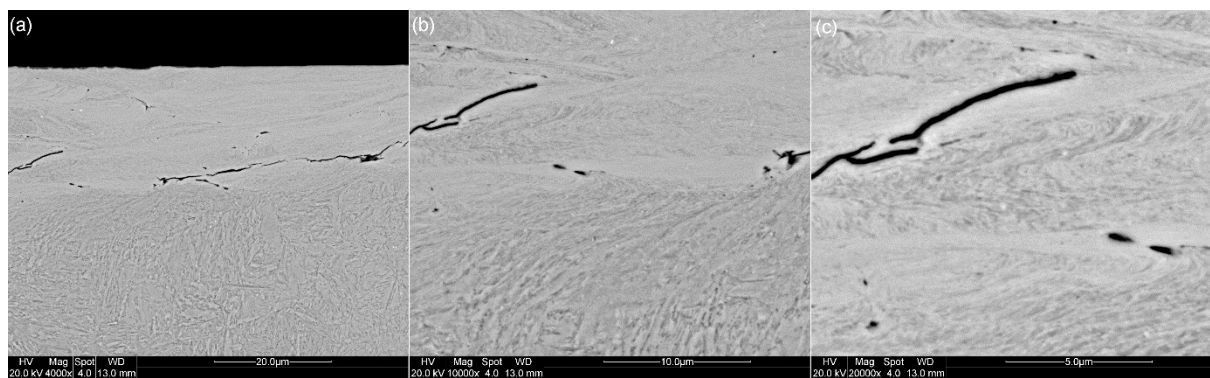
Figure 5.19. BSE SEM micrographs at increasing magnifications in cross-section of an etched cylindrical specimen after fretting at 200 Hz, showing severe deformation and cracking of the TTS layer ( \Delta^* = 50 \mu\text{m} ; P = 450 \text{ N} ; N = 10^6 cycles).
