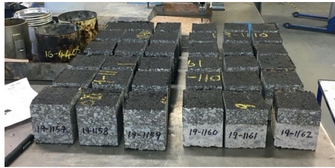
Figure 3.22. Specimens for interface shear bond test after the cut
