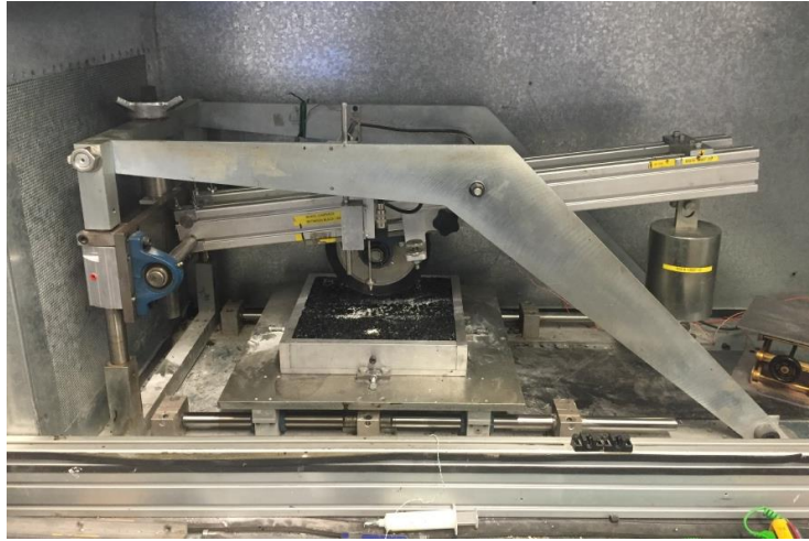
Figure 2.16 Cooper's Wheel Tracker Machine in University of Nottingham (Al-Mosawe 2016)
