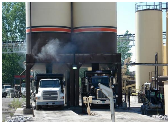
Figure 2.31 Emission demonstration of WMA (on the right) compared to HMA (the left). Photo by NAPA, 2004
