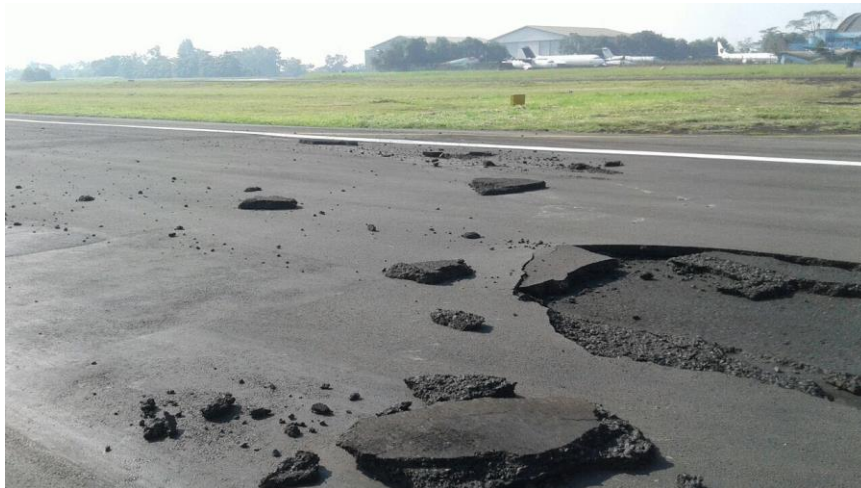
Figure 1.2 Slippage failure of newly laid asphalt overlay at HLP runway (Courtesy of Indonesia Airport Authority)
