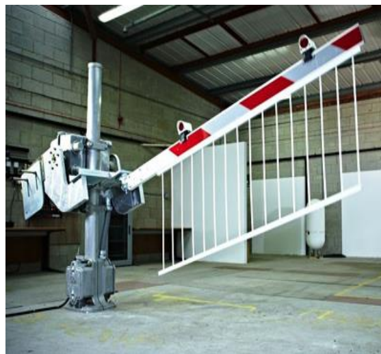
Figure 4-9 Newly Approved Level Crossing Barrier Design with Shroud Removed.
