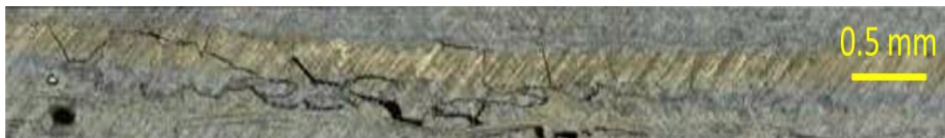
Fig. 6.12 - Magnified image of the crack in the three-point flexural RP-CNP sample
