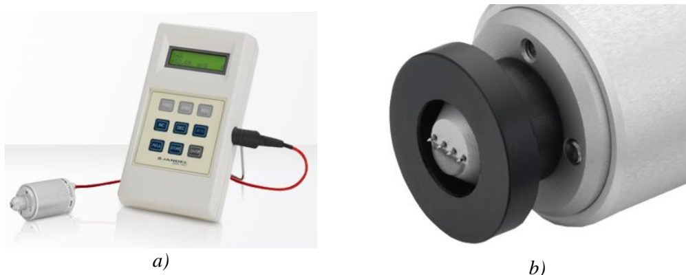
Fig. 3.18 - Jandel HM21 system (a) and head of 4-point probe (b)
