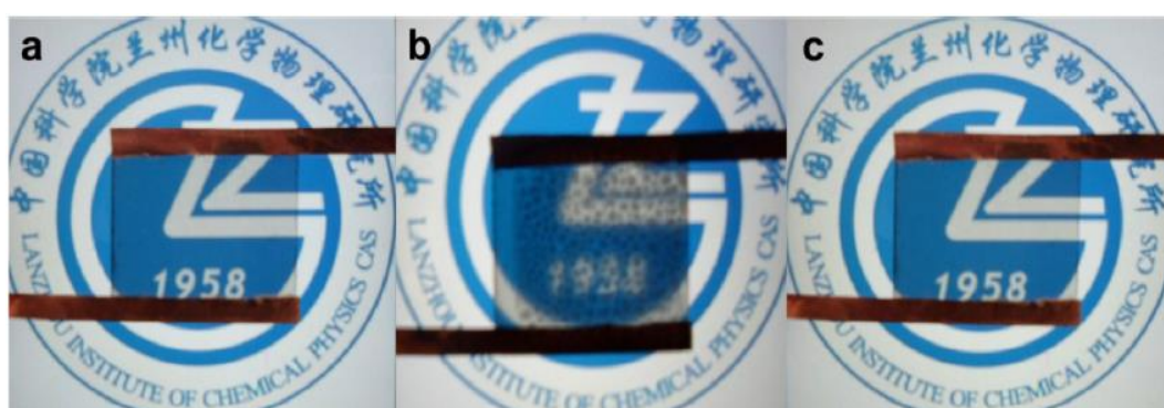
Fig. 2.26 - Defrosting test results of GO/AgNW hybrid film heater: optical photo before (a) and after (b) frost formation, and (c) after the defrosting test operated at 10 V [102]
