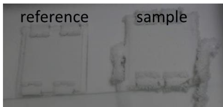
Fig. 4.10 - Ice formed on the sample surface in a cold environment ( -20^{\circ}\text{C} )
