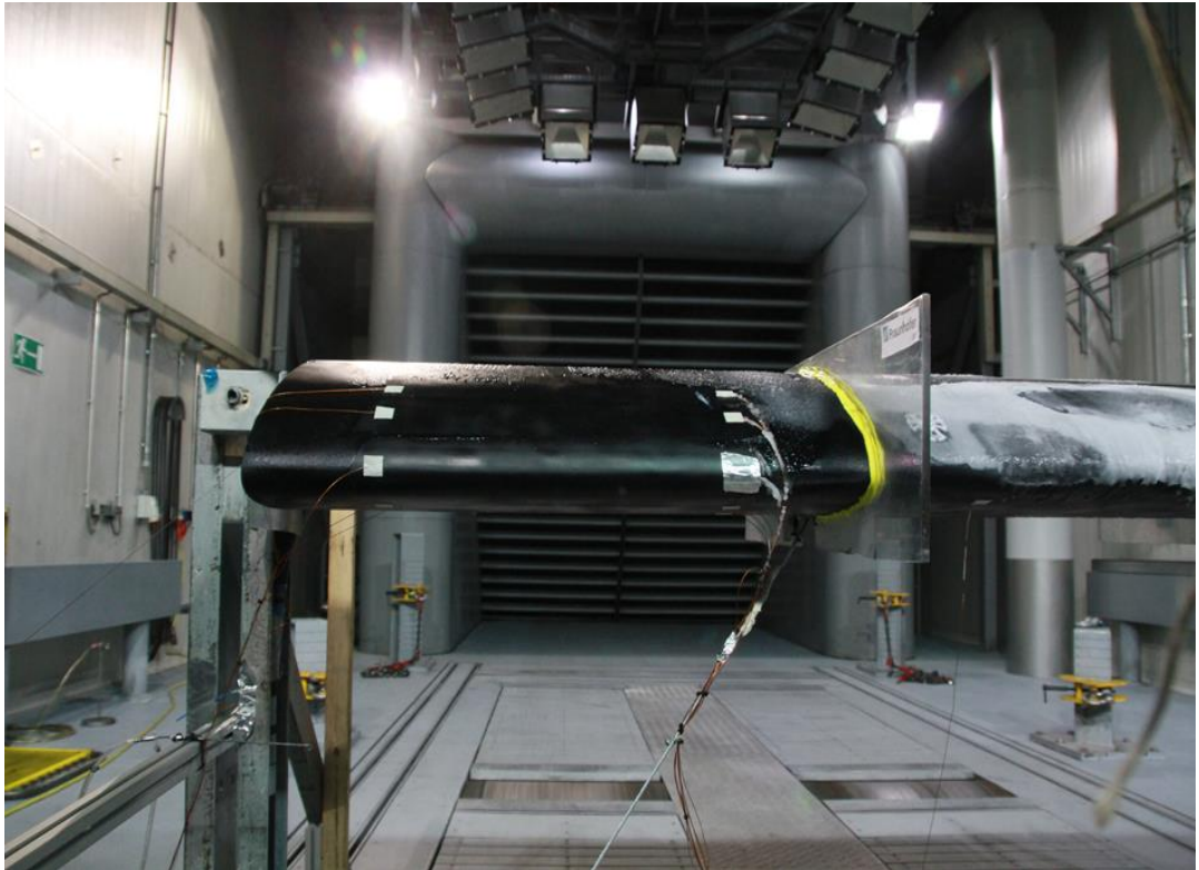
Fig. 2.35 – De-icing test with the ice protection system carbon nanotube based developed by Fraunhofer Institute for Structural Durability and System [127]
