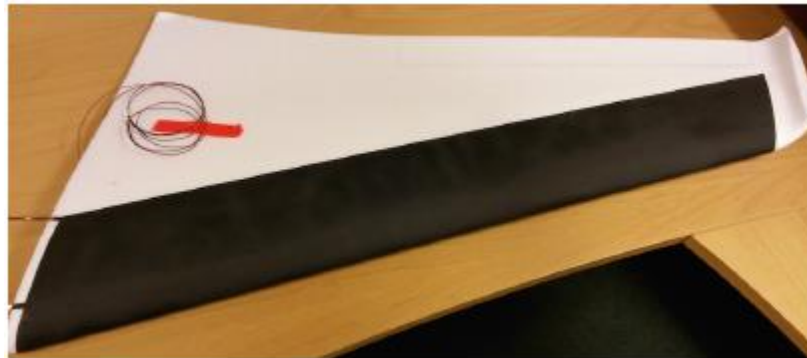
Fig. 2.30 - Wing with electro-thermal protection system [108]
