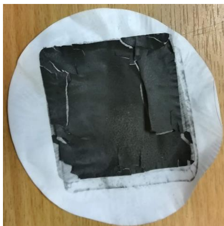
Fig. 5.20 - Example of cracked buckypaper made of AT-T-CNTs
