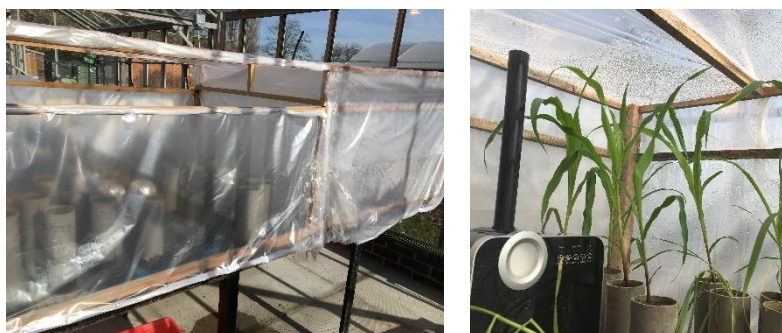
Figure 2. Custom growth chamber inside the glasshouse. Low humidity conditions maintained on the left-hand side, and high humidity on the right. Humidity was provided by a 5L ultrasonic humidifier (Nordcel, CF-2756H). Opaque plastic sheeting surrounded both sides of the chamber to ensure equal light distribution throughout the chamber.
