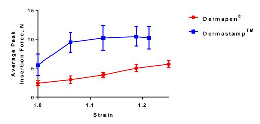
Figure 2-4 Biaxial skin strain and insertion force relationship for commercial microneedle systems Dermapen® and Dermastamp $^{TM}$ . Data expressed as means  $\pm$  SD, n=5.
