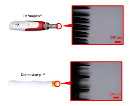
Figure 2-1 Close up microscopy image showing the geometry of microneedles from Dermapen $^{\otimes}$  and Dermastamp $^{\text{TM}}$
