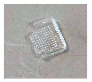
Figure S4- 4 Pyramidal PVPVA microneedle patches fabricated with PVPVA and PEG 400 for both the needle and backing layer. The backing layer shattered as it was too rigid and brittle during the demoulding step.
