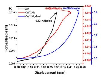
Figure 1-10 Example of a force displacement curve during a microneedle compression test. Reproduced from Zhang et al. <sup>132</sup>
