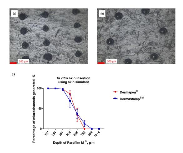
Figure 2-6 Microscopic images of first layer of Parafilm M® stack punctured by stainless steel microneedles by (a)  $Dermapen^{\otimes}$ , (b)  $Dermastamp^{TM}$  Scale bar:300  $\mu m$  (c) Insertion profile of different commercial microneedle systems,  $Dermapen^{\otimes}$  and  $Dermastamp^{TM}$  into Parafilm M® layers, data expressed as means  $\pm$  SD, n=6.
