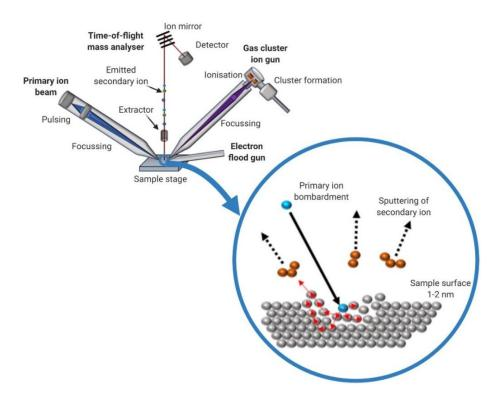
Figure 1-14 A general schematic of the ToF-SIMS instrument. The inset shows a close up of the sample analysis taking place as a result of the collision cascade (red arrows) caused by primary ion bombardment onto the sample surface. Adapted from Saleem & Galla 2010  $^{205}$
