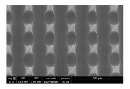
Figure 1-8 An example of a scanning electron microscopy (SEM) image of microneedle fabricated from starchgelatine. Microneedle and SEM image were prepared by the PhD candidate himself, Mr Akmal H Sabri.
