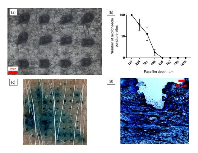
Figure 4-2 (a) Microscopic images of first Parafilm $^{\circ}$  treated by PVPVA microneedles (b) Insertion profile of PVPVA microneedle into Parafilm $^{\circ}$  layers, data is expressed as mean $\pm$  SD for n=6 (c) Microchannels created in ex vivo porcine skin visualised via the release of methylene blue from PVPVA microneedles (d) Optical microscopy image of microneedle channels created when the skin is treated with PVPVA microneedles
