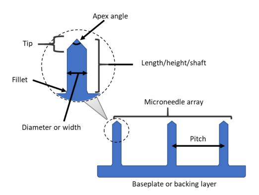
Figure 1-7 Common terminologies used in describing the architecture of a microneedle patch.
