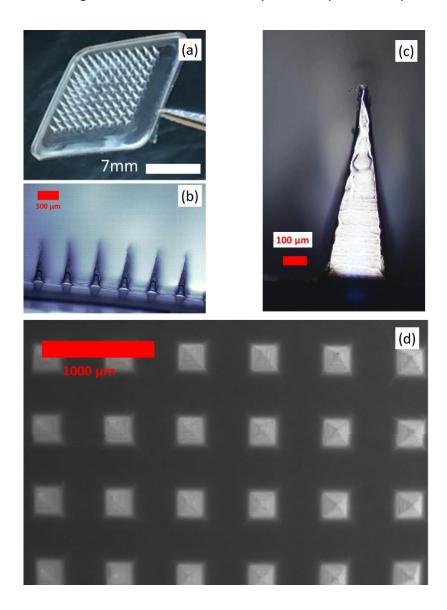
Figure 4-1a) Photograph image of PVPVA microneedles post-fabrication (b) Optical microscopy image of PVPVA microneedles at 12.5x magnification (c) close up microscopy image - of a single PVPVA polymeric microneedle at 50x magnification (d) SEM images of PVPVA microneedles at 39x magnification
