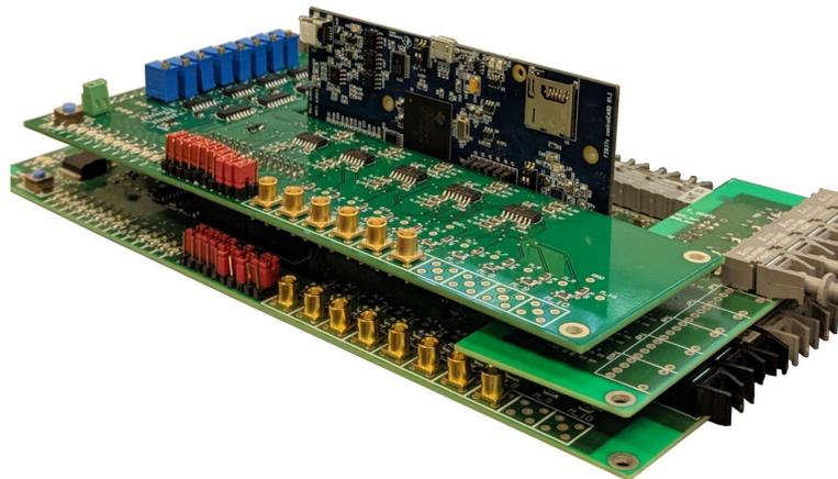
Figure 6.14: Master interface PCB with the expansion board mounted on top
