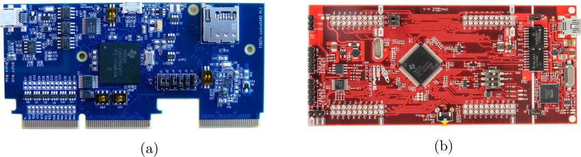
Figure 6.12: (a) TMS320F28379D controlCARD (b) LAUNCHXL-F28377S LaunchPad
