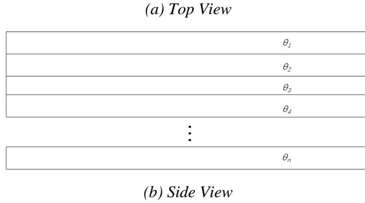
Figure 1 The structure of a composite laminate beam.
