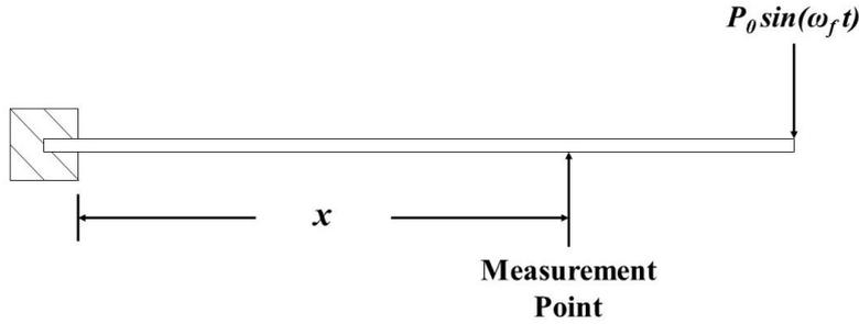
Figure 2. A composite laminate beam under a concentrated harmonic excitation.
