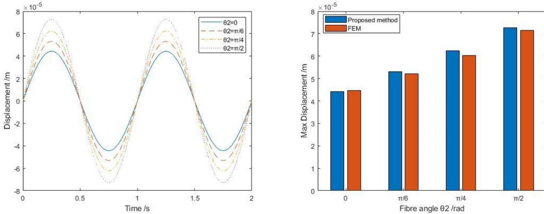
Figure 3. The forced vibration response of a composite laminate beam: (a) Time domain displacement responses. (b) Maximum displacements for different fibre angles.
