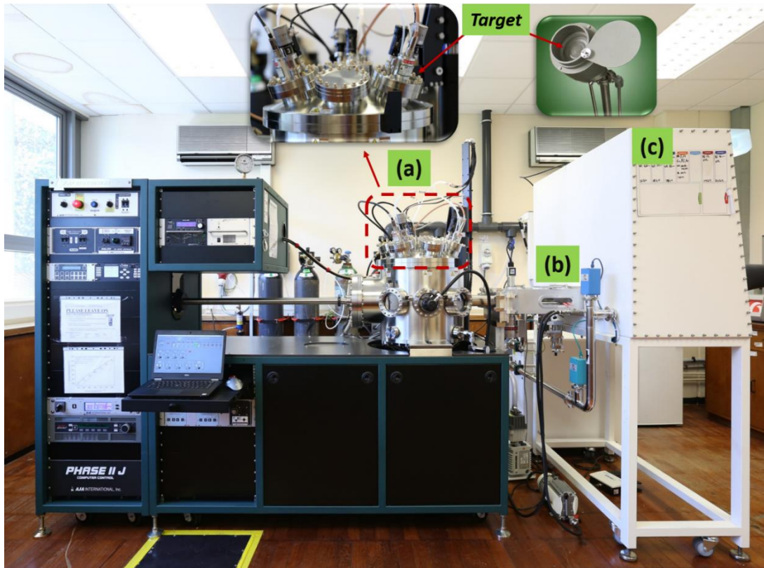
Figure 2.2 - AJA magnetron sputtering system composed of the main chamber (a) with inset presenting the 3 target currently fitted into the system, load lock mechanism for transferring the samples (b) and a glove-box for storage and handling of air sensitive samples (c).
