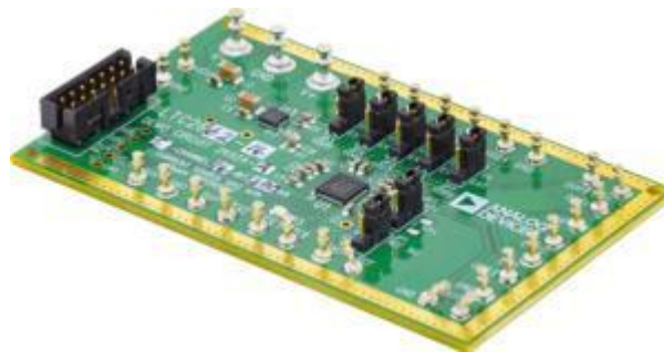
Figure 5.14: DC2692 evaluation board for the LTC chip 2662
