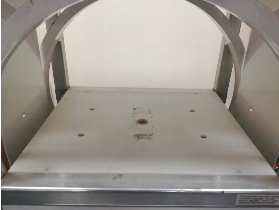
Figure 5.9: NMR surface coil on the 2881 measurement station
