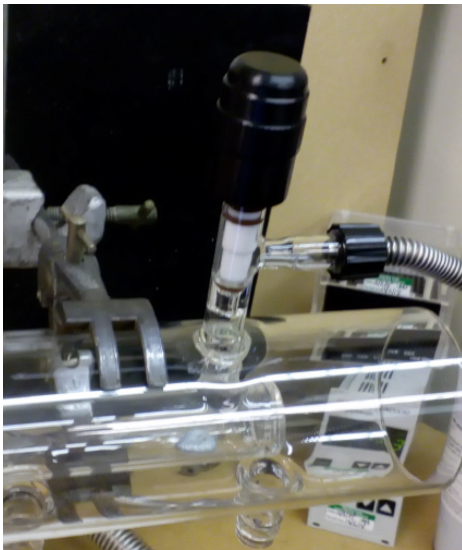
Figure 3.19: Cell connected to gas filling rig via valve stem
