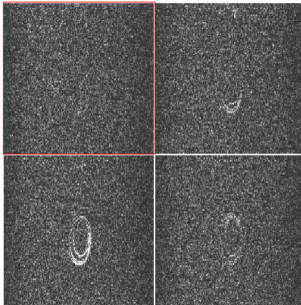
Figure 7.12: Slices 3, 4, 5 and 6 from an eight-slice 3D spoiled GRE sequence with 40 dB attenuation performed on the tube phantom
