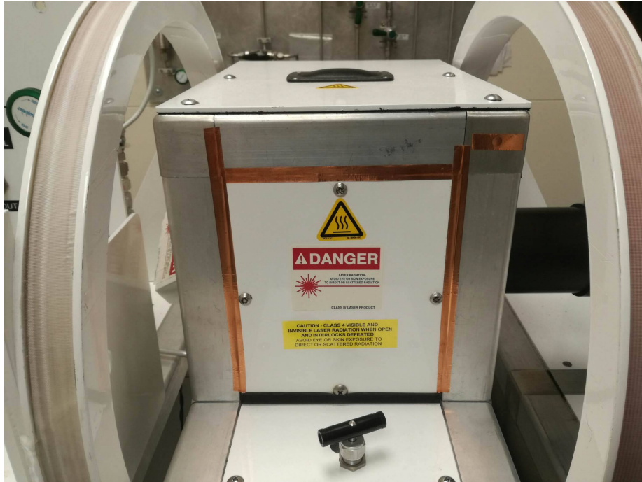
Figure 5.6: Helmholtz coils providing the B_0 field with the cell sitting inside a light-tight enclosure
