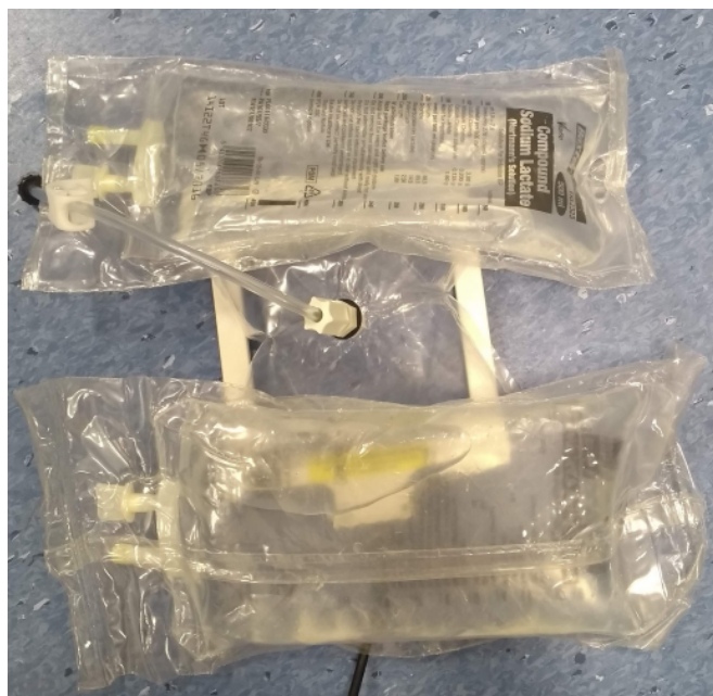
Figure 7.3: Surface coil loaded with HS bags and Tedlar bag with ^{129}\text{Xe} sitting in the coil
