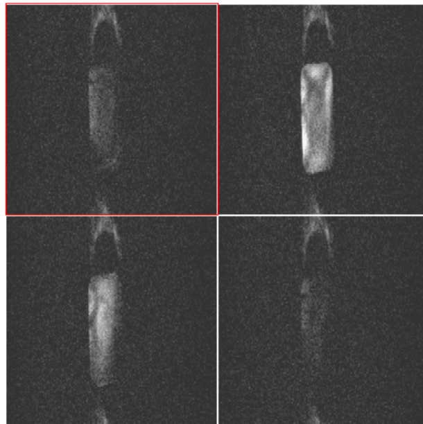
Figure 7.9: Slices 3, 4, 5 and 6 from an eight-slice 3D spoiled GRE sequence with 30 dB attenuation
