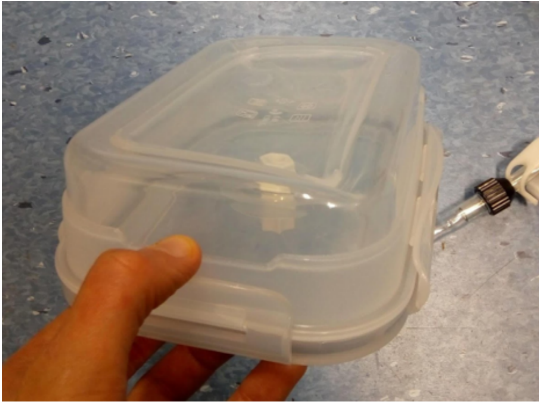
Figure 7.5: Image showing the Tupperware phantom used in the first ^{129}\text{Xe} images on the Upright, there are depressions in the phantom as it has been evacuated in preparation for HP ^{129}\text{Xe} loading.
