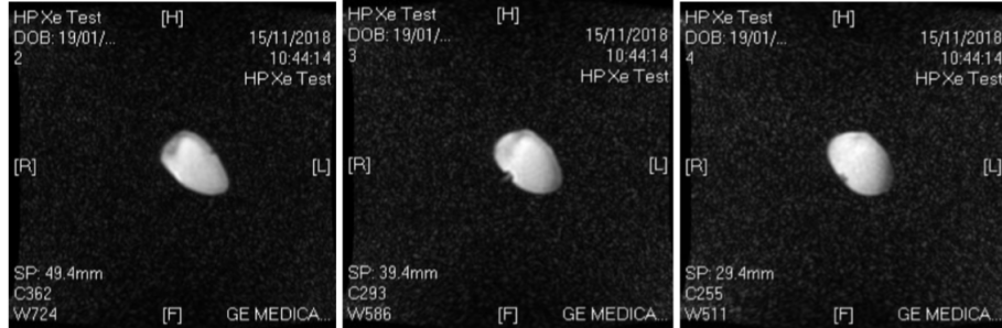
Figure 8.9: Example slices produced with the 2D FGRE sequence with a 48\text{cm}^2 FOV and 10 mm slice thickness and -2 dB RF attenuation, SNR of slice 1 = 34.1
