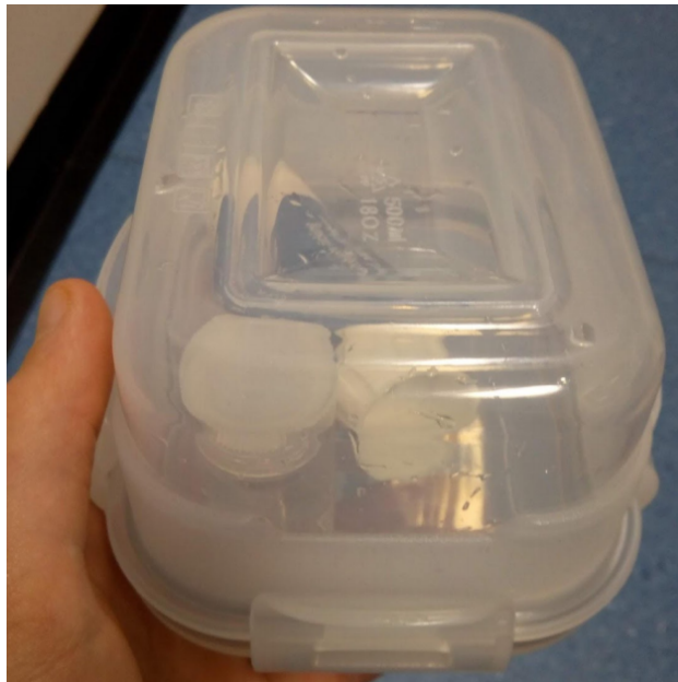
Figure 7.10: Image showing the Tupperware phantom with glue stick and glass voids
