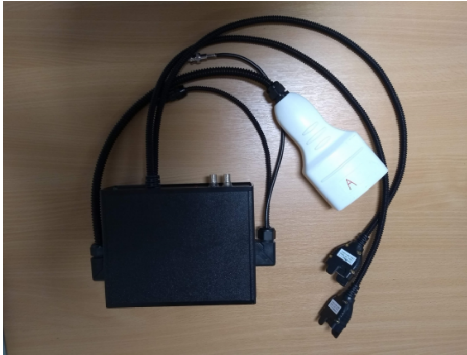
Figure 8.8: Duplexer which connects the coil and the scanner with an inbuilt GE coil ID chip
