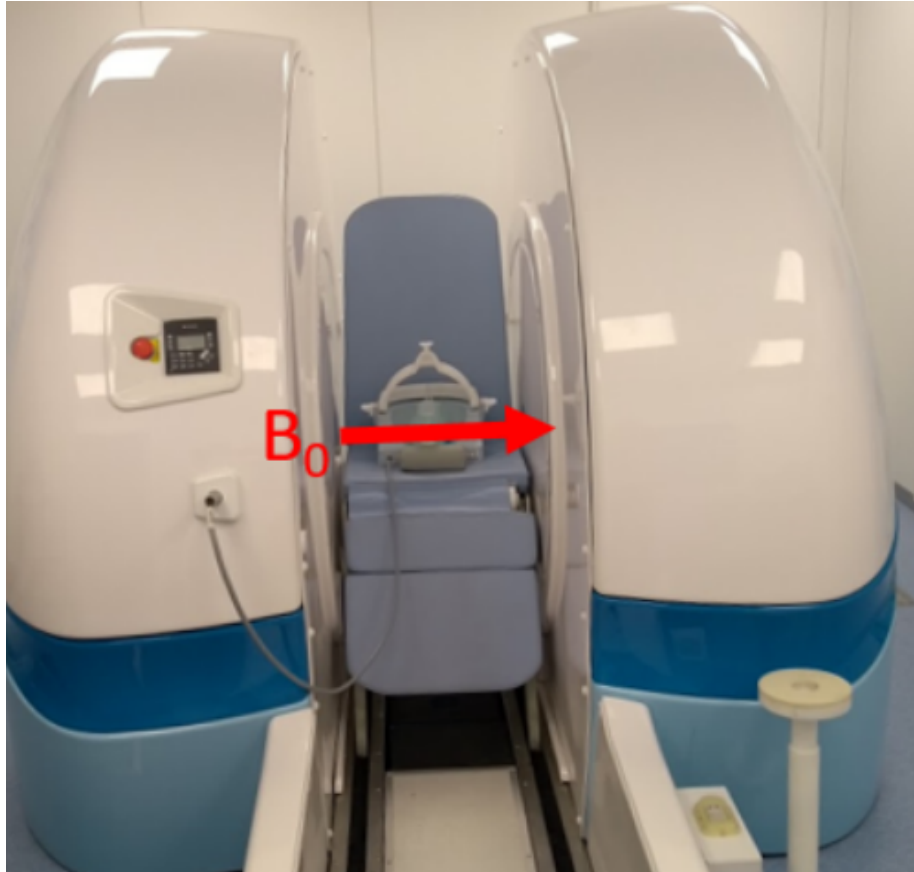
Figure 7.1: 0.5T Paramed upright MRI scanner with B_0 field direction labelled
