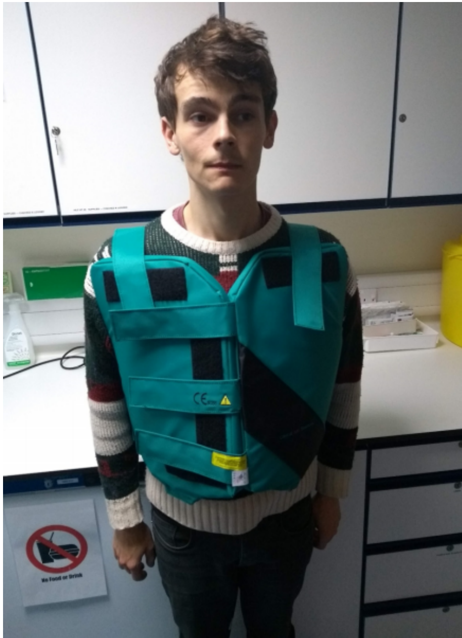
Figure 8.4: Image showing how the subject is positioned inside the CMRS coil
