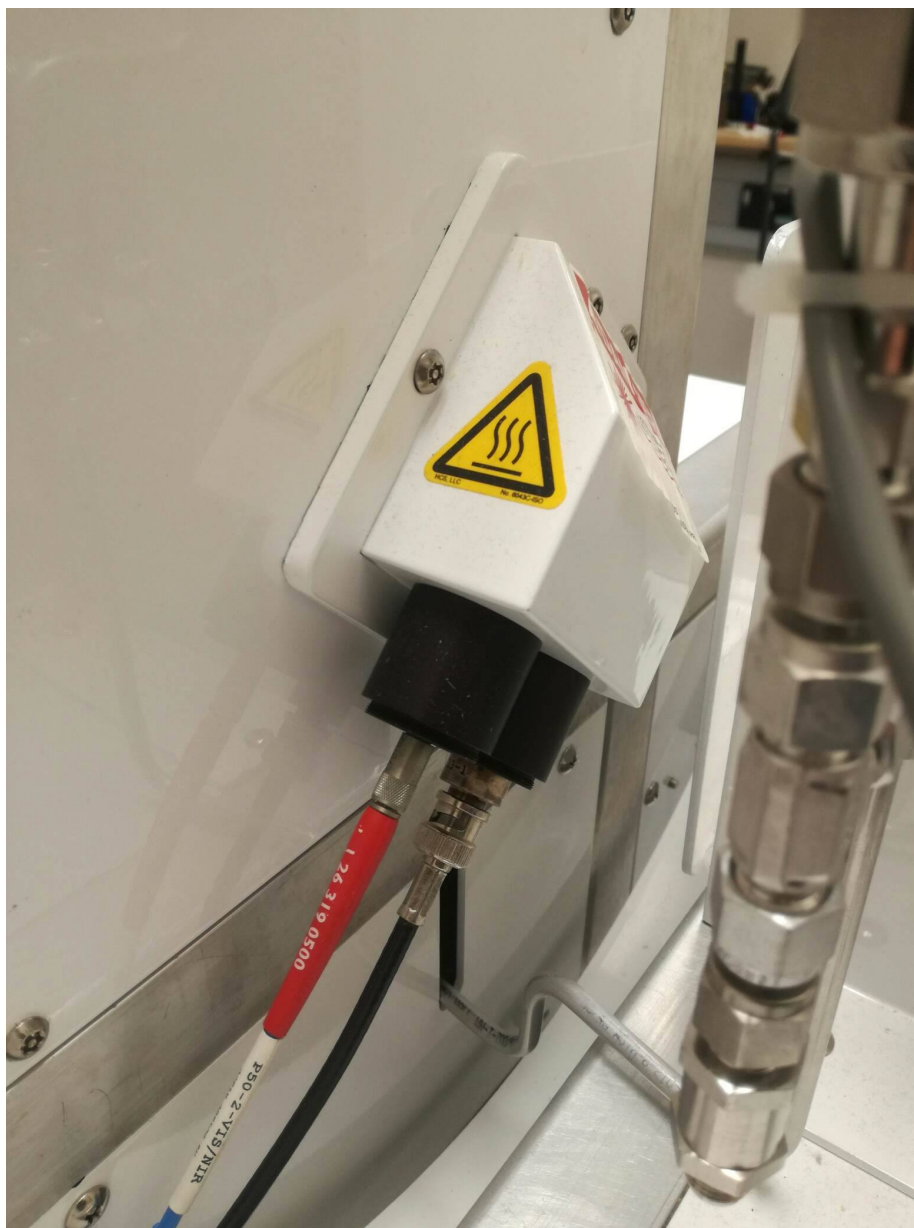
Figure 5.8: Fibre-optic cable coming out to the spectrometer (blue) and cable exiting the photodiode (black)
