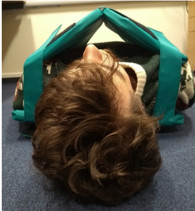
(a) Picture showing the vest deformation in a smaller subject with no pad
