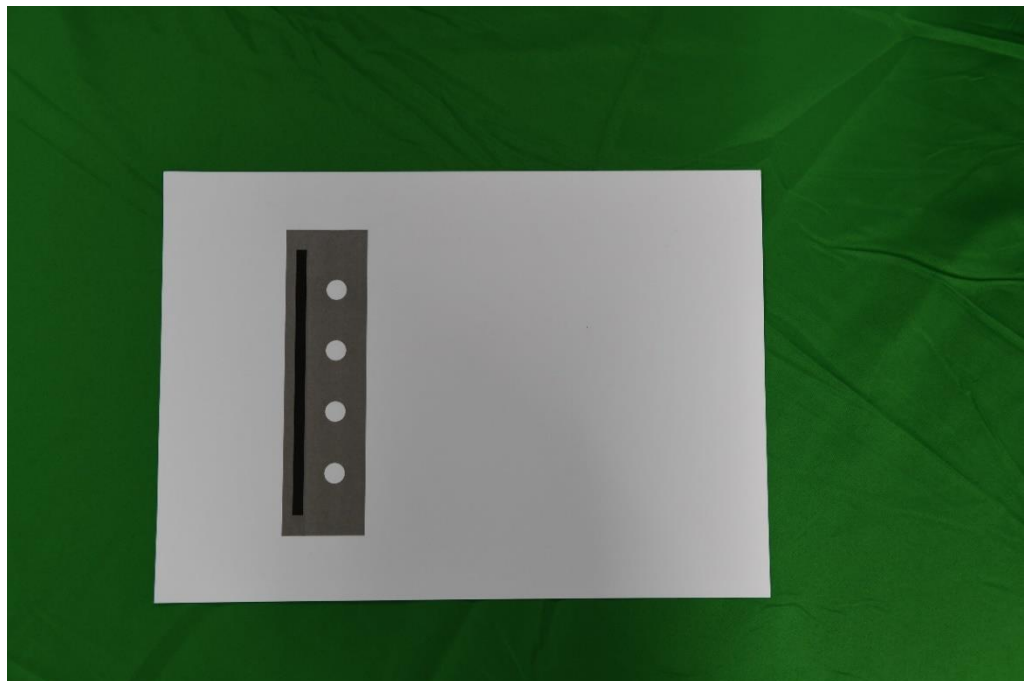
Figure 5.3: A simulated sealant line for a robot worker on the simulated workpiece with the A4 card representing the workspace and the green screen representing the image background that was isolated.
