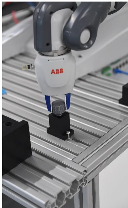
Figure 4.1: Experimental setup for the bolt tightening subtask.
