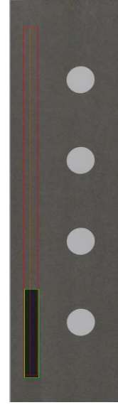
Figure 5.16: Isolated simulated workpiece for the robot worker completing the sealant line with 25% of the specified length applied, perceived and specified sealant lines highlighted.
