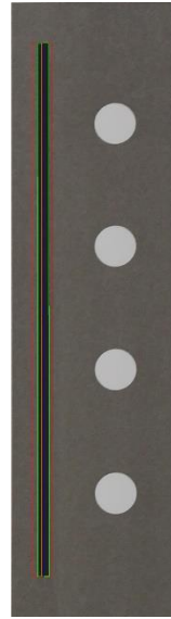
Figure 5.12: Isolated simulated workpiece for the robot worker completing the sealant line with 50% of the specified area applied, perceived and specified sealant lines highlighted.
