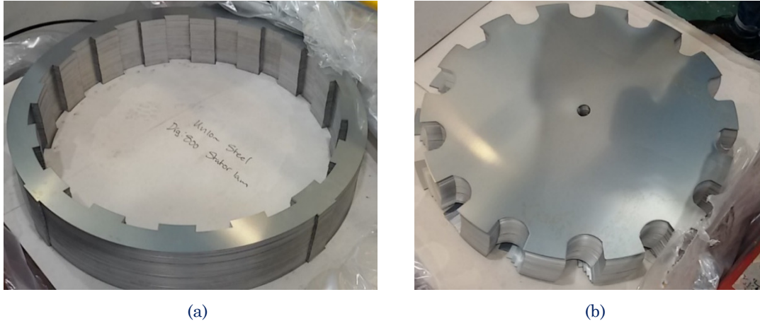
Figure A1_1 SRFLY laminations stacks after delivery: a) stator and b) rotor.
