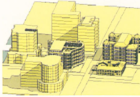
Figure 11.1 Sunlit and shaded areas on a group of building. Image generated by SunCast. model
