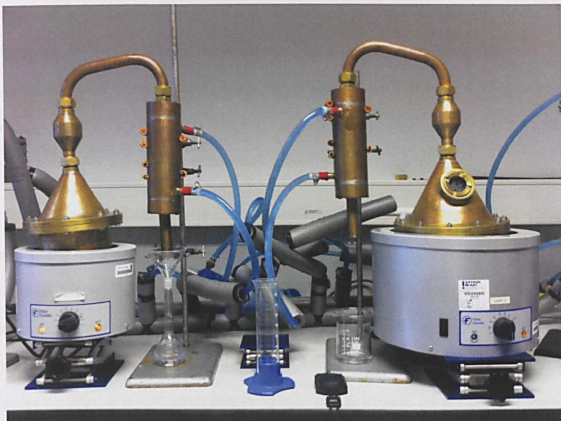
**Figure 6.1 Photograph of distillation apparatus in use.** Both stills have a splash head with an upward sloping lyne arm. The blue liquid is the 5°C cooled glycol which is pumped into the bottom of the copper shell and tube condensers to facilitate condensation.
