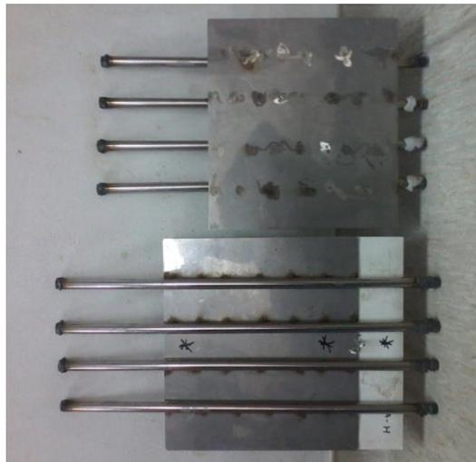
**Figure 6-4:** Rare view of PV/thermal and thermal collector
