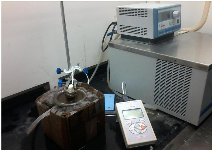
**Figure 4-4:** Thermal conductivity setup
