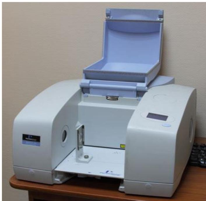
**Figure 4-7:** FTIR instrument of Perkin Elmer
