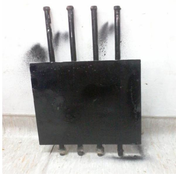
**Figure 6-5:** Solar thermal collector after black coating
