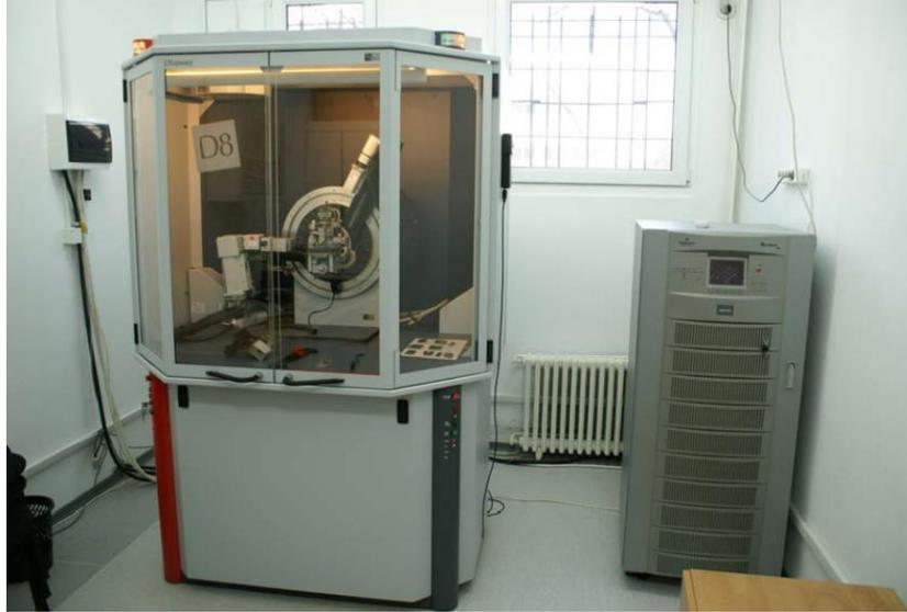
Figure 4-8: X-ray Diffractometer of Bruker
