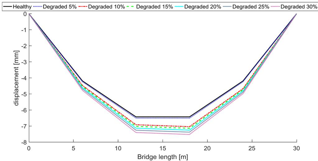
**Figure 4.** Displacements of the healthy and degraded bottom chord on the left hand side of the bridge model
