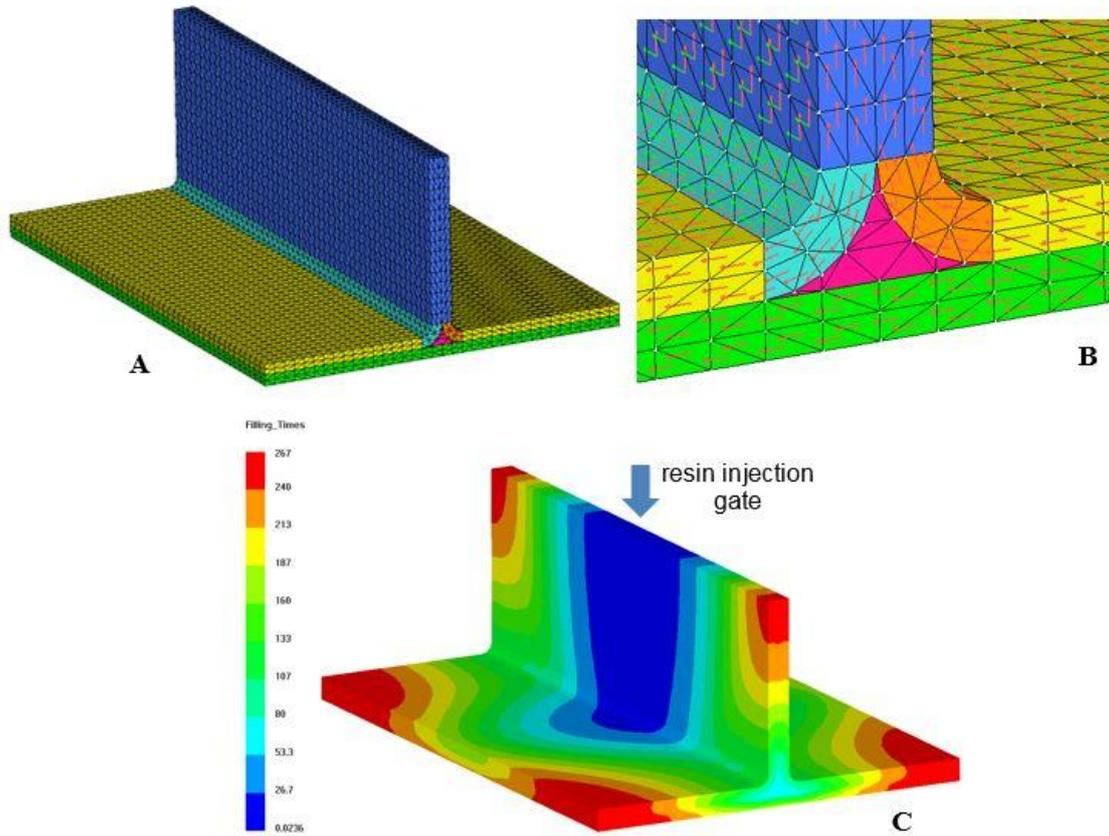
*Figure 5: An illustration of the simulation of infusing one of the sub-components in BAM (T-joint) using PAM-RTM – based on permeability values determined experimentally; (A) 3D mesh of the T-joint geometry; (B) geometrical detail with material orientations; (C) resin flow fronts at different injection times.*
