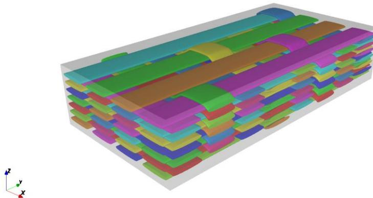
*Figure 10: Illustration of the Layer-to-layer unit cell (designed by Sigmalex using TexGen)*
