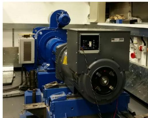
Fig. 11. Experimental test bench of the considered SG.
