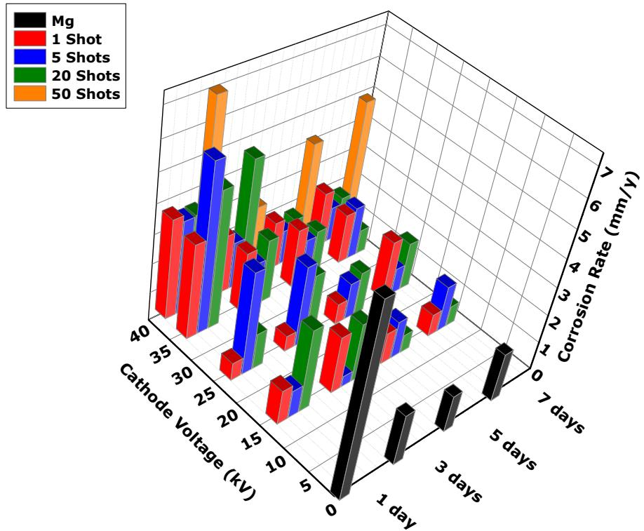
**Figure 6-16** Corrosion rates of Mg and LAEB modified Mg surfaces, immersed up to 7 days in PBS at 37°C. Errors not shown for clarity purposes.
