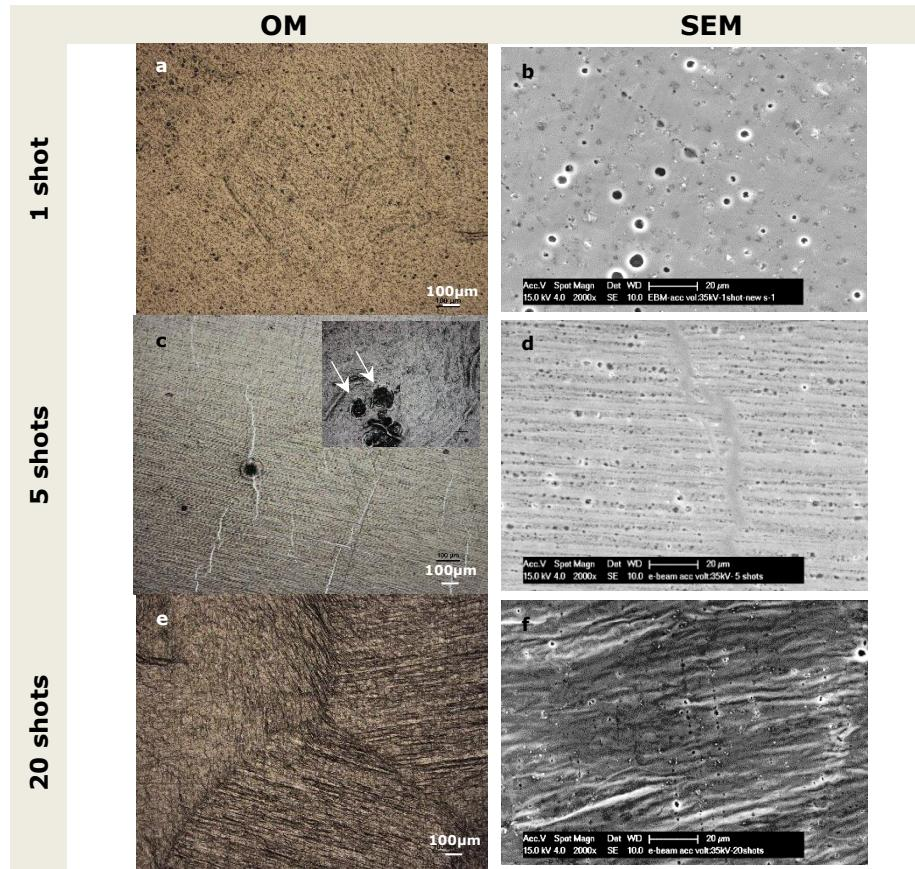
**Figure 6-3** OM and SE images of Mg surfaces modified by LAEB processing (35kV; 1, 5 and 20 pulses).
