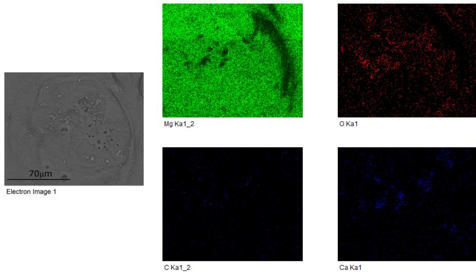
**Figure 6-6** EDS elemental maps for LAEB processed Mg (40 kV; 5 pulses). The presence of Ca is tentatively assigned to an unknown source of cross-contamination
