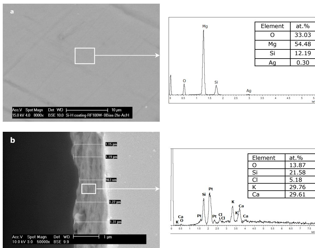
**Figure 5-17** BSE images and associated EDS spectra for: (a) a-Si:H coated Mg in plan-view orientation; (b) a-Si:H coated Mg in cross-sectional orientation.
