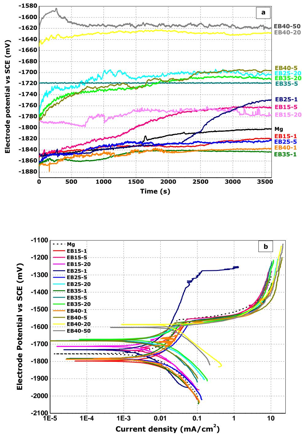
**Figure 6-13** Electrochemical corrosion tests of as-prepared and LAEB processed Mg-surfaces, in PBS at  $37^\circ\text{C}$  (-200 mV to +500 mV): (a) OCP; and (b) potentiodynamic polarization tests.
