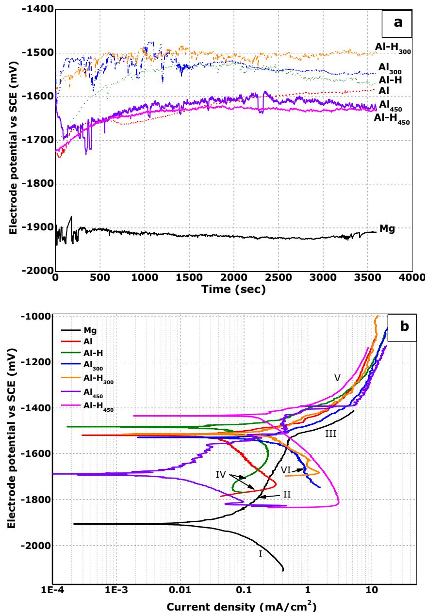
**Figure 5-9** (a) Open circuit potential; & (b) potentiodynamic polarization curves for as-deposited Al and Al-H coatings on Mg; and heat-treated Al<sub>300</sub>, Al-H<sub>300</sub>, Al<sub>450</sub> and Al-H<sub>450</sub> coatings, furnace annealed in air at 300°C and 450°C; immersed in PBS at 37°C.
