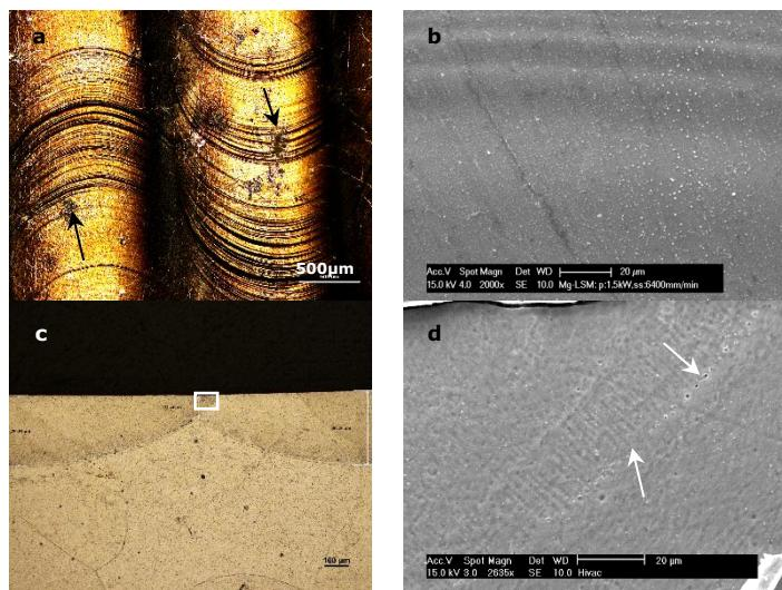
**Figure 6-23** OM and SE images of Mg surfaces LSM processed at 1500 W, 6300 mm/minute with a laser spot size of 3 mm: (a) overlapped laser track width; in plan view (b) SE of Mg particles and cracks on laser tracks; in plan view (c) OM image showing cross section of tracks depth; and (d) SE inset of cross-section of overlapped region.
