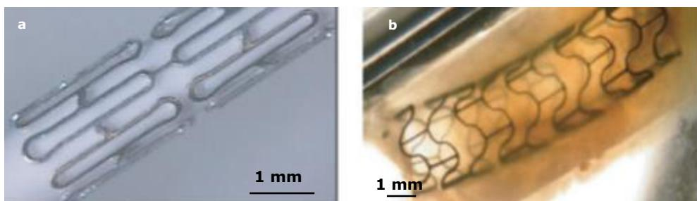
**Figure 2-4** Photo-micrographs showing an Mg-alloy stent (a) unexpanded; and (b) expanded in a coronary artery [24]
