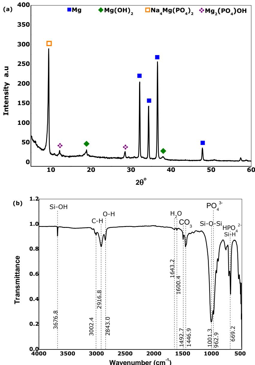
**Figure 5-23** (a) XRD pattern (b) FTIR spectrum for an a-Si:H coating on Mg, corroded in PBS at 37°C.
