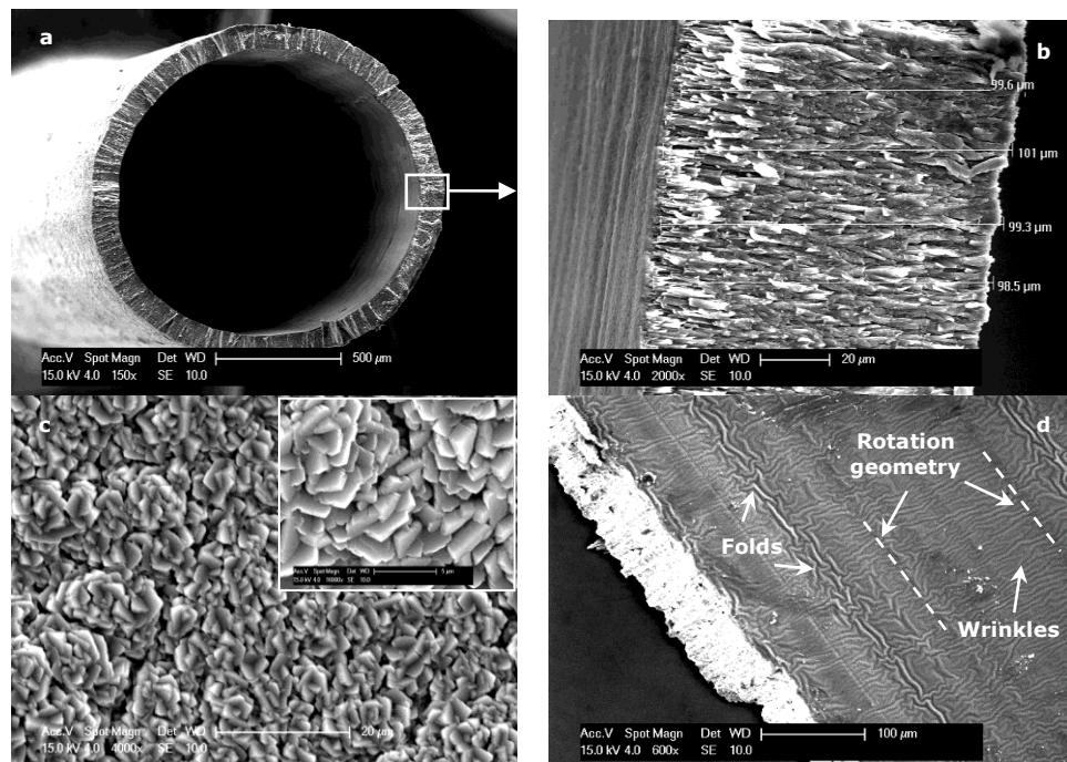
**Figure 4-7** SE images of an as-deposited Mg minitube; (a) fractured cross-section, (b) higher magnification image of the fractured minitube wall; (c) minitube outer surface (with higher magnification image inset); and (d) minitube internal surface.
