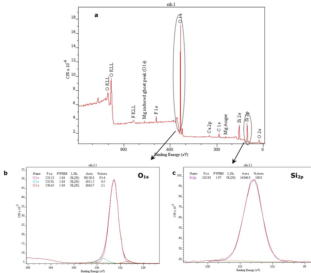
**Figure 5-19** XP-survey scan and high resolution O<sub>1s</sub> and Si<sub>2p</sub> spectra of as-deposited a-Si:H on Mg.
