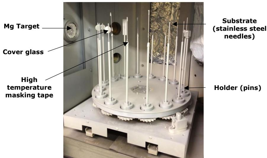
**Figure 3-1** Sample stage and holders used for the fabrication of Mg-minitubes
