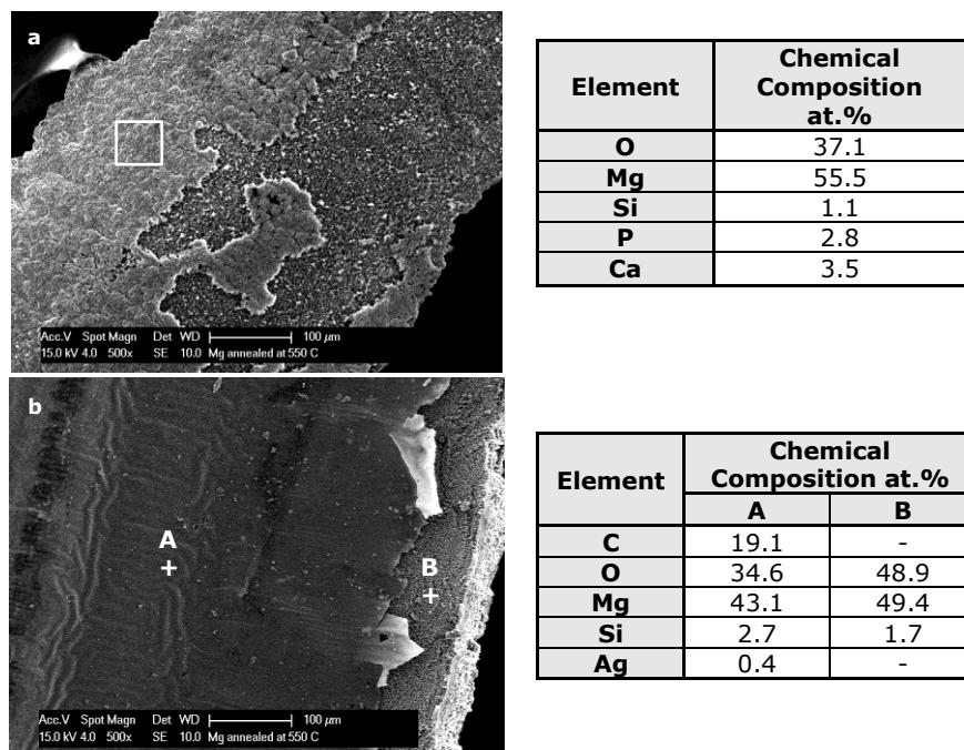
**Figure 4-13** SE images and EDS analyses of: the (a) external surface; and (b) internal surface of a PVD deposited Mg minitube annealed at 550°C.
