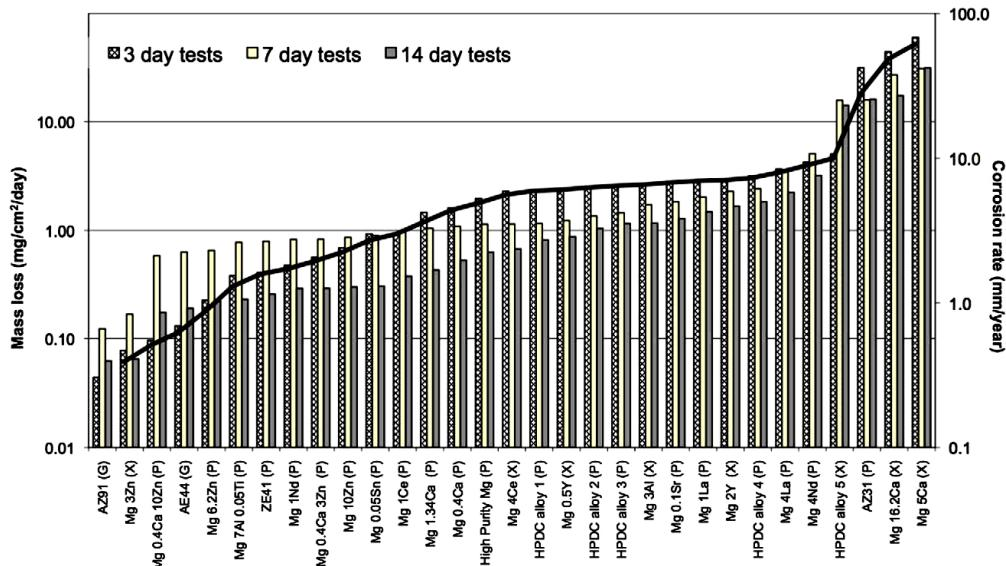
**Figure 2-22** Degradation rates for various Mg-alloys in MEM, at 37°C. The symbol 'G' refers to general corrosion, 'P' pitting corrosion, and 'X' localised corrosion [227].
