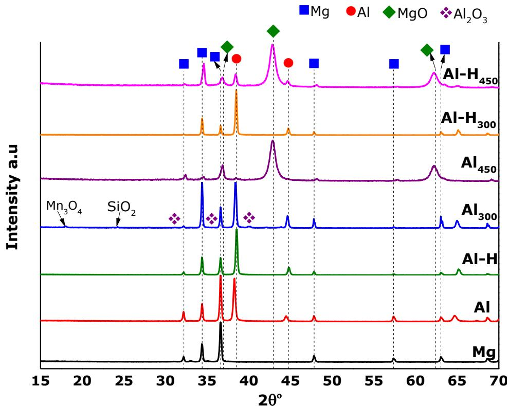
**Figure 5-1** XRD patterns of as-deposited and heat-treated Al and Al-H coatings on Mg.
