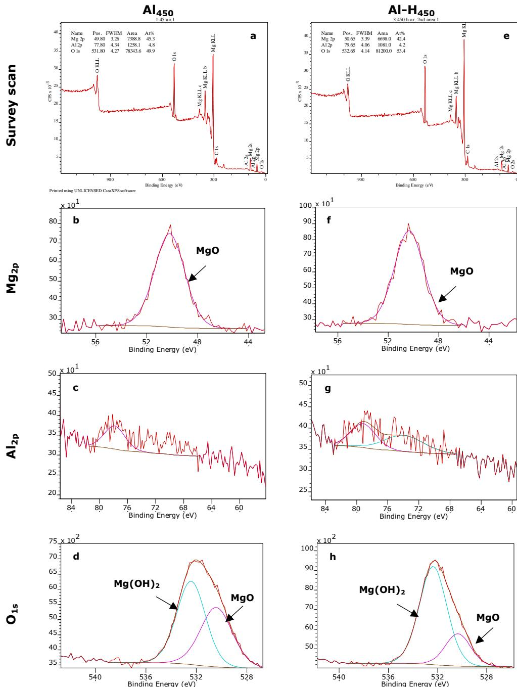
**Figure 5-8** Survey and HR-XPS spectra of (a-d) Al<sub>450</sub> and (e-h) AlH<sub>450</sub>, annealed at 450°C.
