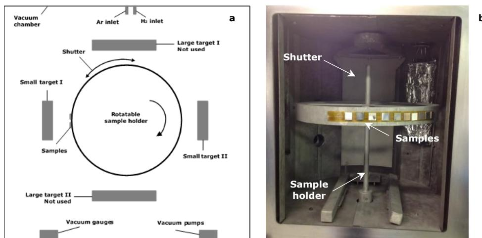
**Figure 3-3** (a) Schematic diagram showing targets and sample arrangement inside the PVD system (adapted from [228]); and (b) Mg samples mounted on the sample holder, prior to PVD coating.
