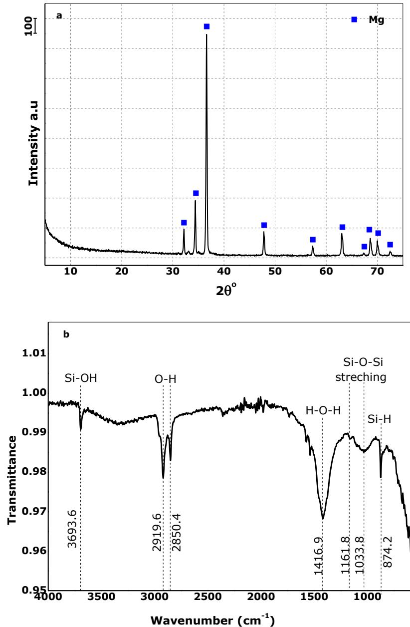
**Figure 5-16(a)** XRD pattern of an a-Si:H coating on Mg; (b) representative FTIR absorption spectrum of an a-Si:H coating on Mg.
