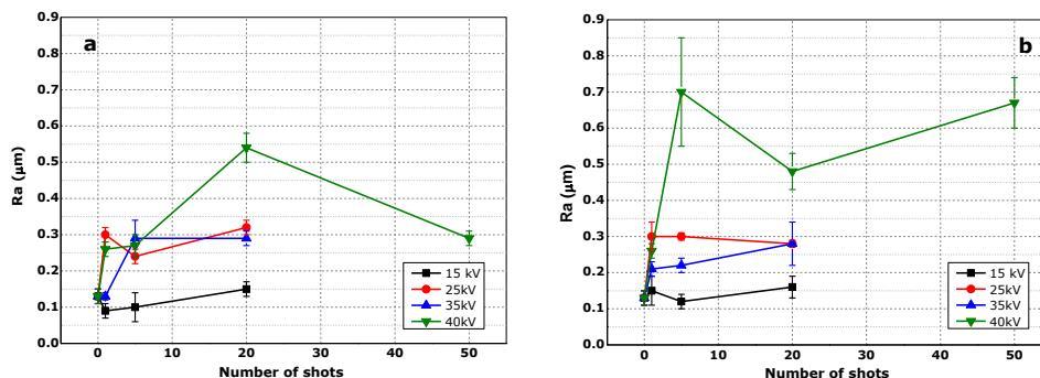
**Figure 6-8** Surface roughness (Ra) as a function of cathodic voltage and number of pulses: (a) in the middle; and (b) at the edges of the EB processed areas.
