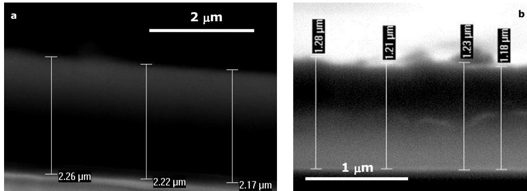
**Figure 5-4** Cross-sectional SE images of as-deposited: a) Al, and b) Al-H coatings, showing how thickness measurements were performed.
