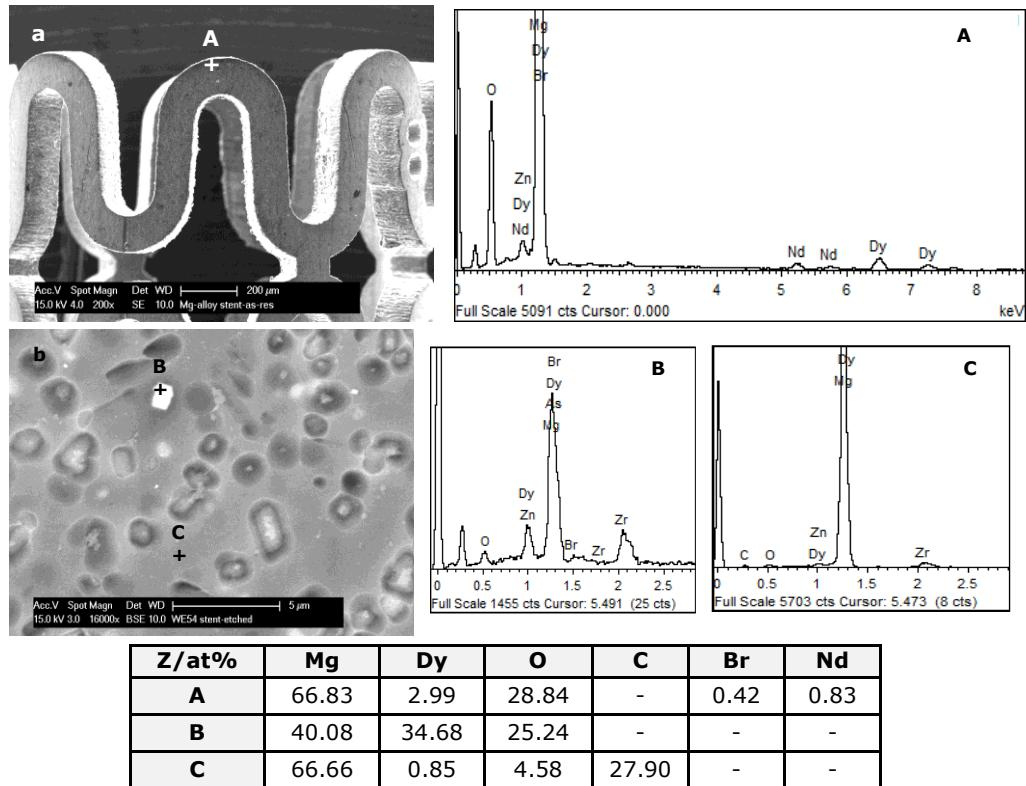
**Figure 4-2** EDS analysis of a commercial Mg-alloy stent: (a) as-received surface in plan-view orientation; (b) surface etched in acetic glycol, in cross-sectional orientation.
