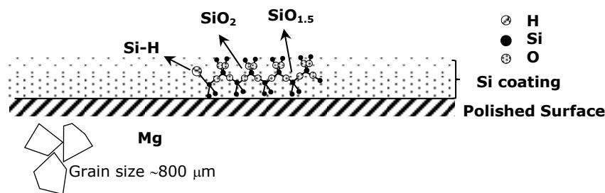
**Figure 5-25** Schematic illustration of a-Si:H coating of Mg.
