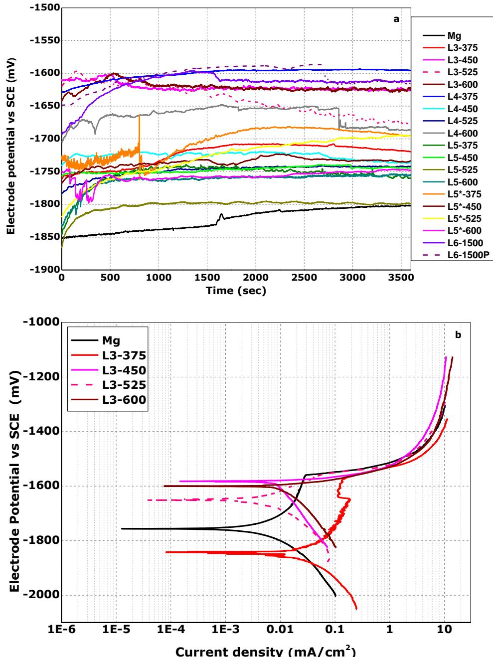
**Figure 6-26** (a) OCP and potentiodynamic polarization curves for as-prepared and LSM processed Mg-surfaces for scanning speeds of: (b) 3600 mm/minute, (c) 4500 mm/minute, (d) 5400 mm/minute, and (e) scanning speed of 5400 and 6300 mm/minute (spot size 3 mm).
