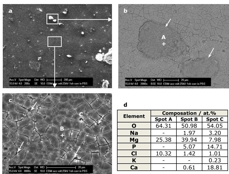
**Figure 6-15** Corrosion morphology of an Mg surface, LAEB modified (25 kV, 1 pulse), after potentiodynamic polarization testing in aerated PBS at 37°C. (a) An overview of the corrosion morphology; (b) BSE image of the reaction products; (c) SE image of the passivation layer; and (d) associated EDS data.
