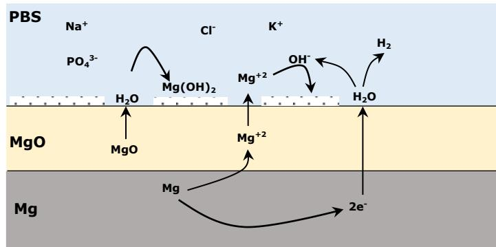
**Figure 4-22** Schematic showing the competing processes of dissolution and film formation on an MgO/Mg surface.
