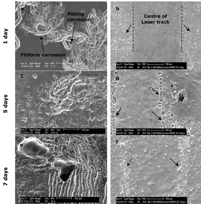
**Figure 6-29** Corrosion morphologies of: (a,c,e) as-polished; and (b,d,f) LSM processed Mg surfaces, in plan view orientation, after immersion corrosion testing for 1, 5 and 7 days, respectively, in PBS at 37°C.
