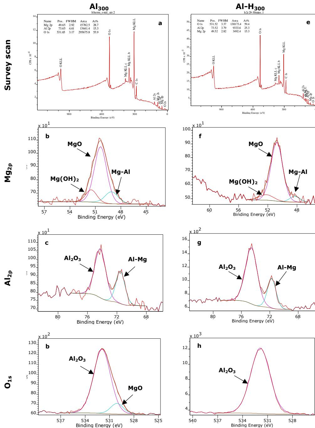
**Figure 5-7** Survey scan and HR-XPS of coatings annealed at 300°C: (a-d) Al<sub>300</sub>; and (e-h) Al-H<sub>300</sub>.
