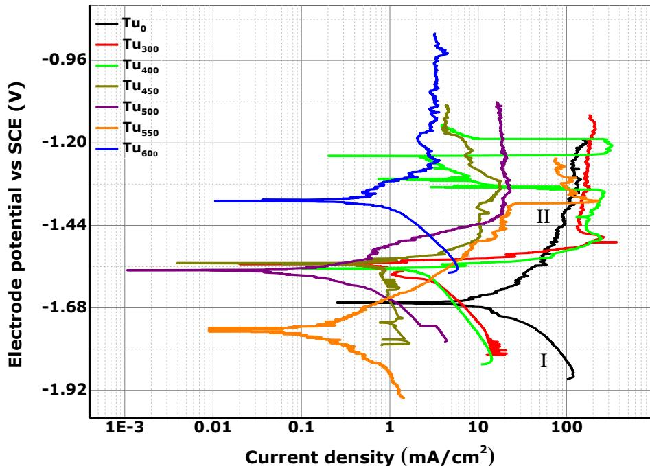
**Figure 4-19** Potentiodynamic polarization curves for as-deposited & annealed Mg-minitubes in PBS at  $37\pm 1^\circ\text{C}$ .
