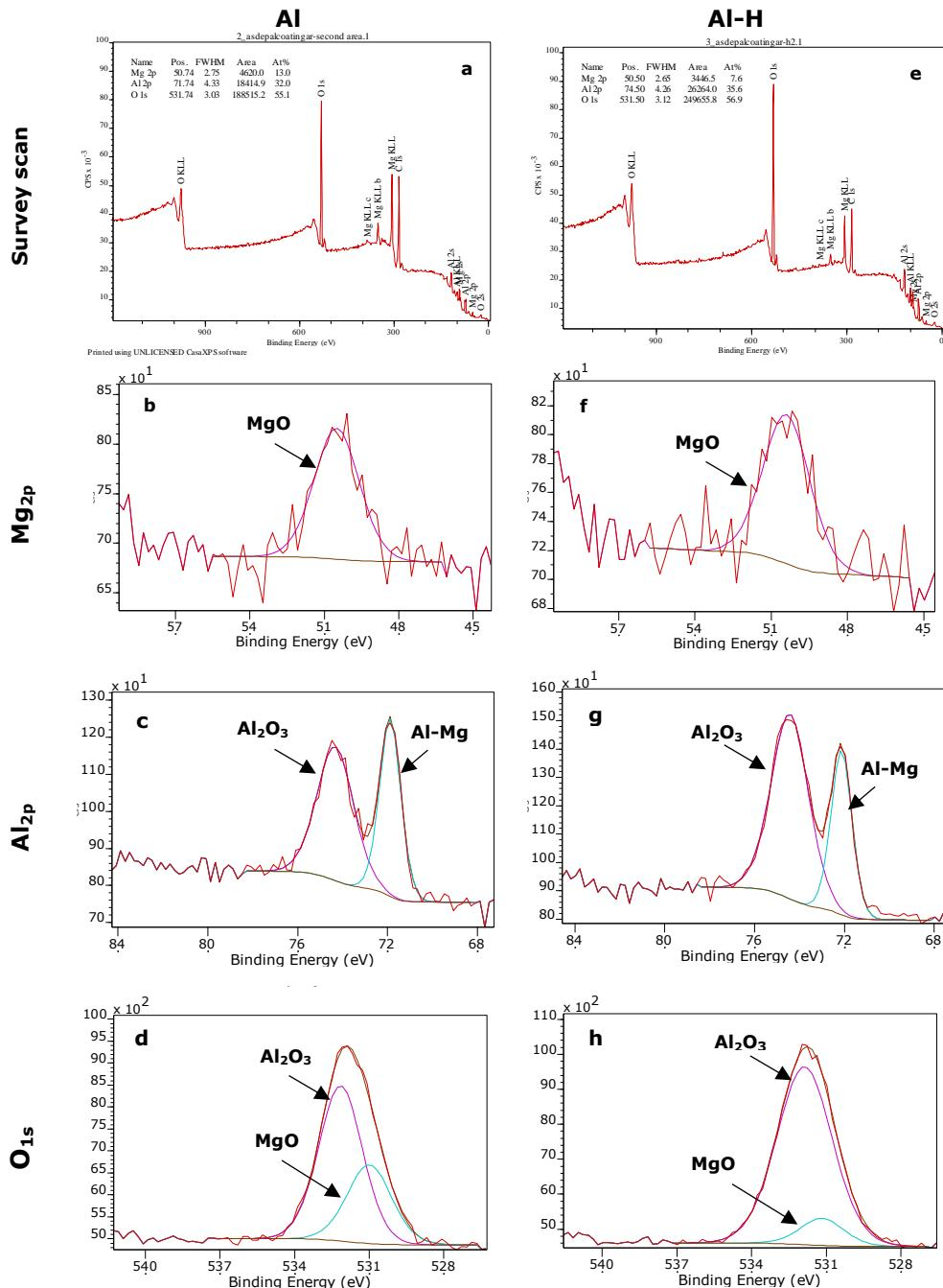
**Figure 5-6** Survey and HR-XPS of as-deposited Al: (a) survey scan; (b) Mg<sub>2p</sub>; (c) Al<sub>2p</sub>; and (d) O<sub>1s</sub>; and Al-H: (e) survey scan; (f) Mg<sub>2p</sub>; (g) Al<sub>2p</sub>; and (h) O<sub>1s</sub>.
