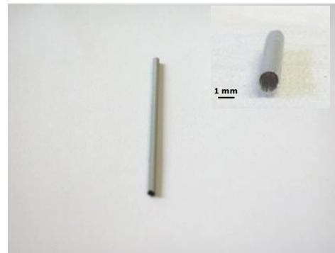
**Figure 4-6** Photograph of an as-deposited Mg minitube.
