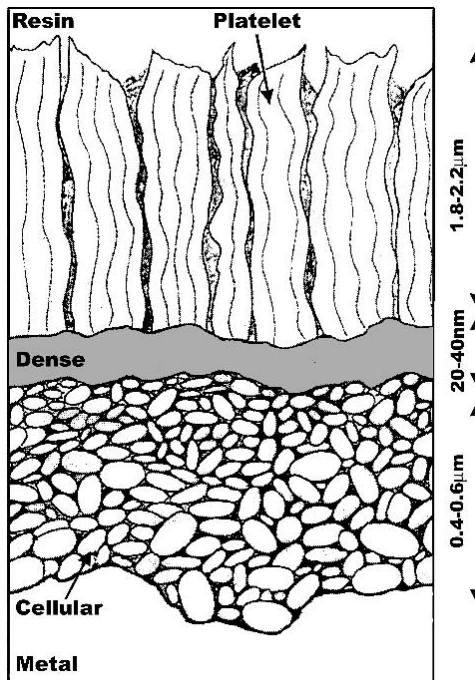
**Figure 2-10** Schematic illustration of the passivation film structure formed on Mg immersed in water (after 48 h) [93].
