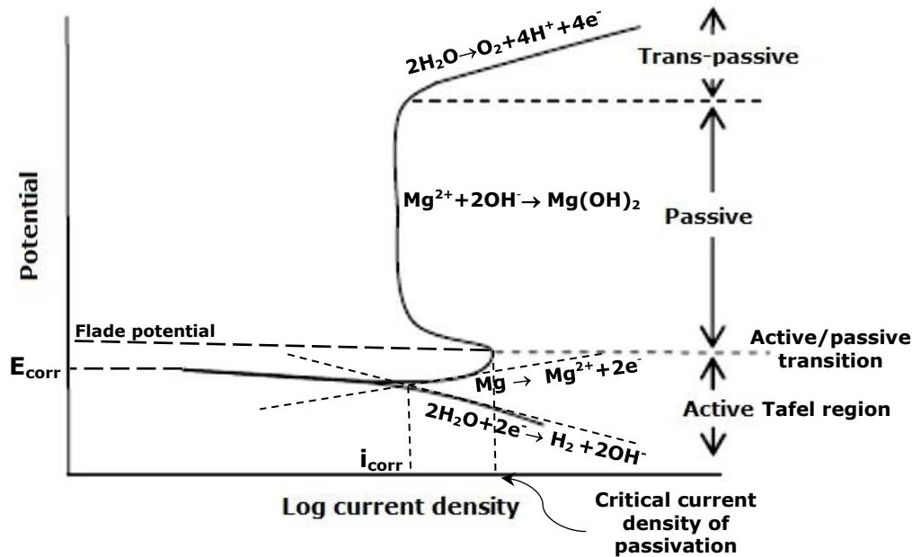
**Figure 2-15** Typical polarization curve illustrating active-passive behaviour and the extraction of key parameters. The active region refers to hydrogen evolution and Mg dissolution; the passive region refers to the formation of a passivation film on the Mg surface; and the trans-passive region refers to oxygen evolution.
