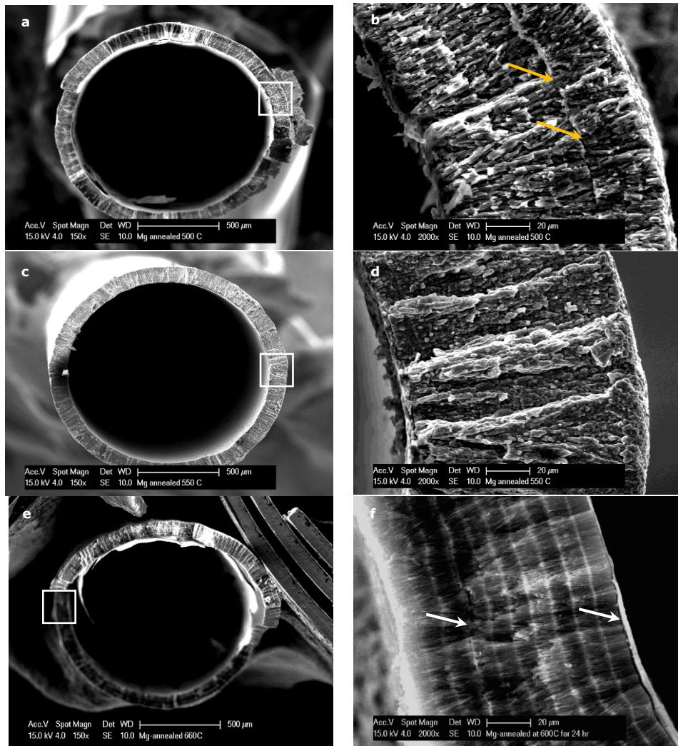
**Figure 4-12** SE images of Mg minitubes annealed for 24 h: at (a,b) 500°C; (c,d) 550°C; and (e,f) 600°C, respectively.
