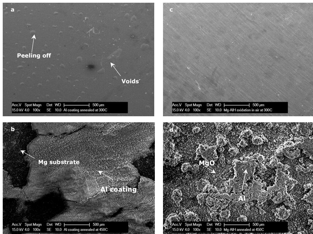
**Figure 5-3** SE images of Al and Al-H coatings annealed in open air, at 300°C for 5 h and 450°C for 2 h: (a) Al<sub>300</sub>; (b) Al<sub>450</sub>; (c) Al-H<sub>300</sub> and (d) Al-H<sub>450</sub>.
