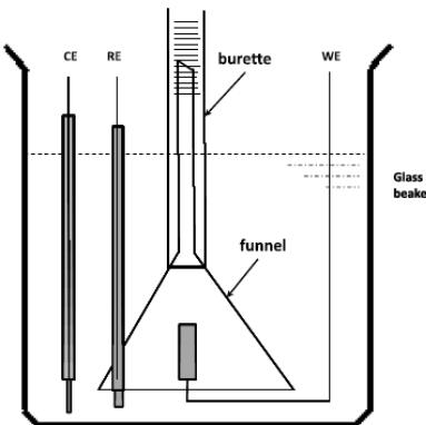
**Figure 2-14** Schematic showing the experimental arrangement for  $H_2$  gas evolution experiments [102]
