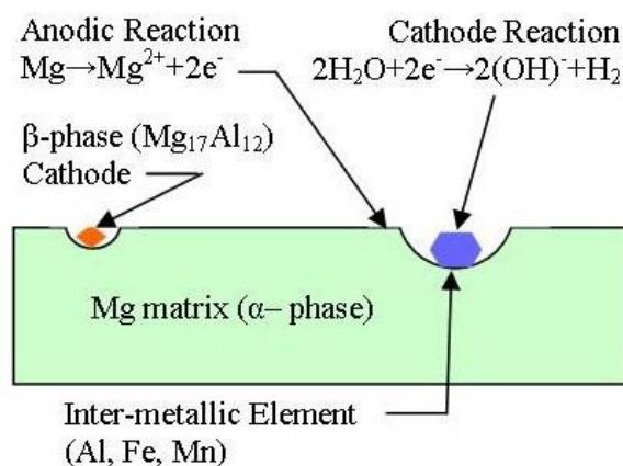
**Figure 2-11** Galvanic corrosion in the presence of intermetallic elements [99]
