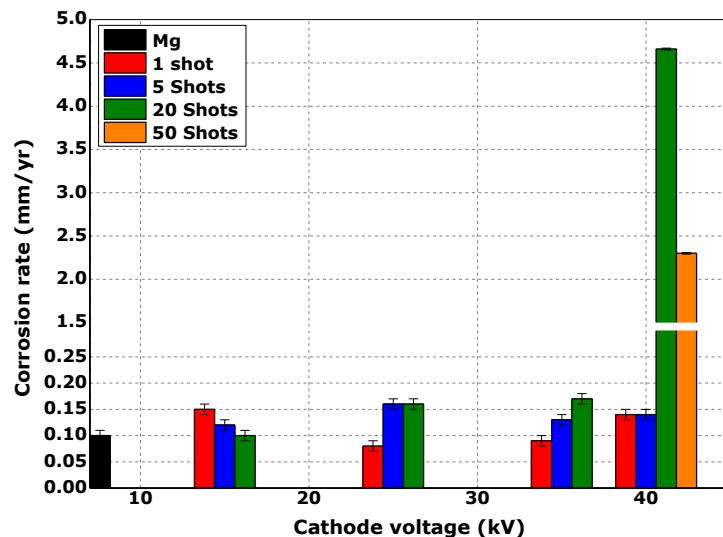
**Figure 6-14** Corrosion rate as a function of kV and number of pulses
