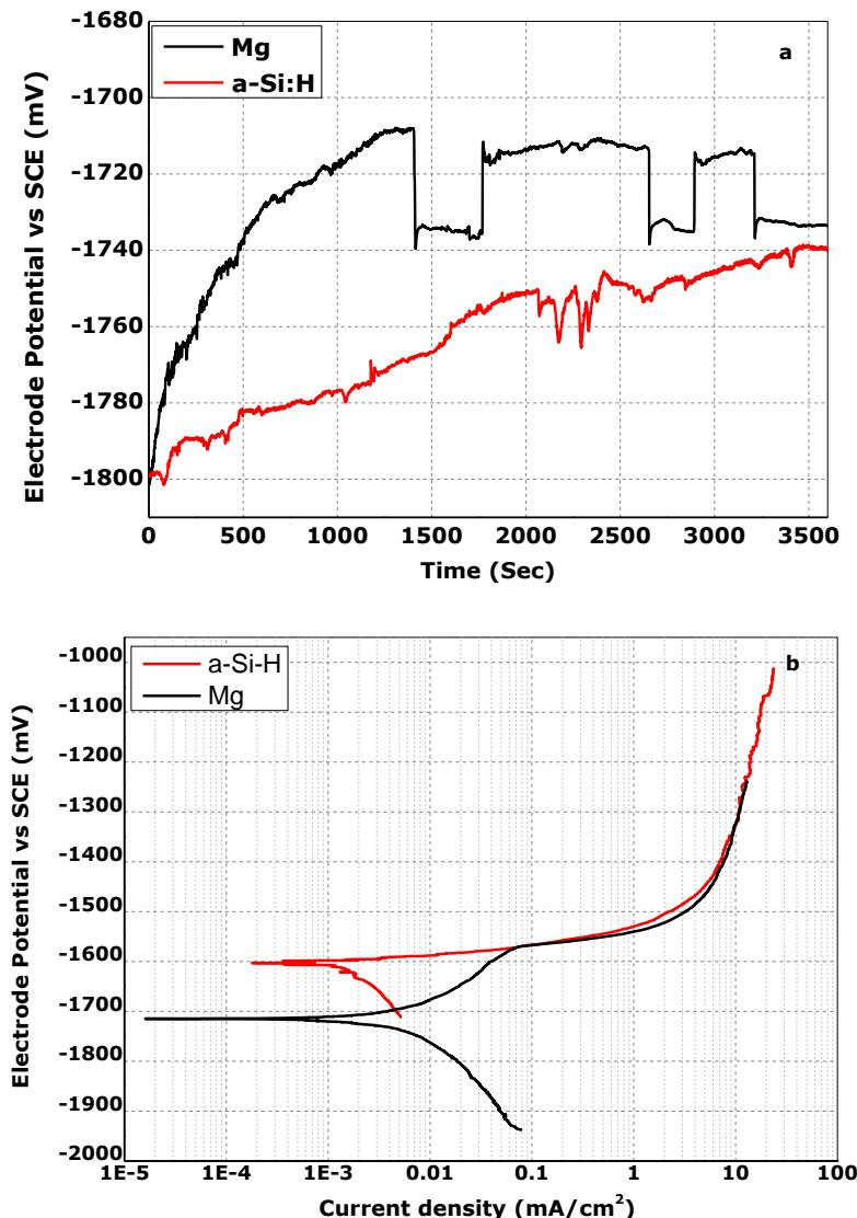
**Figure 5-20** (a) OCP and (b) potentiodynamic polarization curves for as-polished Mg and a-Si:H coated Mg
