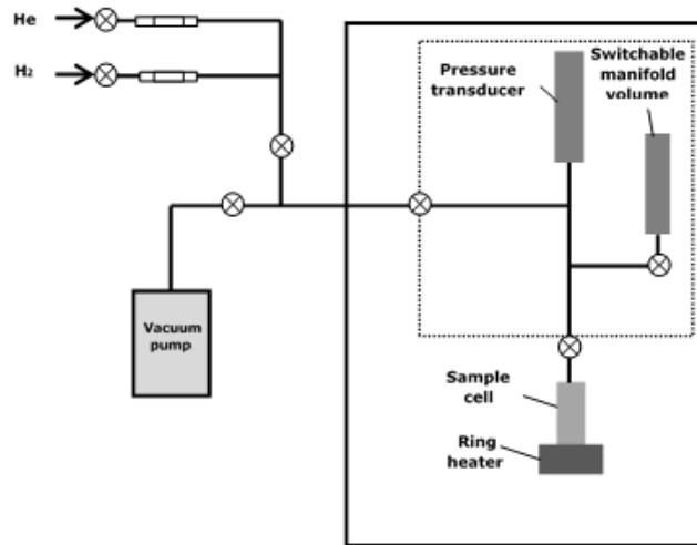
**Figure 3-2** Key components of the Sieverts heat-treatment apparatus, adapted from [228].
