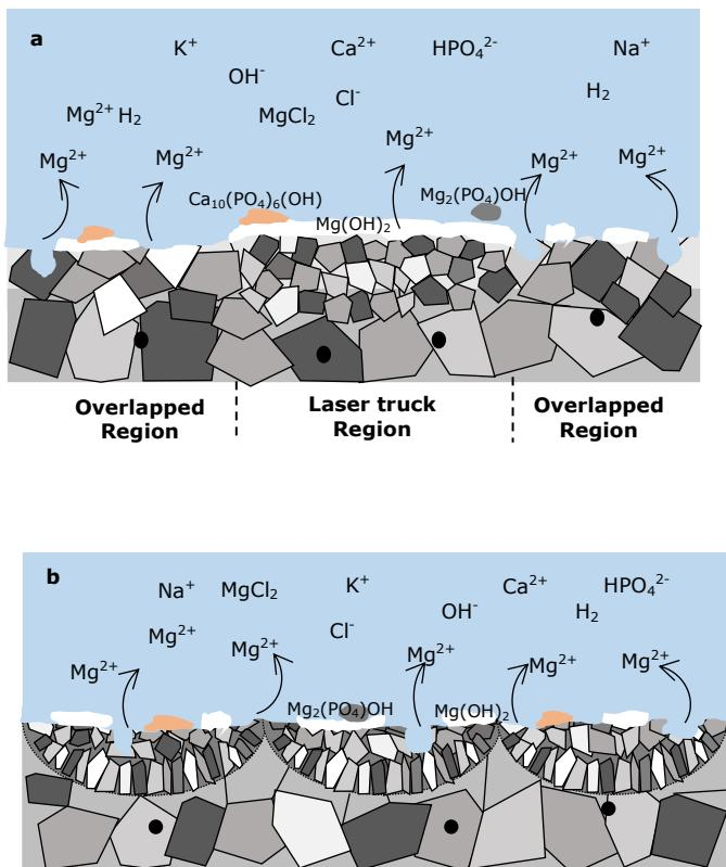
**Figure 6-32** Schematic illustration of corrosion mechanism of LSM Mg surface: (a) Low energy LSM processed surface; and (b) high energy LSM processed surface.
