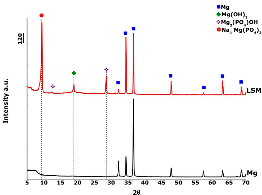
**Figure 6-30** XRD patterns of as-polished and LSM processed Mg surfaces after 1 day immersion corrosion testing in PBS at 37°C.
