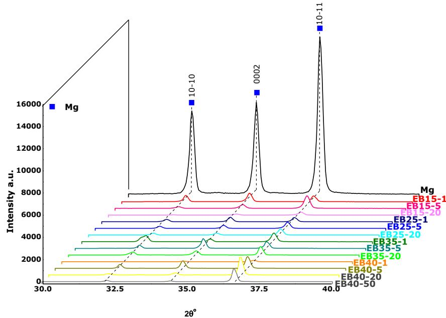
**Figure 6-10** XRD patterns of as-prepared and LAEB processed Mg surfaces. Low intensity of EB modified Mg suggests the modified layer had not recovered full crystallinity.
