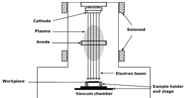
**Figure 3-4** Schematic illustration of an Sodick PF32A LAEB machine, adapted from [193].
