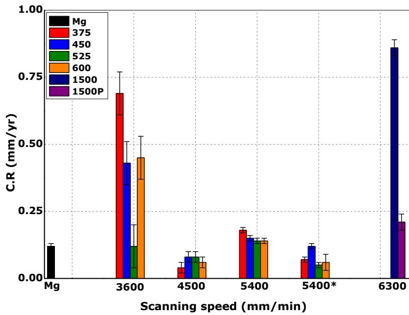
**Figure 6-27** Corrosion rate as a function of laser scanning speed, for various laser powers.
