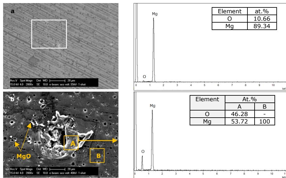
**Figure 6-5** EDS analyses of LAEB processed Mg surfaces: (a) 35 kV; 1 pulse; and (b) 40 kV; 1 pulse.
