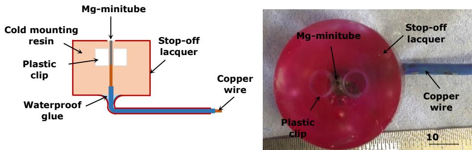
**Figure 3-11** (a) Schematic diagram; and (b) photograph of an Mg minitube working electrode.
