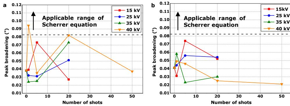
**Figure 6-11** Peak broadening of as-prepared and LAEB processed Mg surfaces, as a function of kV and number of pulses: using (a) 0002 and (b) 10-11 diffraction peaks.
