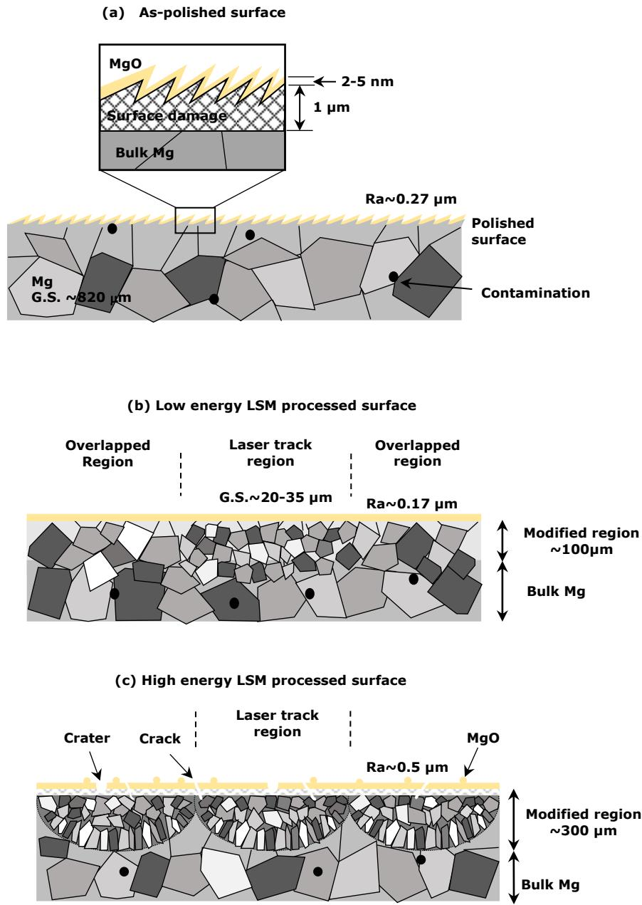
**Figure 6-31** Schematic diagrams showing the proposing mechanisms of surface modification under LSM irradiation: (a) as-polished surface; (b) low energy LSM processed surface; and (c) high energy LSM processed surface.
