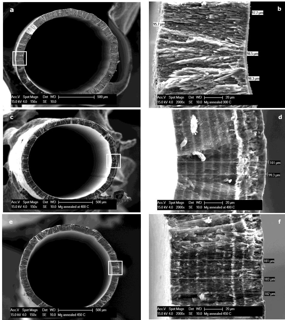
**Figure 4-11** SE images of Mg minitubes annealed at: (a,b) 300°C; (c,d) 400°C; and (e,f) 450°C, respectively.
