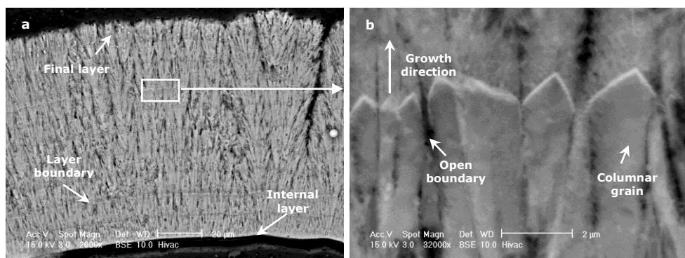
**Figure 4-8** BSE images of an as-deposited Mg minitube, etched with acetic glycol.
