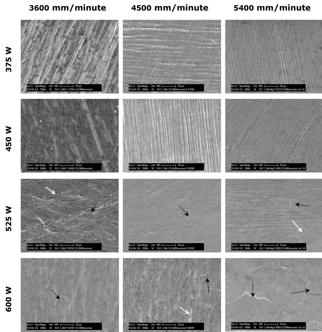
**Figure 6-21** SE images of Mg surfaces following LSM surface processing. The black arrowed areas indicate a refinement of surface morphology with the perception of small sized grains. The white arrows indicate presence of remnant deep polishing marks
