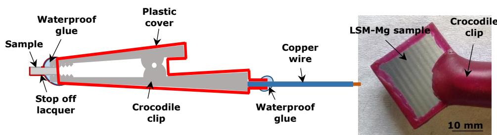
**Figure 3-10** (a) Schematic diagram of LSM, EBM and PVD coating working electrodes; and (b) photograph of an LSM working electrode.
