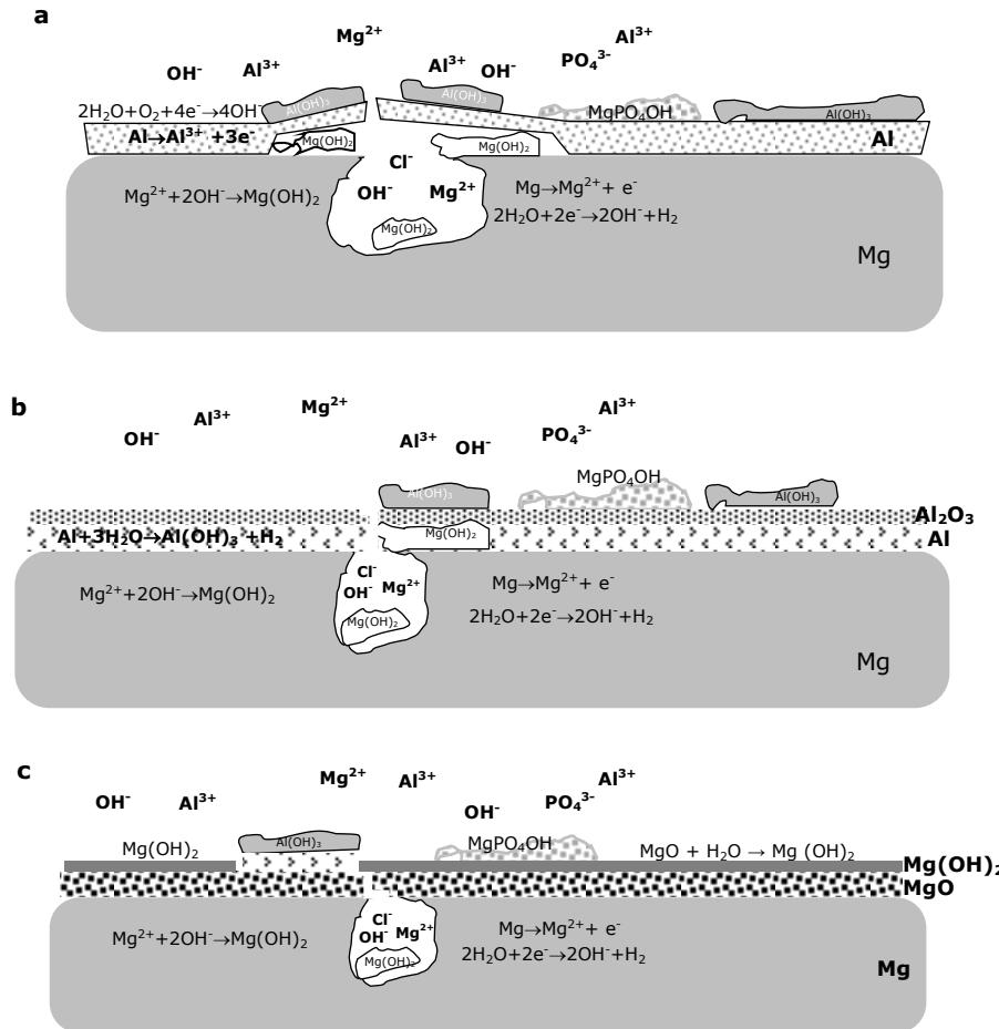
**Figure 5-14** Schematic illustration of the corrosion process of Al/Al-H coated Mg upon immersion in PBS at 37°C: (a) as-deposited; (b) annealed at 300°C; and (c) annealed at 450°C.
