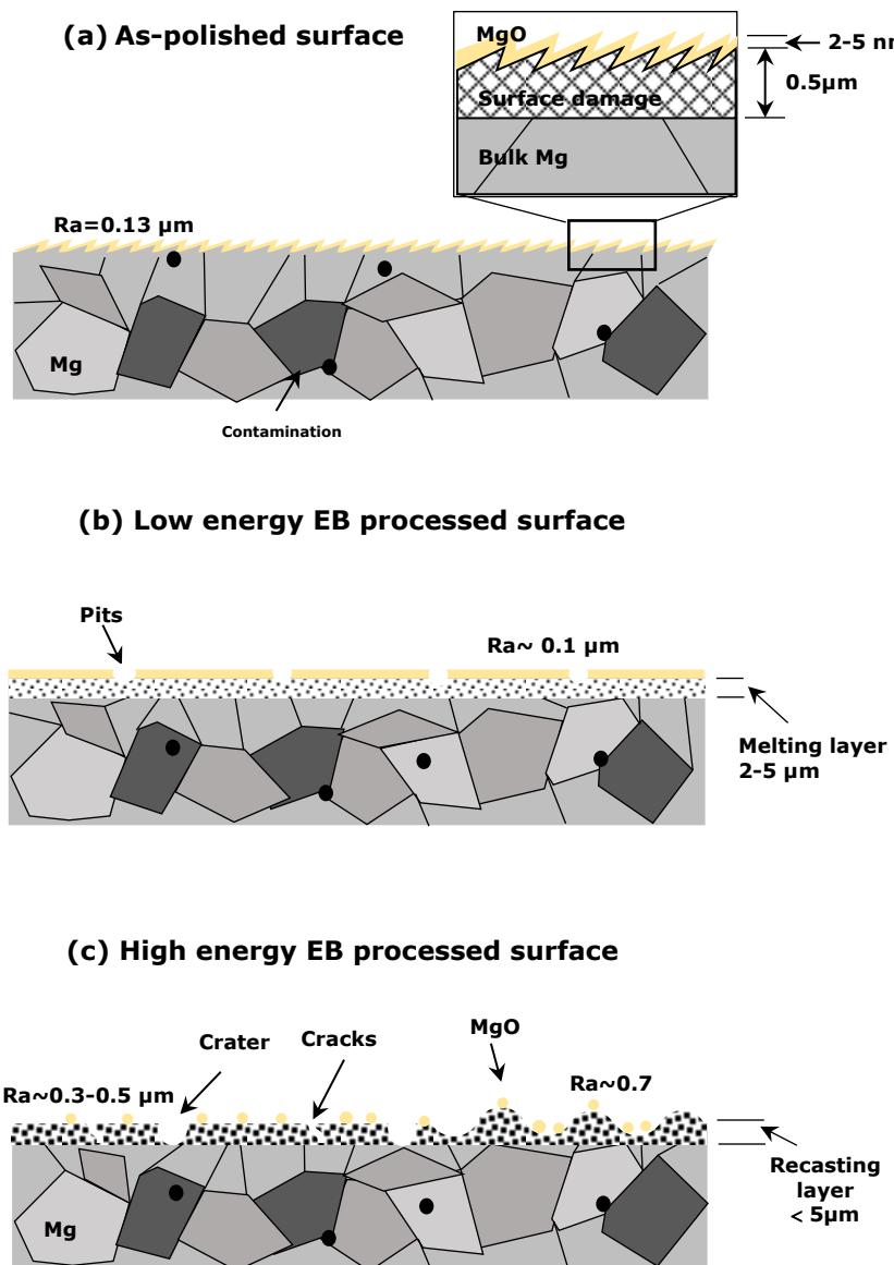
**Figure 6-18** Schematic of LAEB modification of Mg surface: (a) as-polished Mg surface; (b) low energy EB processed Mg surface; (c) over processed - high energy EB processed Mg surface. Note in (c) the RHS represents the edge region while the LHS of the schematic represents the central region.
