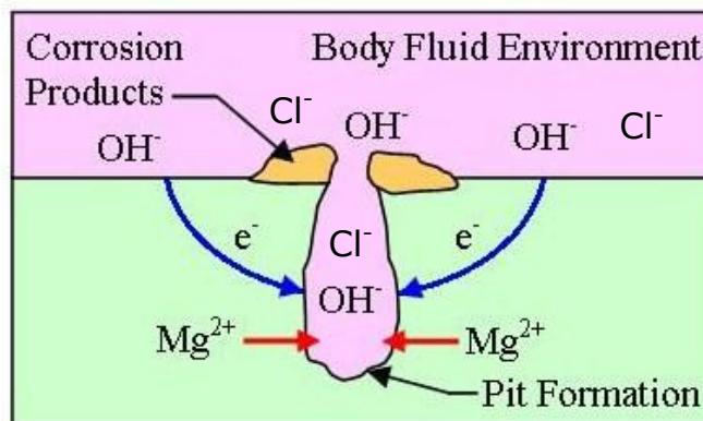
**Figure 2-12** Pitting corrosion on the surface of Mg [99].
