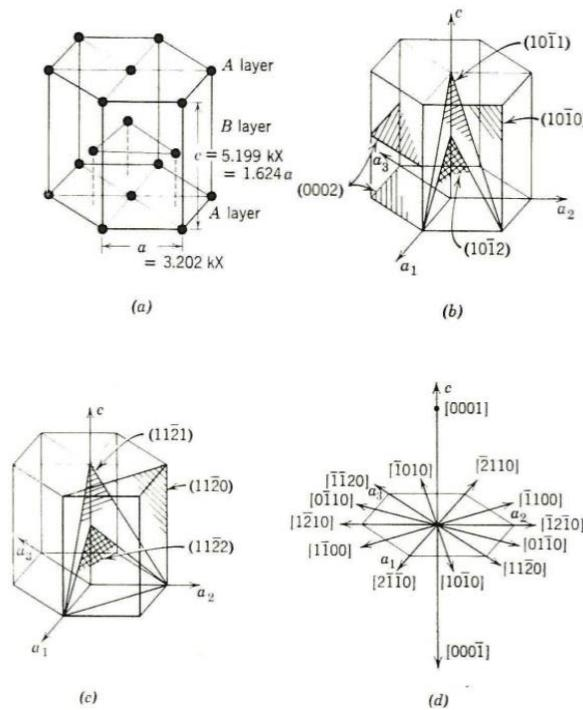
**Figure 2-6** Magnesium crystal structure: a) lattice positions; b,c) principle basal, pyramidal and prismatic planes; d) principal directions [73].
