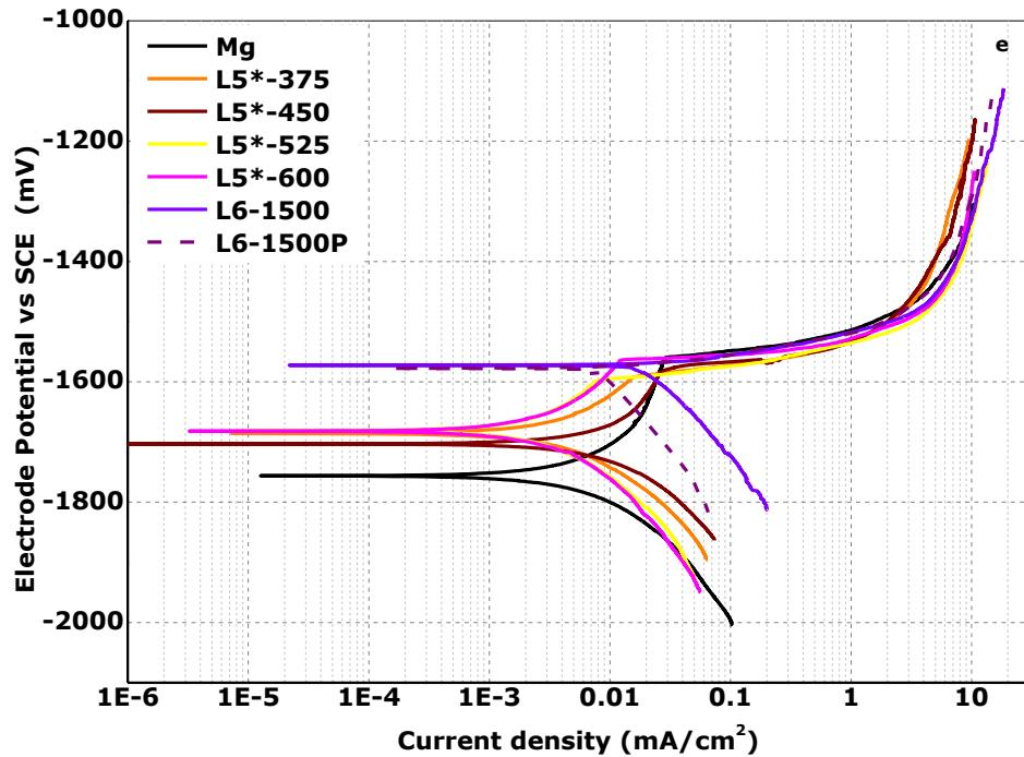
**Figure 6-26** continued... potentiodynamic polarization curves for as-prepared and LSM processed Mg-surfaces for scanning speeds of: (e) 5400 and 6300 mm/min (spot size 3 mm).
