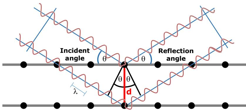
**Figure 3-8** Schematic illustration of constructive interference of scattered waves (Bragg diffraction:  $n\lambda = 2d \sin \theta$ ) [236]
