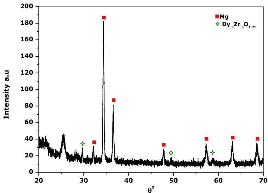
**Figure 4-3** XRD pattern from a commercial prototype Mg-alloy stent. Showing strong diffraction peaks for Mg and lower intensities matching  $\text{Dy}_{0.5}\text{Zr}_{0.5}\text{O}_{1.75}$  (data card number: 01-078-1293)
