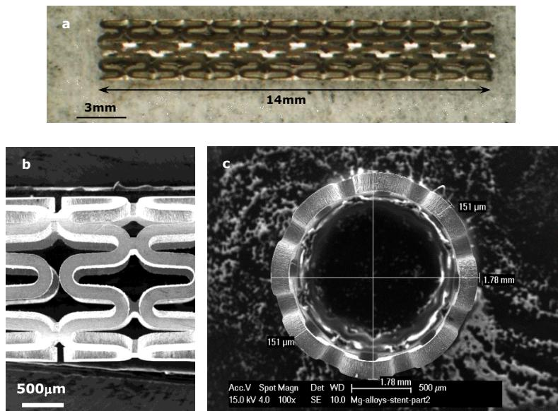
**Figure 4-1** Images of a commercial prototype Mg-alloy stent: (a) OM image of laser-cut stent made from Mg-alloy tube; (b) SE image of stent zigzag loops before expansion; and (c) SE image of circular end showing dimensions of the stent.
