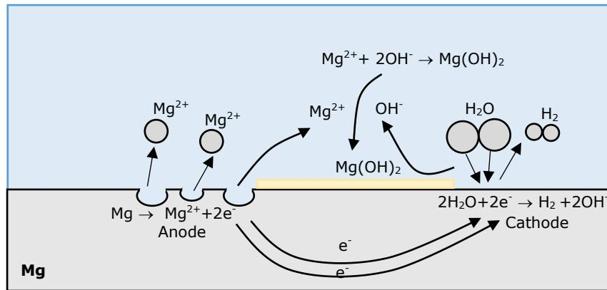
**Figure 2-8** Coupled electrochemical reactions occurring at different sites on a Mg surface in aqueous solution
