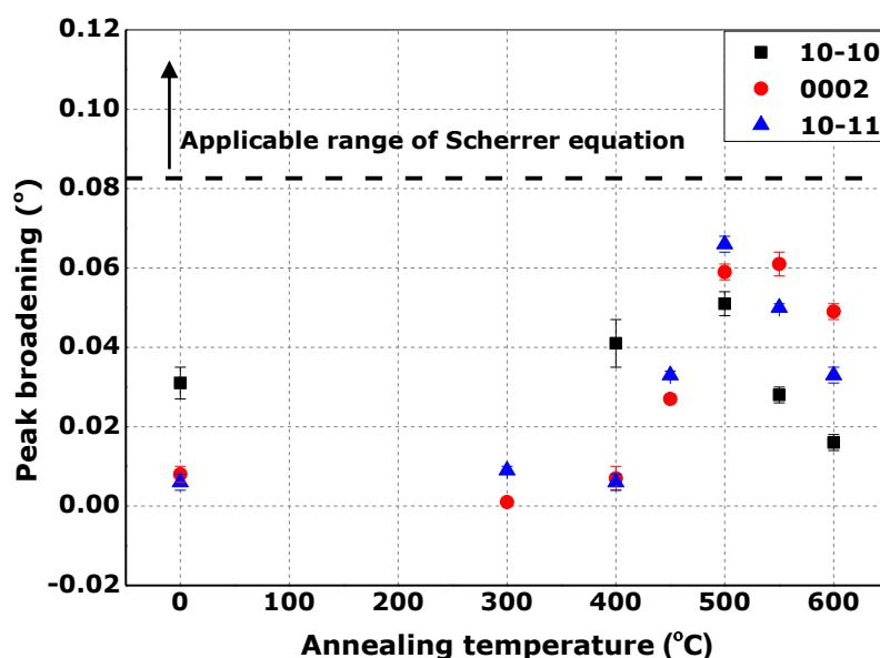
**Figure 4-15** Peak broadening of Mg  $10\bar{1}0$ , 0002 and  $10\bar{1}1$  diffraction peaks for different annealing temperatures.
