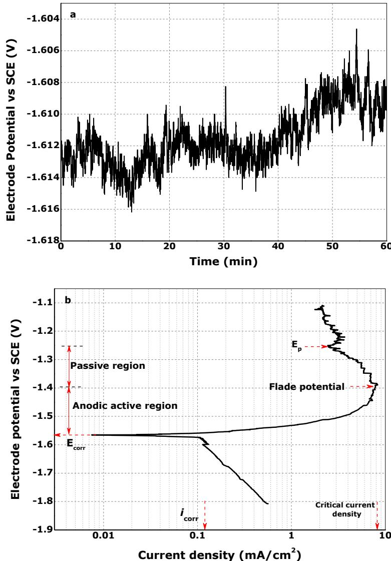
**Figure 4-4** (a) OCP; and (b) Potentiodynamic polarization curves for the commercial prototype Mg-alloy stent, in PBS at 37°C.
