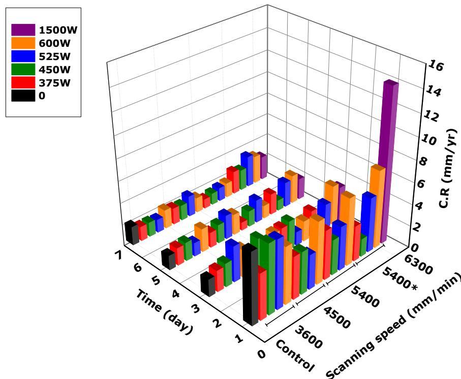
**Figure 6-28** Corrosion rate data for Mg and LSM modified Mg surfaces immersed up to 7 days in PBS at 37°C.
