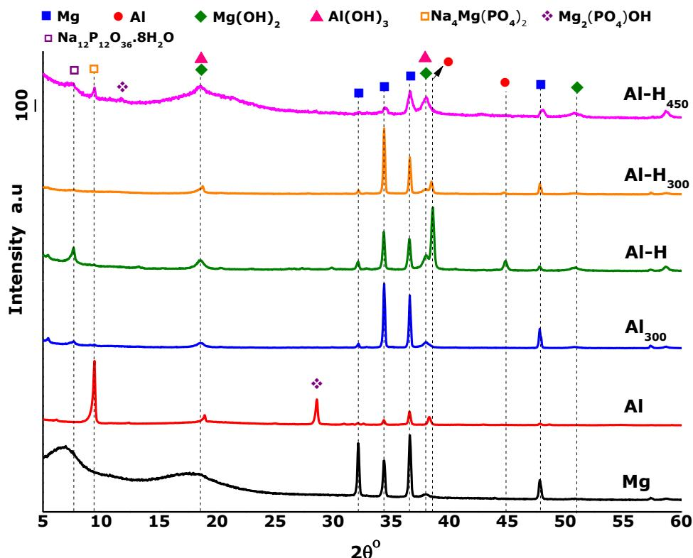
**Figure 5-11** XRD patterns of as-deposited and heat-treated Al and Al-H coatings on Mg substrates after potentiodynamic polarization corrosion tests in PBS at 37°C.
