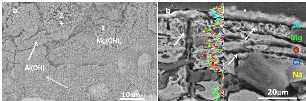
**Figure 5-10** BSE images of corrosion morphologies of: (a) as-deposited Al-H in plan-view; and (b) as-deposited Al coating in cross-sectional view, after potentiodynamic polarization corrosion testing.
