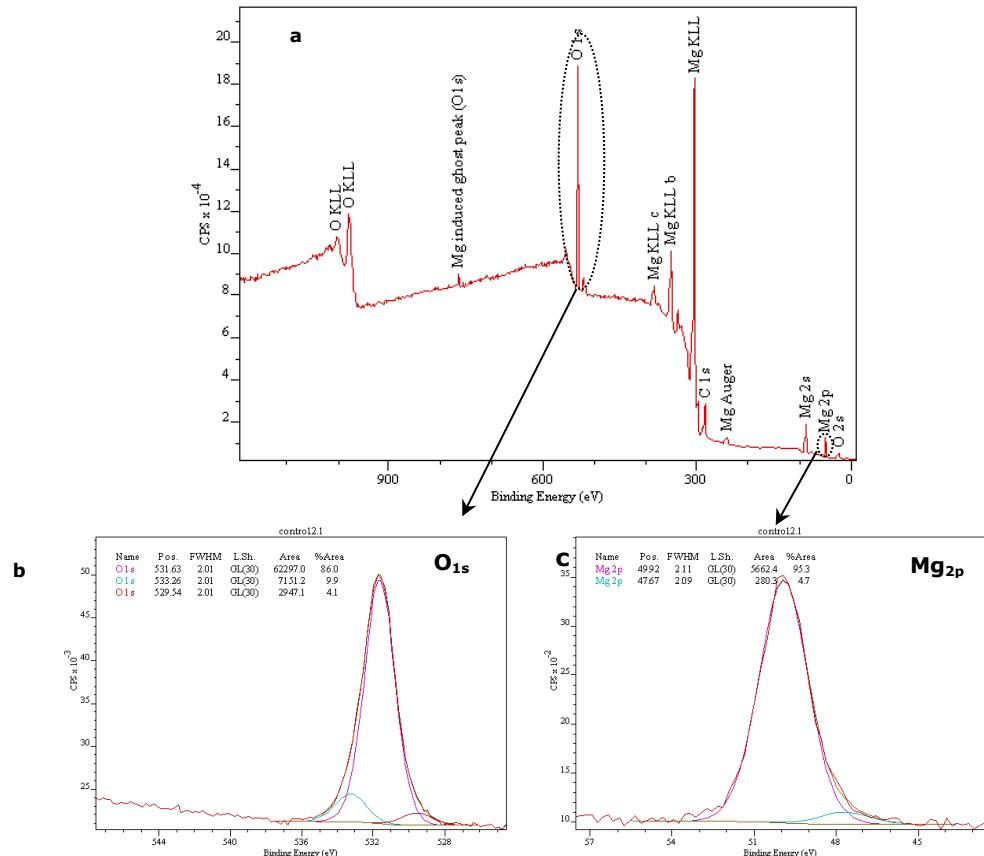
**Figure 5-18** XP-survey scan and high-resolution O<sub>1s</sub> and Mg<sub>2p</sub> spectra of the Mg substrate.
