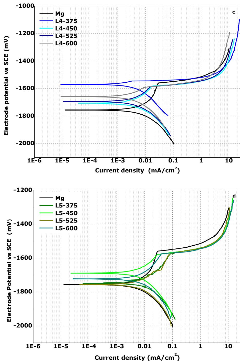
**Figure 6-26** continued..., potentiodynamic polarization curves for as-prepared and LSM processed Mg-surfaces for scanning speeds of: (c) 4500 mm/minute, and (d) 5400 mm/minute(spot size 2 mm)
