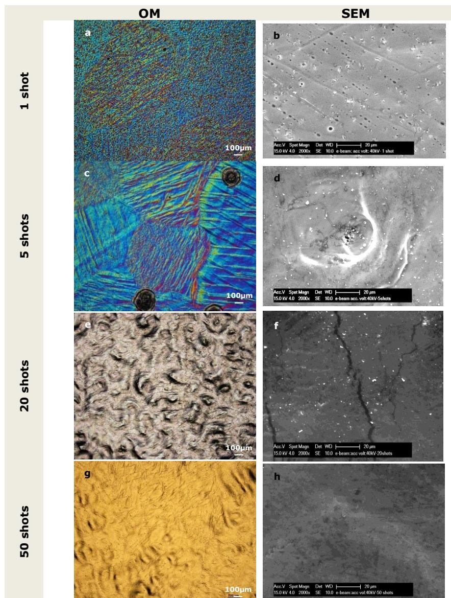
**Figure 6-4** OM and SE images of Mg surface modified by LAEB processing (40 kV; 1, 5, 20 and 50 pulses).
