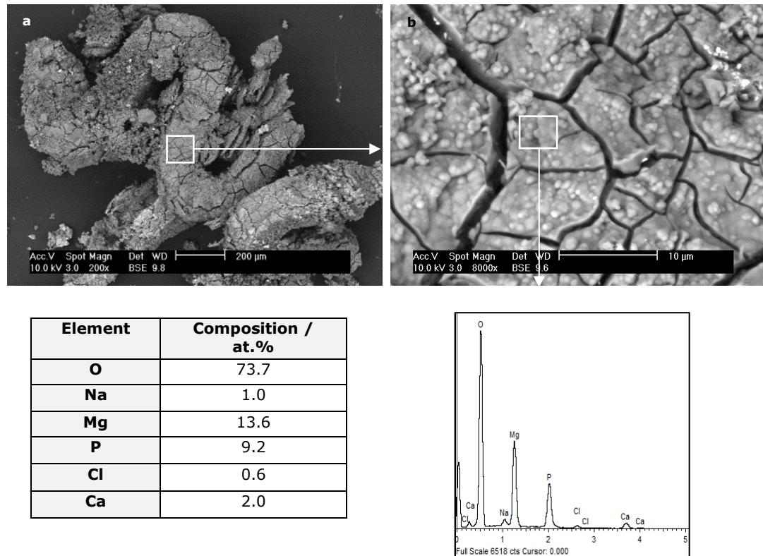
**Figure 4-5** BSE images and associated ED spectrum of a commercial prototype Mg-alloy stent after potentiodynamic polarization testing.
