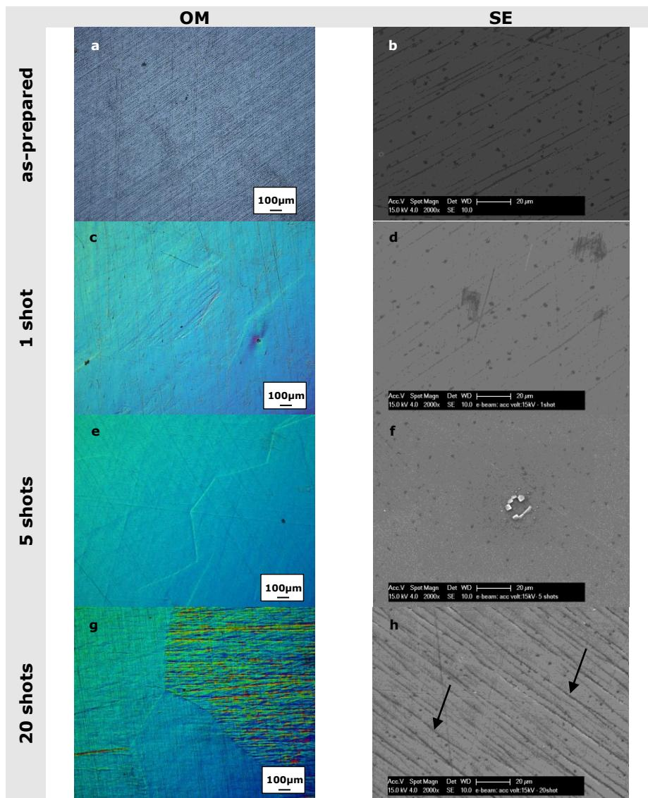
**Figure 6-1** OM and SE images of Mg surfaces modified by LAEB processing (15 kV; 1, 5 and 20 pulses), arrows indicate the presence of polishing damage on the Mg surface.
