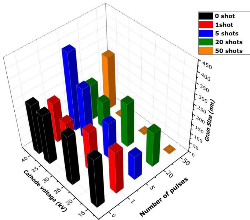
**Figure 6-12** Average grain size of Mg samples irradiated by LAEB as a function of cathode voltage and number of shots
