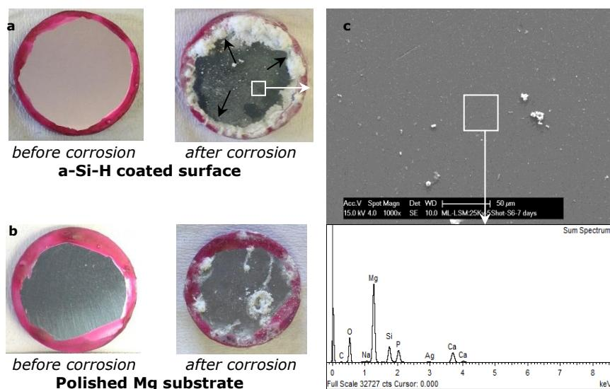
**Figure 5-22** OM images, SE image and ED spectrum for corroded a-Si:H coated Mg, after immersion in PBS at  $37^\circ\text{C}$  for 7 days.
