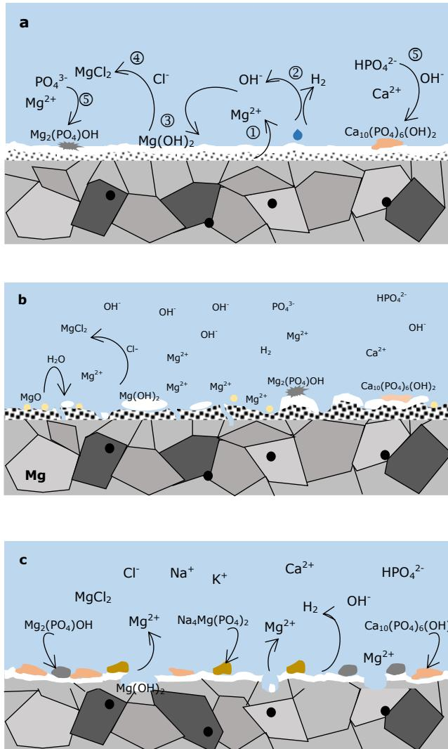
**Figure 6-19** Schematic illustration of corrosion mechanism of EB- Mg modified surface: (a) Low energy EB processed surface at initial stage of corrosion; (b) high energy EB processed surface at initial stage of corrosion; (c) corrosion of Mg after dissolution of modified layer
