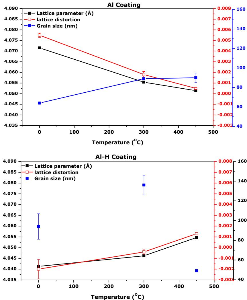
**Figure 5-13** Variation of Al lattice parameter, lattice distortion and grain size as a function of annealing temperature.
