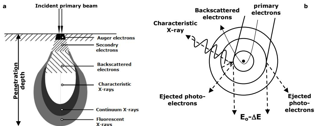
**Figure 3-7** (a) Volume of interaction of incident electron beam with material; (b) the origin of backscattered electrons (BSE) and characteristic X-rays.
