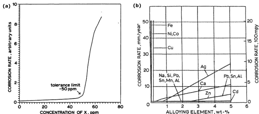
**Figure 2-17 (a)** General curve showing the effect of an impurity element (x) on the corrosion rate of Mg; the corrosion rate increases rapidly above the tolerance limit of  $\sim 50$  ppm. (b) The effect of alloying additions on corrosion behaviour of binary Mg-alloys in 3% NaCl solution [127].
