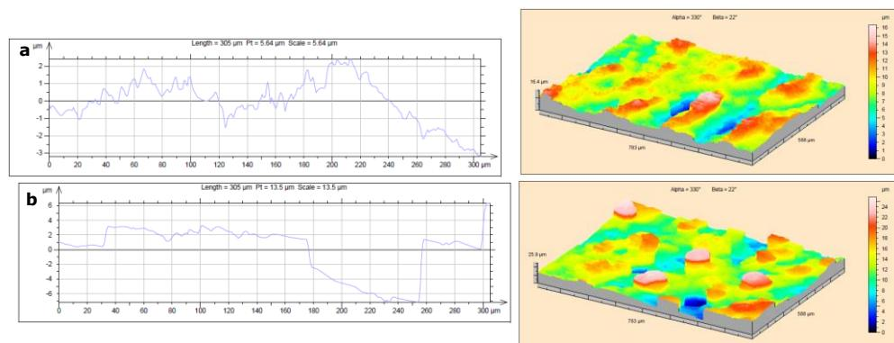
**Figure 6-9** Surface roughness profiles for LAEB processed Mg (40 kV cathode voltage; 50 pulses): (a) Middle region; and (b) edge region.
