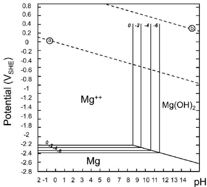
**Figure 2-18** E-pH diagram for Mg in  $H_2O$  at  $25^\circ C$ ; the water stability region lies between the (a) and (b) lines. At potentials below (a), hydrogen is evolved; whilst above (b), oxygen is evolved. (Adapted from [112] [131]).
