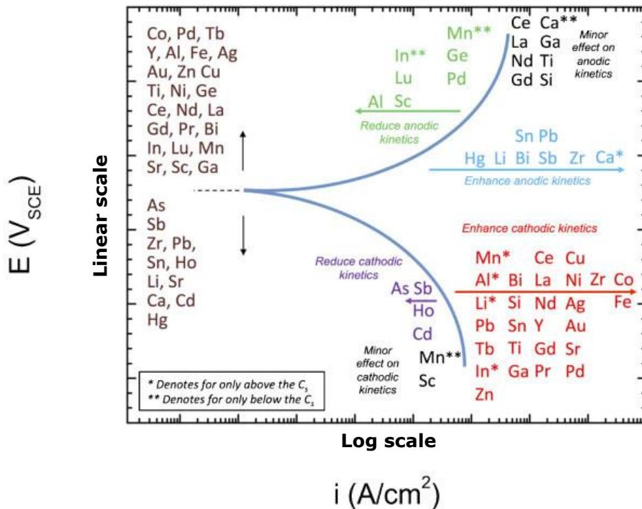
**Figure 2-23** Schematic representation of electrochemical effect of alloying elements. Plot shows the ability of alloying additions to modify anodic or cathodic kinetics (or both), leading to changes in the resultant corrosion rate ( $i_{corr}$ ), along with changes in corrosion potential ( $E_{corr}$ ). CS represents solid solubility [112].
