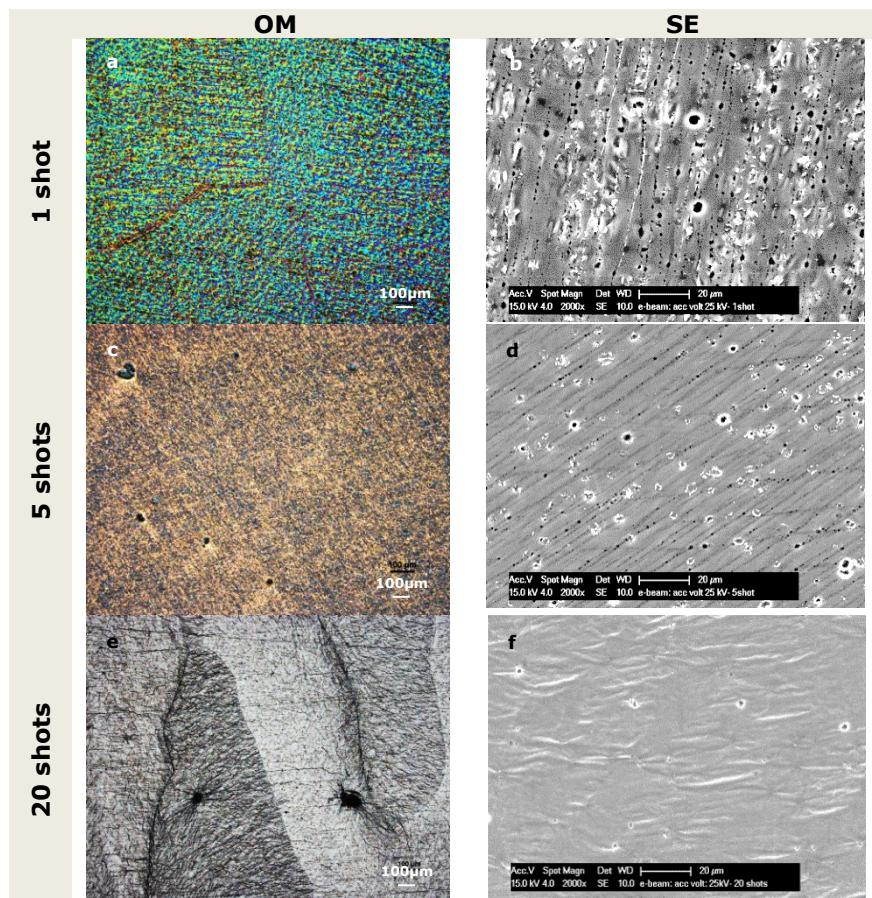
**Figure 6-2** OM and SE images of Mg surfaces modified by LAEB processing (25 kV; 1, 5 and 20 pulses)
