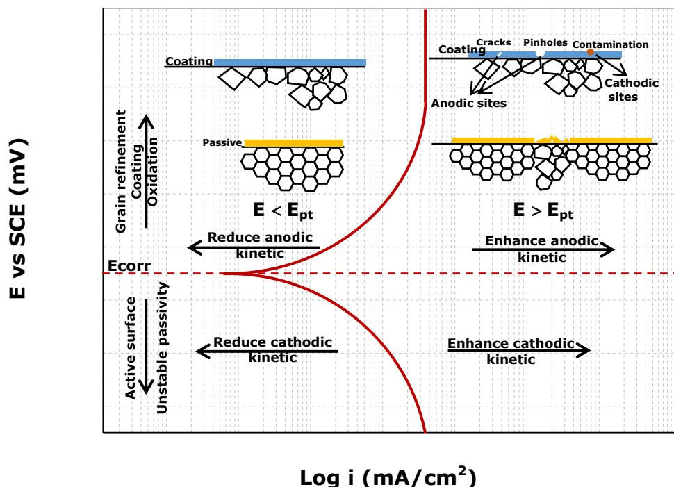
**Figure 7-1** Schematic diagram summarising the effects of surface modification processes on the corrosion kinetics of pure Mg
