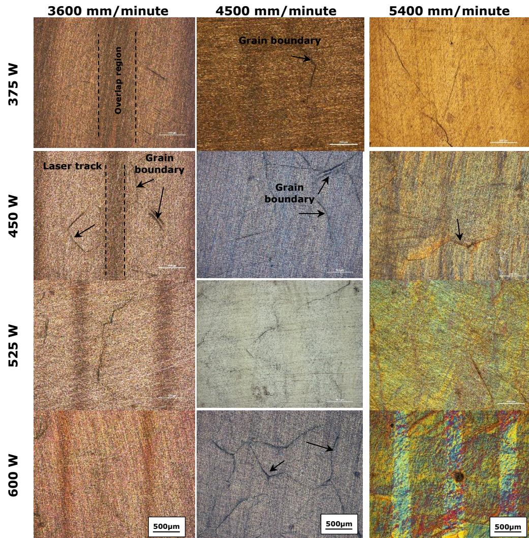
**Figure 6-20** OM images of Mg surfaces following LSM modification.
