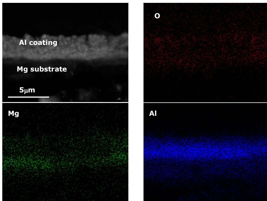
**Figure 5-5** EDS elemental maps of Al-H<sub>300</sub> coated Mg in cross-section, after heat treatment at 300°C
