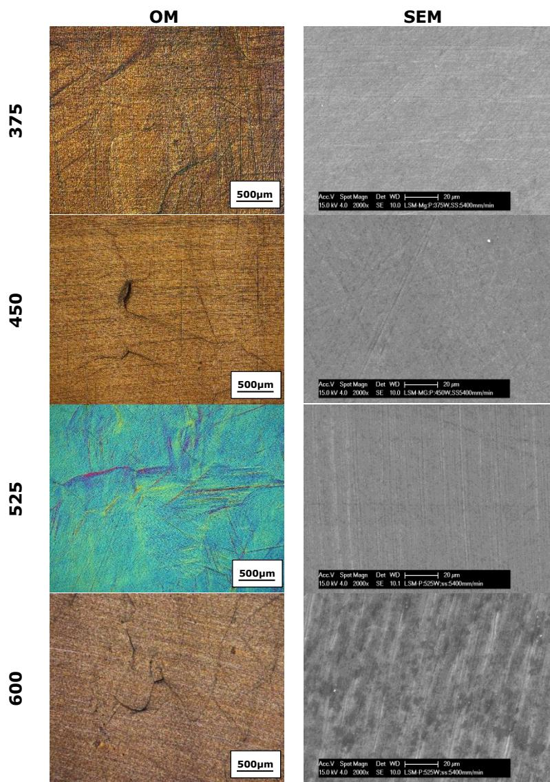
**Figure 6-22** OM and SE images of Mg surfaces LSM processed at 5400 mm/minute with a laser spot size of 3 mm.
