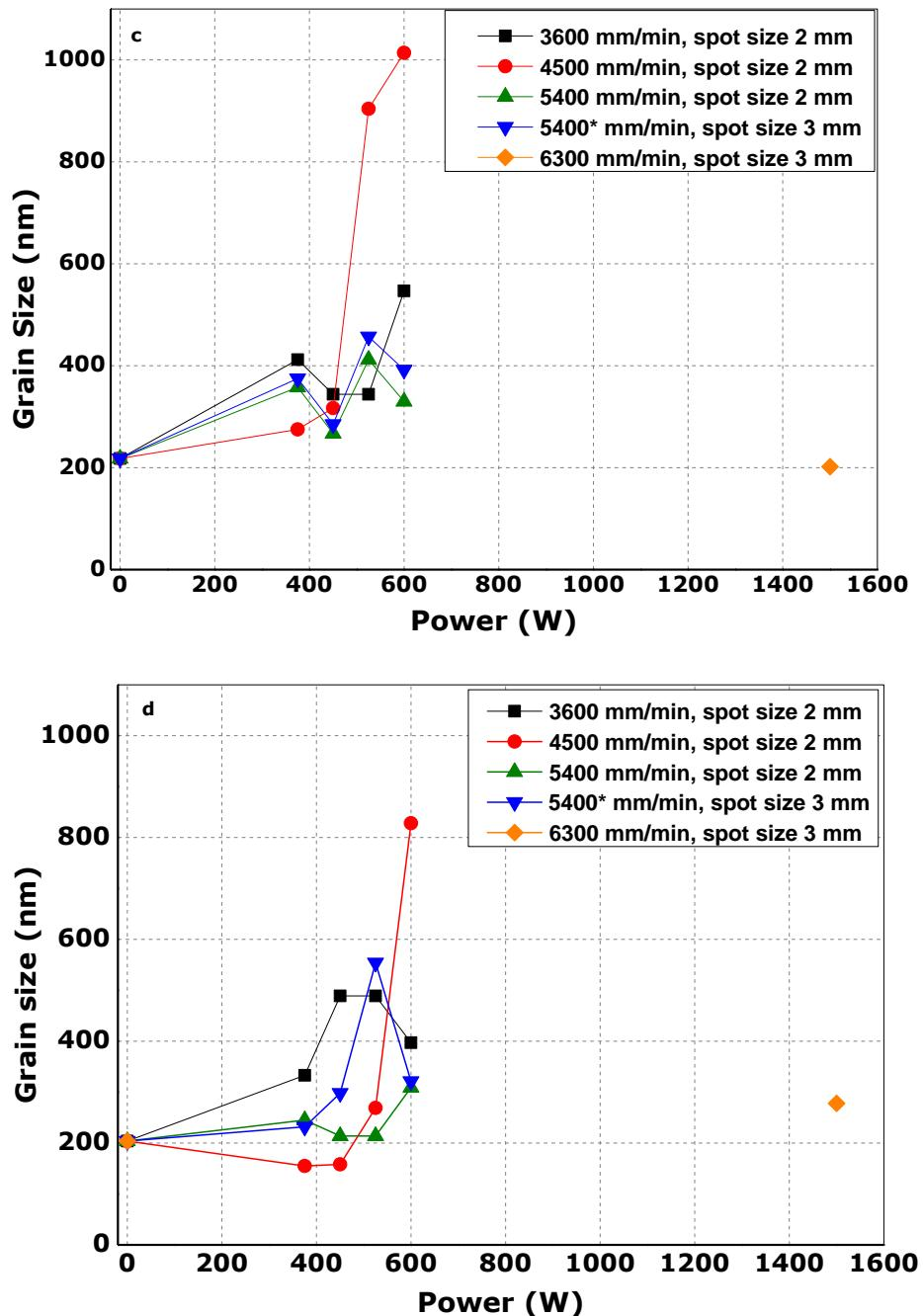
**Figure 6-25** continued... Grain size values from: (c) 0002 and (d) 10 $\bar{1}$ 1 diffraction peaks.
