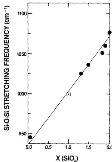
**Figure 5-24** Si-O-Si stretching vibrations as a function of oxygen composition in  $\text{SiO}_x$  [313].
