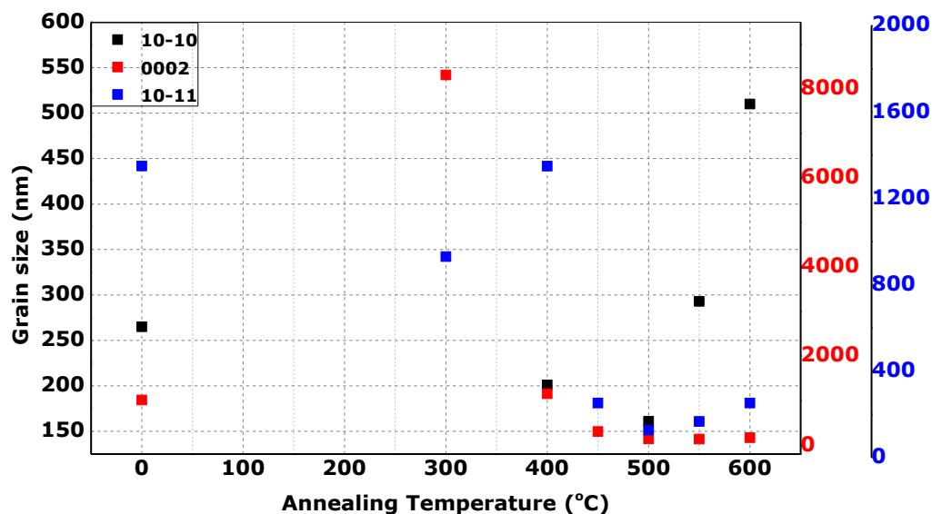
**Figure 4-16** Grain size variation of Mg for as-deposited and annealed Mg minitubes, determined from three different planes.
