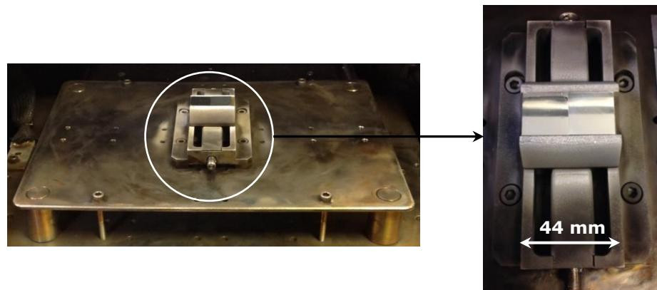
**Figure 3-5** Sample stage and holder for the Sodick PF32A LAEB machine.
