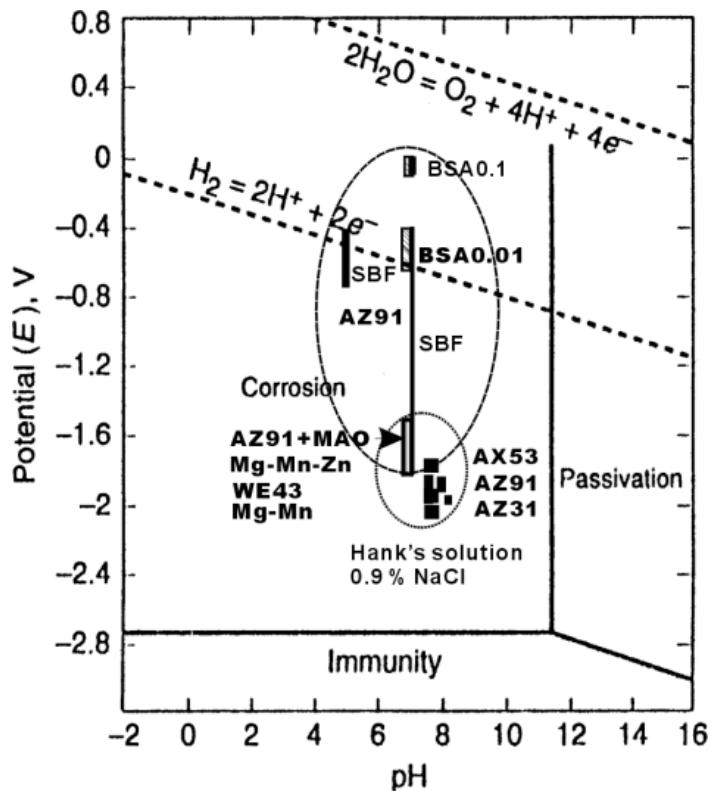
**Figure 2-19** pH-potential diagram of Mg and its alloys in various SBF and bovine serum albumin (BSA) [27]
