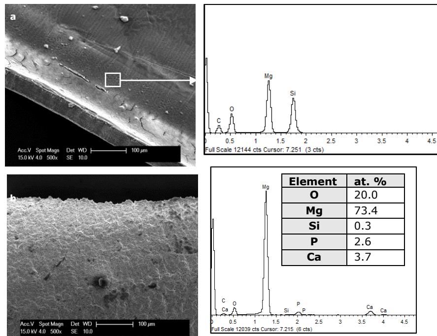
**Figure 4-9** ED spectra acquired from the (a) internal surface; and (b) outer surface of a fragment of an as-deposited Mg minitube
