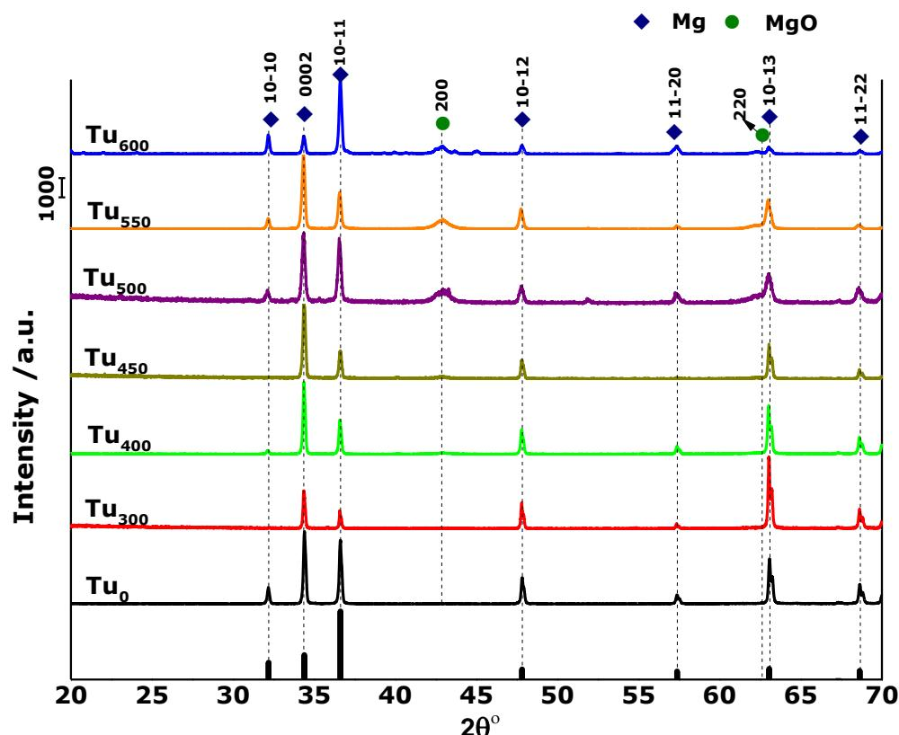
**Figure 4-14** XRD patterns of the Mg minitubes, as-deposited and following annealing for 24 h ( $300 - 600^{\circ}\text{C}$ ). (Expected intensities for polycrystalline Mg peaks presumably for equiaxed grains:  $10\bar{1}0$ , 25;  $0002$ , 36;  $10\bar{1}1$ , 100;  $10\bar{1}2$ , 15;  $11\bar{2}0$ , 12;  $10\bar{1}3$ , 16; and  $11\bar{2}2$ , 13).
