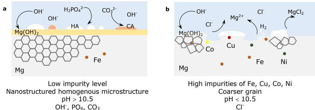
**Figure 2-20** Schematic diagram summarising parameters: (a) positively and (b) negatively affecting the corrosion behaviour of Mg.
