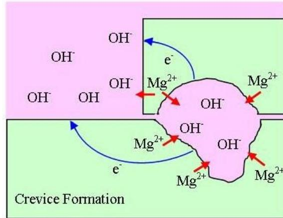
**Figure 2-13** Crevice corrosion of Mg in solution [99].
