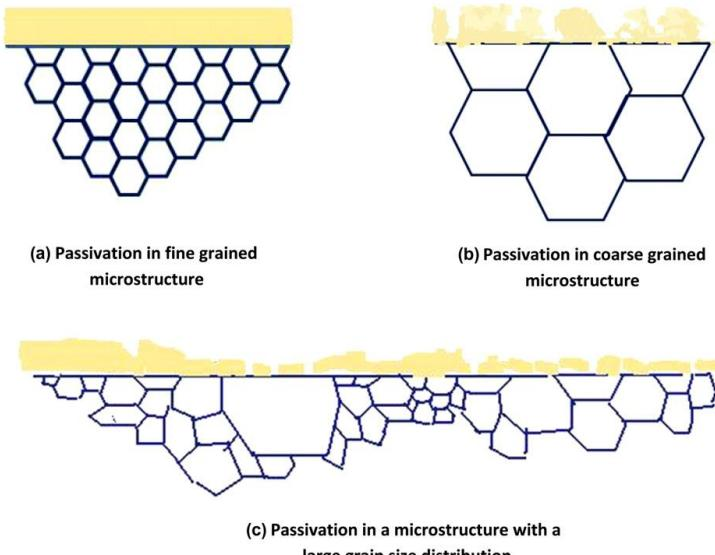
**Figure 2-16** Formation of passive layers in: (a) a fine-grained microstructure; (b) a coarse-grained microstructure; and (c) a microstructure with a large grain size distribution [124].
