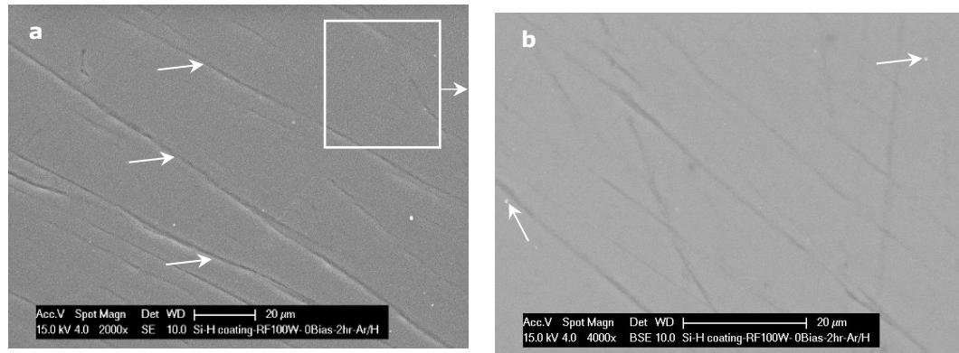
**Figure 5-15** (a) SE and (b) BSE images of RF-MS coated a-Si:H /Mg.
