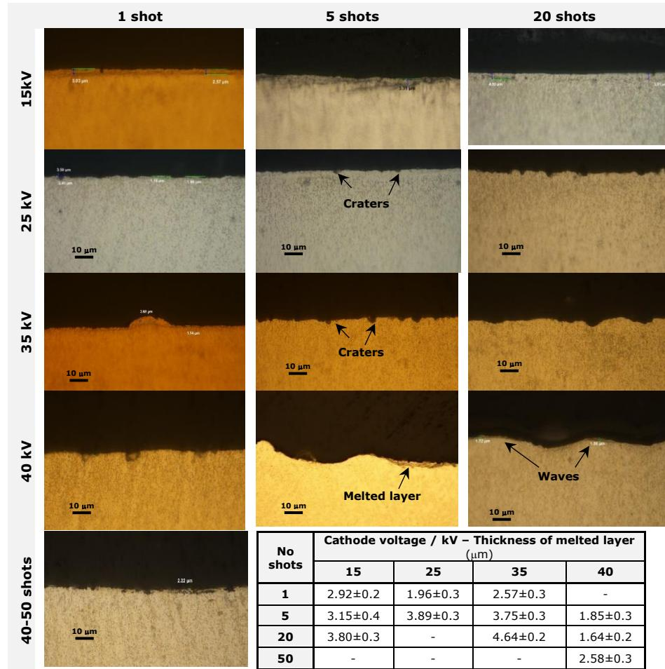
**Figure 6-7** OM images showing cross sectional morphologies of LAEB treated Mg; Table summarising melted layer thicknesses in  $\mu\text{m}$ . The bar in the images represents 10  $\mu\text{m}$ .
