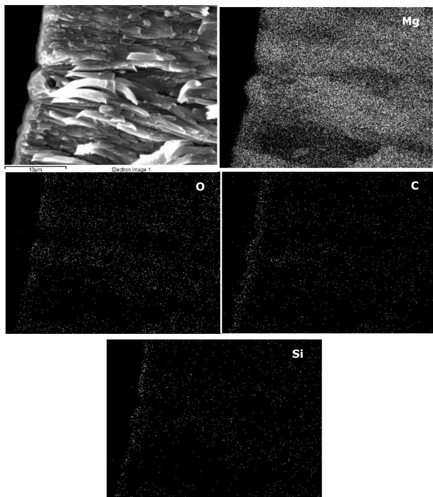
**Figure 4-10** EDS elemental map for an as-deposited minitube in cross-section, showing Mg and the enhancement of Si, C and O at the internal edge (associated SE image).
