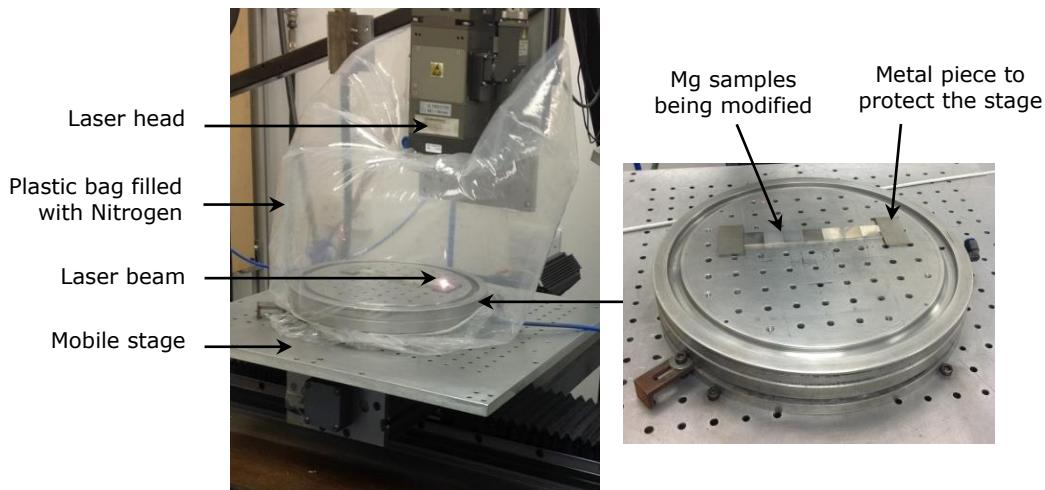
**Figure 3-6** LSM processing arrangement.
