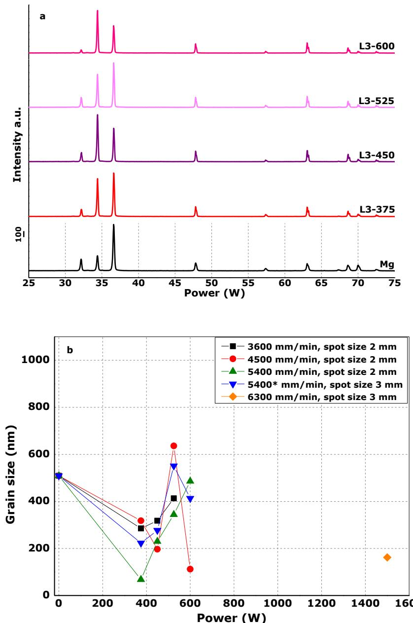
**Figure 6-25** (a) XRD patterns of as-prepared and LSM processed Mg surfaces, as a function of laser power (at 3600 mm/minute scan speed); and grain size values from: (b)  $10\bar{1}0$ , (c)  $0002$  and (d)  $10\bar{1}1$  diffraction peaks.
