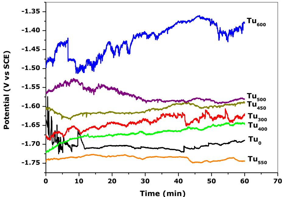
**Figure 4-18** OCP data for as-deposited & annealed Mg-minitubes in PBS at 37°C.
