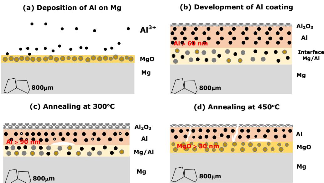
**Figure 5-12** Schematic diagrams illustrating the deposition and evolution of Al deposited coatings on Mg, as a function of annealing.
