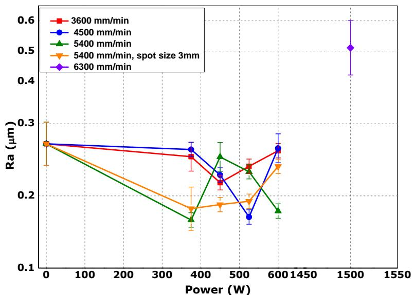
**Figure 6-24** Mg surface roughness ( $R_a$ ) as a function of laser power and scan speed.
