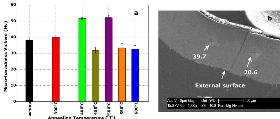
**Figure 4-17** (a) Micro-hardness values for as-deposited and annealed Mg-minitubes, as a function of annealing temperature and corresponding standard error; (b) SE image of Vickers micro-hardness indentation patterns on an as-deposited Mg minitube.
