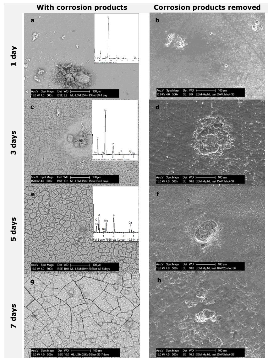
**Figure 6-17** BSE and SE images of corroded LAEB-treated Mg surfaces, after immersion in PBS for 1,3,5 and 7 days
