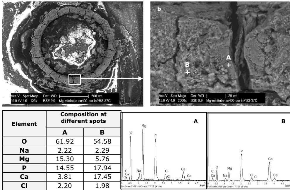
**Figure 4-20** (a,b) BSE images of the corrosion topography of an Mg-minitube annealed at 400°C, after potentiodynamic polarisation testing.
