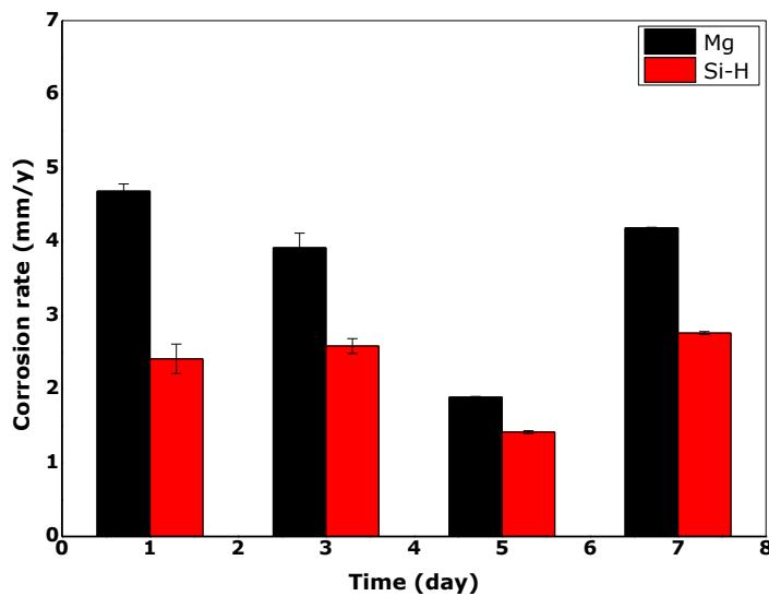
**Figure 5-21** Corrosion rates of the as-polished Mg substrate and a-Si:H coated Mg, after 1, 3, 5 and 7 days.
