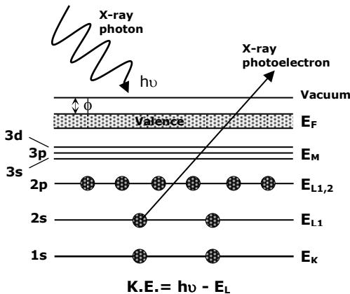
**Figure 3-9** Emission of a photoelectron;  $h\nu$  is the X-ray photon energy and  $E_L$  is the binding energy of the photoelectron from an inner core shell [237]
