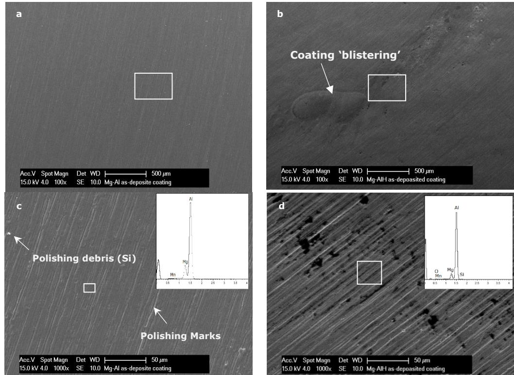
**Figure 5-2** SE images of as-deposited coatings on polished Mg substrates: (a) Al deposited in Ar; (b) Al-H deposited in Ar/H<sub>2</sub>; (c) high magnification of as-deposited Al with EDS inset; and (d) high magnification, as-deposited Al-H, with EDS inset.
