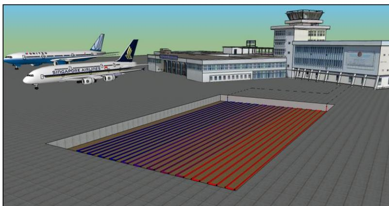
Figure 5- A PSHP under a thick concrete pavement in Airport
