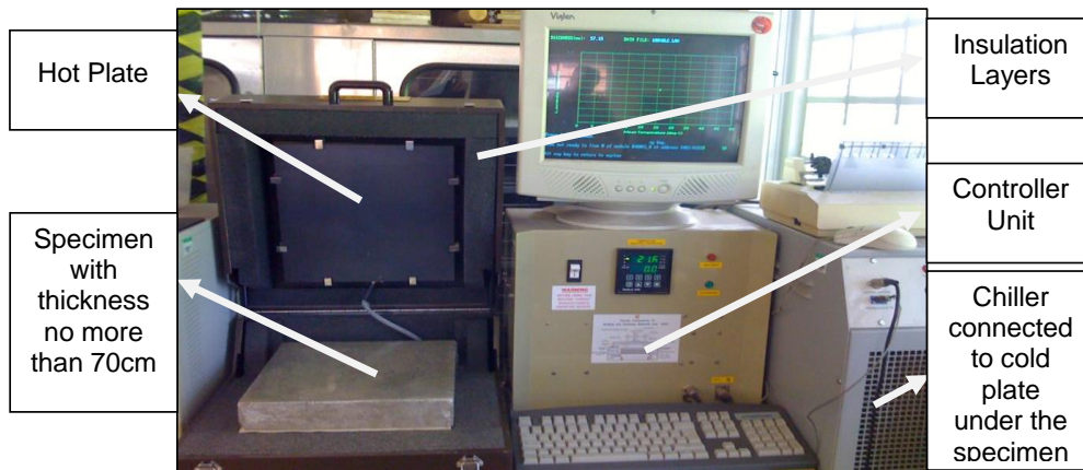
Figure 9- apparatus to measure thermal conductivity of building materials
