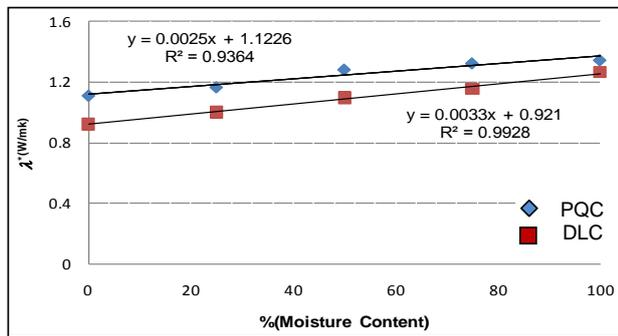
Figure 10-Moisture-dependent thermal conductivity of PQC and DLC
