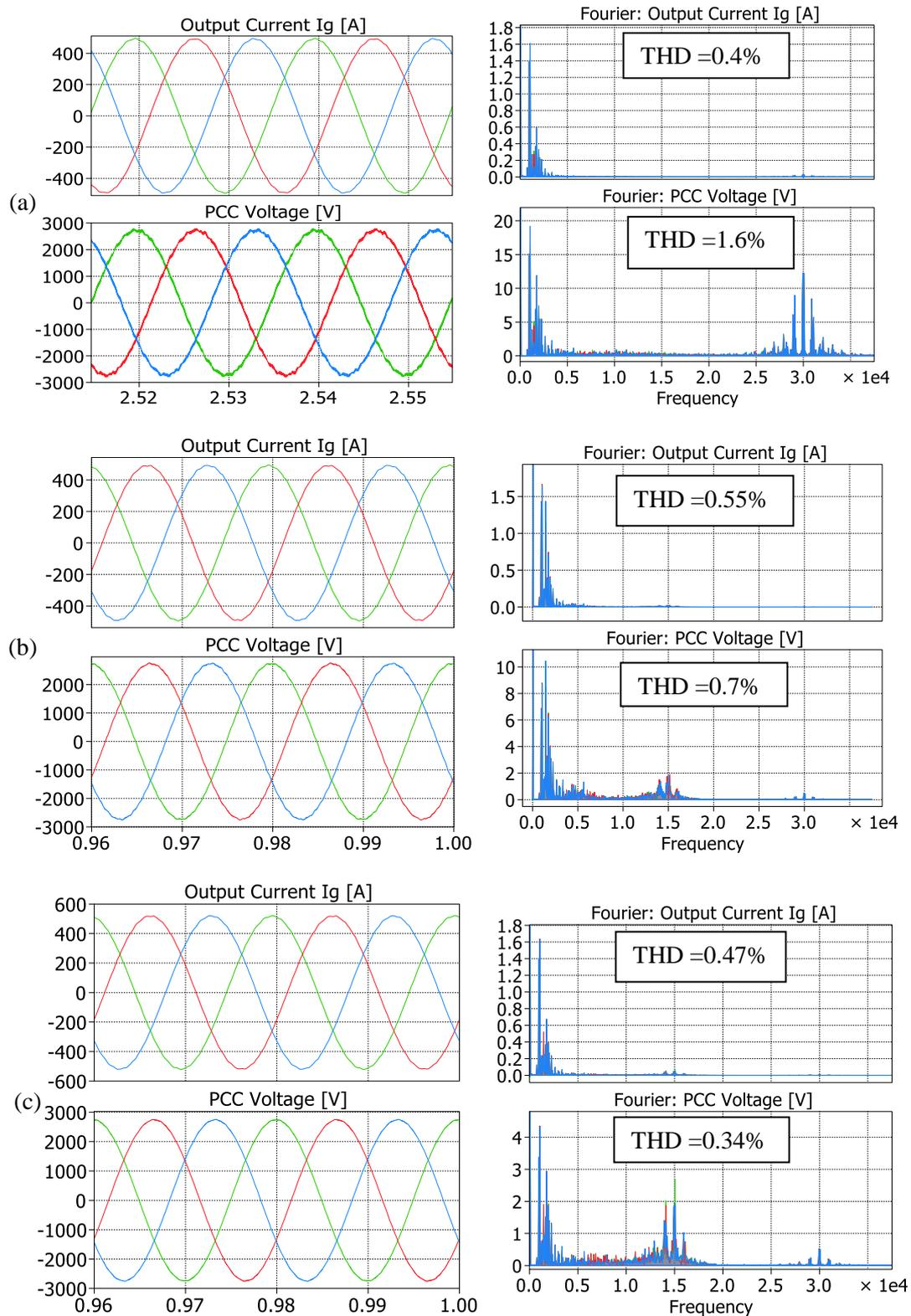
Fig. 4-19a-c: Steady state output current and PCC voltage during active filtering a)without voltage filtering b)using  $C_{f0}/R_{f0}$  and  $L_2=2.8\text{mH}$ ,  $L_g=0.8\text{mH}$  and using  $C_{f0}/R_{f0}$  and  $L_2=2.8\text{mH}$ ,  $L_g=0.4\text{mH}$  (50% grid impedance variation). Corresponding FFT shown on the right column.
