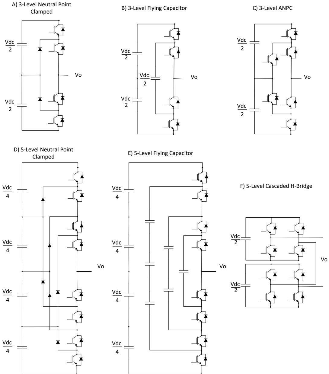
Fig. 2-1: Single phase representation of multilevel topologies: a) 3-level NPC ; b) 3-level FLC; c) 3-level ANPC; d) 5-level NPC; e) 5-level FLC and e) 5-level CHB
