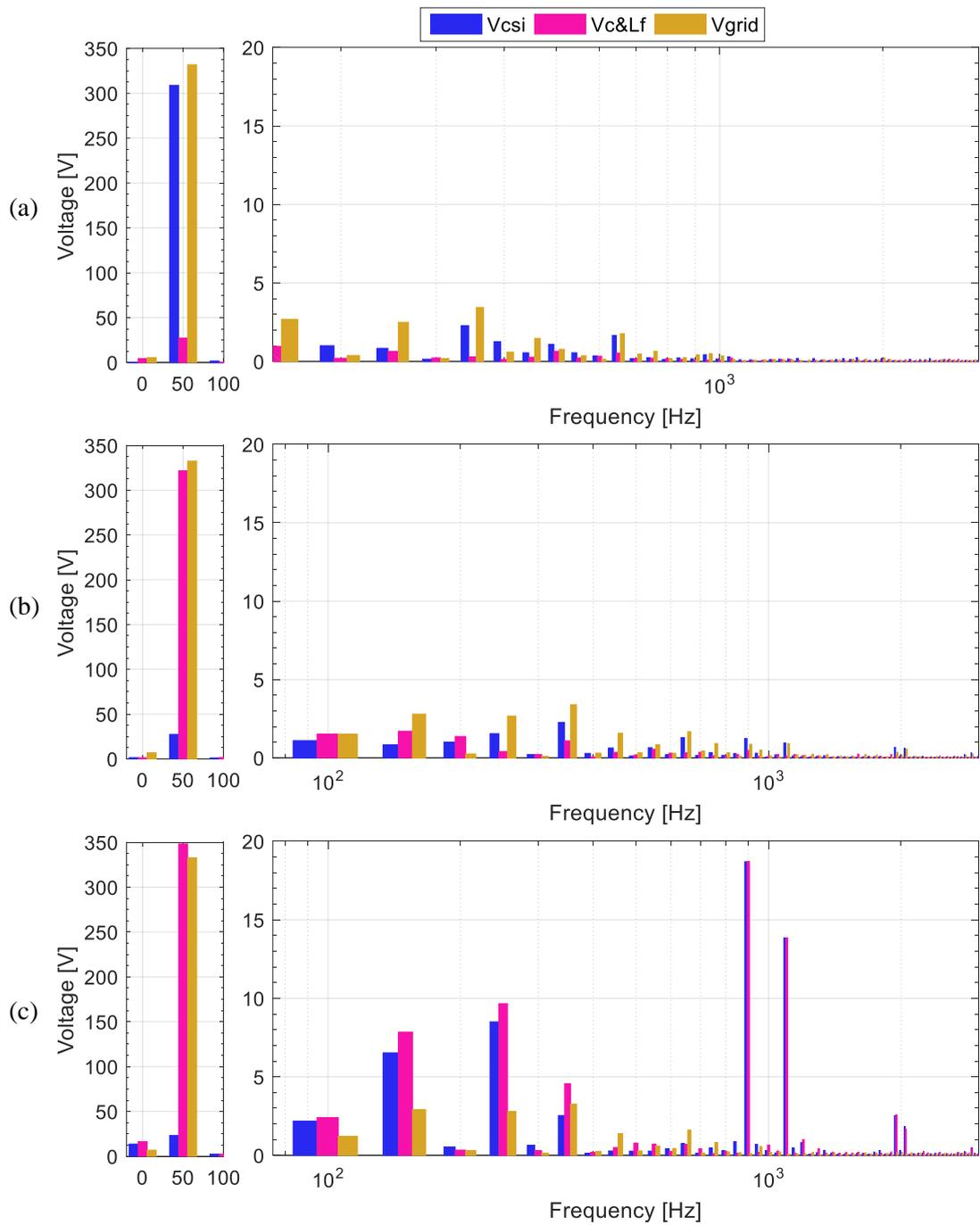
Fig 7-9: FFT of Phase A voltage of the Grid ( $V_{grid}$ ), Series capacitor ( $V_{c\&Lf}$ ) and CSI phase voltage ( $V_{csi}$ ) during: a) No PWM; b) PWM enabled showing fundamental voltage reduction; and c) full system operation (harmonic cancellation).
