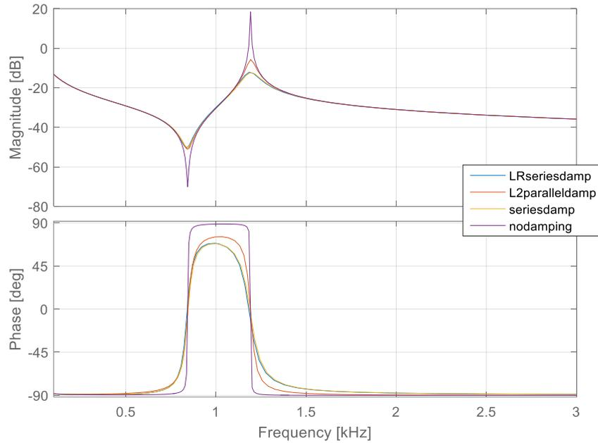
Fig. 4-9: Frequency response under different passive damping scenarios
