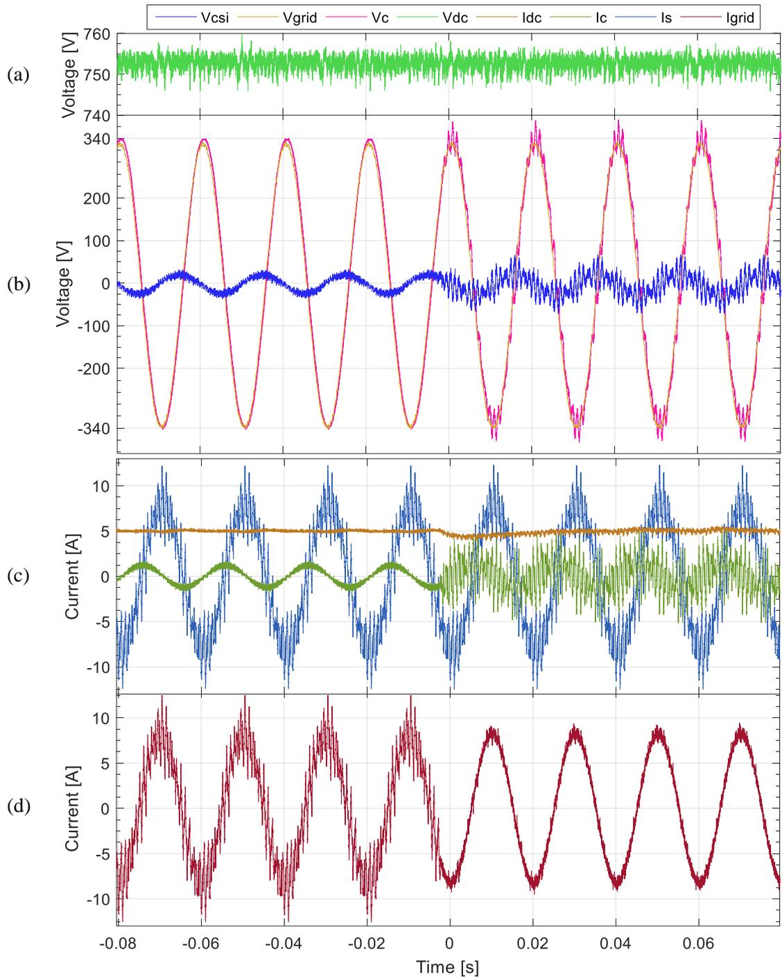
Fig 6-3: Experimental results showing activation of ripple cancellation for VSI and CSI for  $K=0.1$  for Phase A: a) VSI DC-link voltage ( $V_{dc}$ ); b) Series capacitor ( $V_c$ ), CSI ( $V_{csi}$ ) and grid ( $V_{grid}$ ) phase voltages; c) CSI DC-link current ( $I_{dc}$ ), Main VSI current ( $I_s$ ) and series capacitor current ( $I_c$ ); and d) combined grid side current ( $I_{grid}$ ).
