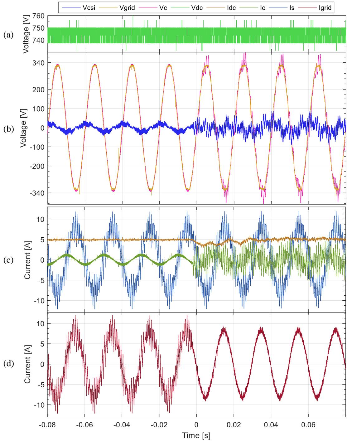
Fig 7-30: Experimental results showing activation of ripple cancellation for VSI and CSI for  $K=0.12$  for Phase A: a) VSI DC-link voltage ( $V_{dc}$ ); b) Series capacitor ( $V_c$ ), CSI ( $V_{csi}$ ) and grid ( $V_{grid}$ ) phase voltages; c) CSI DC-link current ( $I_{dc}$ ), Main VSI current ( $I_s$ ) and series capacitor current ( $I_c$ ); and d) combined grid side current ( $I_{grid}$ ).
