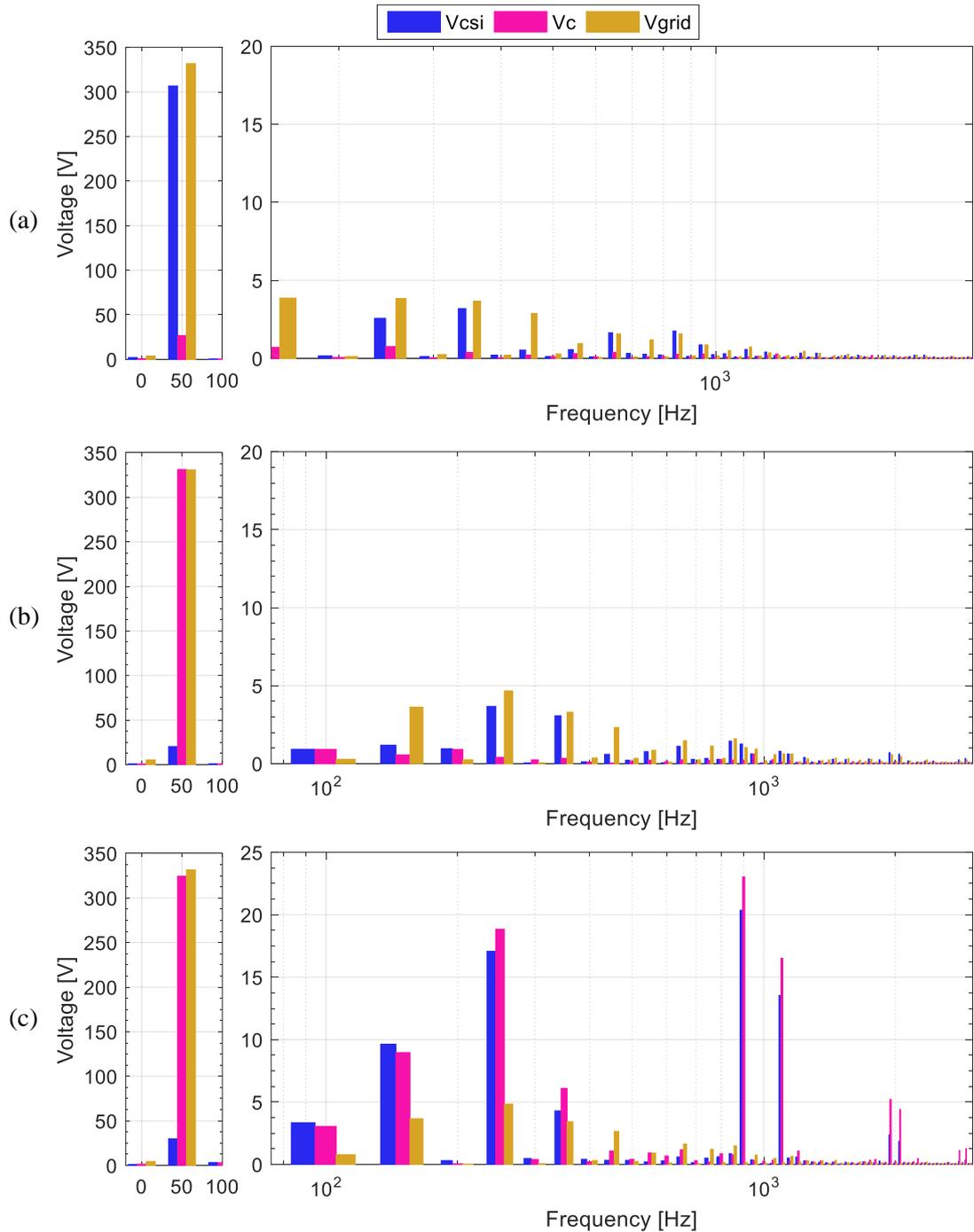
Fig 7-33: FFT of Phase A voltage of the Grid ( $V_g$ ), Series capacitor ( $V_c$ ) and CSI phase voltage ( $V_{csi}$ ) during: a) No PWM; b) PWM enabled showing fundamental voltage reduction; and c) full system operation (harmonic cancellation).
