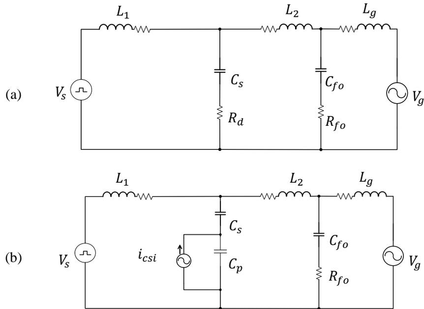
Fig. 4-17a-b: Single Phase Equivalent Circuit with output RC filter during: a) passive filtering; and b) during active filtering.
