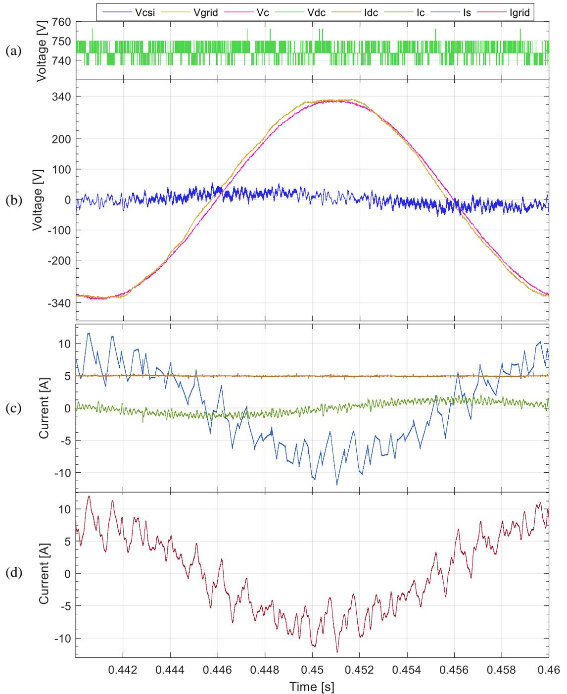
Fig 7-41: Experimental results showing one steady state cycle before ripple cancellation for VSI and CSI for  $K=0.12$  for Phase A: a) VSI DC-link voltage ( $V_{dc}$ ); b) Series capacitor ( $V_c$ ), CSI ( $V_{csi}$ ) and grid ( $V_{grid}$ ) phase voltages; c) CSI DC-link current ( $I_{dc}$ ), Main VSI current ( $I_s$ ) and series capacitor current ( $I_c$ ); and d) combined grid side current ( $I_{grid}$ ).
