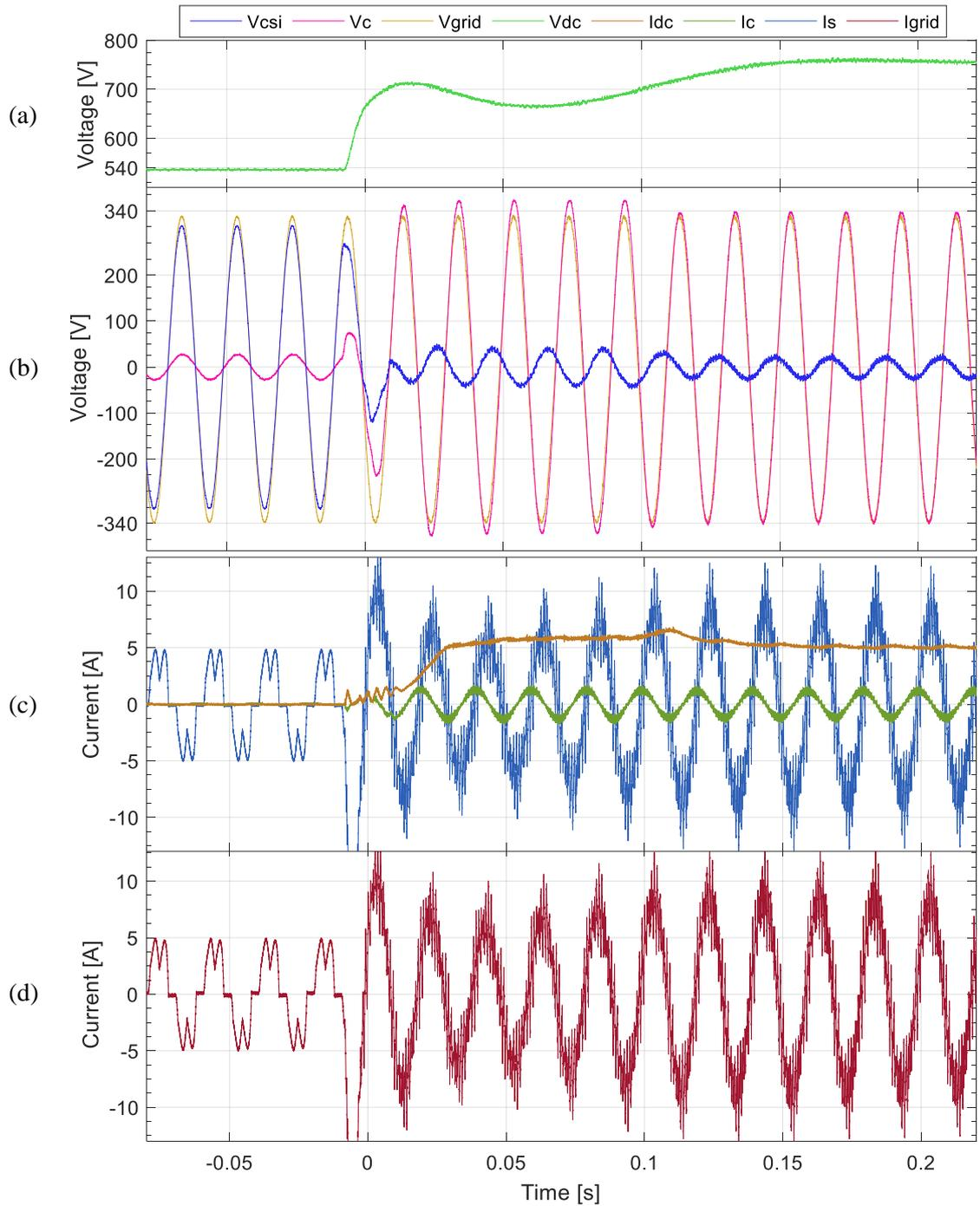
Fig 6-2: Experimental results showing PWM activation for VSI and CSI for  $K=0.1$  (sans ripple cancellation) for Phase A: a) VSI DC-link voltage ( $V_{dc}$ ); b) Series capacitor ( $V_c$ ), CSI ( $V_{csi}$ ) and grid ( $V_{grid}$ ) phase voltages; c) CSI DC-link current ( $I_{dc}$ ), Main VSI current ( $I_s$ ) and series capacitor current ( $I_c$ ); and d) combined grid side current ( $I_{grid}$ ).
