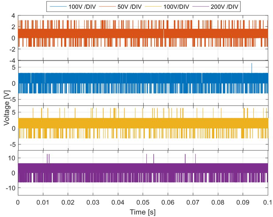
Minimum resolution 1.56V (50V/div) 3.125V (100V/div) and 6.25V (200V/div)
