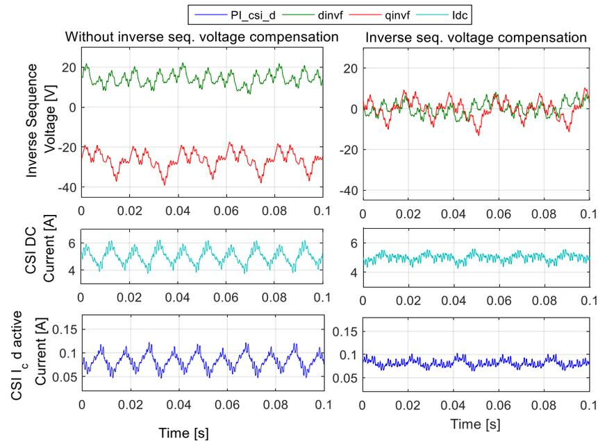
State variables showing inverse sequence voltage dq components before and after compensation while also showing the CSI DC-link current and active current component  $I_{c,d}$ . Both results captured for full hybrid operation.  $K=0.12$ .
