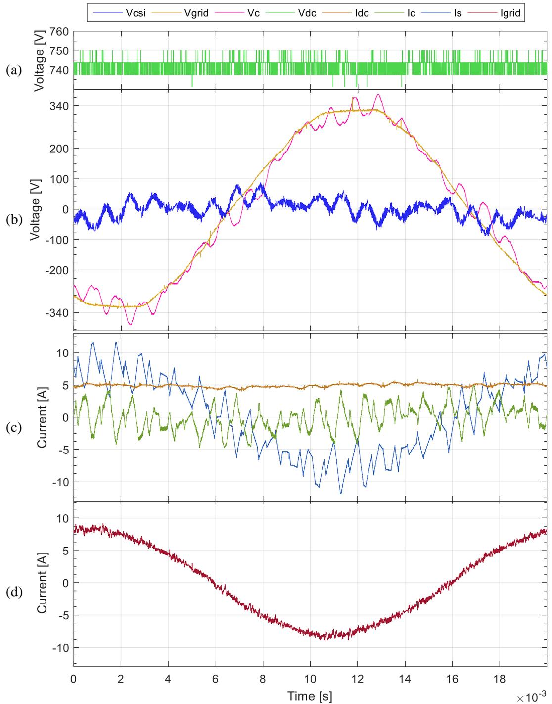
Fig 7-31: Experimental results showing one steady state cycle under full hybrid system operation for VSI and CSI for  $K=0.12$  for Phase A: a) VSI DC-link voltage ( $V_{dc}$ ) ;b) Series capacitor ( $V_c$ ), CSI ( $V_{csi}$ ) and grid ( $V_{grid}$ ) phase voltages; c) CSI DC-link current ( $I_{dc}$ ), Main VSI current ( $I_s$ ) and series capacitor current ( $I_c$ ) ; and d) combined grid side current ( $I_{grid}$ ).
