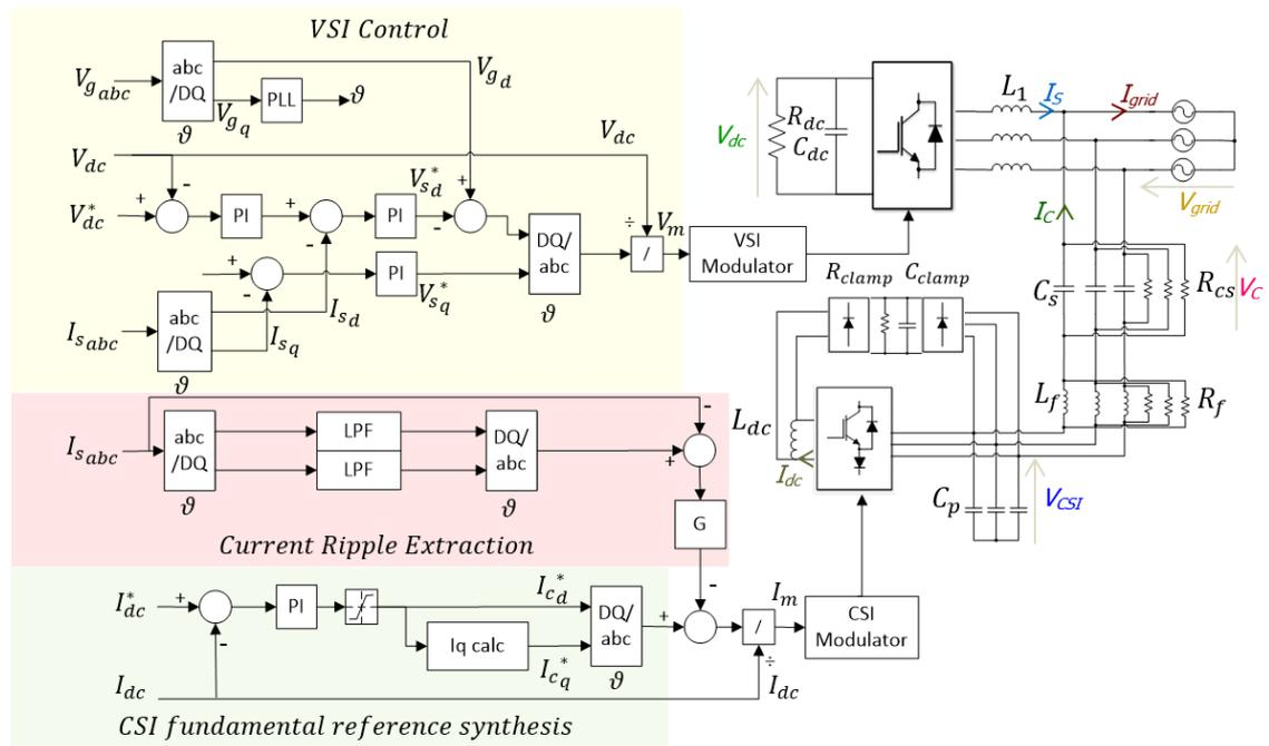
Fig. 5-15: Equivalent control system diagram and circuit interconnection
