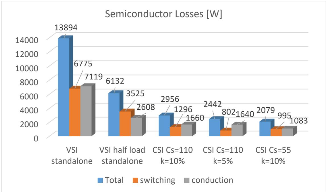
Fig. 3-20: Estimated semiconductor losses for VSI at full and half load operation and CSI at different series capacitance and voltage reduction operating points
