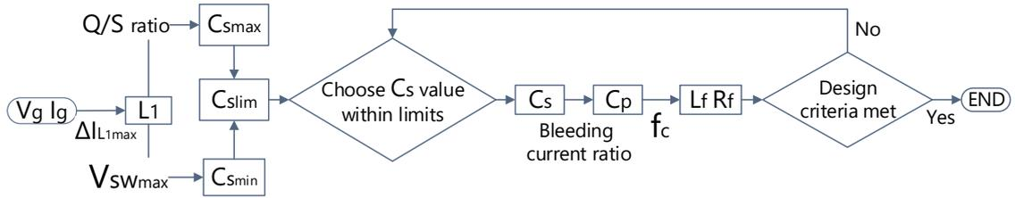
Fig 3-2 : Flowchart of the design procedure for the passive components of the hybrid converter
