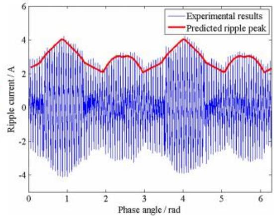
Fig. 20. Experimental results of current ripple with DPWM.
