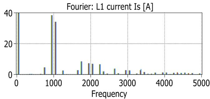
Fig. 4-6: Main VSI inductor (L1) current harmonics
