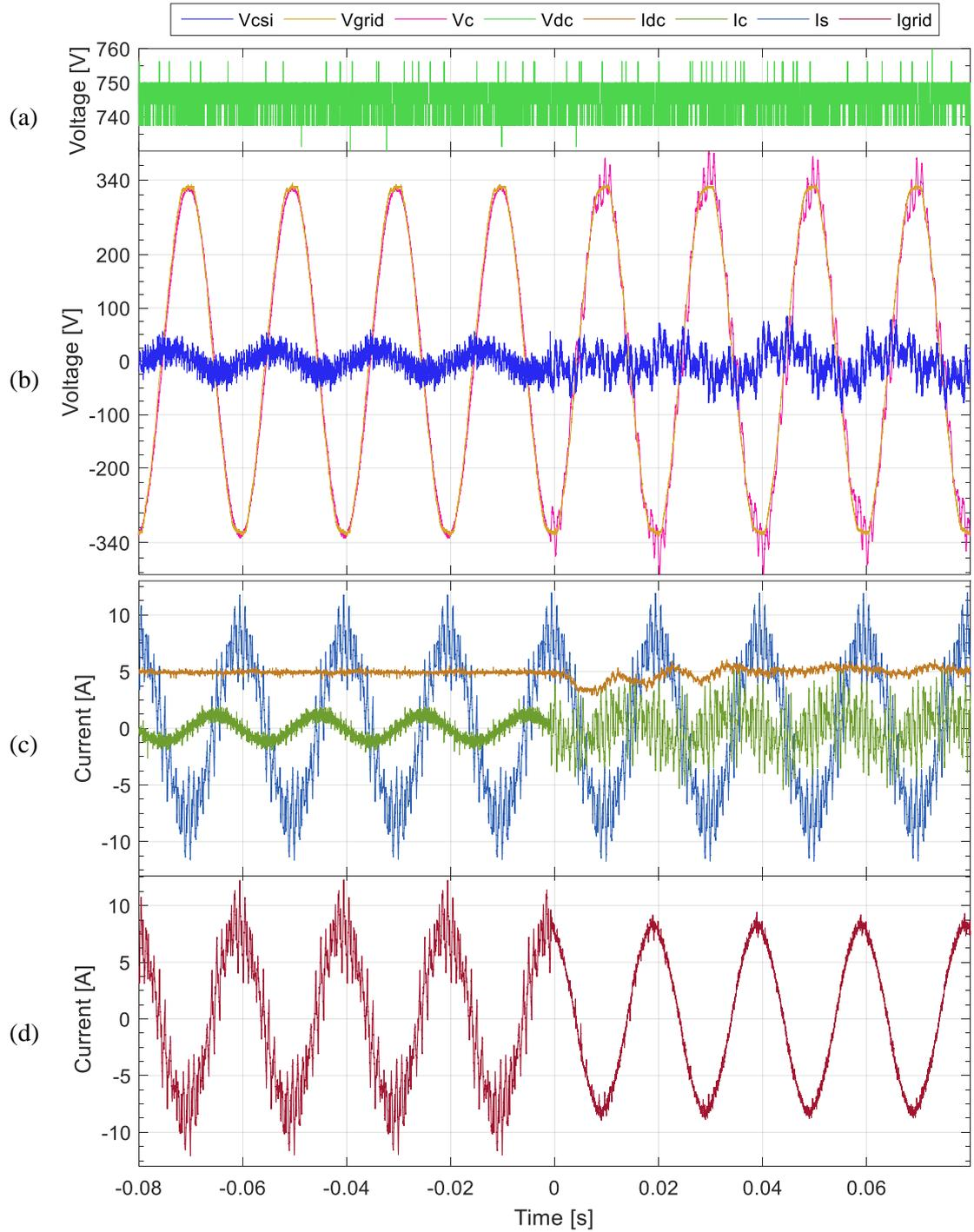
Fig 7-40: Experimental results showing activation of ripple cancellation for VSI and CSI for  $K=0.12$  for Phase A: a) VSI DC-link voltage ( $V_{dc}$ ); b) Series capacitor ( $V_c$ ), CSI ( $V_{csi}$ ) and grid ( $V_{grid}$ ) phase voltages; c) CSI DC-link current ( $I_{dc}$ ), Main VSI current ( $I_s$ ) and series capacitor current ( $I_c$ ); and d) combined grid side current ( $I_{grid}$ ).
