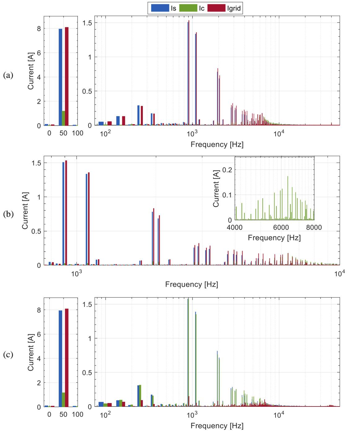
Fig 7-43: FFT of Phase A VSI current ( $I_s$ ), CSI current ( $I_c$ ) and grid current ( $I_{grid}$ ): a) before ripple cancellation up to 50 kHz; b) zoom in between 700Hz and 10kHz before cancellation; and c) full system operation on a semi logarithmic scale.
