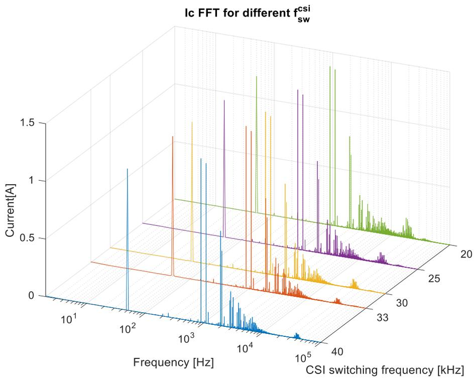
Fig 6-13: Cumulated FFT for CSI current harmonics for different CSI switching frequencies.
