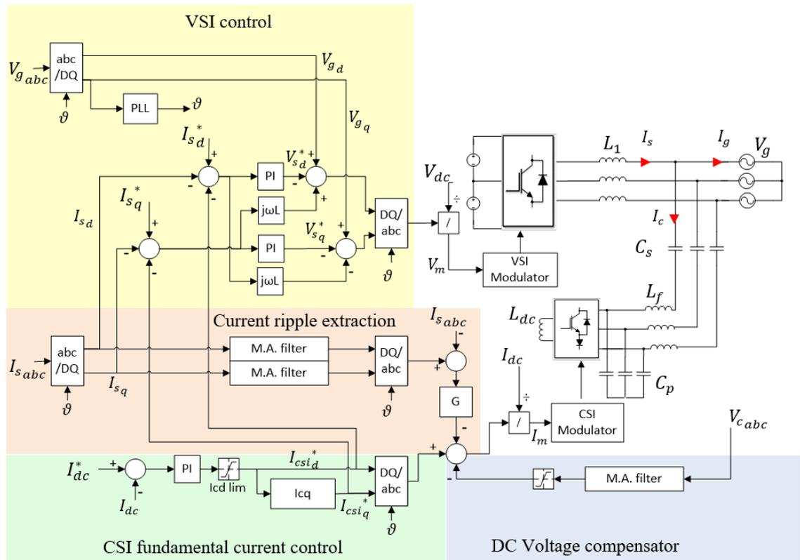
Fig. 3-9: Control scheme of the hybrid assembly
