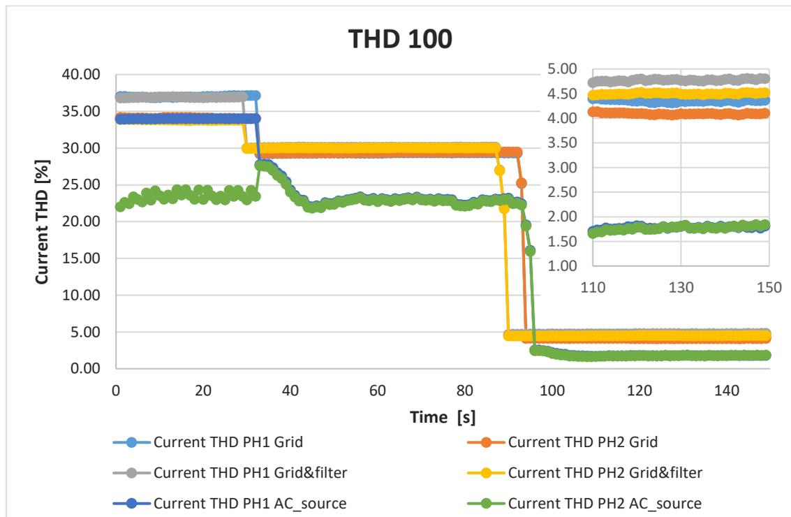
Fig 8-3: Power analyser grid current THD100 measurement for different configurations
