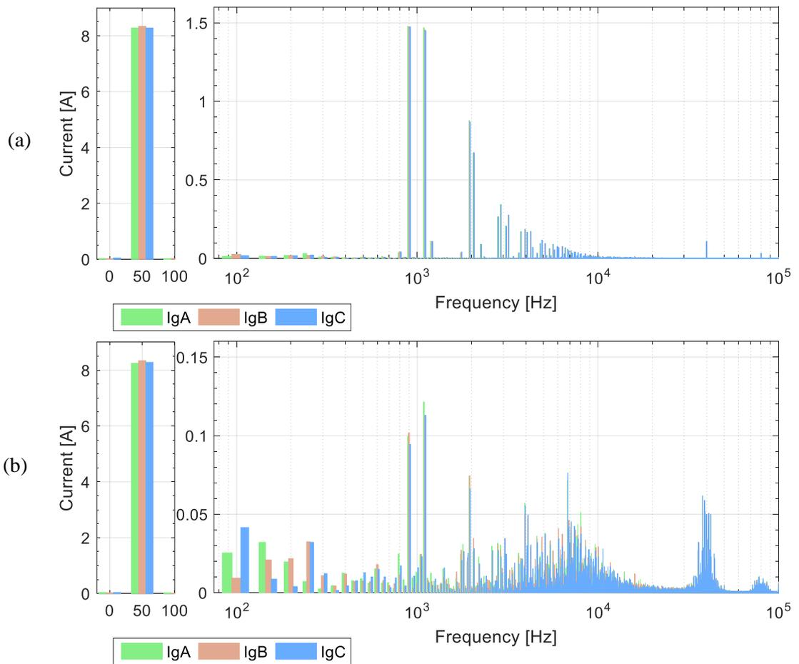
Fig 8-6: FFT of three phase grid currents and CSI dc current under electronic AC source connection: a) before harmonic cancellation; and b) after harmonic cancellation.
