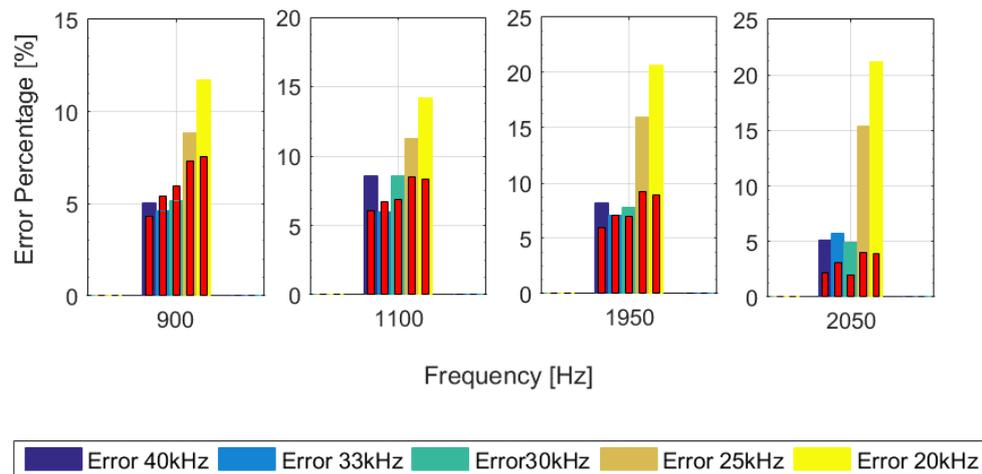
Fig 6-17: Bar charts showing resulting total error in reduction for each of the main current harmonics for different CSI switching frequencies and superimposed (in red) the error due to amplitude mismatch produced by the CSI.
