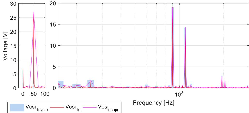
Correlation between FFT methods: Result shows the superimposed FFT waveform of phase A CSI voltage acquired using different methods:
