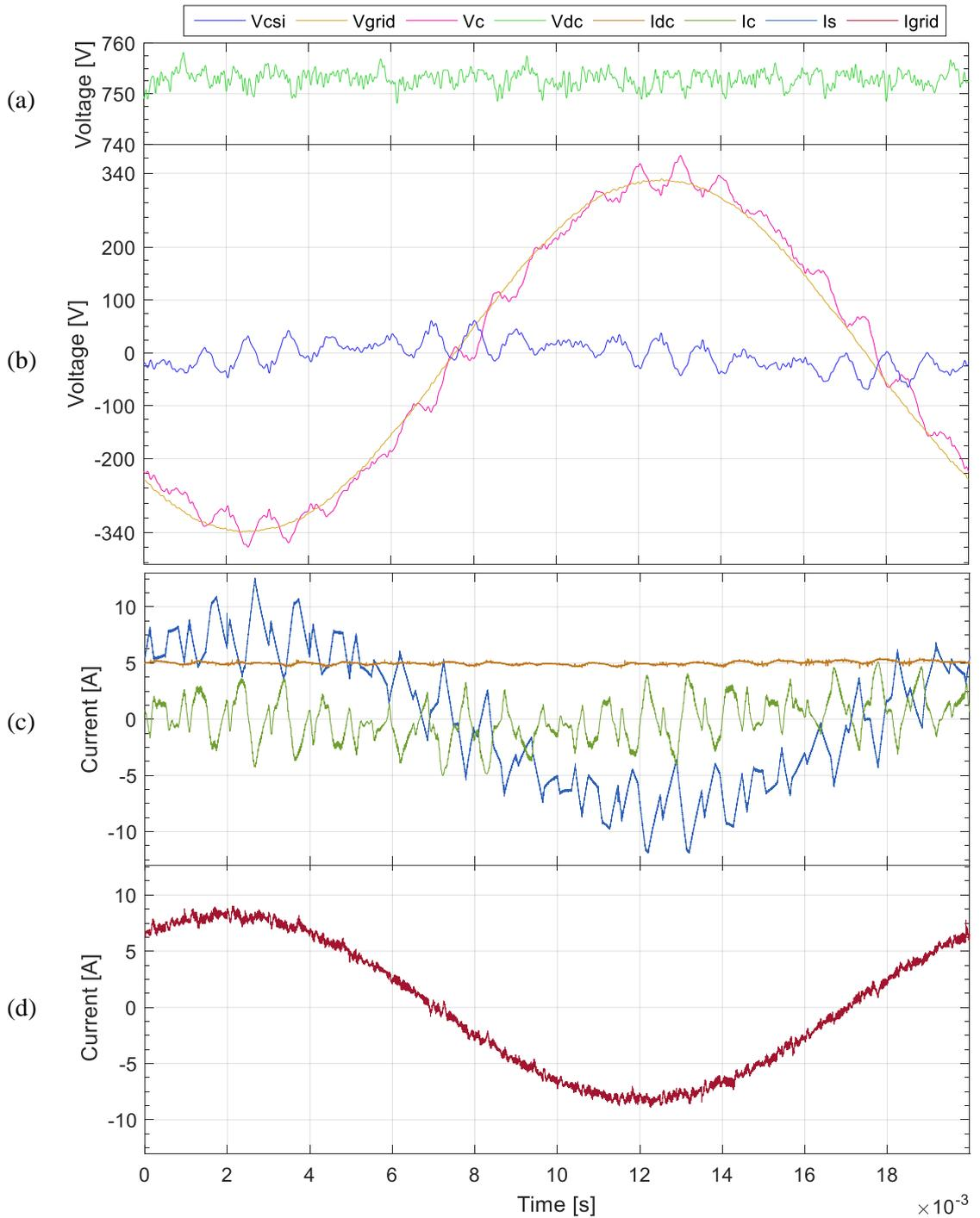
Fig 6-4: Experimental results showing one steady state cycle under full hybrid system operation for VSI and CSI for  $K=0.1$  for Phase A: a) VSI DC-link voltage ( $V_{dc}$ ); b) Series capacitor ( $V_c$ ), CSI ( $V_{csi}$ ) and grid ( $V_{grid}$ ) phase voltages; c) CSI DC-link current ( $I_{dc}$ ), Main VSI current ( $I_s$ ) and series capacitor current ( $I_c$ ); and d) combined grid side current ( $I_{grid}$ ).
