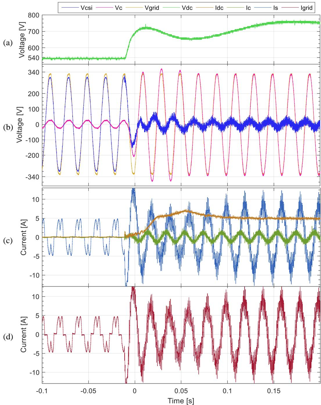
Fig 7-39: Experimental results showing PWM activation for VSI and CSI for  $K=0.12$  (sans ripple cancellation) for Phase A: a) VSI DC-link voltage ( $V_{dc}$ ); b) Series capacitor ( $V_c$ ), CSI ( $V_{csi}$ ) and grid ( $V_{grid}$ ) phase voltages; c) CSI DC-link current ( $I_{dc}$ ), Main VSI current ( $I_s$ ) and series capacitor current ( $I_c$ ); and d) combined grid side current ( $I_{grid}$ ).
