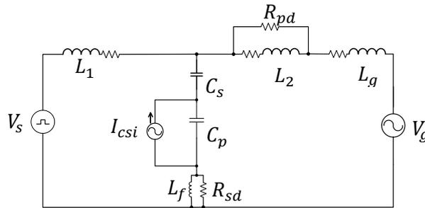
Fig. 4-8: Single Phase Equivalent circuit showing passive damping options
