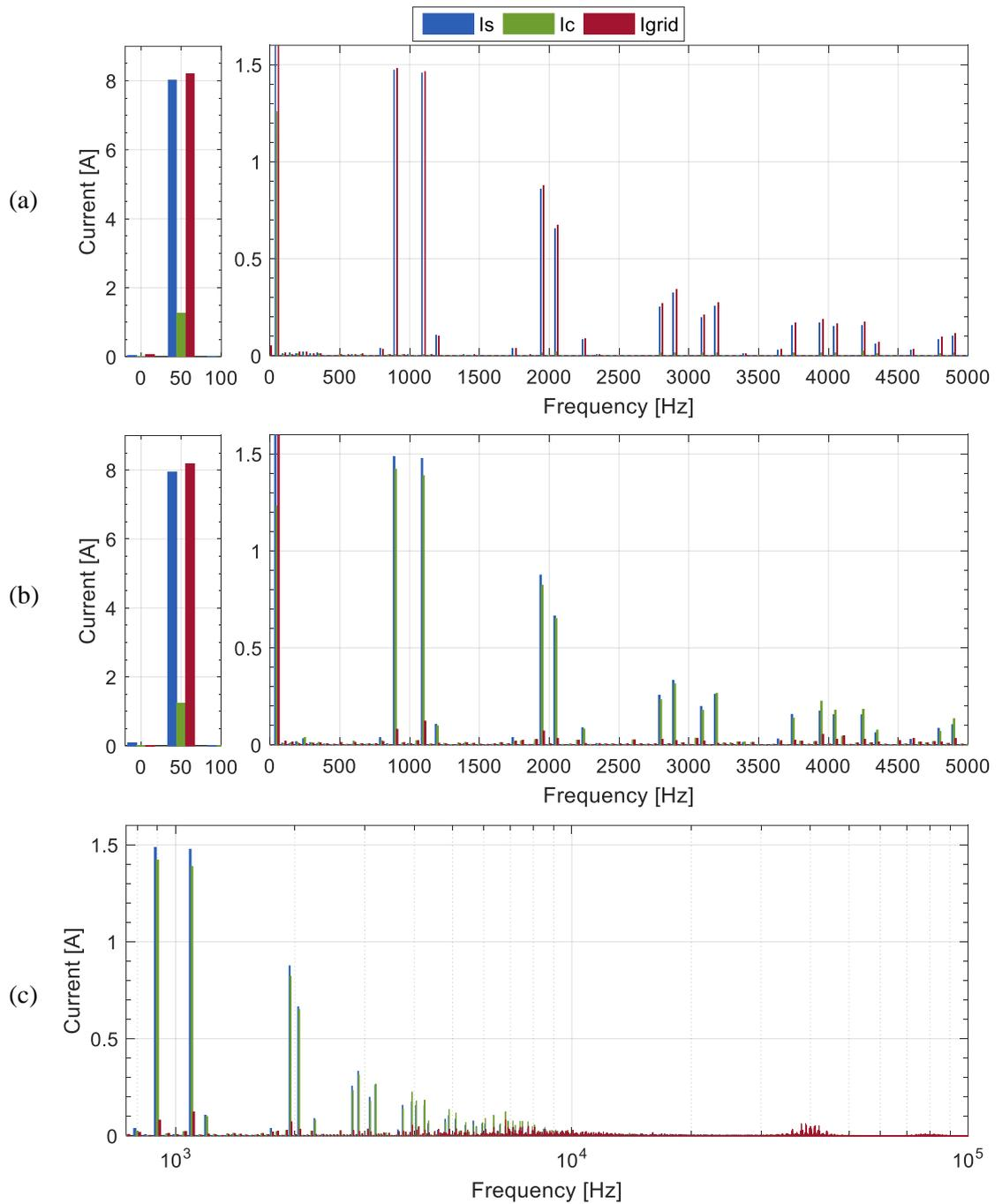
Fig 6-6: FFT of Phase A VSI current ( $I_s$ ), CSI current ( $I_c$ ) and grid current ( $I_{grid}$ ) : a) without ripple cancellation ; b) full system operation up to 5 kHz; and c) expanded to show harmonics from 700Hz to 100kHz on a semi logarithmic scale.
