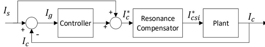
Fig. 4-10: Active damping implementation for Ripple Cancellation
