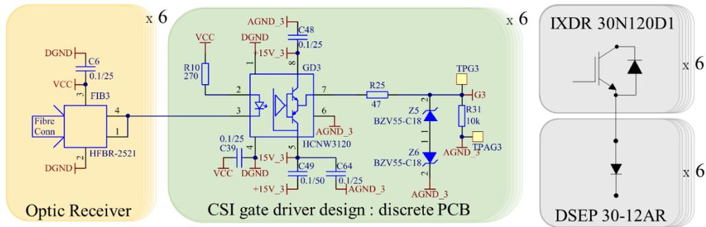
Fig. 5-1: Overview of gate driver configuration and CSI switches
