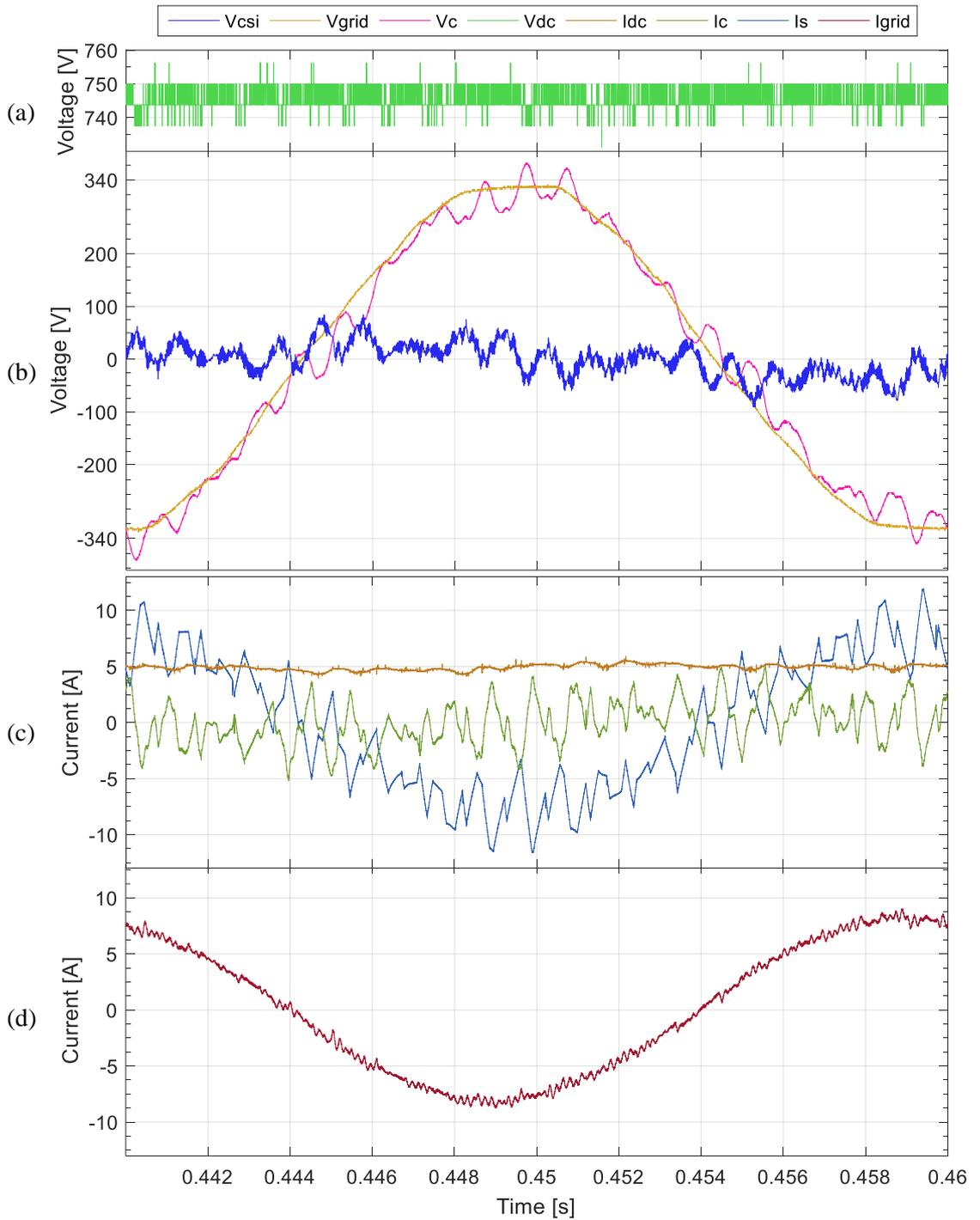
Fig 7-42: Experimental results showing one steady state cycle under full hybrid system operation for VSI and CSI for  $K=0.12$  for Phase A: a) VSI DC-link voltage ( $V_{dc}$ ); b) Series capacitor ( $V_c$ ), CSI ( $V_{csi}$ ) and grid ( $V_{grid}$ ) phase voltages; c) CSI DC-link current ( $I_{dc}$ ), Main VSI current ( $I_s$ ) and series capacitor current ( $I_c$ ); and d) combined grid side current ( $I_{grid}$ ).
