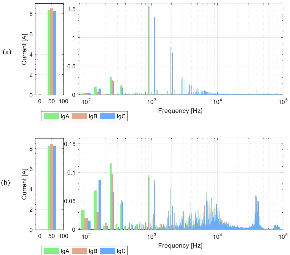
Fig 8-8: FFT of three phase grid currents and CSI dc current under real grid connection: a) before harmonic cancellation; and b) after harmonic cancellation.
