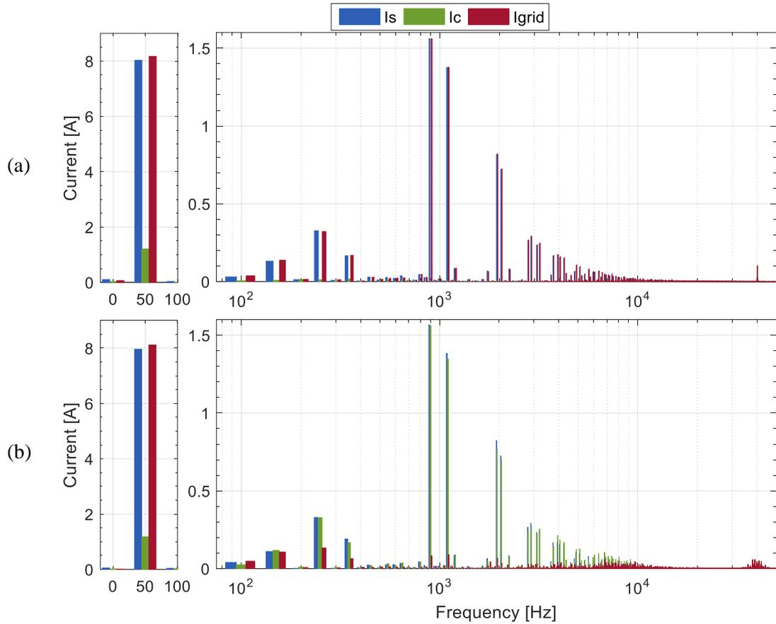
Fig 7-32: FFT (up to 50 kHz) of Phase A VSI current ( $I_s$ ), CSI current ( $I_c$ ) and grid current ( $I_{grid}$ ): a) without ripple cancellation; and b) full system operation on a semi logarithmic scale.
