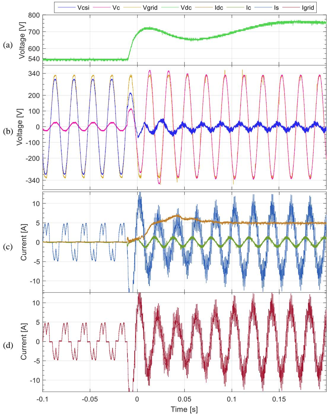
Fig 7-29: Experimental results showing PWM activation for VSI and CSI for  $K=0.12$  (sans ripple cancellation) for Phase A: a) VSI DC-link voltage ( $V_{dc}$ ); b) Series capacitor ( $V_c$ ), CSI ( $V_{csi}$ ) and grid ( $V_{grid}$ ) phase voltages; c) CSI DC-link current ( $I_{dc}$ ), Main VSI current ( $I_s$ ) and series capacitor current ( $I_c$ ); and d) combined grid side current ( $I_{grid}$ ).
