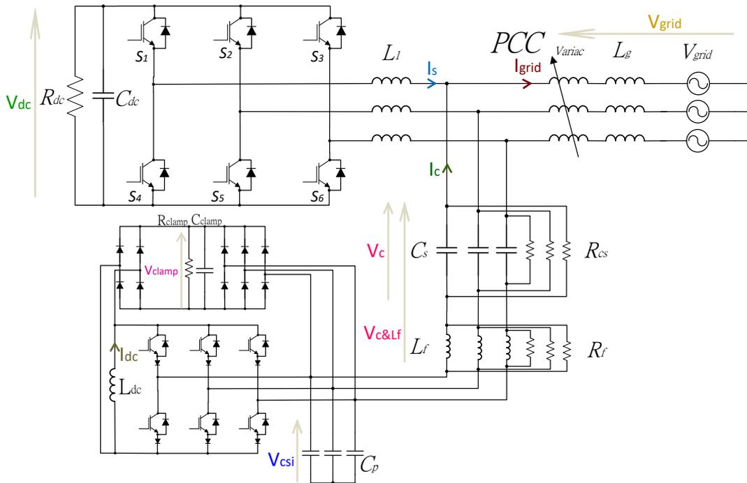
Fig 7-4: Circuit topology of the experimental setup connected to the real power grid.
