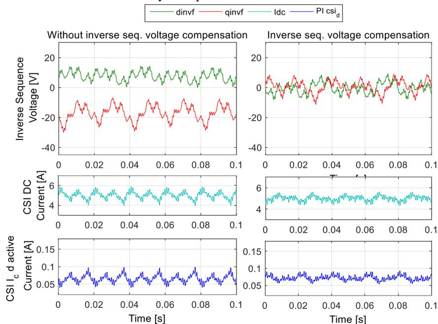
State variables showing inverse sequence voltage dq components before and after compensation while also showing the CSI DC-link current and active current component  $I_{c,d}$ . Both results captured for full hybrid operation.  $K=0.12$ . Using AC filter at the point of PCC.
