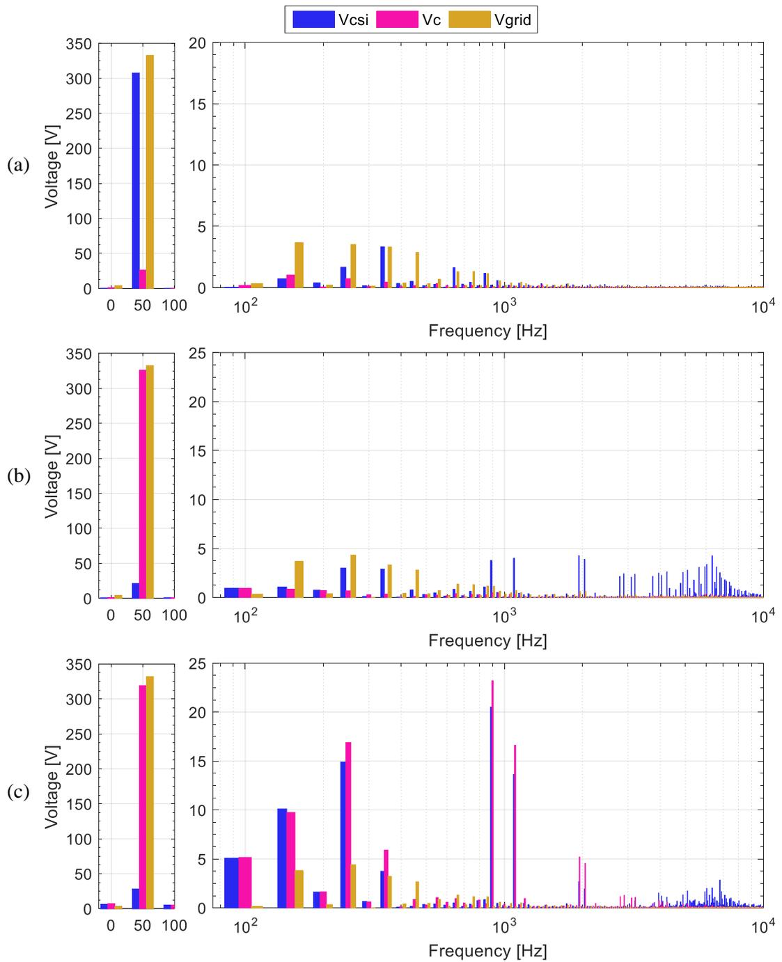
Fig 7-45: FFT of Phase A voltage of the Grid ( $V_g$ ), Series capacitor ( $V_c$ ) and CSI phase voltage ( $V_{csi}$ ) during: a) No PWM; b) PWM enabled showing fundamental voltage reduction; and c) full system operation (harmonic cancellation).
