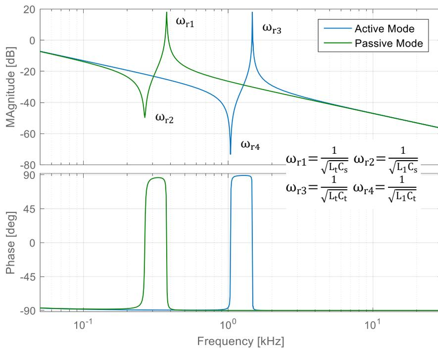
Fig. 4-7: Converter Voltage to Converter Current Bode plot for active and passive filtering mode.
