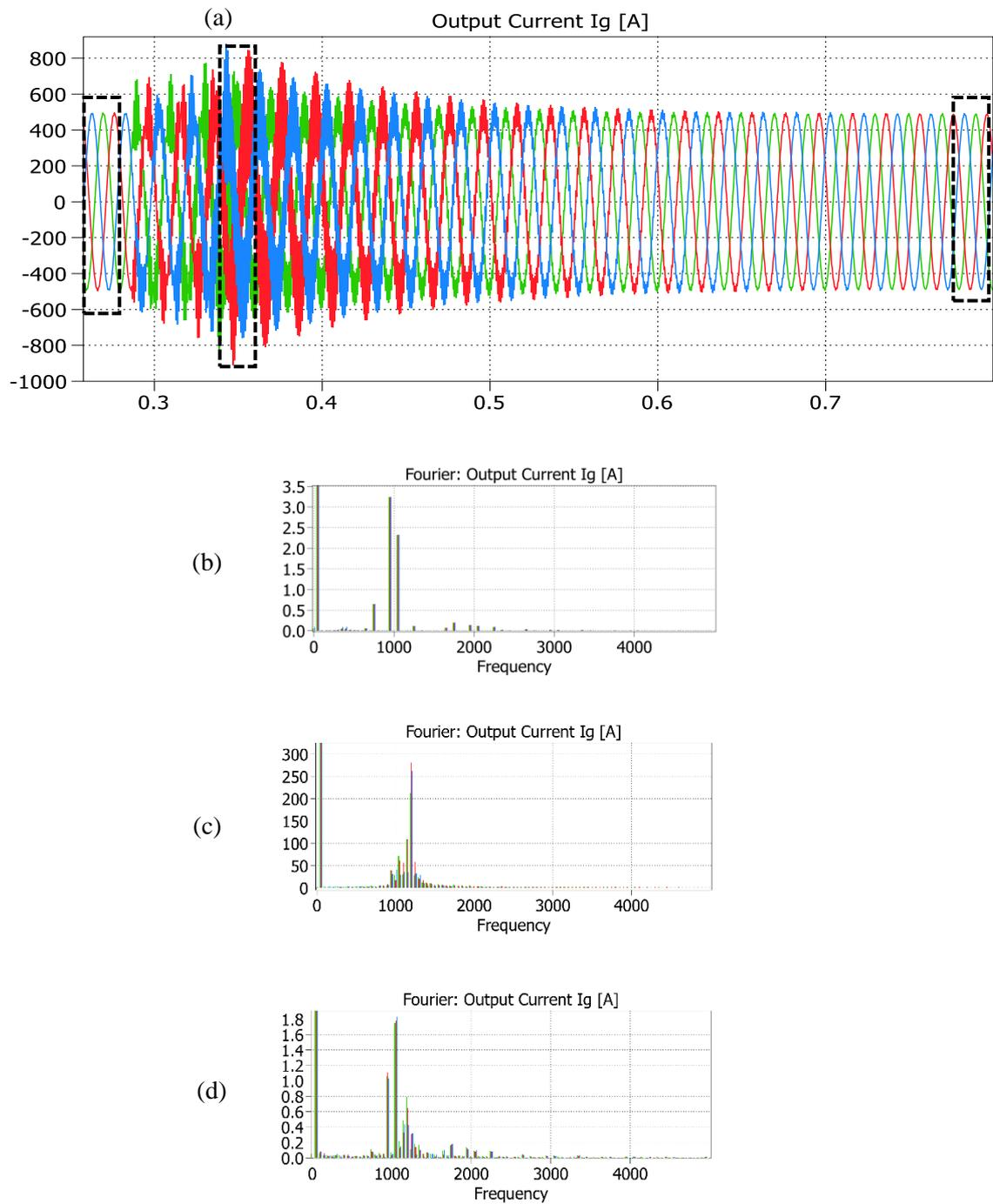
Fig. 4-12a-d: Transient operation showing activation of CSI at  $t_1=0.28$ s followed by LC circuit resonance build-up and activation of the resonance compensator at  $t_2=0.36$ s followed by resonance being actively damped ( $t>0.7$ s). b)-c)-d) FFT of the MV grid currents when b) CSI was off and switching ripple is passively damped by the LCL filter; c) just before active damping activation ( $t=0.34-0.36$ ); d) at end of simulation when resonance levels are not visible.
