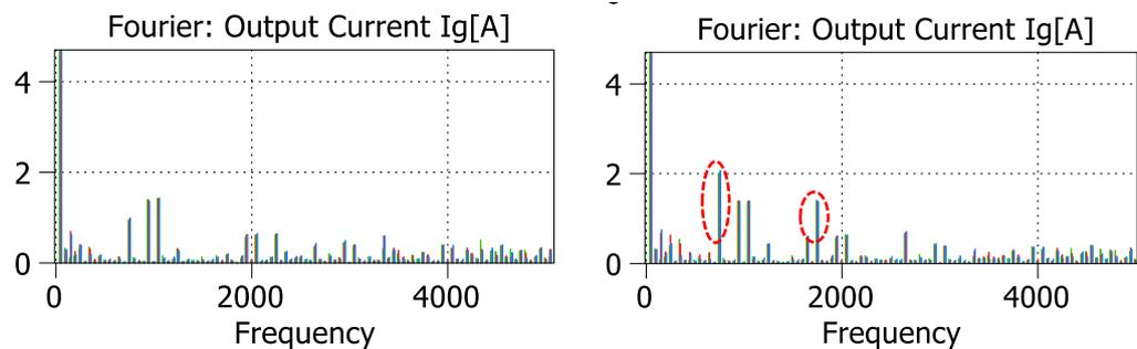
Fig. 3-19: Harmonic content of filtered grid current for moving average filter windows of 2ms (left) and 1ms used for improving transient response (right).
