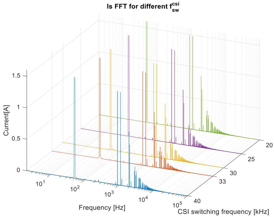
Fig 6-12: Cumulated FFT for VSI current harmonics excluding the fundamental component for different base sampling frequencies defined by the CSI switching frequency.
