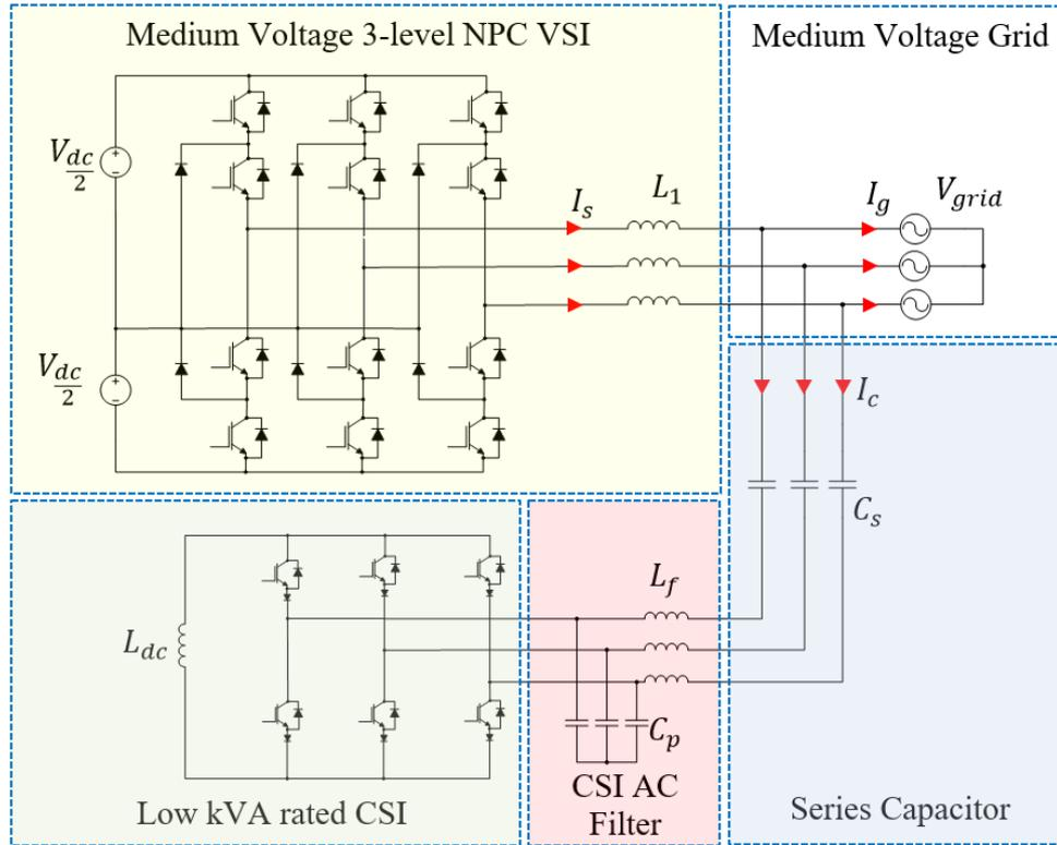
Fig. 3-1: Hybrid system topology highlighting the main features
