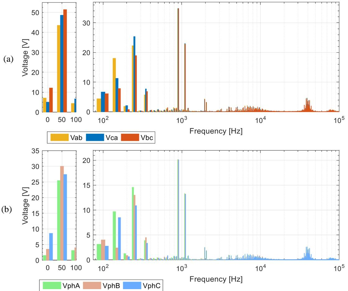
Fig 7-37: FFT of the CSI input voltages under full system steady state operation showing the harmonics in: a) the three CSI line-line voltages and b) the three phase-neutral CSI voltages.
