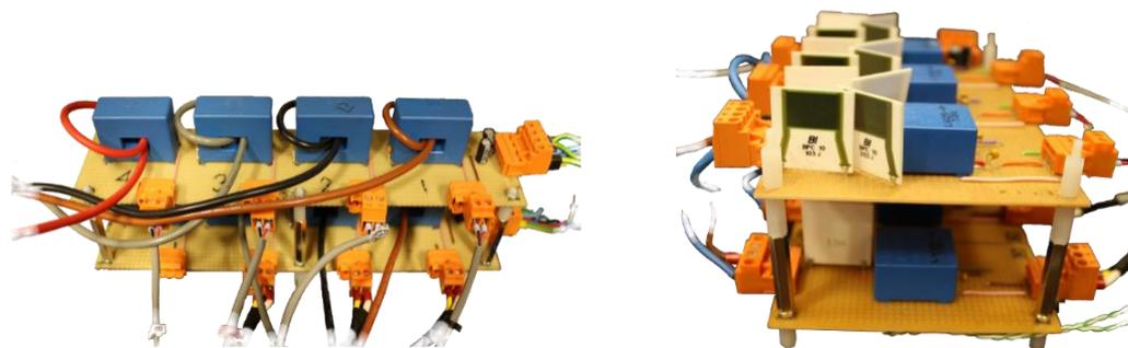
Fig. 5-13: Picture of current and voltage sensing boards
