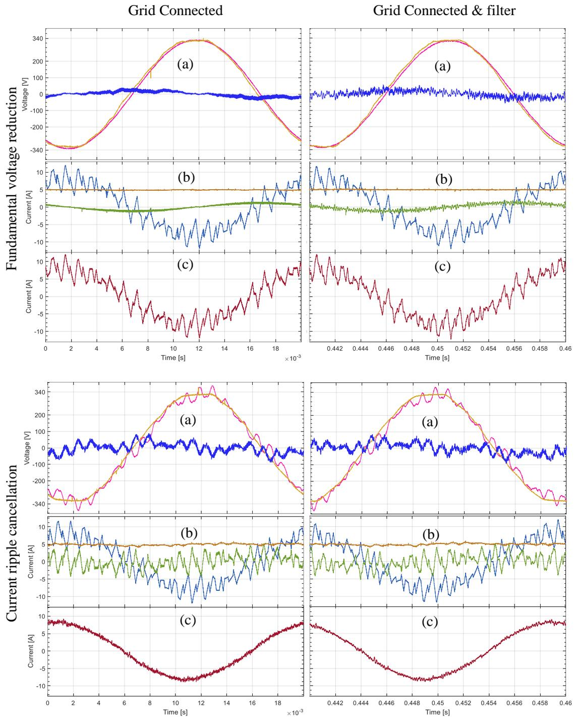
Experimental results showing: a) Series capacitor ( $V_c$ ), CSI ( $V_{csi}$ ) and grid ( $V_{grid}$ ) phase voltages; b) CSI DC-link current ( $I_{dc}$ ), Main VSI current ( $I_s$ ) and series capacitor current ( $I_c$ ); and c) combined grid side current ( $I_{grid}$ ). The results are shown for one steady state cycle for the following cases: before (top) and after (bottom) ripple cancellation. Without added grid impedance (left) and with added grid impedance showing resonance (right)
