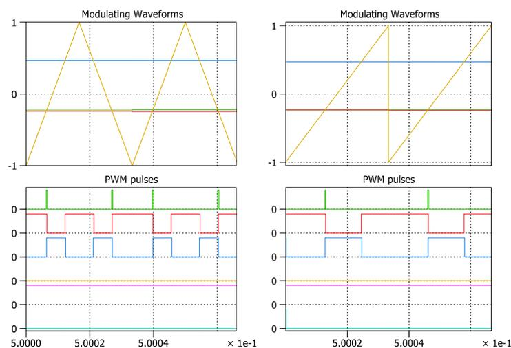
Fig. 5-9. Pulse generation for two carrier wave periods shown for triangular carrier and sawtooth carrier waveforms.
