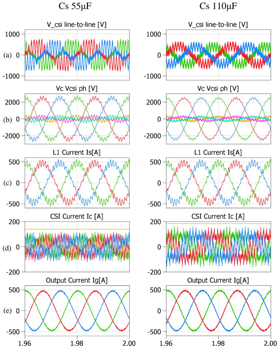
Fig. 3-13: Simulation waveforms during steady state operation considering the two series capacitor values a) Line-To-Line CSI Voltages; b) Line-To-Neutral CSI And Series Capacitor Voltages; c) Input (Main Converter) Current through the Interface Inductor (L1). d) CSI Current; e) Cumulated Output Current;
