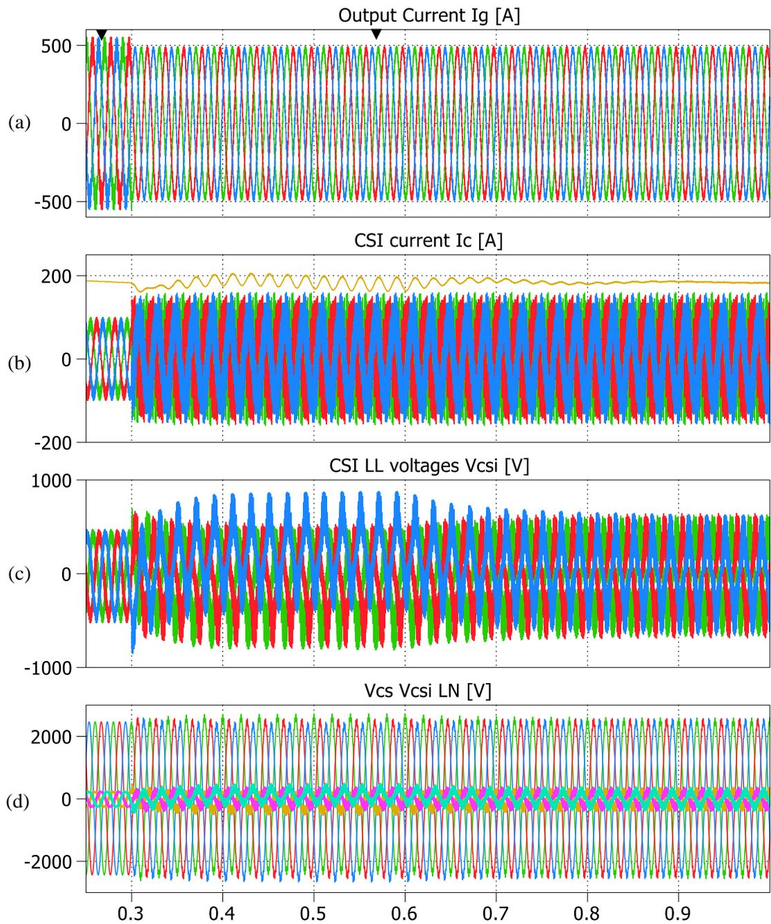
Fig. 3-16: DC voltage compensator validation showing activation of current ripple cancellation at  $t=0.3s$  including DC current disturbances and activation of DC voltage compensator at  $t=0.6s$ .
