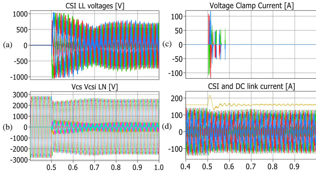
Fig. 4-13a-d: Transient between passive and active filtering mode at  $t_1$  showing a) CSI l-l voltage b) Series capacitor and CSI phase voltages c) Voltage clamp current and d) Series capacitor current along with CSI DC link current.
