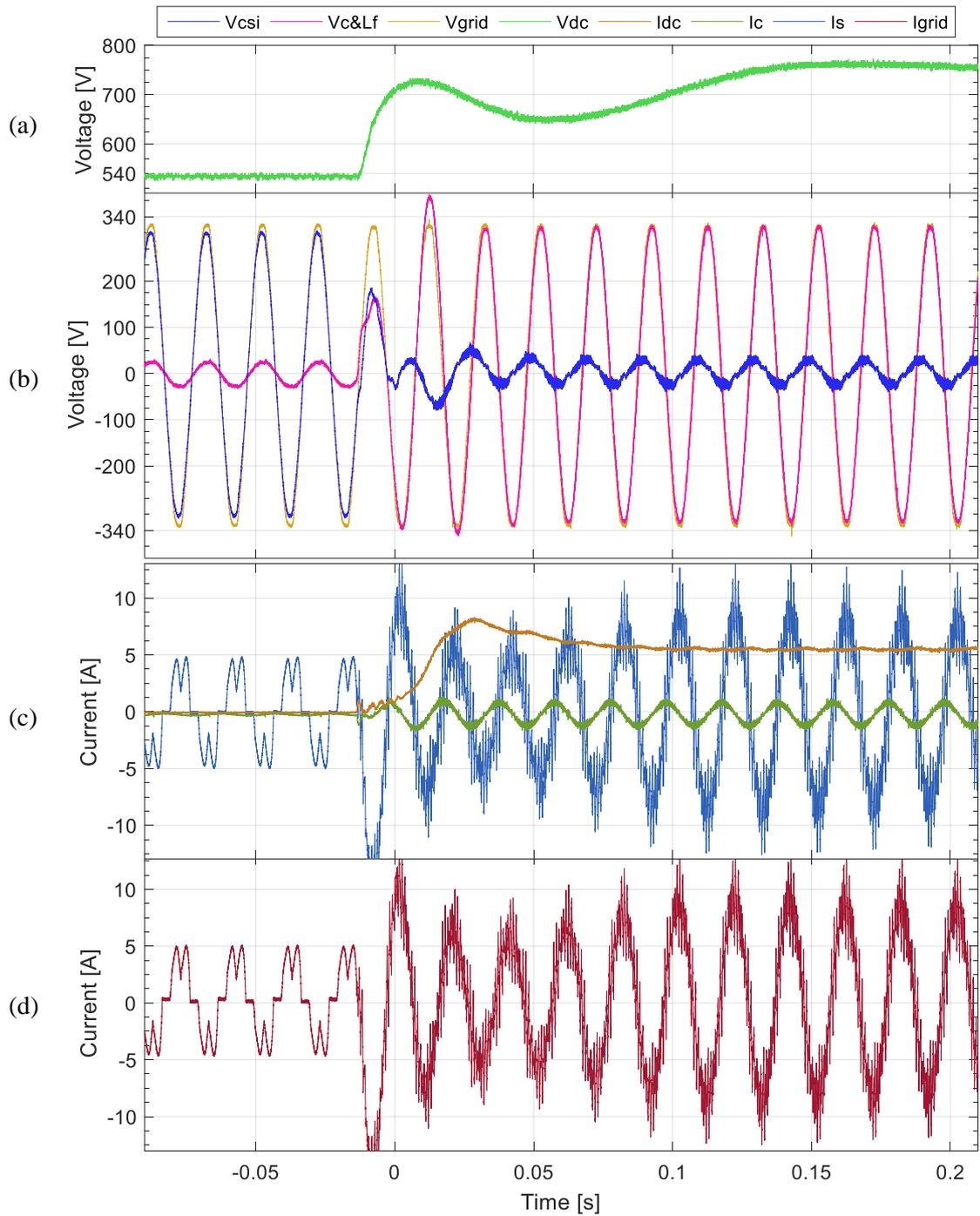
Fig 7-5: Experimental results showing PWM activation for VSI and CSI for  $K=0.15$  (sans ripple cancellation) for Phase A: a) VSI DC-link voltage ( $V_{dc}$ ); b) Series capacitor and filter ( $V_{c\&Lf}$ ), CSI ( $V_{csi}$ ) and grid ( $V_{grid}$ ) phase voltages; c) CSI DC-link current ( $I_{dc}$ ), Main VSI current ( $I_s$ ) and series capacitor current ( $I_c$ ); and d) combined grid side current ( $I_{grid}$ ).
