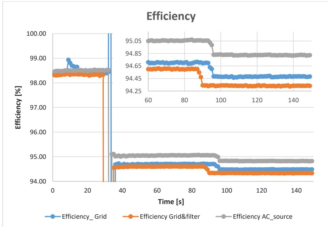
Fig 8-4: Power analyser efficiency measurement for different configurations
