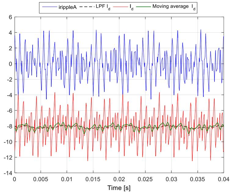
Fig 7-17: VSI current dq components captured through the dsp host interface for two cycles
