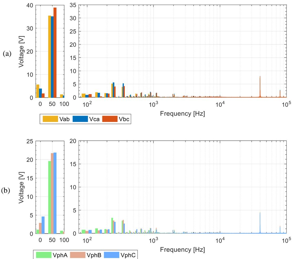
Fig 7-35: FFT of the CSI input voltages under fundamental voltage reduction mode showing the harmonics in: a) the three phase line-line CSI voltages and b) the three phase-neutral CSI voltages.
