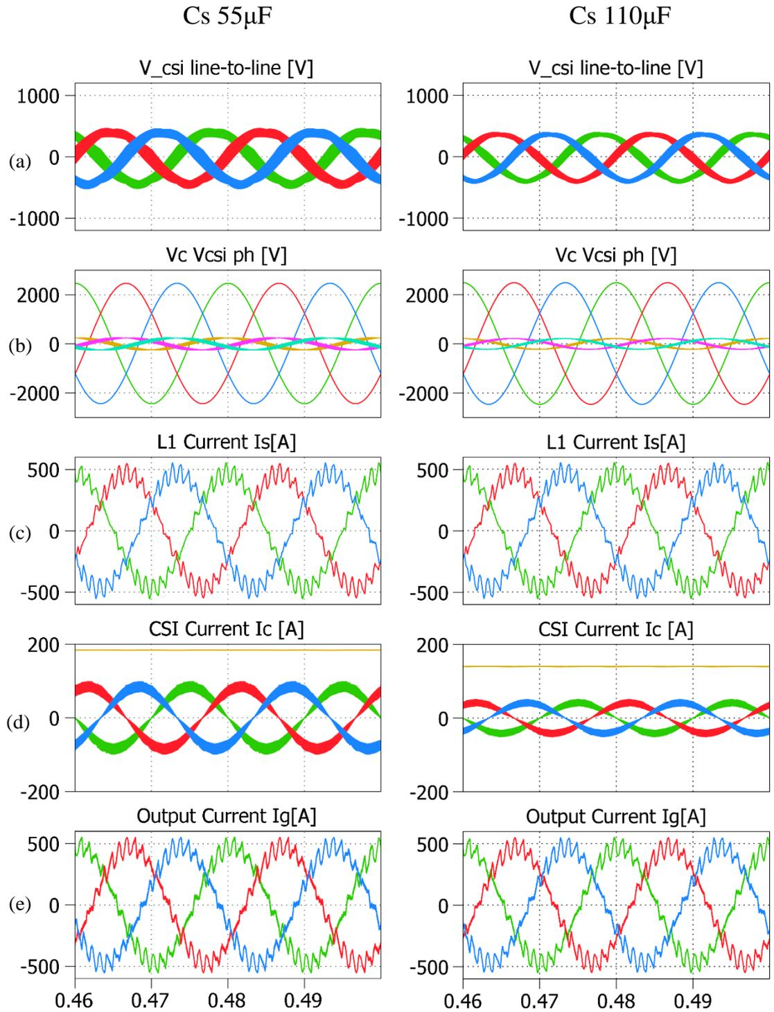
Fig. 3-12: Simulation waveforms during steady state operation before ripple cancellation considering the two series capacitor values a) Line-To-Line CSI Voltages; b) Line-To-Neutral CSI And Series Capacitor Voltages; c) Input (Main Converter) Current through the Interface Inductor (L1). d) CSI Current; e) Cumulated Output Current;
