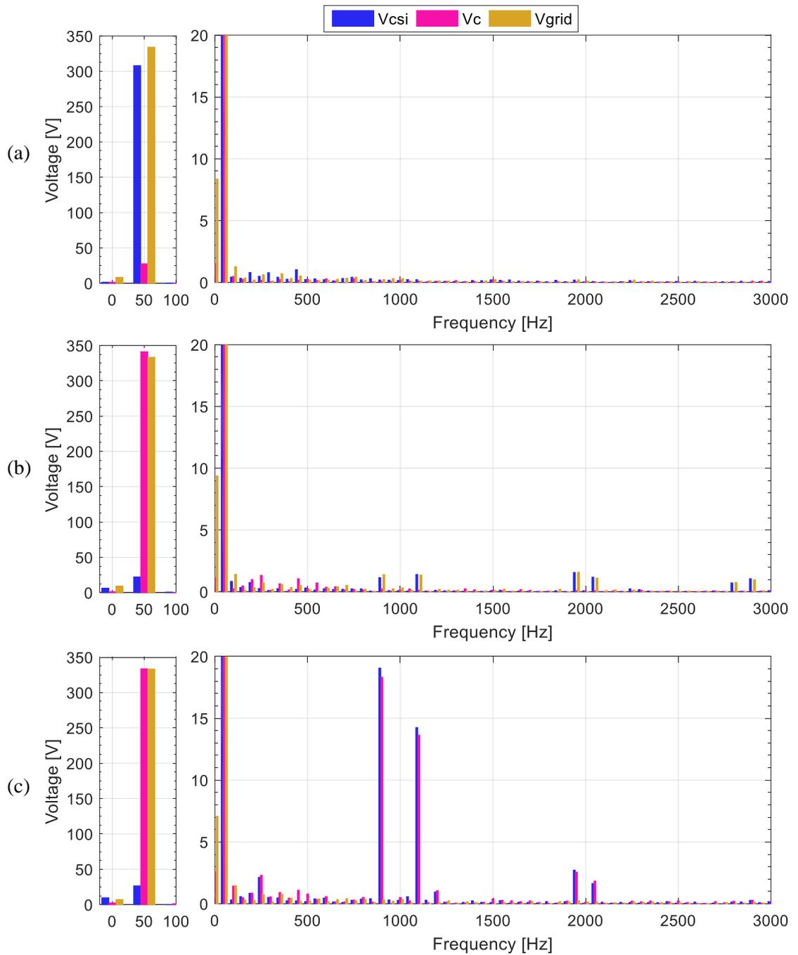
Fig 6-5: FFT of Phase A voltage of the Grid ( $V_g$ ), Series capacitor ( $V_c$ ) and CSI phase voltage ( $V_{csi}$ ) during: a) No PWM; b) PWM enabled showing fundamental voltage reduction; and c) full system operation (harmonic cancellation).
