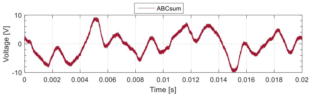
Fig 7-2: Zero sequence component in grid voltage
