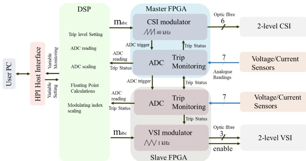
Fig. 5-7. Control platform system overview showing basic functionality associated with each element/board of the control platform
