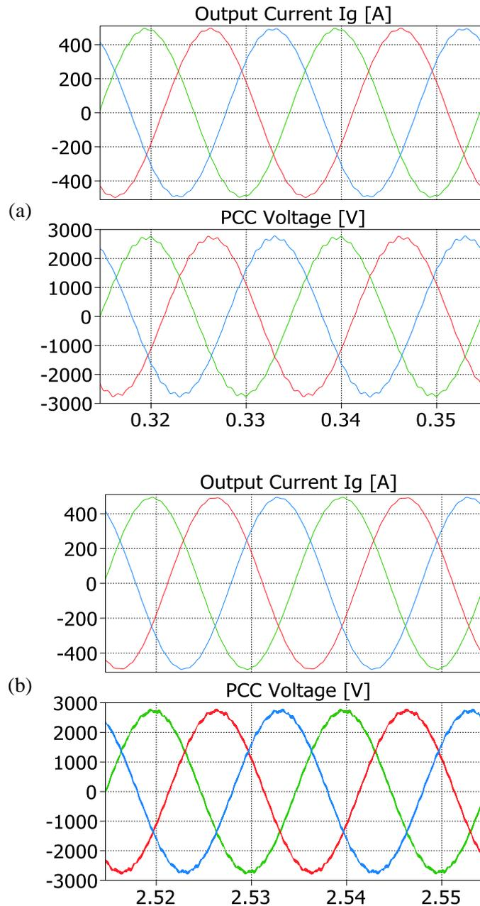
Fig. 4-16a-b: Steady state output current and PCC voltage a) during passive filtering mode and b) during active filtering.
