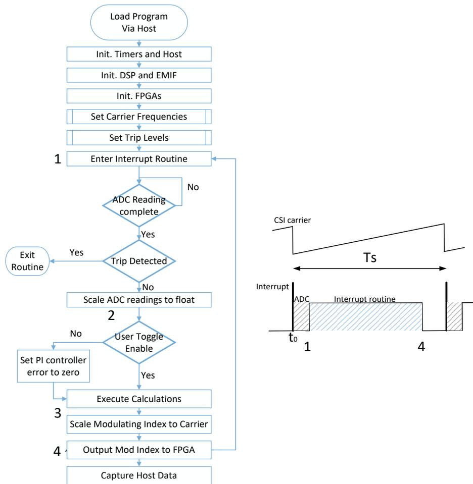
Fig. 5-16: Flowchart of DSP initialisation procedure and execution of the main interrupt routine
