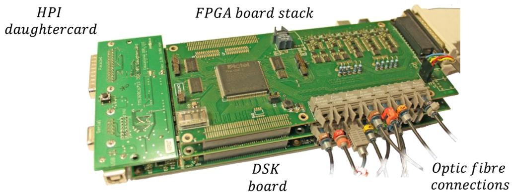
Fig. 5-6. Picture of Control platform utilising two FPGA boards and HPI daughtercard mounted on the DSK board.
