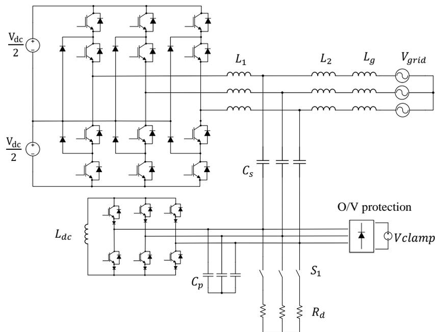
Fig. 4-4: Hybrid converter topology with LCL filter interconnection
