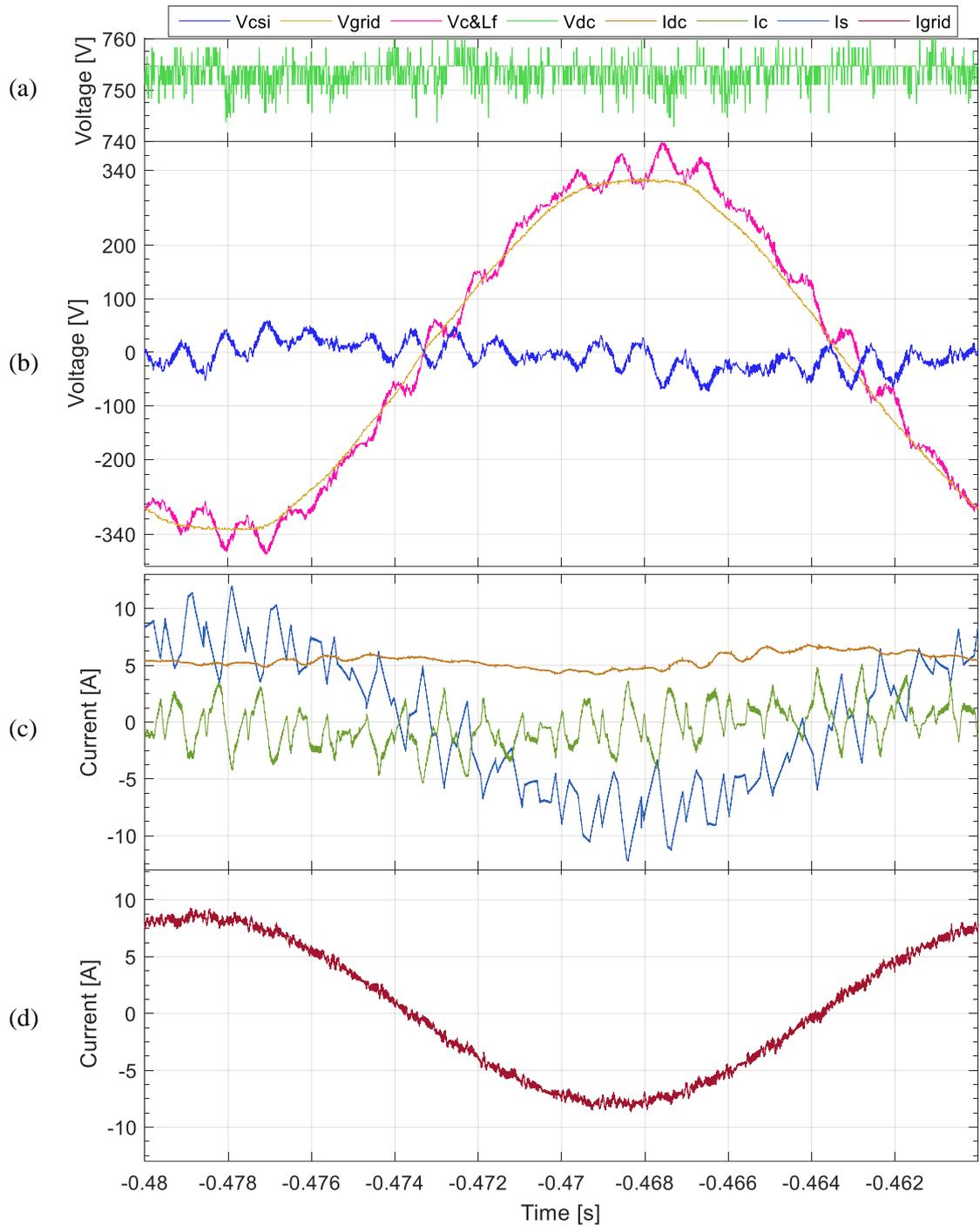
Fig 7-7: Experimental results showing one steady state cycle under full hybrid system operation for VSI and CSI for  $K=0.15$  for Phase A: a) VSI DC-link voltage ( $V_{dc}$ ); b) Series capacitor and filter ( $V_{c\&Lf}$ ), CSI ( $V_{csi}$ ) and grid ( $V_{grid}$ ) phase voltages; c) CSI DC-link current ( $I_{dc}$ ), Main VSI current ( $I_s$ ) and series capacitor current ( $I_c$ ); and d) combined grid side current ( $I_{grid}$ ).
