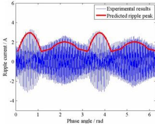
Fig. 19. Experimental results of current ripple with SVPWM.
