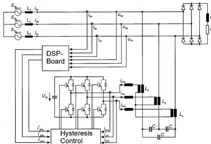
Fig. 2-3: Hybrid active power filter connected to LC filter as proposed in [81]
