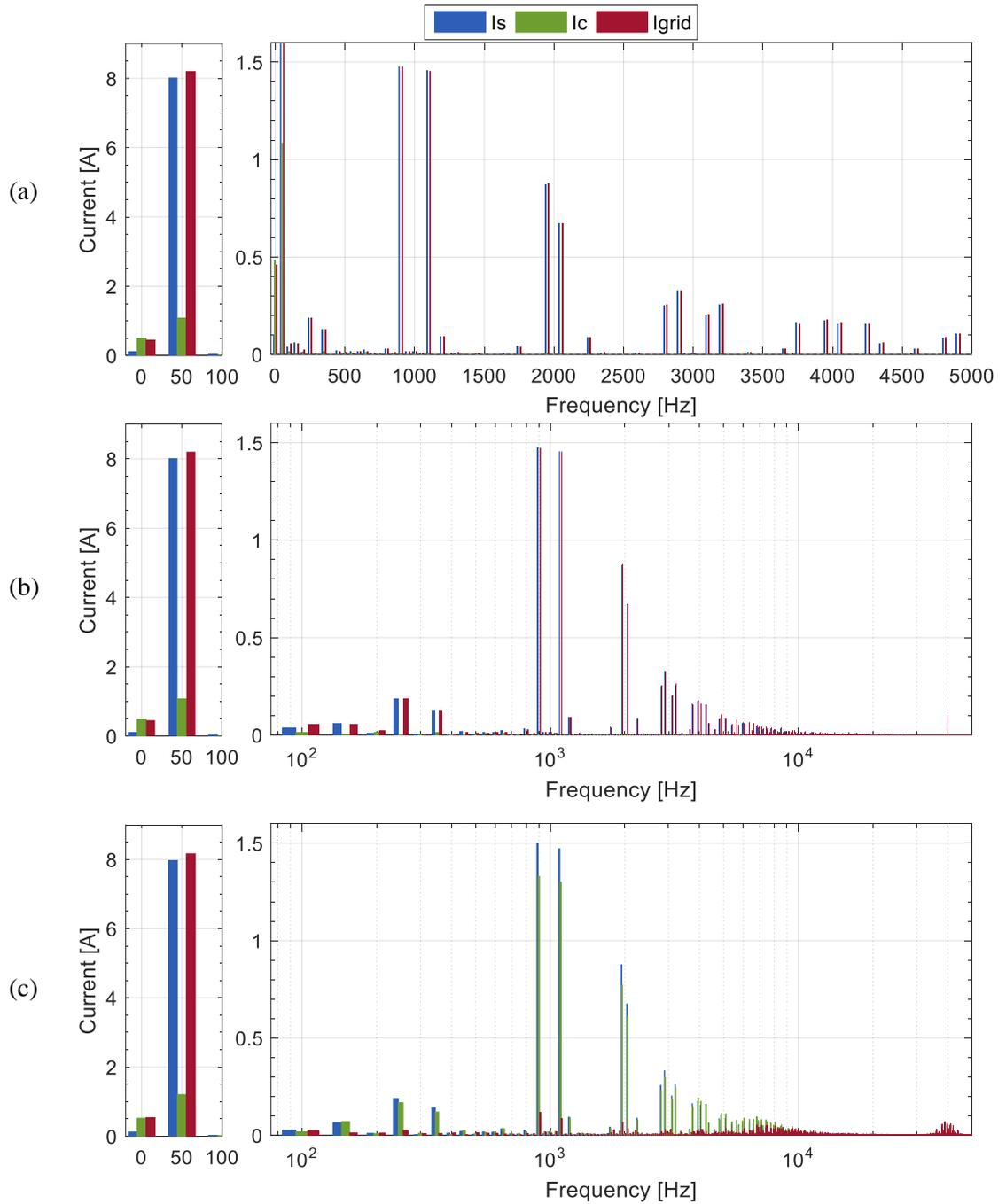
Fig 7-8: FFT of Phase A VSI current ( $I_s$ ), CSI current ( $I_c$ ) and grid current ( $I_{grid}$ ) : a) without ripple cancellation up to 5 kHz ; b) without ripple cancellation showing harmonics up to 50kHz on a semi logarithmic scale; and c) full system operation up to 50kHz on a semi logarithmic scale.
