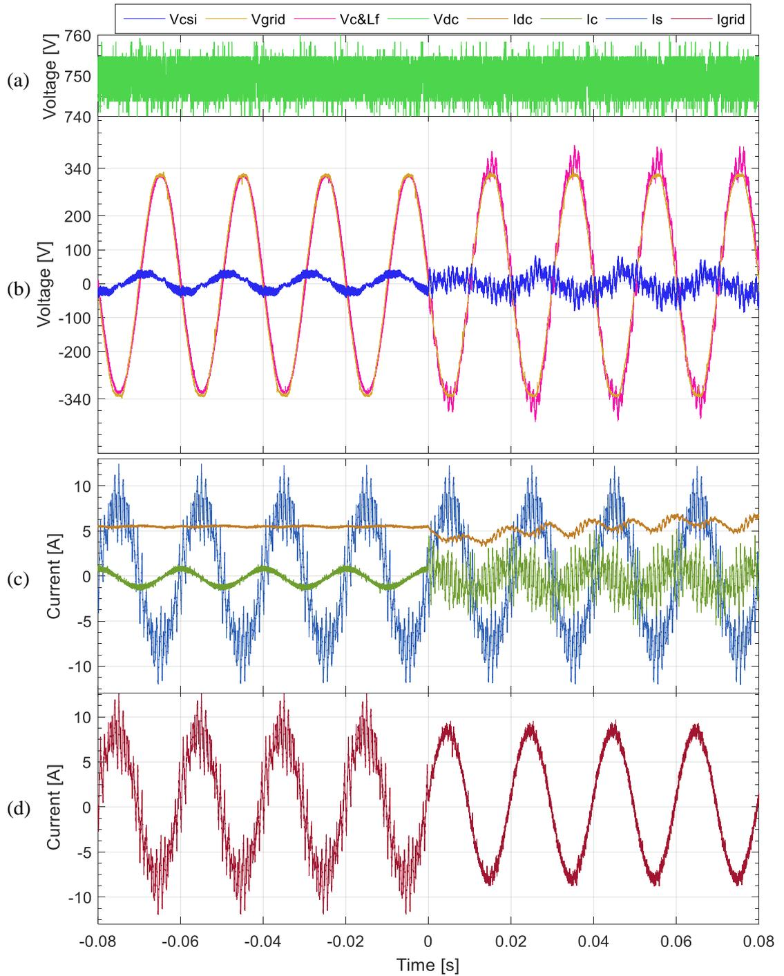
Fig 7-6: Experimental results showing activation of ripple cancellation for VSI and CSI for  $K=0.15$  for Phase A: a) VSI DC-link voltage ( $V_{dc}$ ); b) Series capacitor and filter ( $V_{c\&Lf}$ ), CSI ( $V_{csi}$ ) and grid ( $V_{grid}$ ) phase voltages; c) CSI DC-link current ( $I_{dc}$ ), Main VSI current ( $I_s$ ) and series capacitor current ( $I_c$ ), ; and d) combined grid side current ( $I_{grid}$ ).
