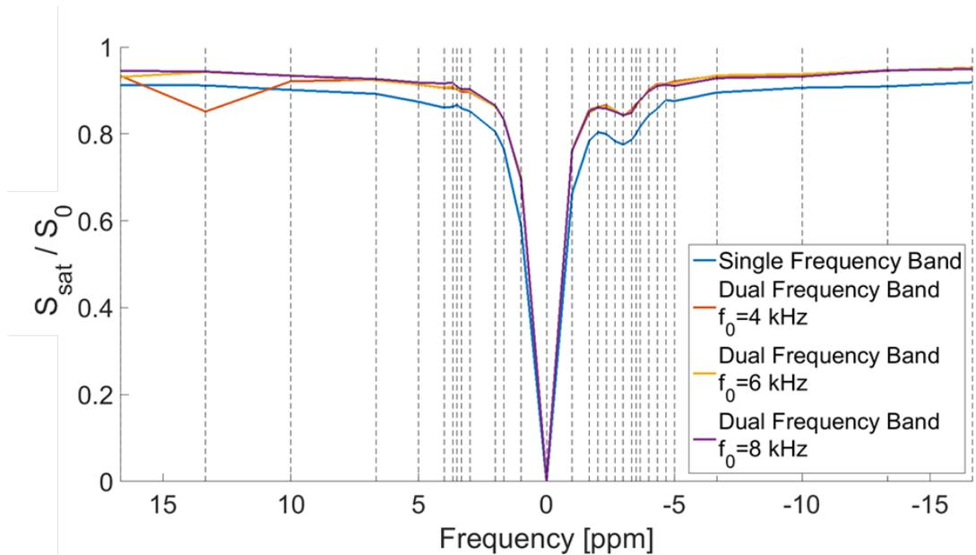
**Figure 3.19:** The z-spectra ( $B_{1,rms} = 0.43 \mu\text{T}$ ) acquired for single frequency saturation and dual-frequency saturation ( $\alpha:\beta=1:1$ ) with the location of the fixed  $f_0$  frequency located at 4, 6 and 8 kHz. Note that the peak at 13 ppm is the fixed saturation when  $f_0 = 4 \text{ kHz}$ . The vertical dashed lines represent the location of sampled frequencies in the z-spectrum.
