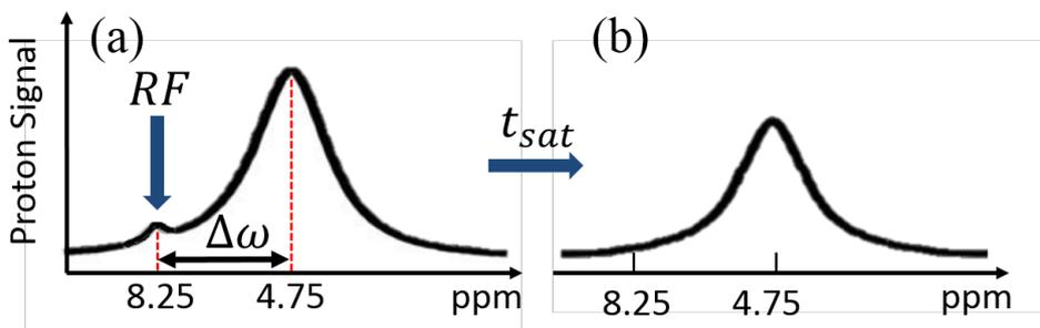
**Figure 3.3:** Solute protons are saturated at their specific resonance frequency in the proton spectrum (here 8.25 ppm for amide protons). This saturation is transferred to water (4.75 ppm) at exchange rate  $k$ . After a period  $t_{sat}$ , this effect becomes visible on the water signal (b).
