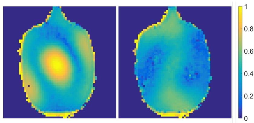
(a) Nominal  $B_1$  magnitude profiles for both RF transmit channels
