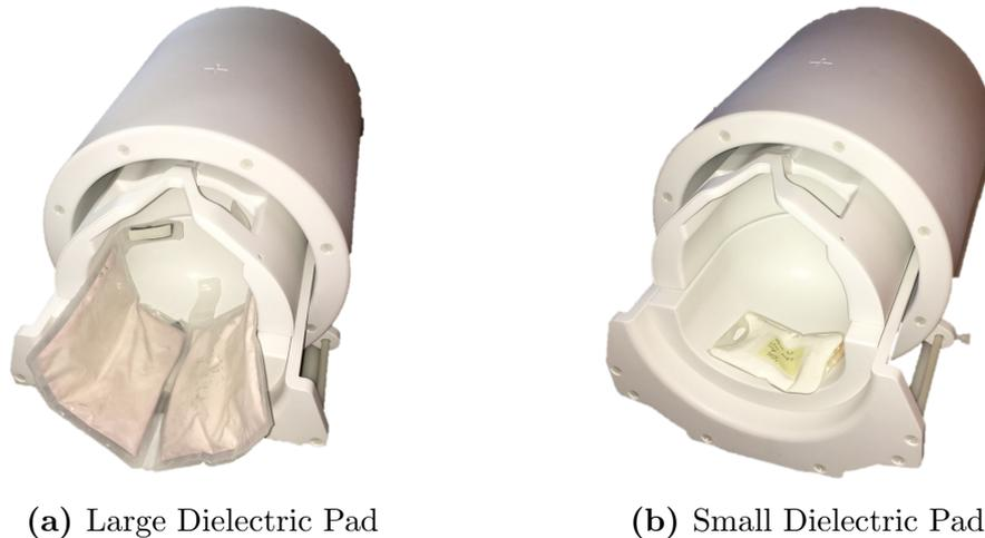
**Figure 2.3:** The positioning of the (a) large and (b) small dielectric pads in the Nova Medical volume transmit/receive coil.
