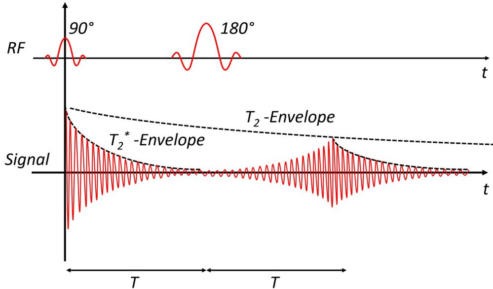
**Figure 1.7:** Schematic of spin-echo sequence consisting of a  $90^\circ$  excitation pulse and a  $180^\circ$  refocusing pulse to stimulate an echo used to measure  $T_2$ .
