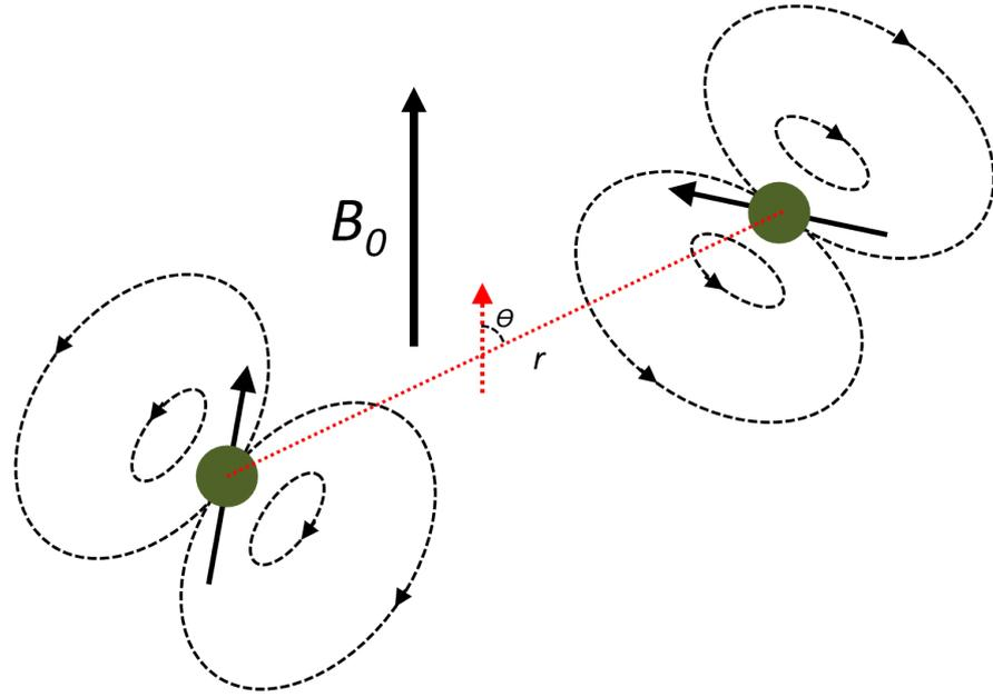
**Figure 1.9:** Two randomly tumbling magnetic dipole moments that are separated by the distance  $r$ . They are in close proximity such that they both influence the magnetic field each experiences, and the fluctuations in the magnetic field they experience due to the tumbling, induces relaxation processes.
