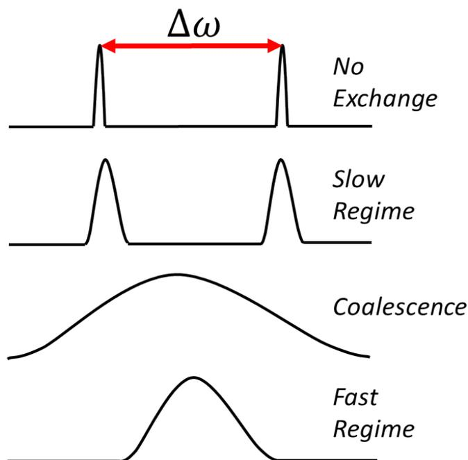
**Figure 3.5:** Schematic of the NMR spectrum for symmetrical two-site exchange and the dependence of the frequency of exchange in the slow regime, two distinctive peaks, occurs when  $k_{ex} < |\frac{\Delta\omega}{2}|$ . Coalescence, the merging of the two NMR peaks,  $k_{ex} = |\frac{\Delta\omega}{2}|$  and the fast regime, one NMR peak detectable,  $k_{ex} > |\frac{\Delta\omega}{2}|$ .
