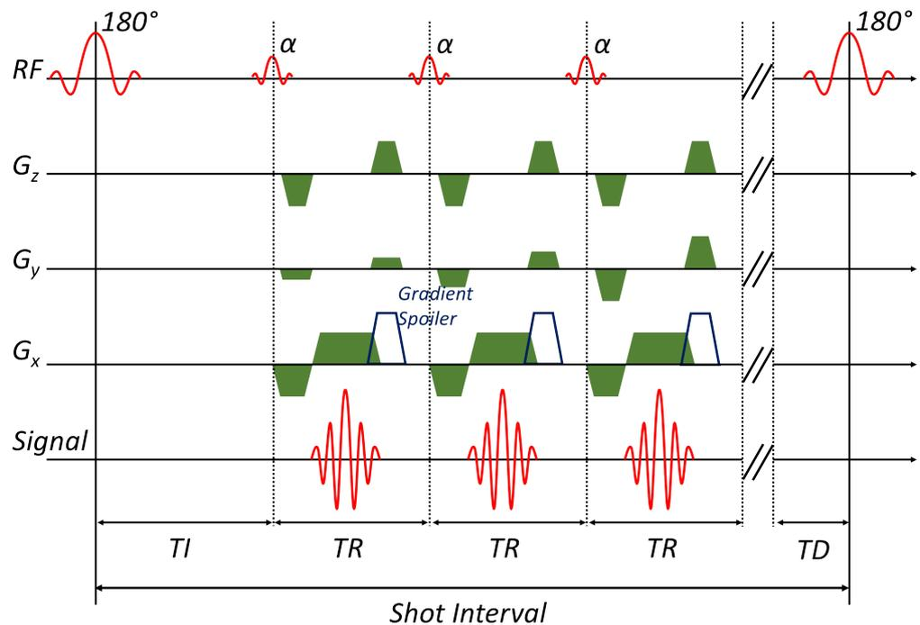
**Figure 1.14:** Magnetisation Prepared Rapid Gradient Echo (MPRAGE) sequence schematic.
