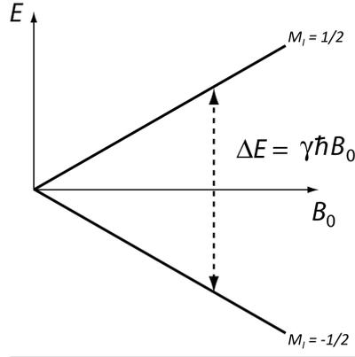
**Figure 1.3:** Energy level diagram for  $I = 1/2$  system, such as a Hydrogen atom.
