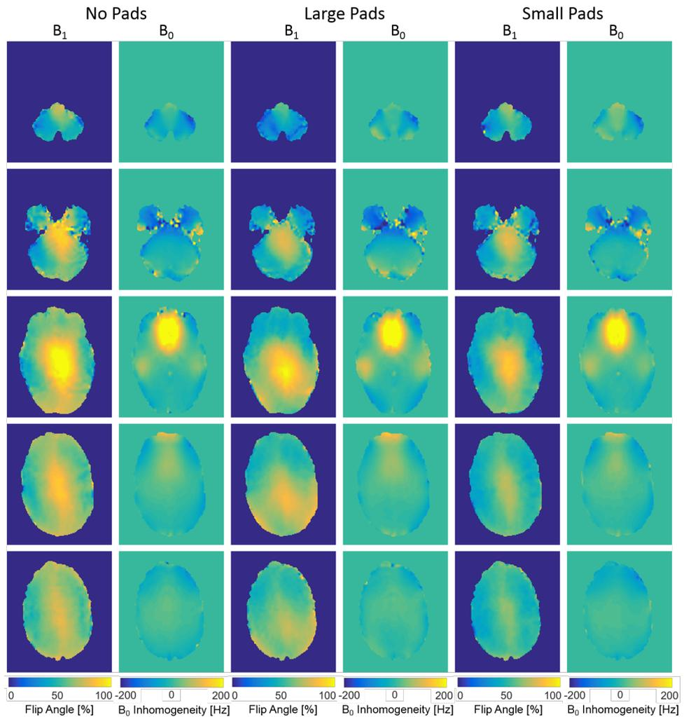
**Figure 2.5:** The  $B_0$  (in Hz) and  $B_1$  (in percentage of achieved flip angle) field maps for the large, small and no dielectric pads.
