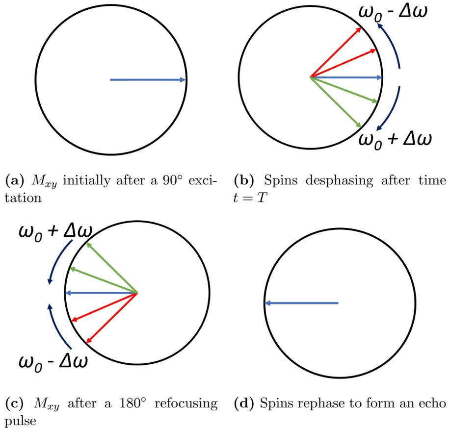
**Figure 1.8:** Schematic of the spin evolution in a spin-echo sequence.
