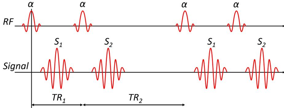
**Figure 1.17:** Timing diagram for the  $B_1$  mapping sequence (API) showing RF pulses and detected signals for the two TRs.
