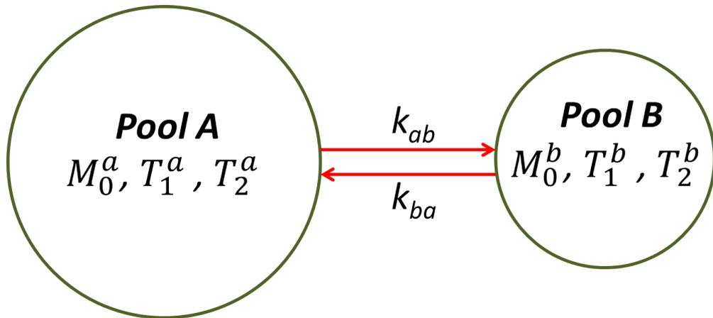
**Figure 3.6:** The two-pool model with exchange.  $M_0^{a,b}$  are the relative concentration of protons in exchange pools,  $T_2^{a,b}$  are the transverse relaxation times for both pools,  $T_1^{a,b}$  the longitudinal relaxation rate,  $k_{a,b}$  and  $k_{b,a}$  the exchange rate constants governing exchange between the pools.
