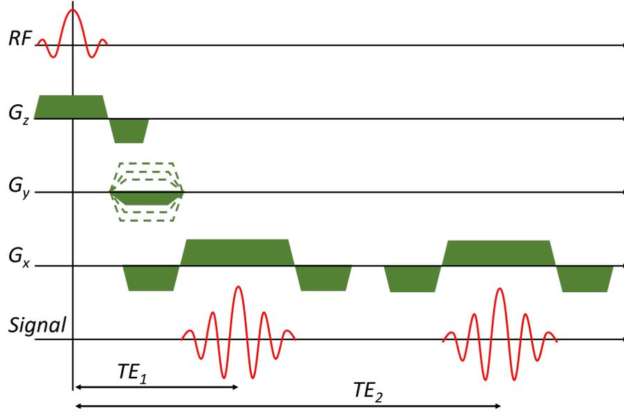
**Figure 1.16:** Dual Gradient Echo used to measure the  $B_0$  field.
