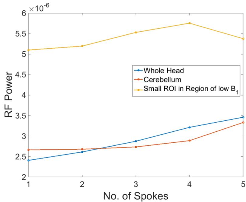
**Figure 2.12:** The RF power (Equ.2.8) for each spoke for the three target excitations.
