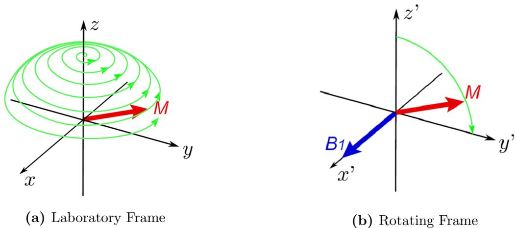
**Figure 1.4:** The evolution of the bulk magnetisation  $\mathbf{M}$  after the application of an on-resonance RF pulse in the (a) laboratory and the (b) rotating frame of reference.
