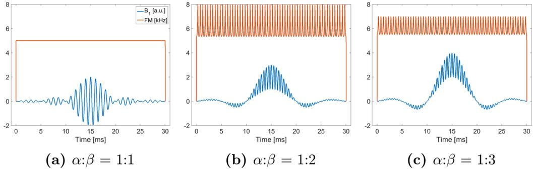
**Figure 3.13:** The amplitude (blue) and frequency (red) modulations of the designed dual-frequency band saturation RF pulses.
