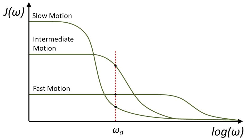
**Figure 1.10:** Spectral density function  $J(\omega)$  for three molecules with different correlation times  $\tau_c$ .
