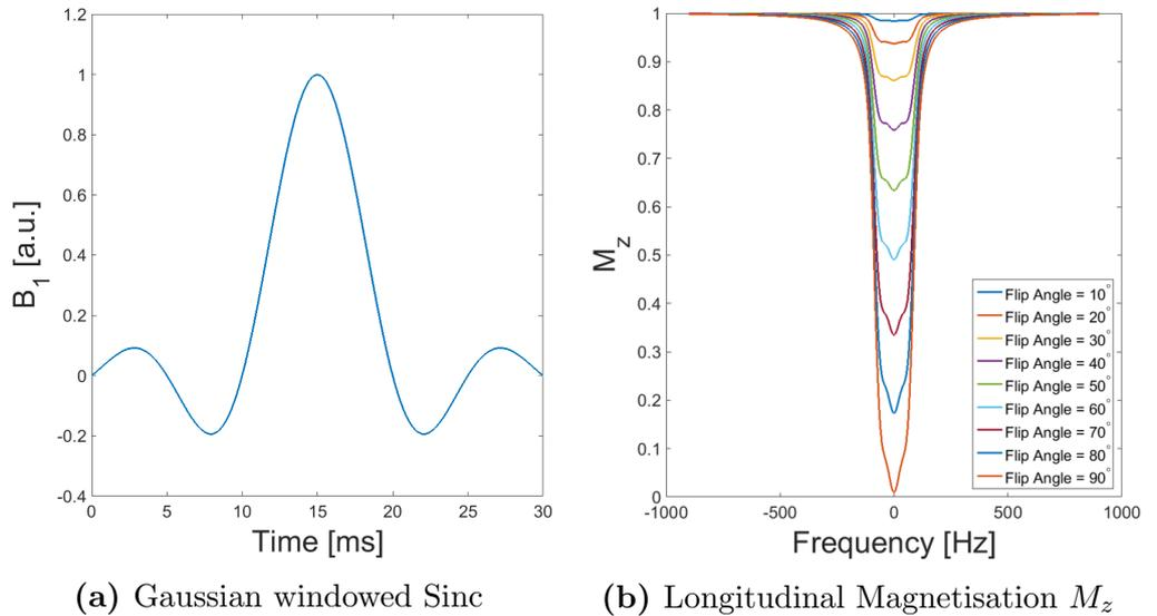
**Figure 3.12:** The (a) Gaussian windowed sinc (with normalised amplitude) and (b) the longitudinal magnetisation frequency profile for flip angles between 10° and 90° showing that the bandwidth of the magnetisation broadens for larger flip angles. As a result, Lorentzians with wider full width half maximums (FWHM) are fitted for the direct saturation in Lorentzian lineshape model fitting for higher  $B_1$  powers.
