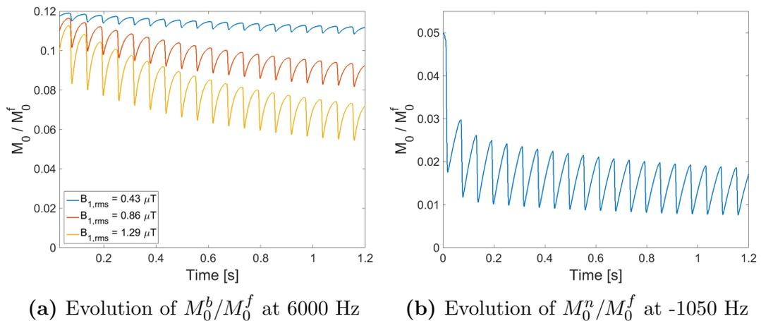
**Figure 3.15:** The evolution of the macromolecular bound pool  $M_0^b$  and the NOE pool  $M_0^n$  during the application of dual-frequency saturation pulses,  $\alpha:\beta = 1:1$ ,  $1:2$  and  $1:3$ .
