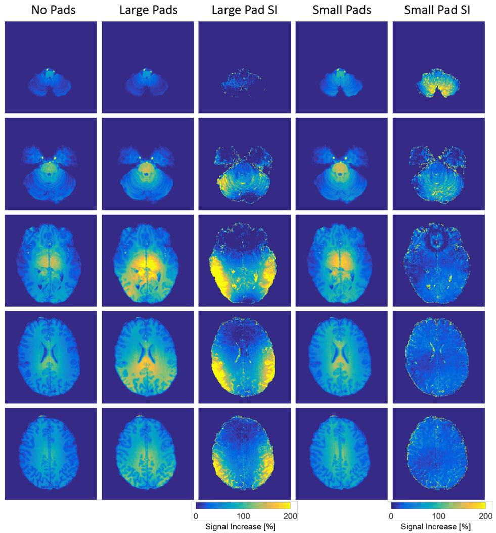
**Figure 2.4:** MPRAGE images with no dielectric pads, small and large dielectric pads (set to the same scale) and the percentage Signal Increase (SI) between small or large dielectric pads and no pads.
