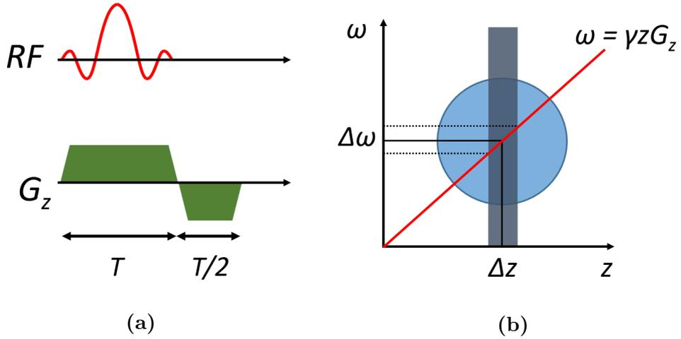
**Figure 1.11:** (a) An RF excitation pulse of  $\Delta\omega$  bandwidth applied over a slice selection gradient, followed by a negative rewind to refocus the signal. (b) A slice of thickness  $\Delta z$  is excited.
