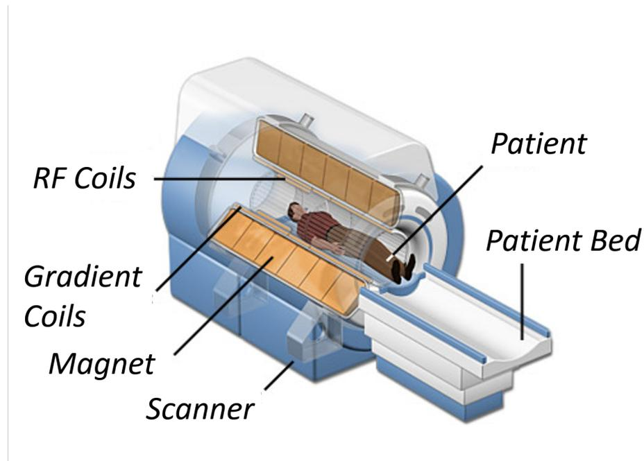
**Figure 2.1:** Schematic of a whole-body MRI scanner indicating the location of the main magnet, gradient and RF coils.
