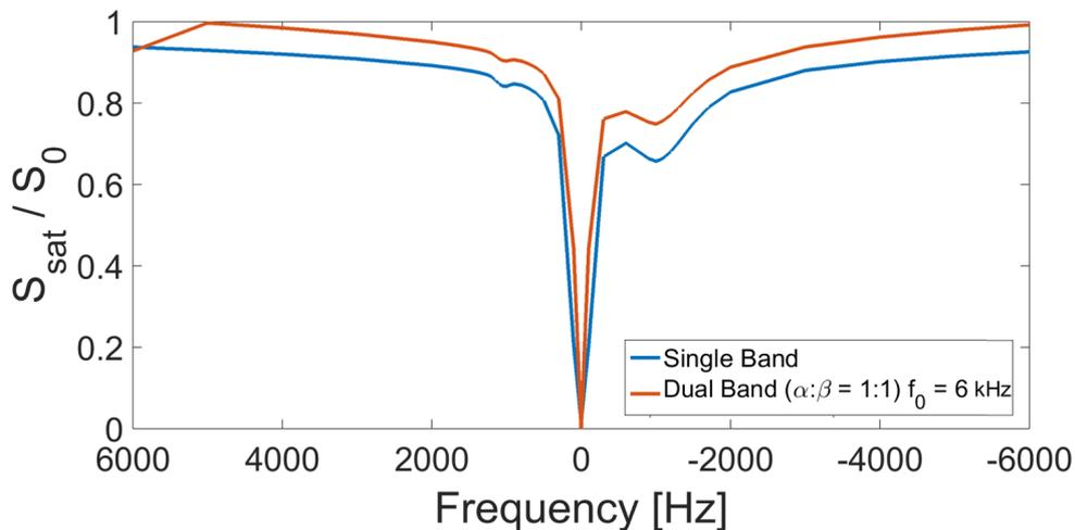
**Figure 3.16:** Simulated z-spectra for the single and dual-frequency band saturation for  $B_{1,rms} = 0.43 \mu\text{T}$ .
