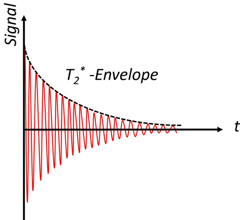
**Figure 1.5:** A free induction decay (FID) signal with a  $T_2^*$  envelope.
