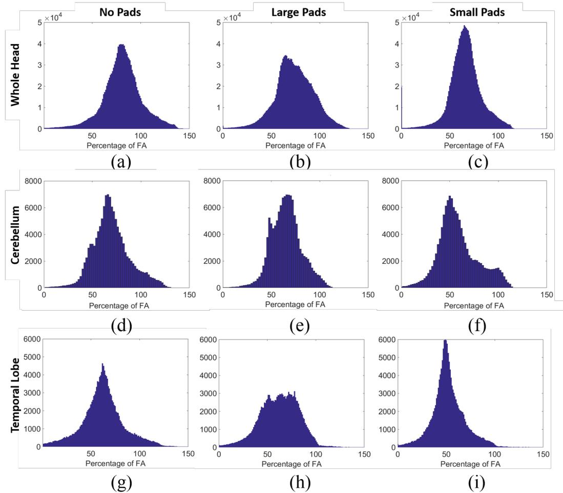
**Figure 2.6:** Histograms for the achieved flip angle: (a-c) whole head for no dielectric pads, large and small dielectric pads respectively. (d-f) the cerebellum for no dielectric pads, large and small dielectric pads respectively. (g-i) the temporal lobes for no dielectric pads, large and small dielectric pads respectively.
