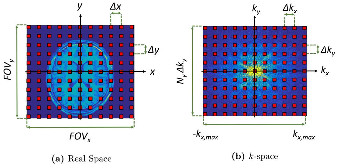
**Figure 1.12:** The relationship between the FOV, spatial resolution and sampling between real space and  $k$ -space.
