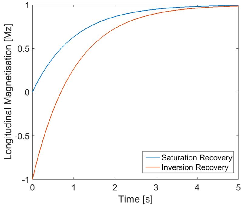
**Figure 1.6:** The longitudinal magnetisation signal recovery for  $T_1 = 1$  s in a saturation and inversion recovery experiment (i.e. following a  $90^\circ$  or  $180^\circ$  pulse).
