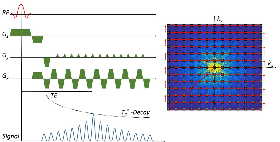
**Figure 1.15:** Schematic of Gradient Echo-EPI sequence (left) and the  $k$ -space trajectory (right).
