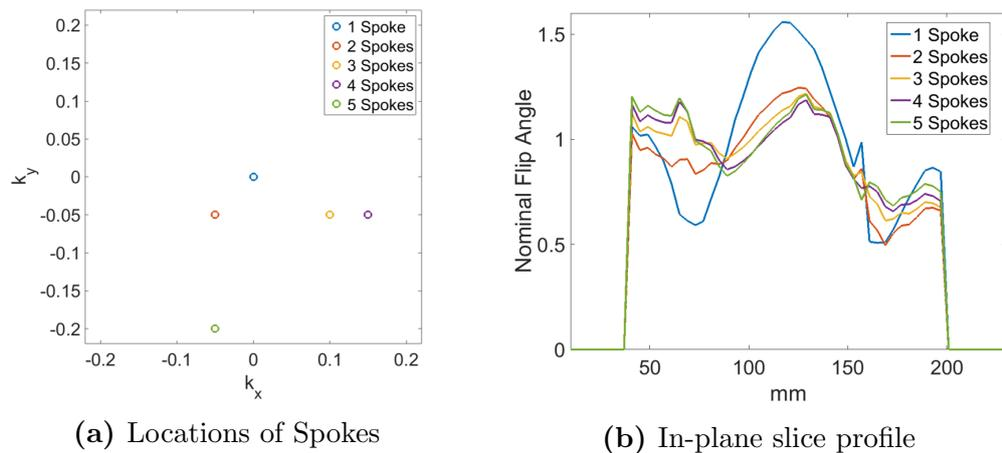
**Figure 2.10:** (a) The location of the spokes in  $k$ -space and (b) the through plane  $B_1$  transmit profile for the  $N$  spokes for the whole head excitation pulse design.
