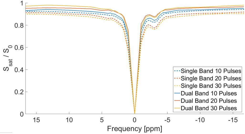
**Figure 3.17:** The z-spectra ( $B_{1,rms} = 0.43 \mu\text{T}$ ) achieved for single frequency saturation and dual-frequency saturation ( $\alpha = \beta = 1$ ) with the (a) 10, (b) 20 and (c) 30 RF saturation pulse in the saturation train.
