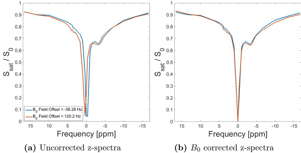
**Figure 3.21:** (a) Two z-spectra (without MT suppression) in the WM with large  $B_0$  field frequency offsets showing the shift in the z-spectra around 0 ppm. (b) The respective  $B_0$  corrected z-spectra.
