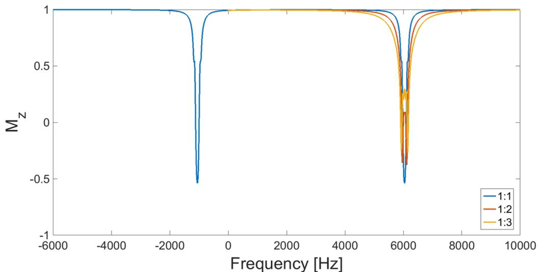
**Figure 3.14:** The longitudinal magnetisation  $M_z$  after the application dual-frequency pulses with  $\alpha : \beta$  ratios of  $f_1$  and  $f_0$  was of 1:1, 1:2 and 1:3 with  $B_{1,sat}$  in the  $f_1$  pulse of  $2.44 \mu\text{T}$ .
