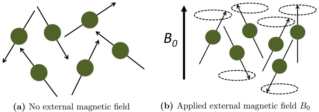
**Figure 1.1:** The nuclear magnetic moments are initially (a) randomly orientated. In an applied magnetic field  $B_0$ , (b) spins align parallel or antiparallel to the direction of the field and precess at the Larmor frequency  $\omega_0$ .
