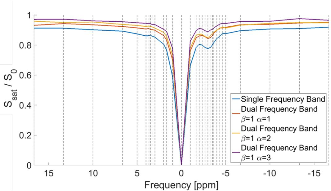
**Figure 3.18:** The z-spectra ( $B_{1,rms} = 0.43 \mu\text{T}$ ) acquired for single frequency saturation and dual-frequency saturations for  $\alpha:\beta$  ratios of 1:1, 1:2 and 1:3. The vertical dashed lines represent the location of sampled frequencies in the z-spectrum.
