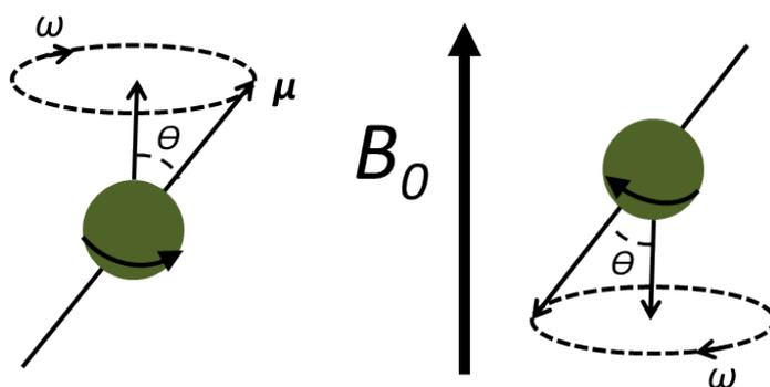
**Figure 1.2:** The precession (at Larmor frequency  $\omega_0$ ) of a proton's spins under the influence of an external magnetic field  $B_0$ .
