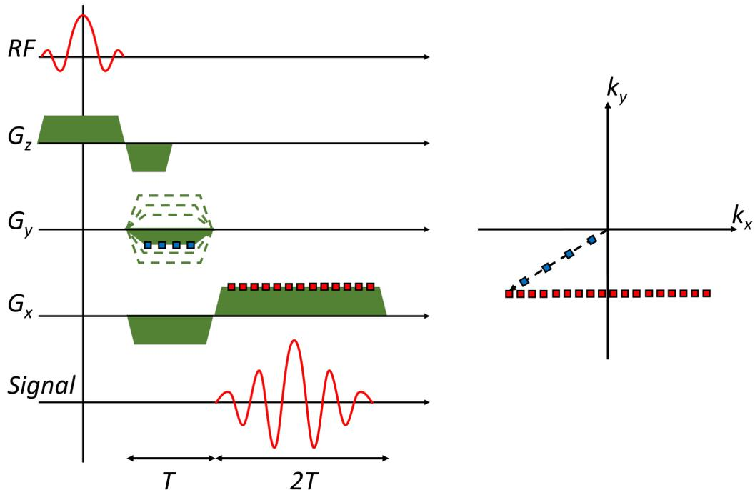
**Figure 1.13:** Schematic of gradient echo sequence and  $k$ -space trajectory.
