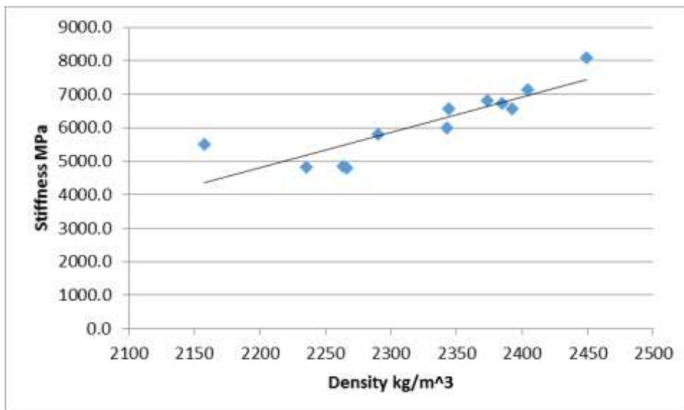
**Figure 5: Effect of Density on the Stiffness**
