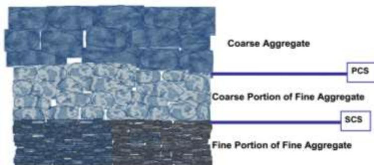
Figure 3: The Three Fractions of the Gradation (Vavrik, 2002)
