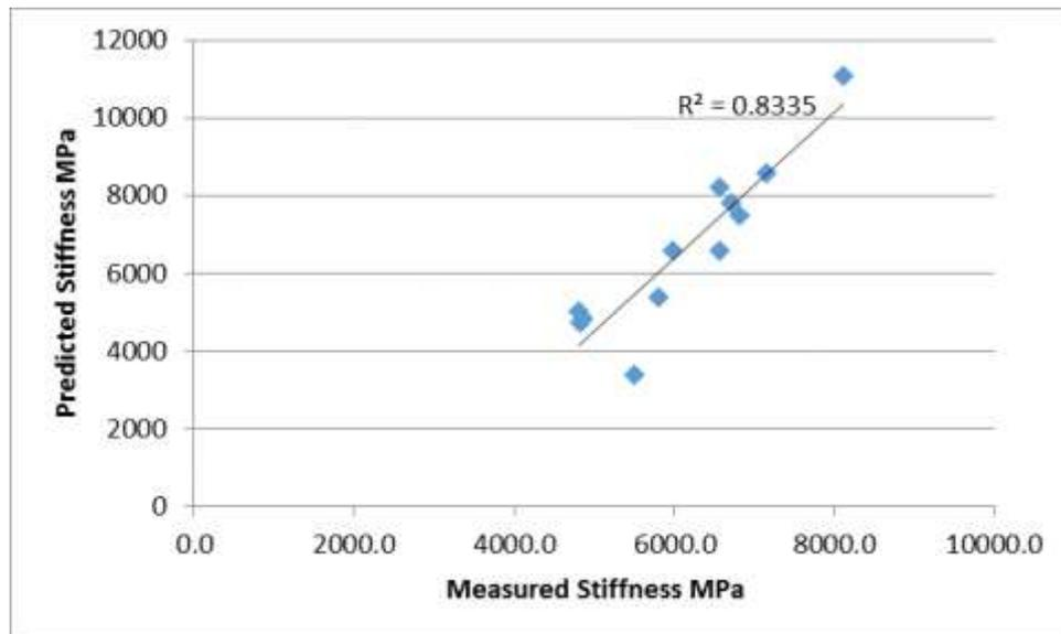
**Figure 6: Measured and Predicted Stiffness for Brown's Model**
