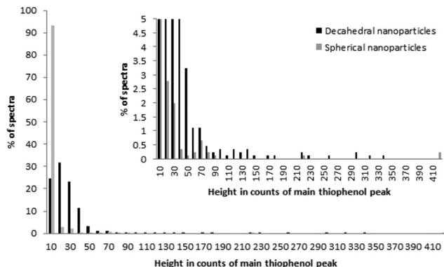
**Fig. 5** The data presented in Fig. 2 plotted as a histogram in which the intensity of Raman-scattered light recorded at the maximum of the C–C band in thiophenol has been placed into bins of 10 counts. Inset – a magnified representation of the data with low percentages. The histogram compares the data taken with a 36 nm silver decahedral nanoparticle to that taken with a 40 nm silver spherical nanoparticle.
