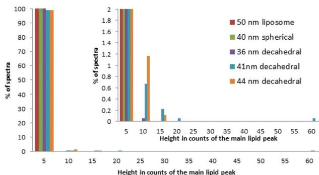
**Fig. 9** The data presented in Fig. 6 plotted as a histogram in which the intensity of Raman-scattered light recorded at the maximum of the lipid peak at  $2935\text{ cm}^{-1}$  has been placed into bins of 10 counts. Inset – a magnified representation of the data with low percentages.
