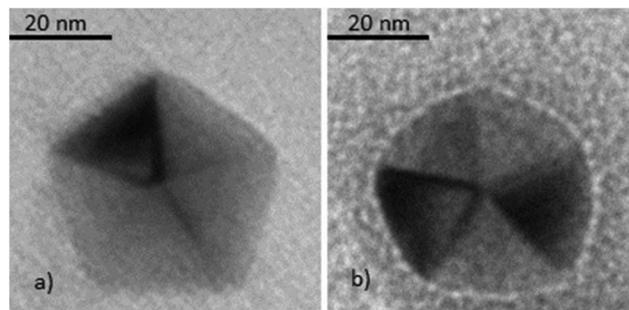
**Fig. 2** Transmission electron microscopy (TEM) images of (a) a 41 nm diameter silver decahedral nanoparticle and (b) a membrane-encapsulated 41 nm diameter decahedral nanoparticle. The TEM grids for (a) and (b) were negatively stained with 3% uranyl acetate solution to improve the contrast of the lipid bilayer surrounding the nanoparticles in image (b) and as a control in image (a).
