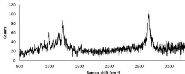
**Fig. 7** A Raman spectrum recorded from an optically-trapped 50 nm lipid vesicle encapsulating a 41 nm diameter decahedral silver nanoparticle. The acquisition time was 1 second and a background signal has been subtracted. The signal-to-noise-ratio is estimated to be between 10 and 15.
