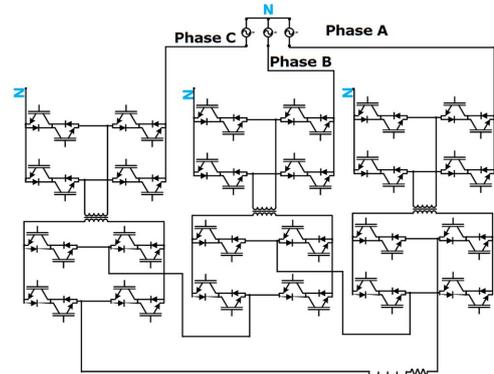
Fig. 1 The proposed isolated AC/AC three phase to single phase topology using three Dual CBM
