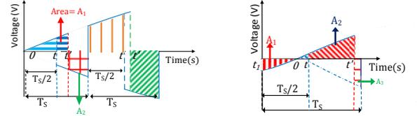
Fig. 12 (a) Selection of switching time  $t'$  to achieve ZASC (b) Selection of  $t'$  to achieve ZASC when the phase of the input voltage is non-zero.
