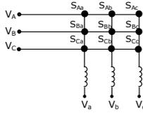
Fig. 6 A direct matrix converter with 9 bidirectional switches
