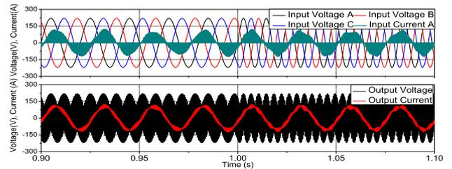
Fig. 8 Output frequency regulation at 40Hz regardless of the input frequency change, i.e 50-86 Hz, applied at time=1s
