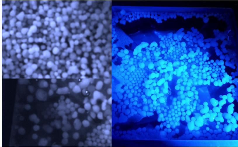
Figure 2: Ice granules in a closed glass cassette vibrated by an electromagnetic shaker, in a temperature controlled chamber at  $-3^{\circ}\text{C}$ . Top left: A dry granular gas, after 5 minutes of shaking. Bottom left: After 20 minutes of shaking, larger coalesced particles appear alongside pockets of close packed particles. Right: Once all of the granules stopped moving after 65 minutes of shaking, the cassette was opened.
