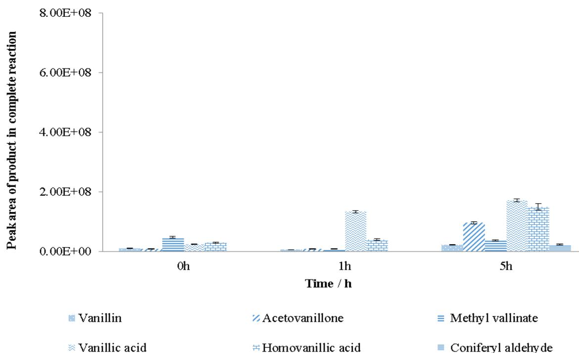
**Figure 4.11 (a):** The time course profile of Kraft lignin degradation by MnP in the presence of MnSO<sub>4</sub> (complete reaction)
