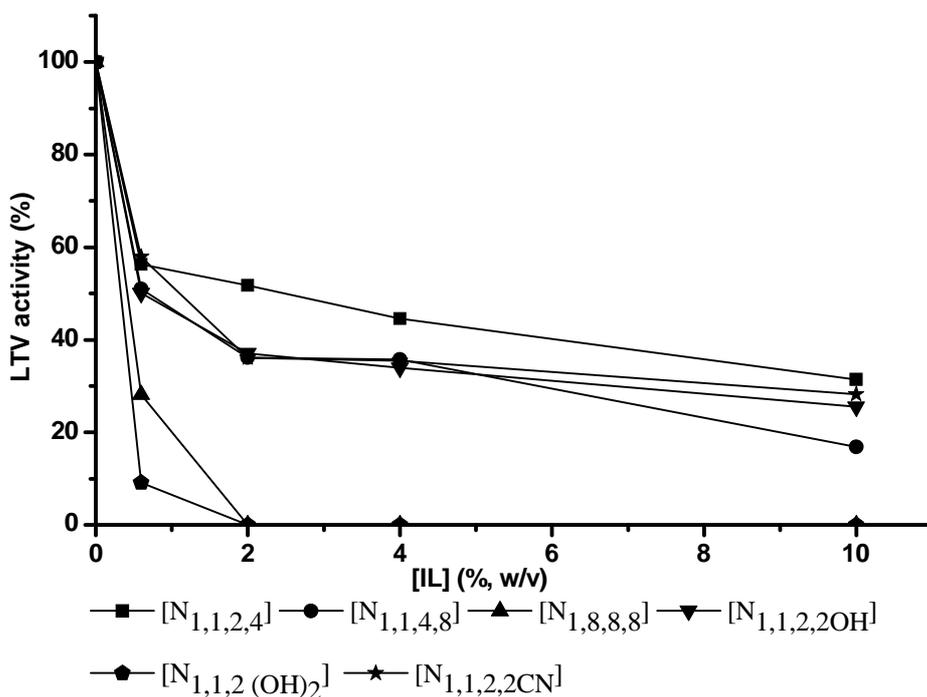
**Figure 5.7(c):** The effect of quaternary ammonium salts on LTV activity when NTf<sub>2</sub> is an anion.
