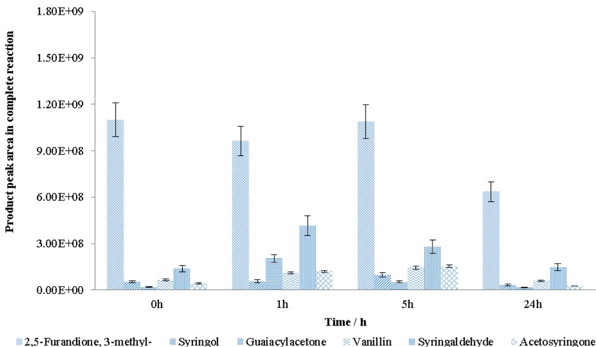
**Figure 3.18 (a):** The time course profile for the product distribution in OSL degradation by LTV in the presence of 20% ethanol (Complete reaction). Data represent the mean of two replicates with the error less than 15%.
