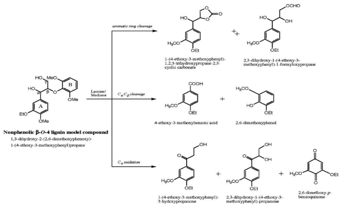
**Figure 1.13 (b):** Laccase-catalysed oxidation of a non-phenolic  $\beta$ -O-4 lignin model compound (Kawai *et al.*, 1999, Kawai *et al.*, 2002)
