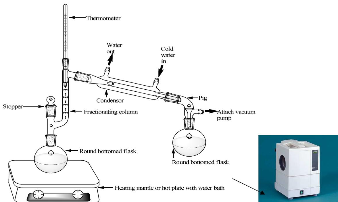
**Figure 2.2:** Schematic illustration for vacuum distillation of veratryl alcohol
