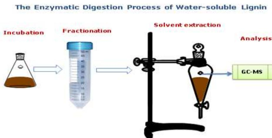
**Figure 2.4:** Schematic representation of water soluble lignosulphonate degradation
