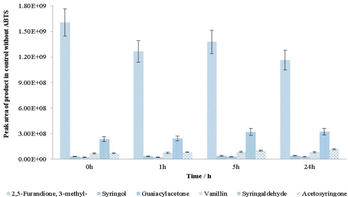
**Figure 3.18 (c):** The time course profile for the product distribution in OSL degradation without ABTS in the presence of 20% ethanol. Data represent the mean of two replicates with the error less than 15%.
