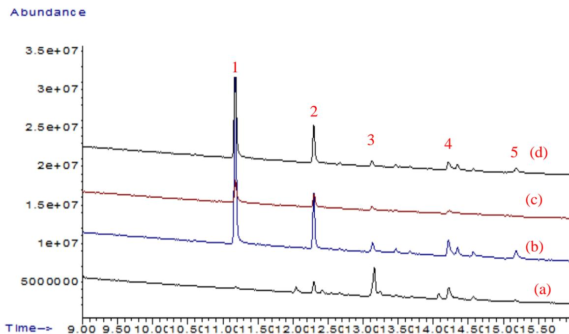
The compounds identified from Kraft lignin degradation by MnP were: vanillin (peak 1, RT=11.20 min), homovanillyl alcohol (peak 2, RT=12.86 min), vanillic acid (peak 3, RT=13.17 min), homovanillic acid (peak4, RT=14.21 min) and coniferyl aldehyde (peak 5, RT=15.50 min). All compounds were identified in the previous analysis, so mass spectra are shown.
