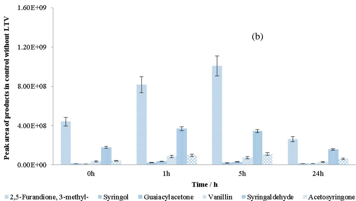
**Figure 3.17 (b):** The time course profile for control reaction (without LTV but with ABTS) of the product distribution in OSL degradation by LTV in the presence of 10% ethanol. Data represent the mean of two replicates with the error less than 15%.
