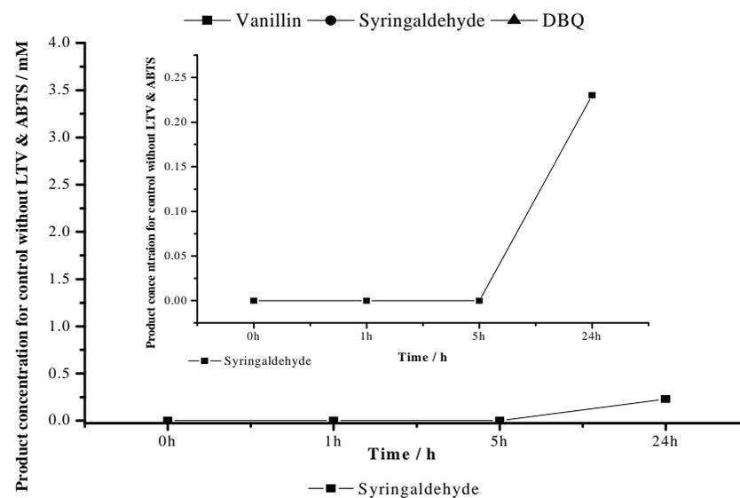
**Figure 3.14:** The effect of extra LTV & ABTS addition over 24 h of incubation at 30 °C. Original reaction mixture included 1 g OSL (29 g/L), 4 mM ABTS (11 mL), 250  $\mu$ L LTV (0.25 mg/ mL) and 100 mM ammonium acetate buffer (23 mL). LTV and ABTS were added for second time after 5 h of reaction with the same concentration and amount as they were added at the start of the reaction.
