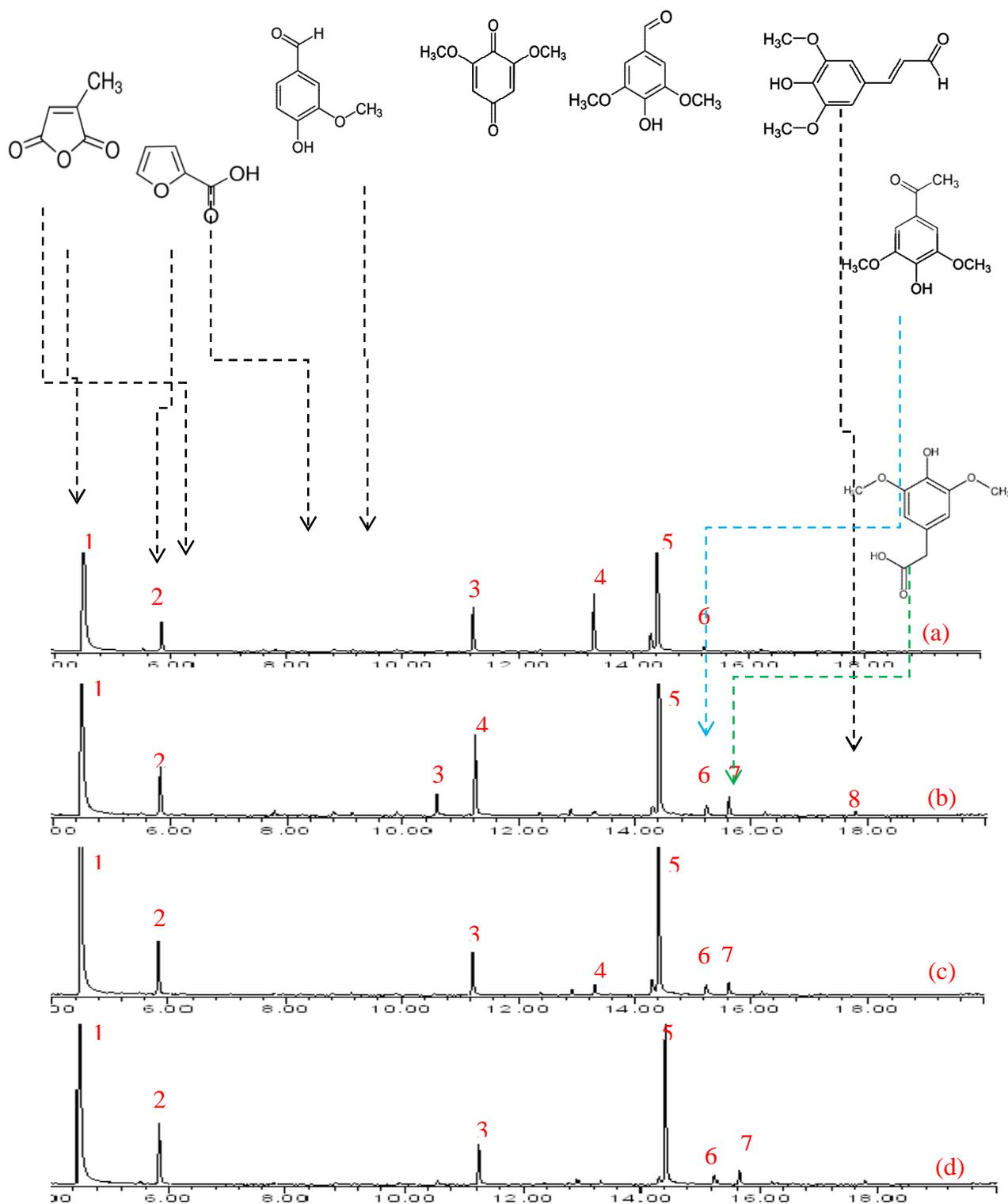
Except acetosyringone (peak 6 at RT=15.23 min) and homosyringic acid (peak 7 at RT=15.63 min), all other chemicals were formed in previous reactions. So, their mass spectra data are not shown. The observed mass spectra of the above 2 new compounds which mainly identified from the control reactions of OSL degradation by LTV at 30 °C for 72 h were as follows:
