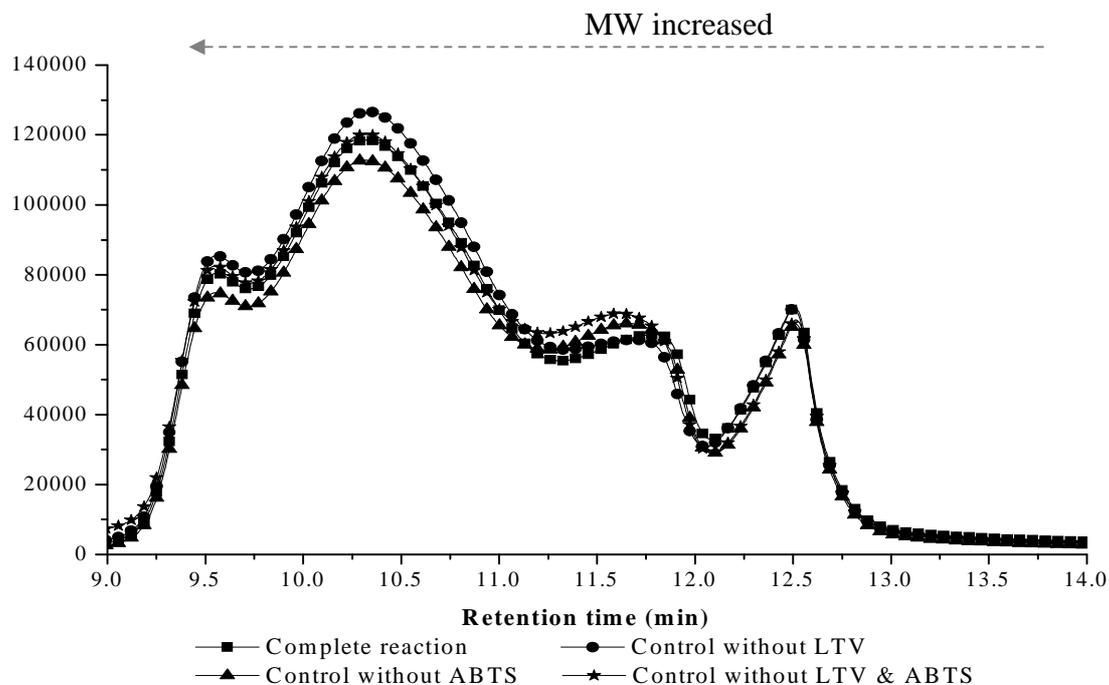
**Figure 4.7(a):** The overlaid GPC chromatograms of Kraft lignin depolymerisation by laccase and mediator at 30 °C at the beginning of the reaction ( $t=0$  h)
