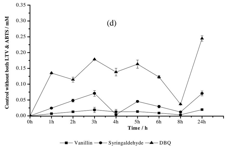
**Figure 3.9:** The product concentration *versus* reaction time graph for Organosolv lignin degradation products at 50 °C for 24 h.
