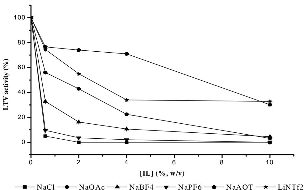
**Figure 5.5 (b):** The effects of anions on LTV activity when equivalent sodium or lithium salts as control.
