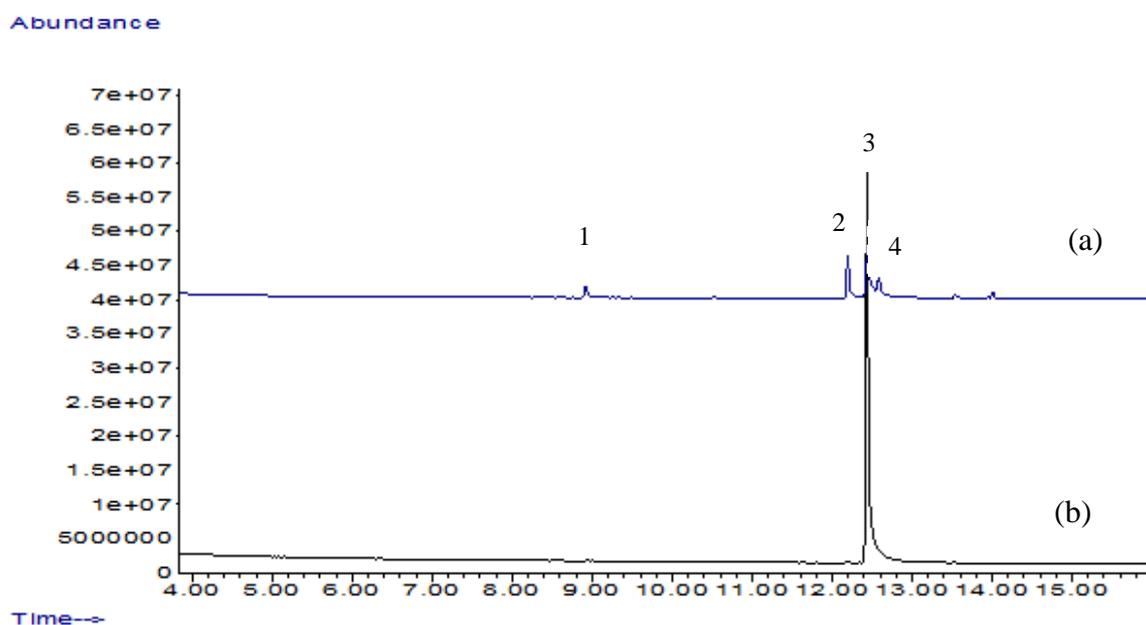
The veratryl alcohol before distillation was appeared at RT = 12.43 min (peak 3) and it was mainly contaminated by 3, 4-dimethoxytoluene (peak 1, RT = 8.92 min), veratraldehyde (peak 2, RT = 12.20 min) and homoveratric acid (peak 4, RT= 12.58 min).
