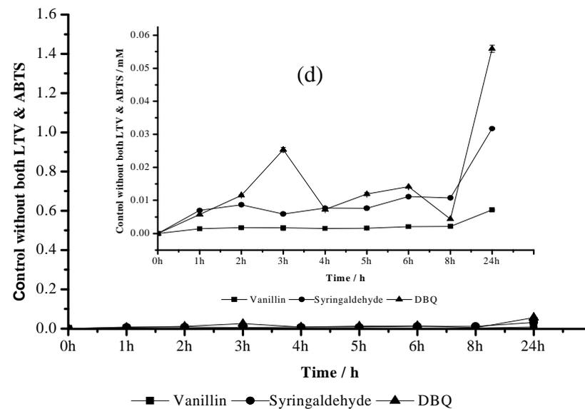
**Figure 3.7:** The product concentration *versus* reaction time graph for Organosolv lignin degradation products at 30 °C for 24h.
