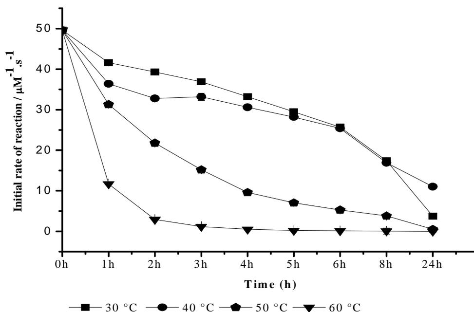
**Figure 3.3:** Thermo-stability test of LTV between 30 and 60 °C.
