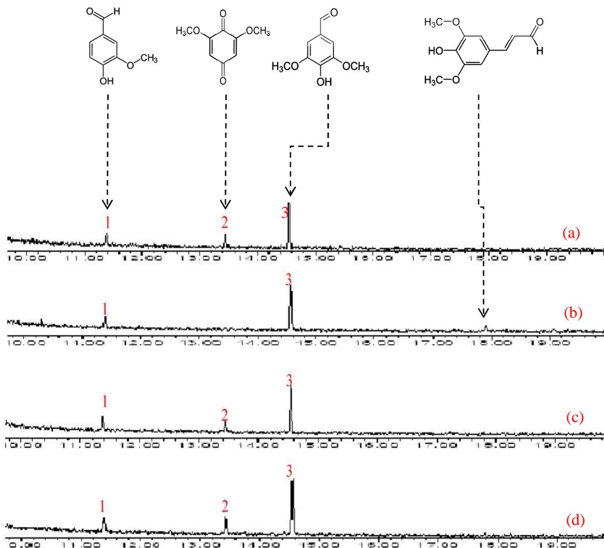
The GC-MS identified major products from organosolv degradation at 60 °C were vanillin (peak 1), DBQ (peak2), syringaldehyde (peak3) and sinapaldehyde (peak4). The organosolv degradation products from the reaction at 60°C are similar with those formed at 40 °C and 50 °C except the peak areas of all products were apparently decreased. It indicates that 60 °C is not an ideal reaction temperature for LTV catalysed OSL degradation.
