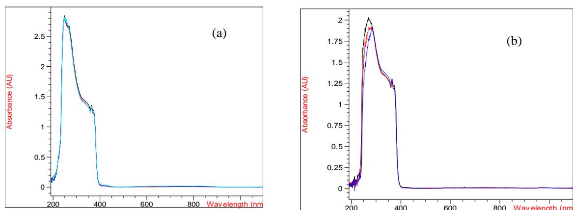
**Figure 5.1:** (a) Spectrum of ABTS after oxidation by LTV as a catalyst in (a); (b) presence of [C<sub>2</sub>mim][Lactate]
