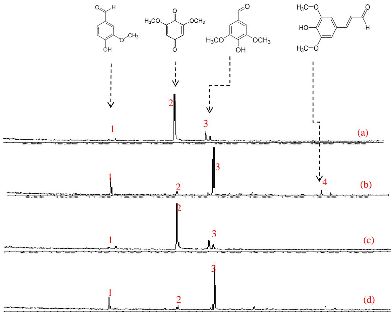
The main products formed from Organosolv degradation by LTV at 30 °C were vanillin (peak 1), DBQ (peak 2), syringaldehyde (peak 3) and trace amount of 3,5-Dimethoxy-4-hydroxycinnamaldehyde (sinnapaldehyde, peak 4).
