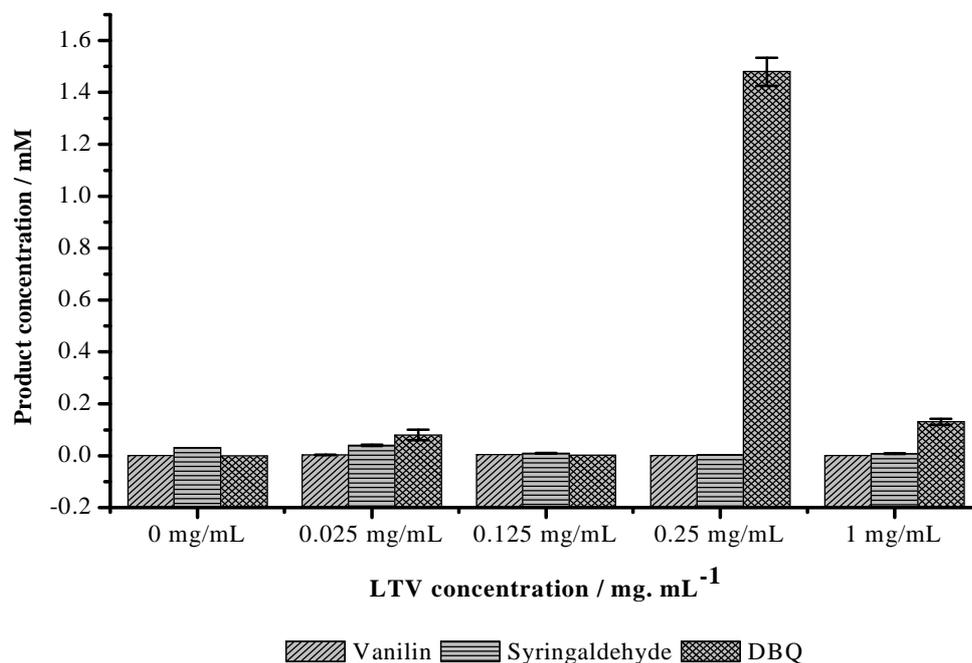
**Figure 3.13:** The effect of laccase concentration on the degradation products of OSL.
