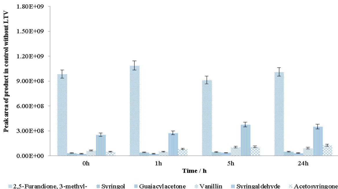
**Figure 3.18 (b):** The time course profile for the product distribution in OSL degradation without LTV in the presence of 20% ethanol. Data represent the mean of two replicates with the error less than 15%.
