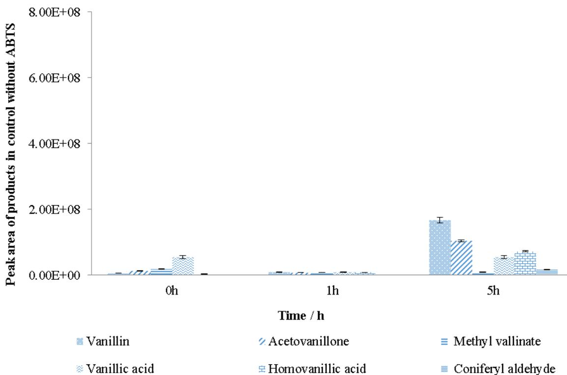
**Figure 4.11 (c):** The time course profile of Kraft lignin degradation in the absence of MnSO<sub>4</sub>
