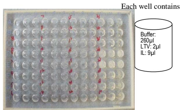
**Figure.2.1 (b)** a visual image of 96 well quartz microplate assays
