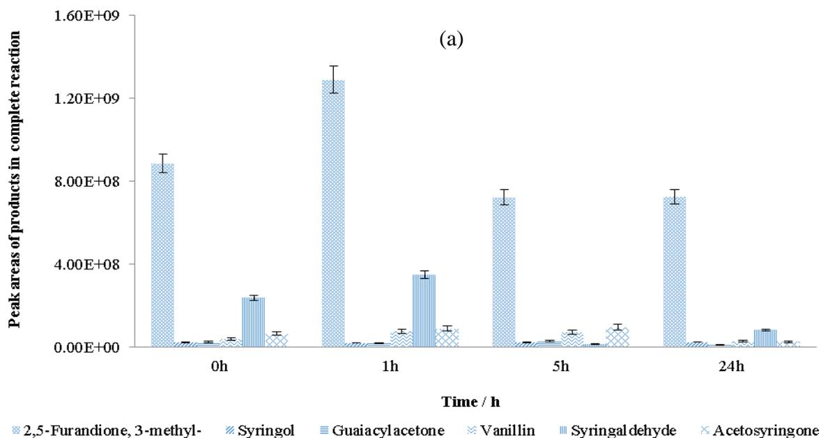
**Figure 3.17(a):** The time course profile of complete reaction (in the presence of both LTV&ABTS) for the product distribution in OSL degradation by LTV in the presence of 10% ethanol. Data represent the mean of two replicates with the error less than 15%.
