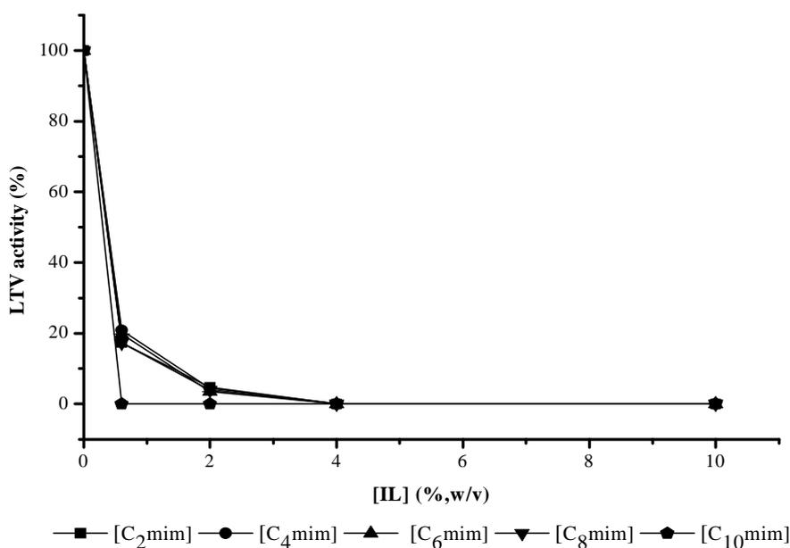
**Figure 5.4 (a):** Effect of IL concentration of different alkyl side chain length of imidazolium chlorides ( [C<sub>x</sub>mim][Cl] ) on LTV activity. Data represent triplicate analyses with a standard deviation less than 0.1. Therefore, the error bar is not shown in the graph.
