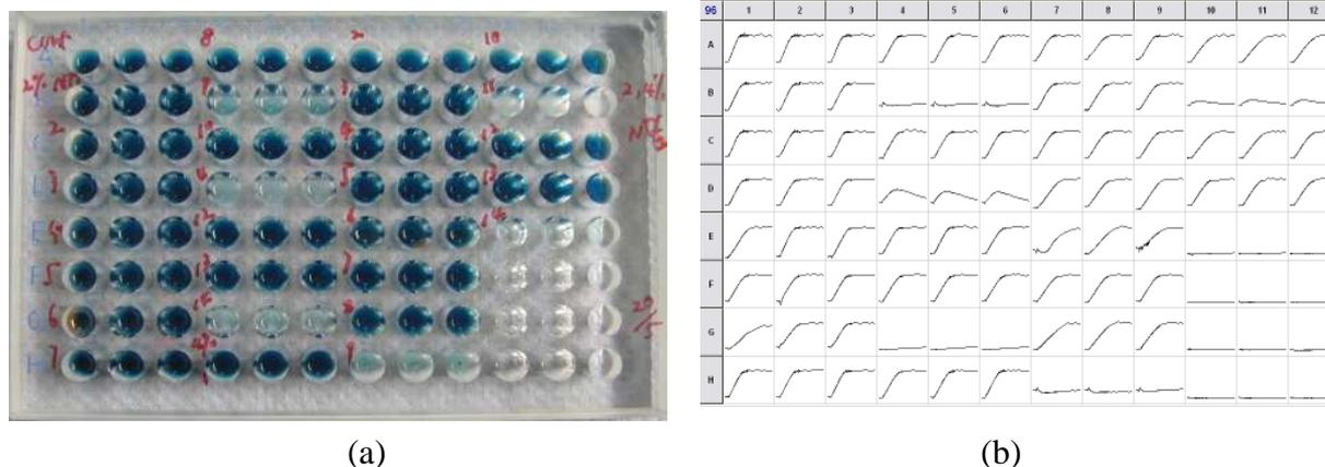
**Figure 5.3:** (a) An image of ABTS colour change in the presence of different ILs in a 96- well plate assay; (b) Comparison of OD<sub>420</sub> for ILs which contained NTf<sub>2</sub> as anion using 2 % to 4 % [IL] to show the difference of the measured activity curve versus control.
