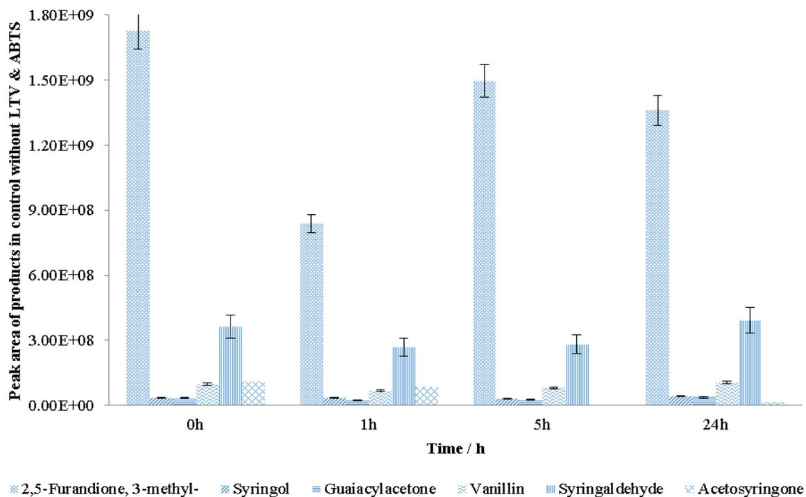
**Figure 3.18 (d):** The time course profile for the product distribution in OSL degradation in the control without both LTV and ABTS. Data represent the mean of two replicates with the error less than 15%.
