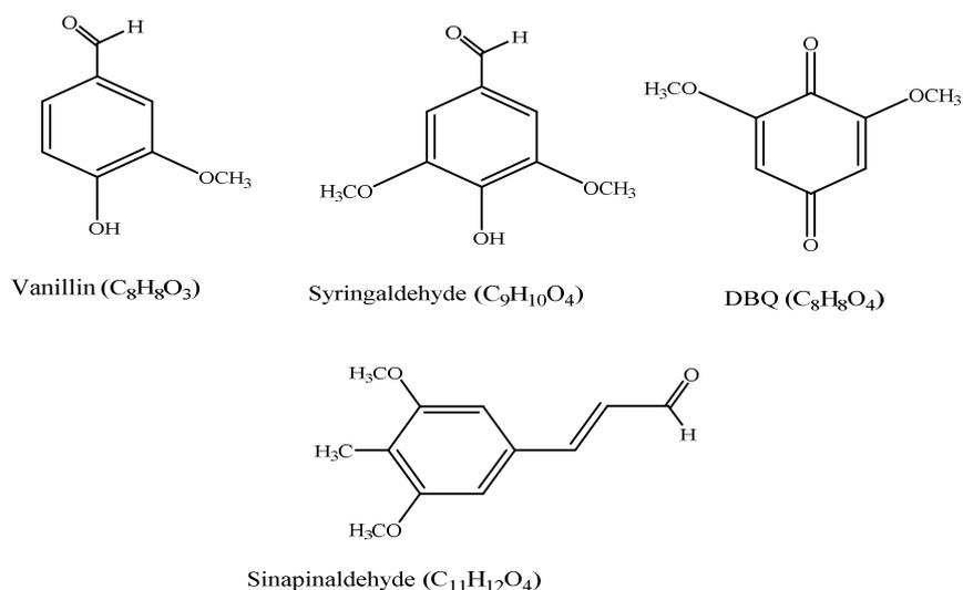
**Figure 3.6:** Chemical structures of Organosolv lignin depolymerisation products
