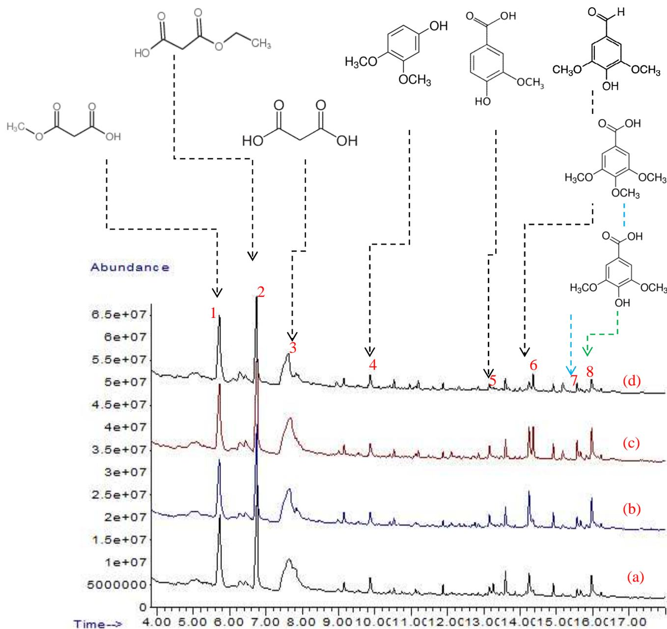
Among the identified compounds formed from both complete reaction and controls, the 3-methoxy-3-oxopropanoic acid (peak 1, RT = 5.69 min), ethyl hydrogen malonate (peak 2, RT = 6.73 min), malonic acid (peak 3, RT = 7.60 min) were unlikely related to the enzymatic degradation reaction and they might come from the reaction components. The 3,4-dimethoxyphenol (peak 4, RT = 10.53
