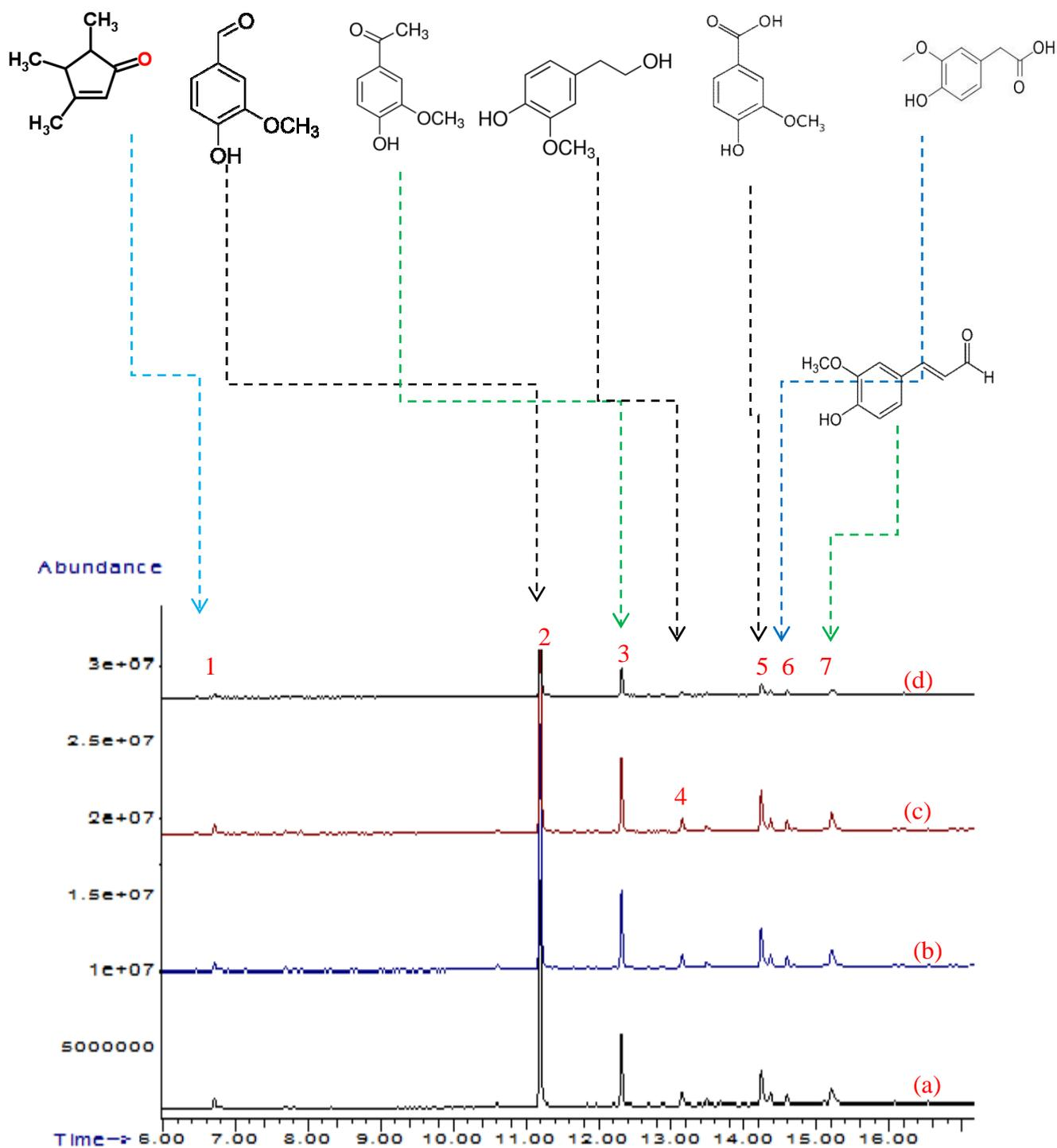
The compounds identified from Kraft lignin degradation by LTV were: 3,4,5-Trimethyl-2-cyclopenten-1-one (peak 1, RT=6.71 min), vanillin (peak 2, RT=11.20 min), acetovanillone (peak 3, RT=12.30 min), homovanillyl alcohol (peak 4, RT=12.86 min), vanillic acid (peak 5, RT=13.17 min), homovanillic acid (peak6, RT=14.21 min) and the 4-Hydroxy-2-methoxycinnamaldehyde (Coniferyl aldehyde, peak 7, RT=15.50 min). Except
