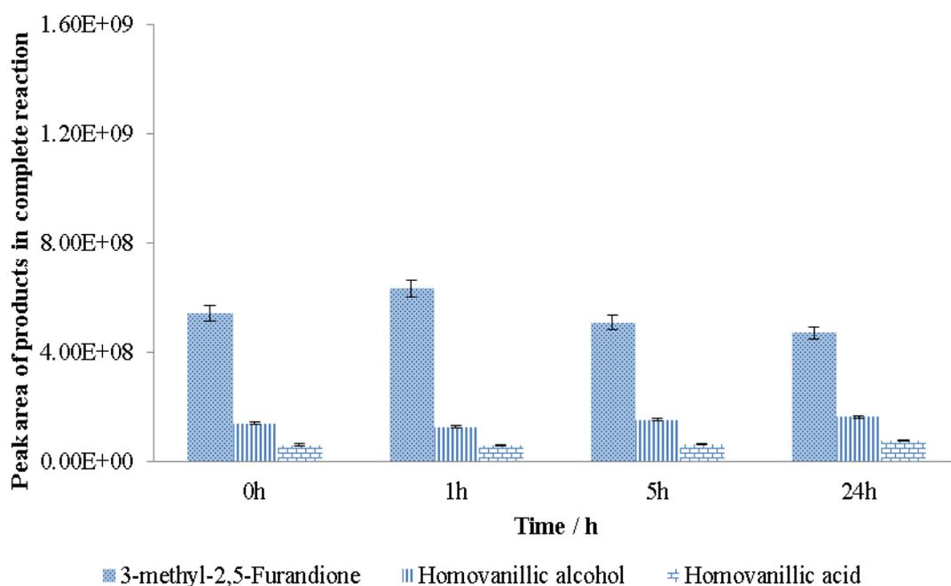
**Figure 4.2 (a):** The time course profile of liginosulphonate digestion by laccase in the presence of ABTS (complete reaction)
