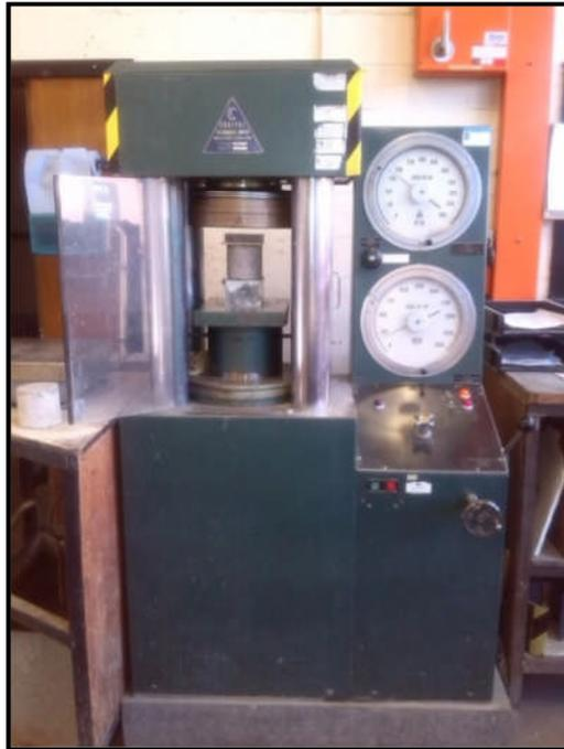
Figure 5.2: UCS testing machine used in this study.
