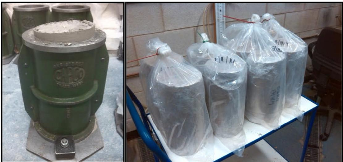
Figure 5.1: Large cylinders (> 300 mm height); b. samples curing.
