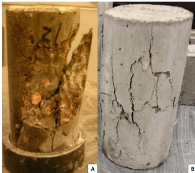
Figure 3.14: Failure pattern under static compressive loading for plain (left) and rubberized (right) concretes (Liu 2013)
