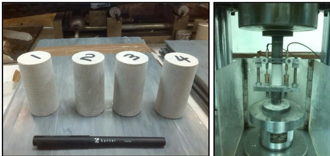
Figure 4.5: a. Aggregate cores and b. testing set-up for UCS of aggregate
