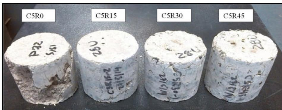
Figure 5.23: Failure patterns of UCS samples containing different rubber contents and 5% cement.
