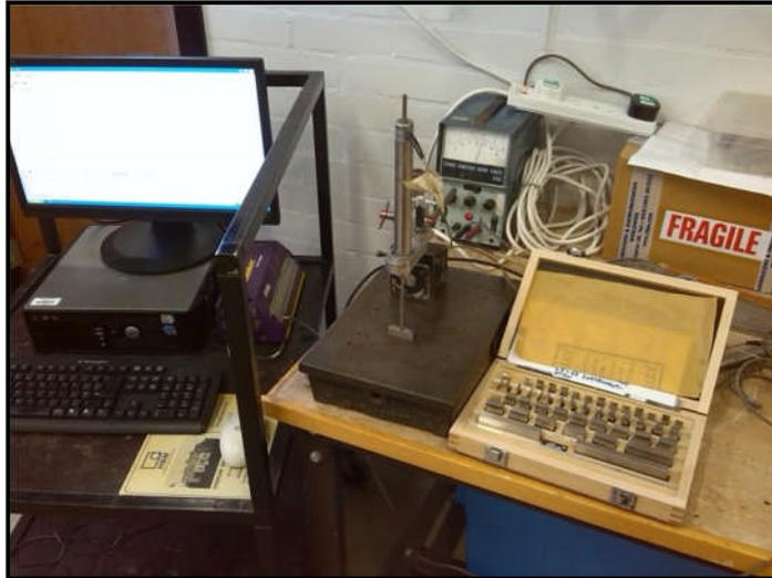
Figure 8.8: Illustration of LVDT calibration using blocks of known thickness
