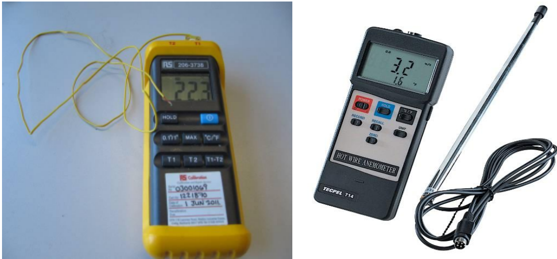
Figure 6.3 Digital thermometer used for refrigerant temperature readings and hot-wire anemometer used for air temperature and velocity
