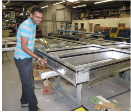
Assembly of inner frame
