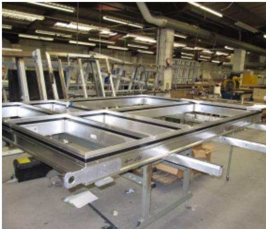
Inner Frame with hanging brackets
