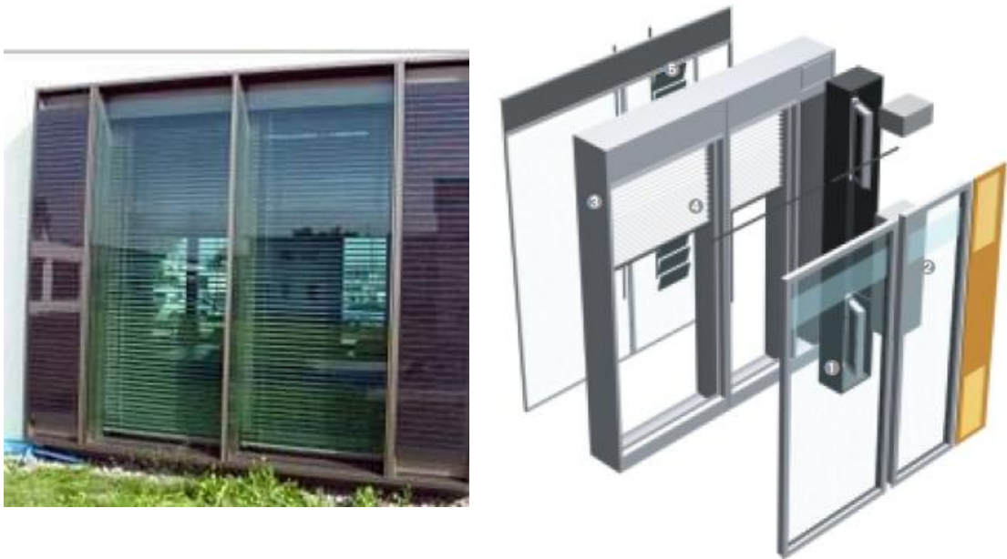
Figure 2.15 TE motion unit as installed at the Hydro test centre and spatial arrangement (Wicona 2010)
