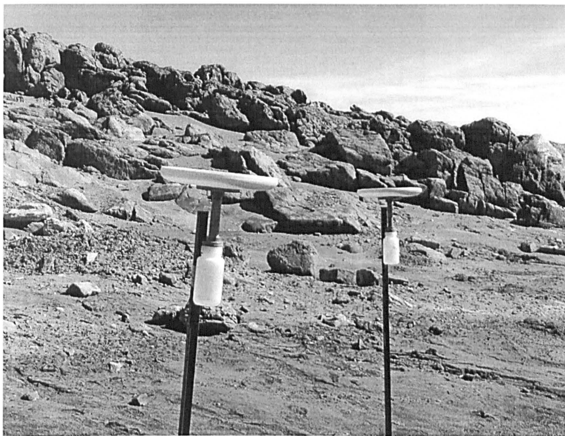
Plate 3.3. A pair of “Frisbee” settled particle samplers in place on Davis Beach.
