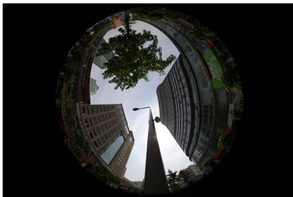
Fig. 5.45: SVF photo of Fumao Mansion taken by fish eye lens
