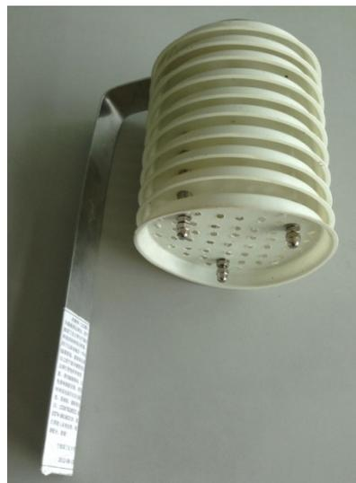
Fig. 4.11: New design of radiation shield
