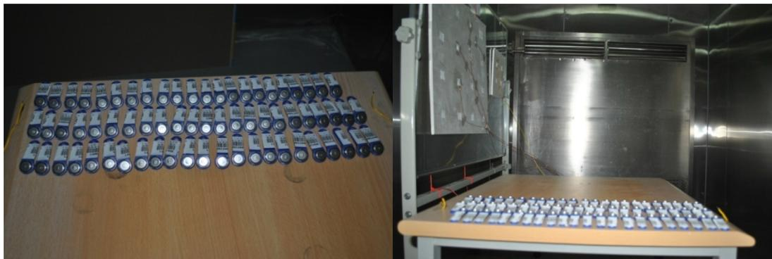
Fig. 4.4: The arrangement of i-Button DS1923 data logger in the chamber
