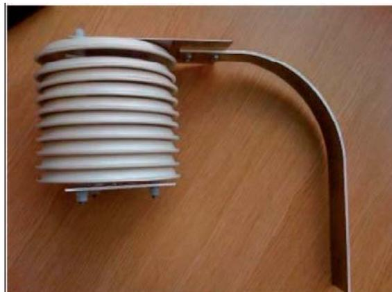
Fig. 4.8: Original design of radiation shield
