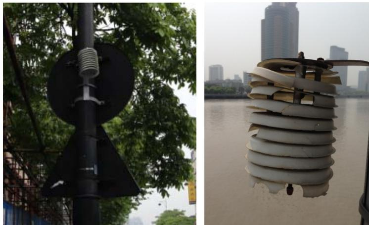
Fig. 4.14: Radiation shield obstructed by direction board (left) and broken solar radiation shield (right)
