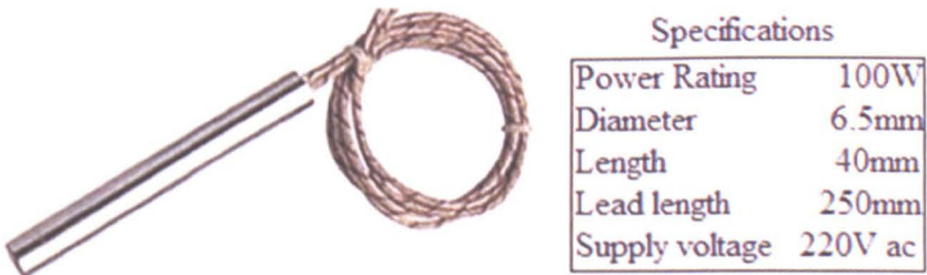
Figure 6-7 Photo and specifications of the electric heater
