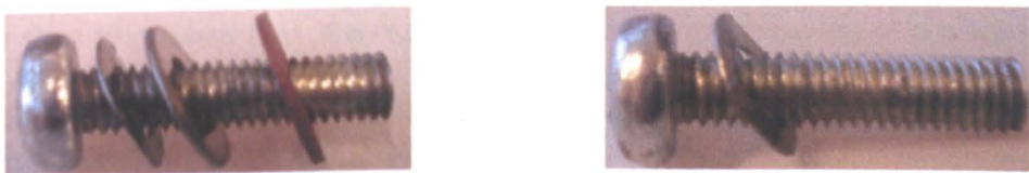
Figure 6-32 Washer configurations in the assembling procedure (from left to right, crinkle washer, flat metal washer and fibre washer)
