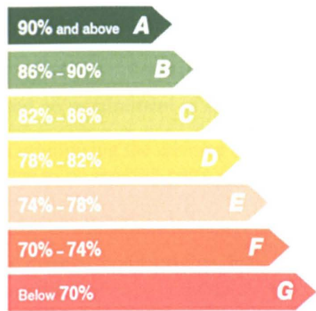
Figure 4-4 Rating chart of domestic boiler by SEDBUK
