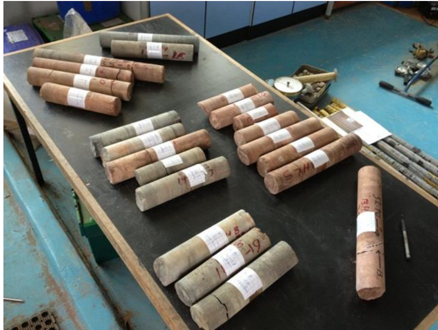
Figure 8.1 Core samples from Surqawshan Dam site
