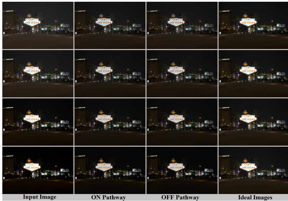
Figure 7.4: Without ON/OFF integration. Outputs from the ON and OFF pathways for the following contrast levels (from top to bottom): low, medium-low, medium-high, and high. The “ideal images” in the right-most column consist of pre-calibrated images with ideal scene contrast. At first glance, the model outputs in the ON and OFF pathways appear the same, and both achieve better contrast in low-contrast conditions. For the high-contrast case, it is difficult to note, by visual inspection alone, any changes in either the ON or OFF pathways. The images shown in this figure correspond to test case number 5 in the dataset.
