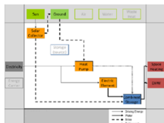
Figure 4.1.4 Solar heat pump system with an unspecified collector and a heat pump unit along with the condenser immersed in a combined storage tank. This system is designed for DHW preparation as well as space heating applications (Ruschenburg et al., 2013).
