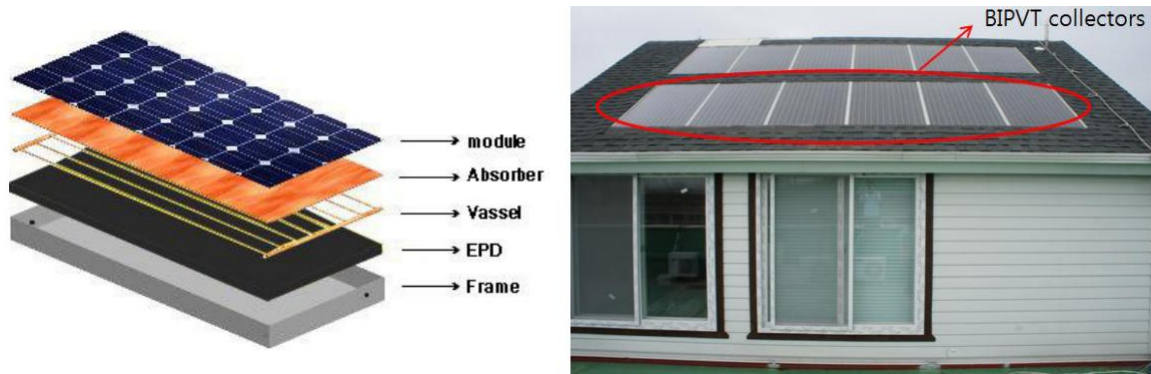
Figure 2.2.6 Conceptual and experimental view of the BiPVT/water unit (Kim et al., 2014)
