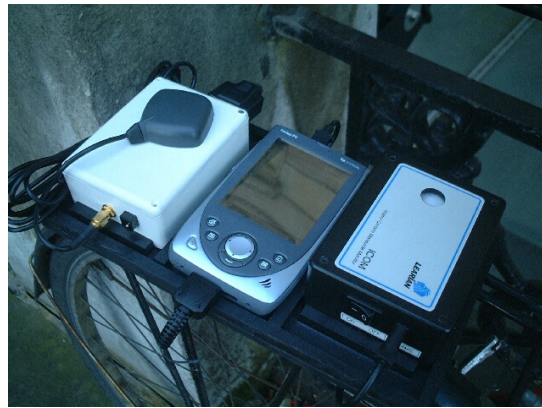
Figure 22: 'Tea-tray' CO Logger installed on a bike
