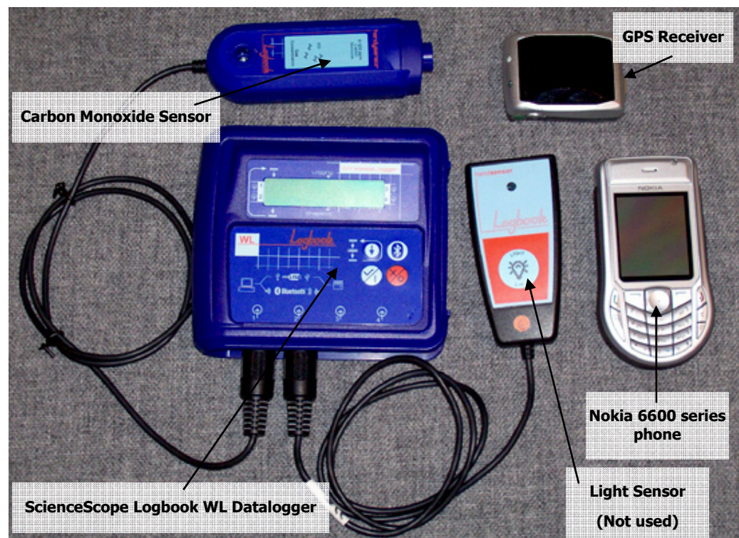
Figure 38: Phone, GPS and Logbook datalogger with sensor modules for light and Carbon Monoxide.
