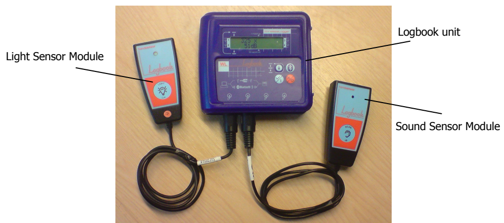
Figure 91: ScienceScope Logbook unit with two sensor modules
